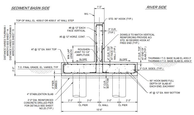
Graphic 6-1. Drawing of End Wall for Sediment Basin.
