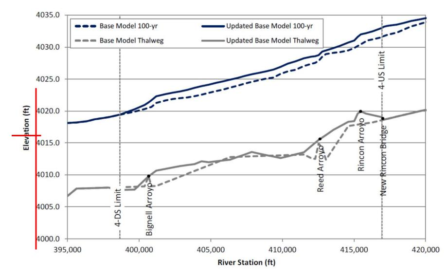
Figure B.4. Predicted water surface profiles from STA 3950+00 to 4200+00 (from Tetra Tech 2015)
