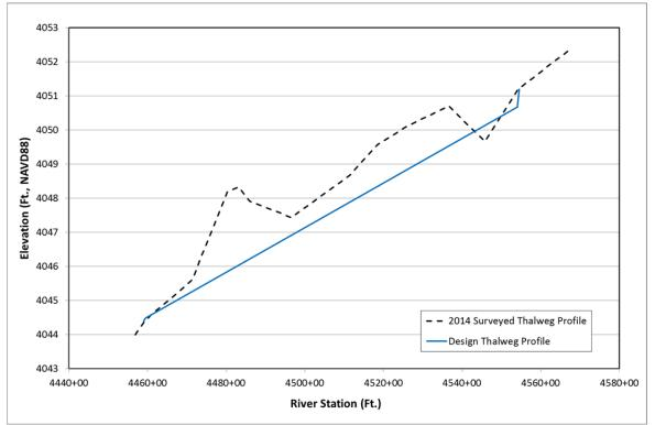
Figure 9-1. Pre-Sediment Removal Thalweg vs. Post-Sediment Removal Thalweg
