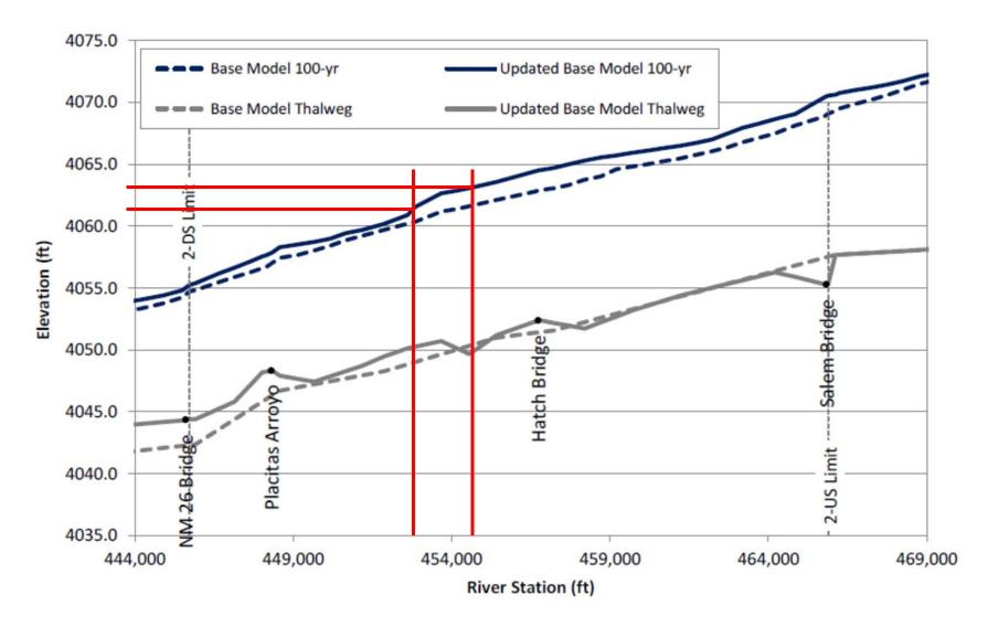
Figure B.6. Predicted water surface profiles from STA 4440+00 to 4690+00 (from Tetra Tech 2015)
