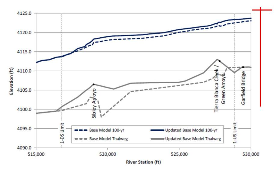
Figure B.7. Predicted water surface profiles from STA 5150+00 to 5300+00 (from Tetra Tech 2015)
