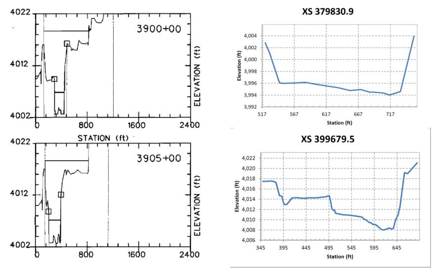
**Figure B.1. Rio Grande Cross-Sections near Rio Grande AT - Hayners Bridge Near Rincon River Gage.** (after USACE 1996 and Tetra Tech 2015)
