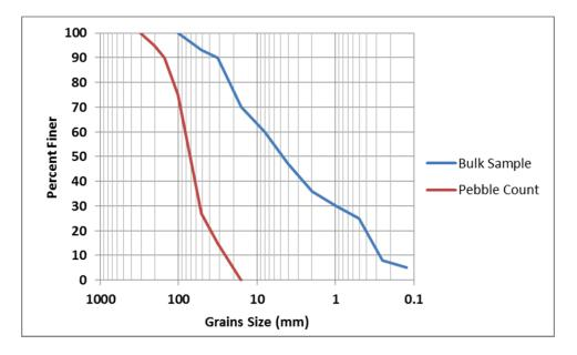
Figure A-10. Digitized Grain Size Curves for the Bulk Sample and Pebble Count Data Collected from Deposits in Problem Area 2
