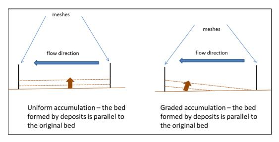
Figure A-15. Uniform and Sloped Filling Patterns.
