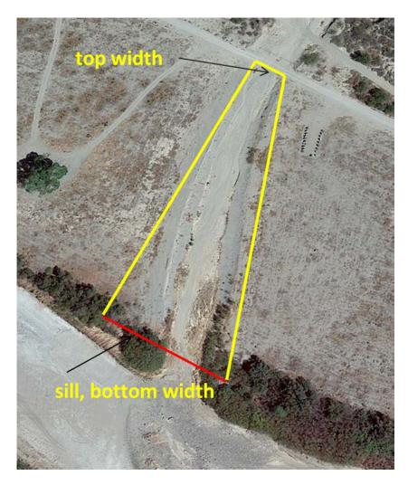
Figure A-18. Map View of Basin-Based Trap and Geometric Parameters (Sill, Top and Bottom Widths)
