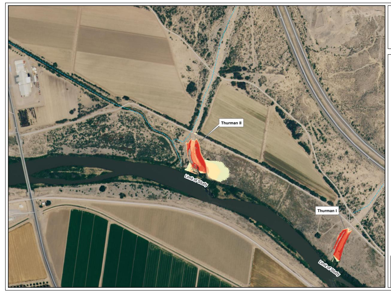
Figure A-23: THURMAN ARROYO I & II Comparison between 100-yr Flood Existing & Post-Project Conditions Inundation Extents
