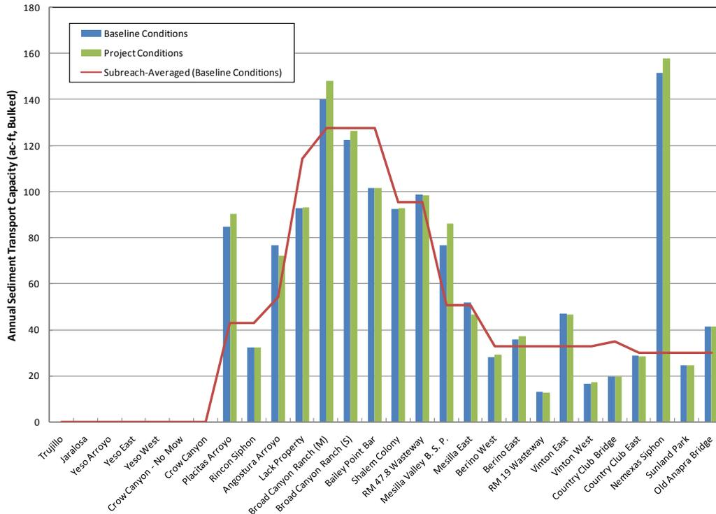
Figure 5.6. Comparison of the annual transport capacity at each of the restoration sites under baseline and project conditions. Also shown is the subreach-averaged annual transport capacity under baseline conditions.
