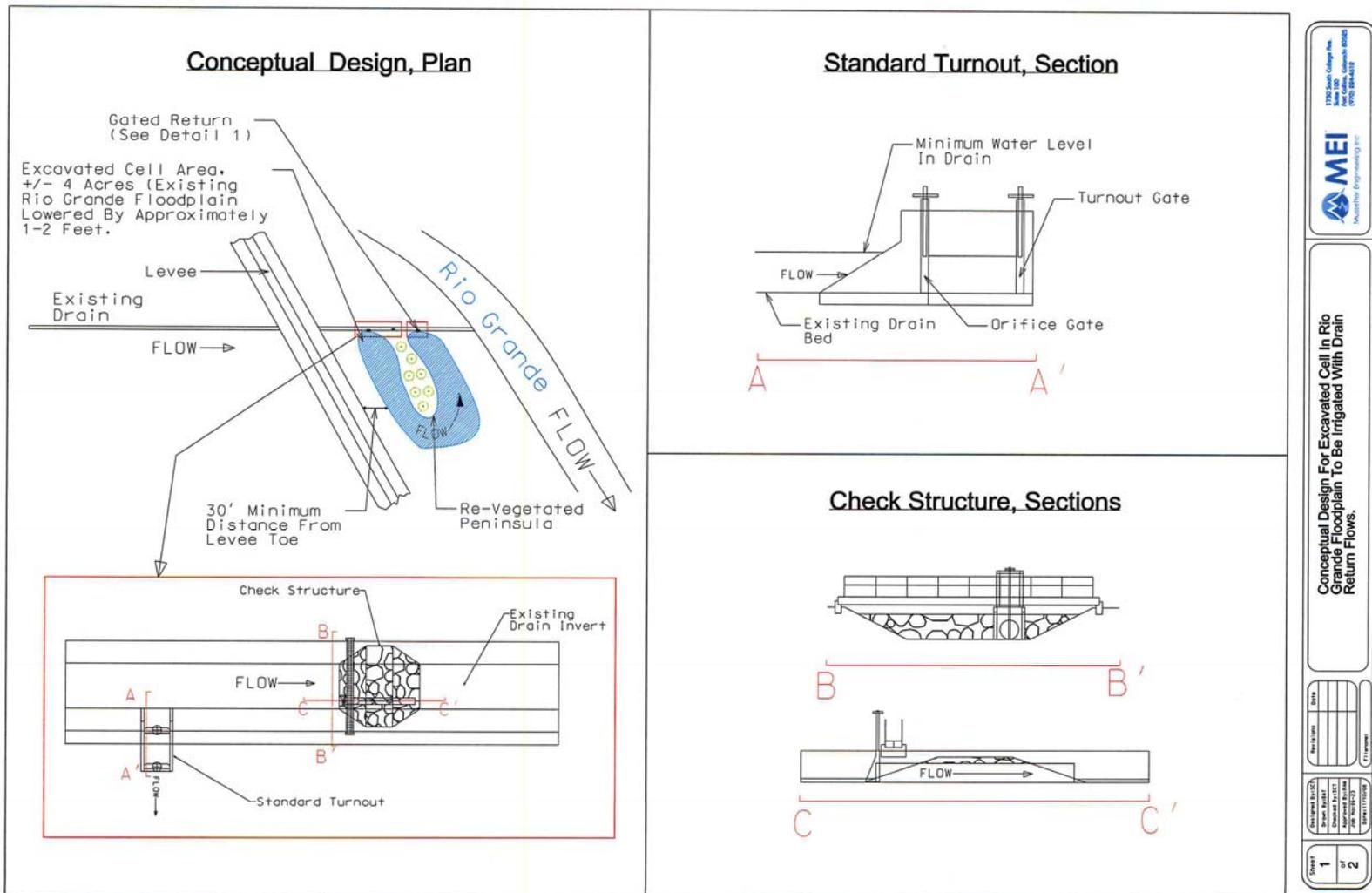
Figure 3.1. Conceptual design for check structure and turnout to provide overbank irrigation adjacent to irrigation wasteways and drains.
