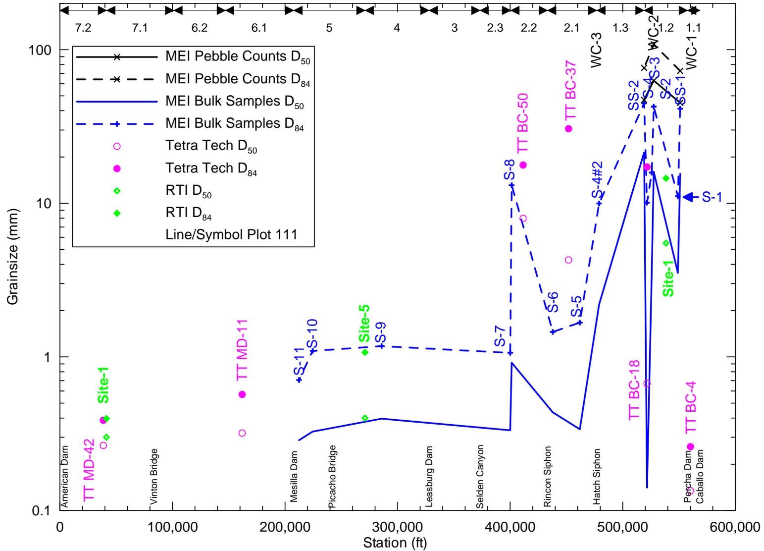
Figure 2.2. Longitudinal profile of  $D_{50}$  and  $D_{84}$  sediment sizes collected by MEI, Tetra Tech, and RTI.
