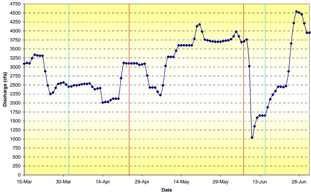
Figure 3.6. Recorded Caballo Dam releases during 1987. Highest target restoration flow was met; no augmentation is necessary.
