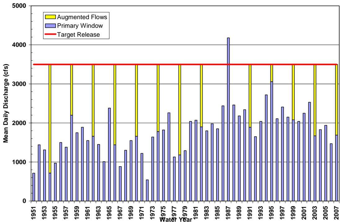
Figure 3.9. Maximum historical flow during the primary restoration release window and the flow augmentation required to meet the restoration objectives for a target release of 3,500 cfs.
