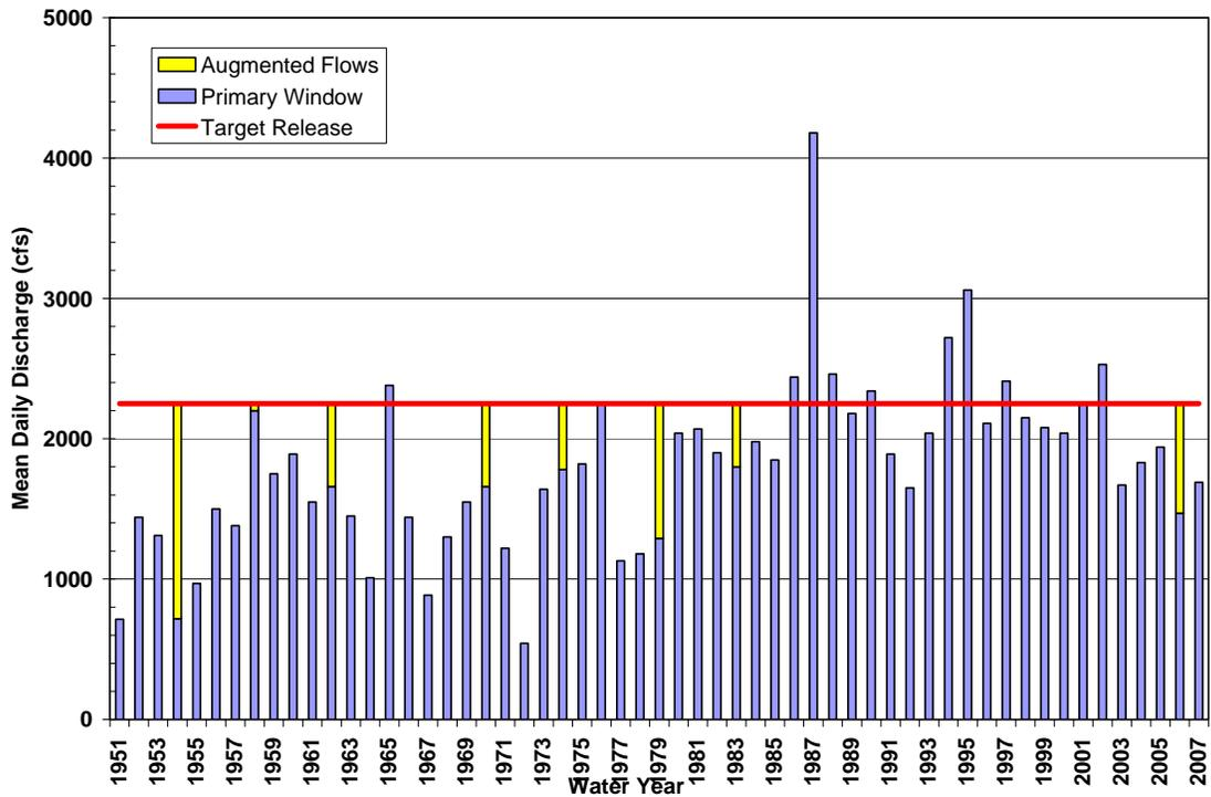
Figure 3.8. Maximum historical flow during the primary restoration release window and the flow augmentation required to meet the restoration objectives for a target release of 2,250 cfs.
