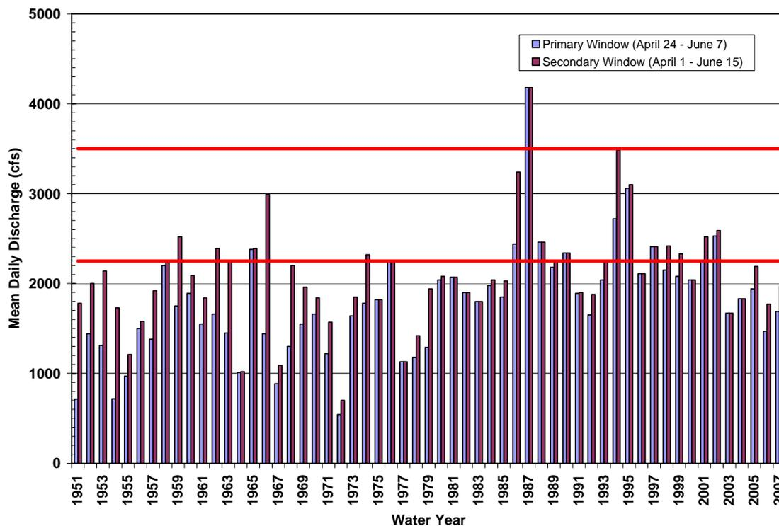
Figure 3.3. Maximum mean daily flow release from Caballo Dam in the primary and secondary target restoration release windows during the period from WY1951 through WY2007.
