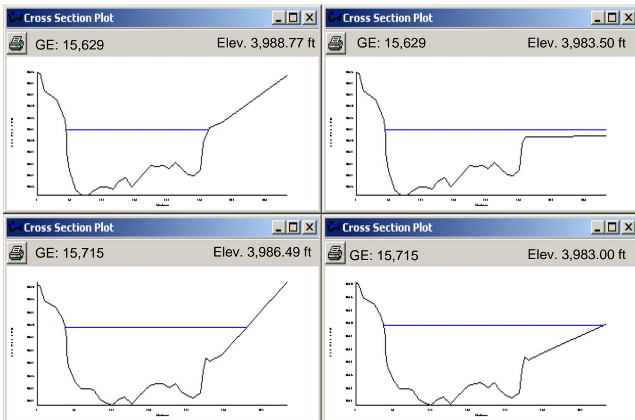
Figure 4.20. Baseline condition (left) and restored cross-section with lowered bank (right). The floodplain element elevations were adjusted to more accurately reflect the DTM data set and the proposed bankline lowering.
