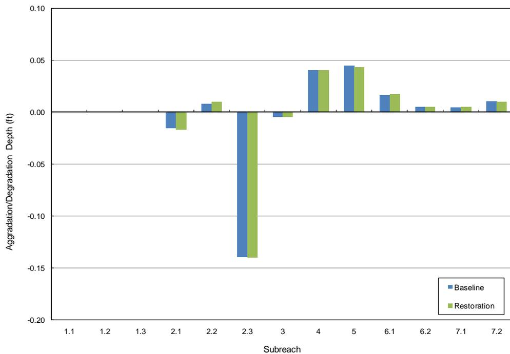
Figure 5.5. Comparison of computed average annual aggradation/degradation depths from the sediment-continuity analyses of baseline and restoration project conditions.
