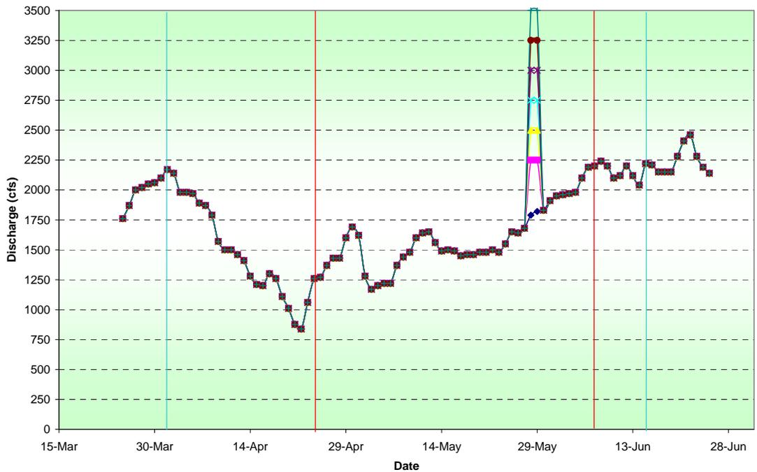
Figure 3.7. Recorded Caballo Dam releases during 1958. Wet year, in which augmentation is possible within the target period.
