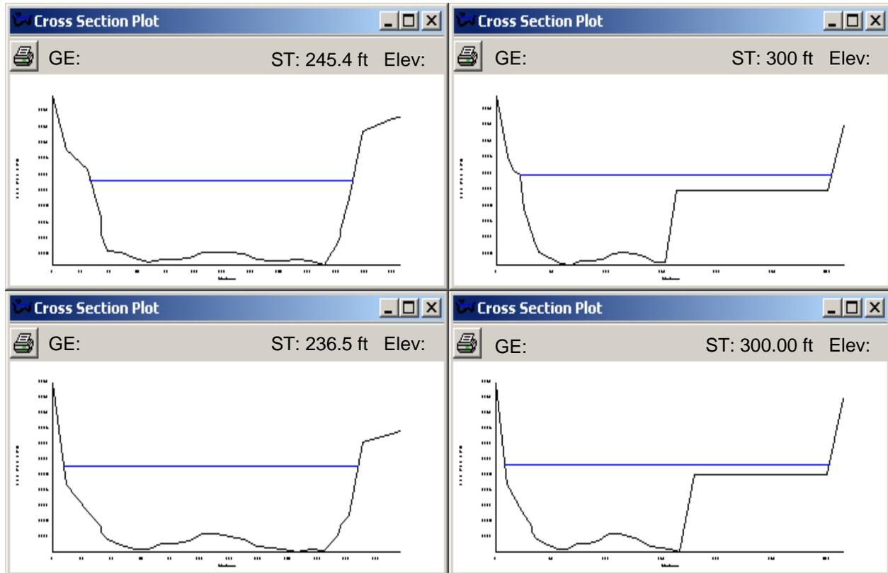
Figure 4.6. Existing (left) and restored (right) Inset floodplain cross sections.
