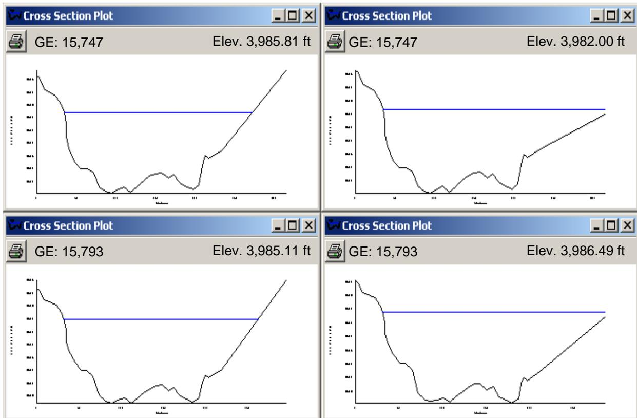
Figure 4.22. Baseline condition (left) and restored cross-section with lowered bank (right). The floodplain element elevations were adjusted to more accurately reflect the DTM data set and the proposed bankline lowering.
