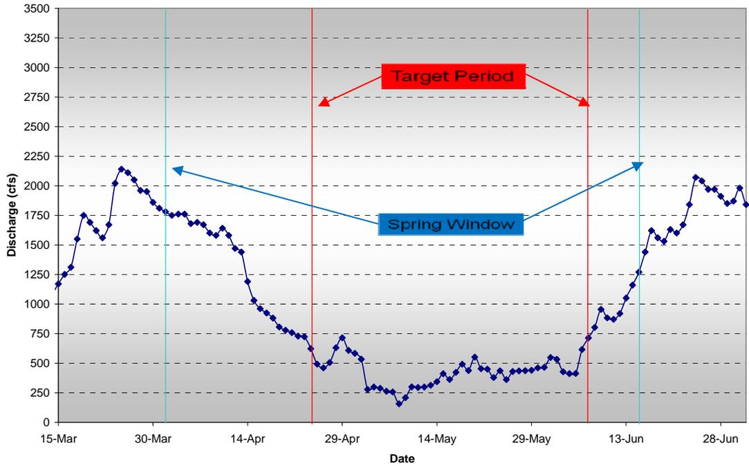
Figure 3.4. Recorded Caballo Dam releases during 1951. No augmentation is shown, but augmentation is possible within the spring window.
