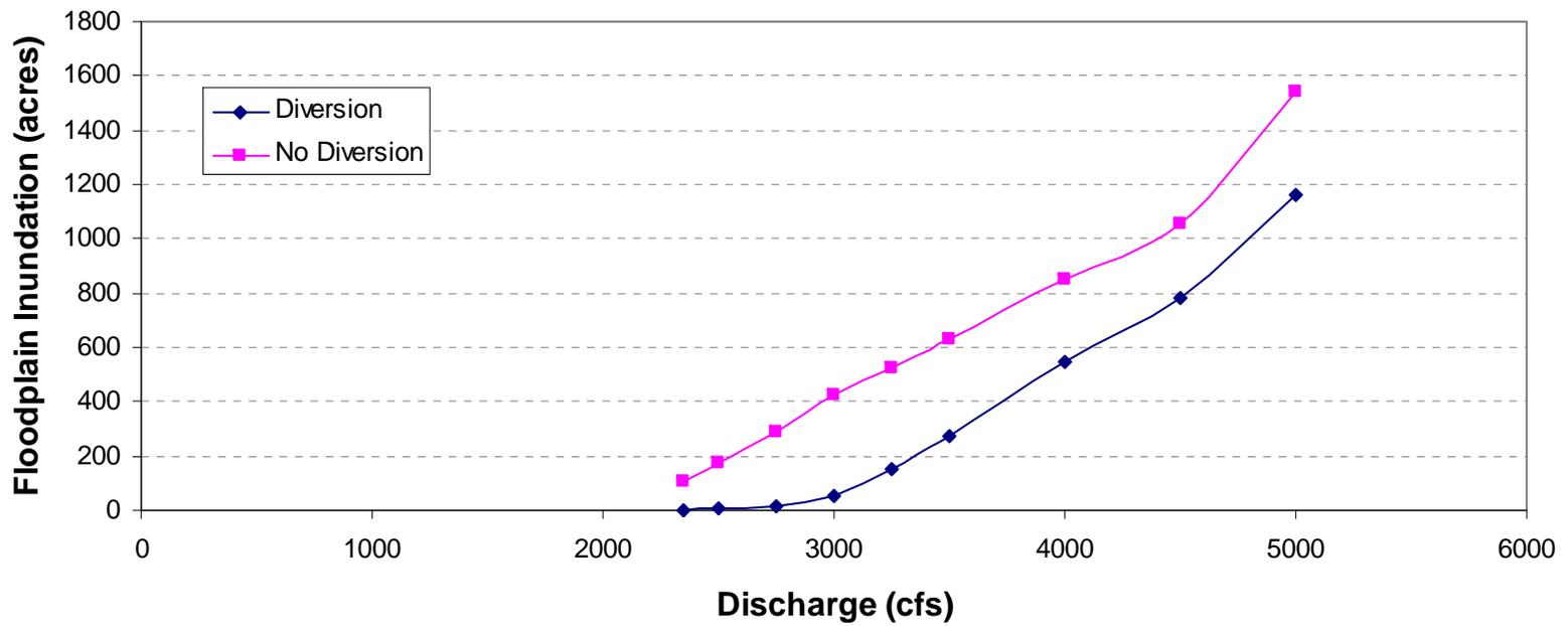
Figure 2.5. Predicted area of inundation for the range of potential restoration release with and without the diversion operating at their typical levels.
