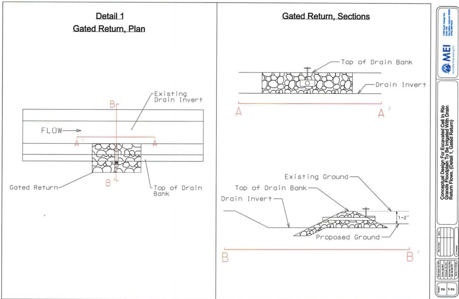
Figure 3.1. Conceptual design for check structure and turnout to provide overbank irrigation adjacent to irrigation wasteways and drains (continued).
