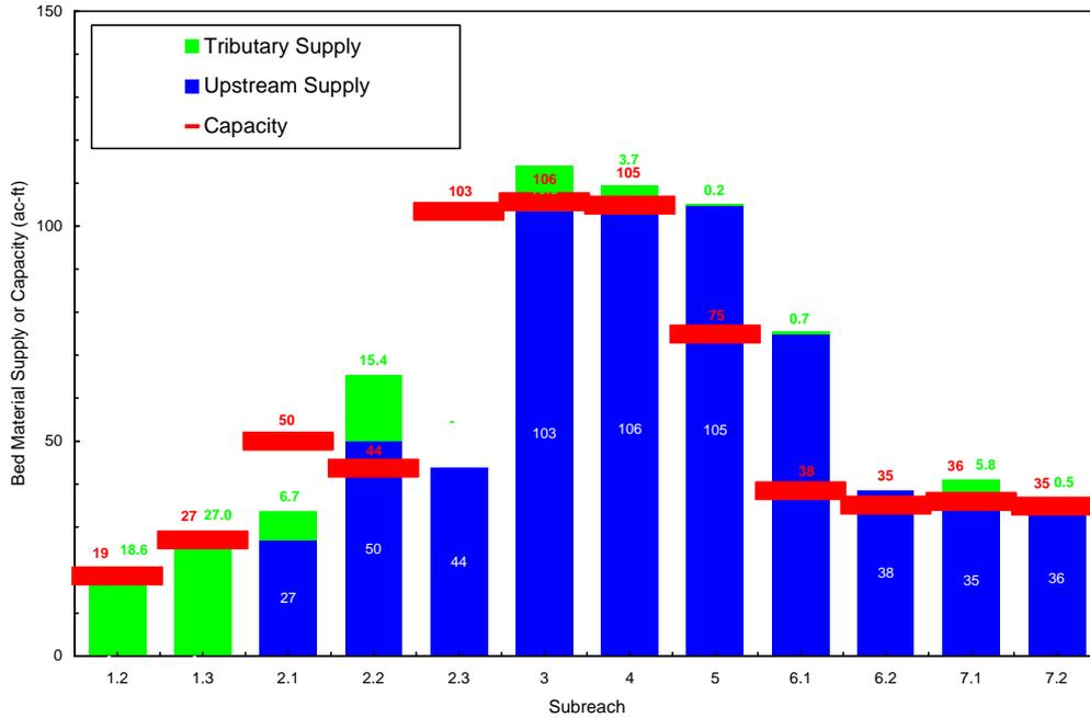
Figure 2.6. Comparison of average annual supply and bed-material transport capacity for each subreach.
