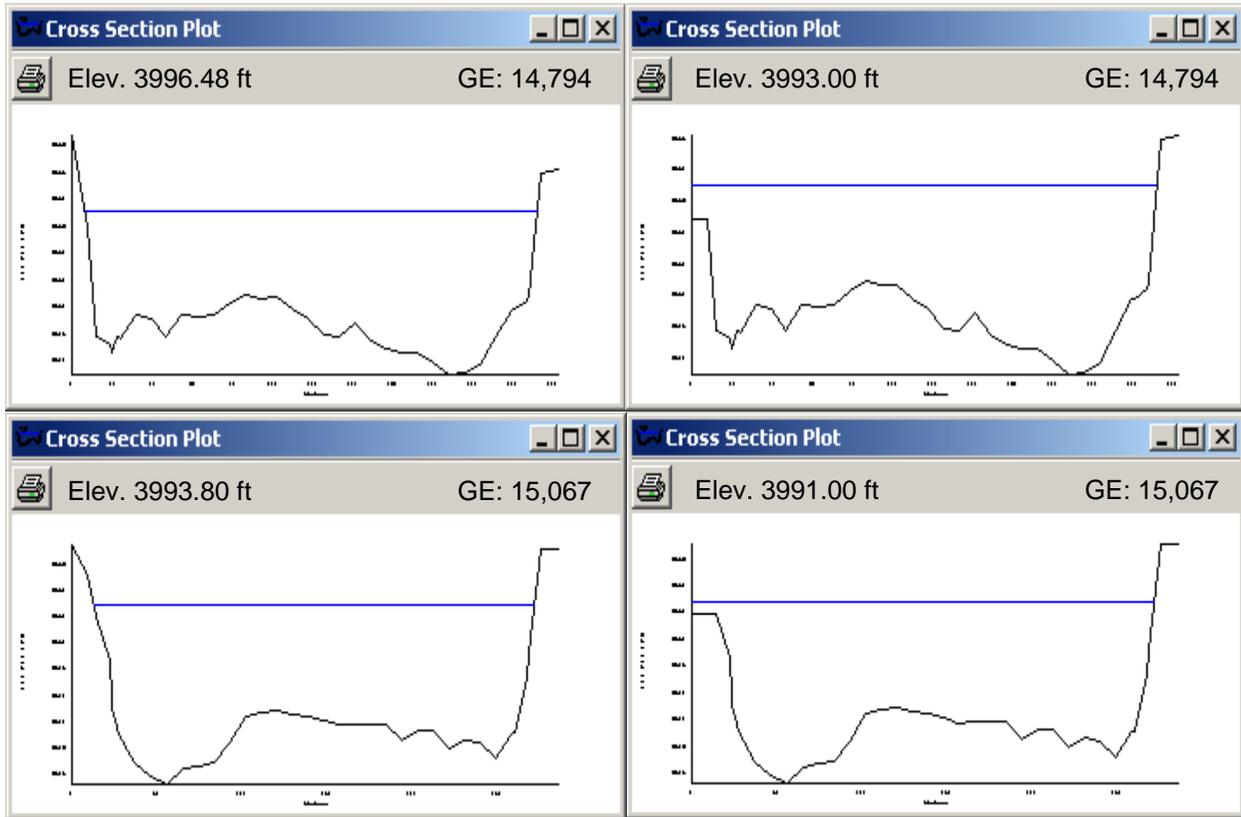
Figure 4.18. Baseline condition (left) and restored cross section with lowered bank (right).
