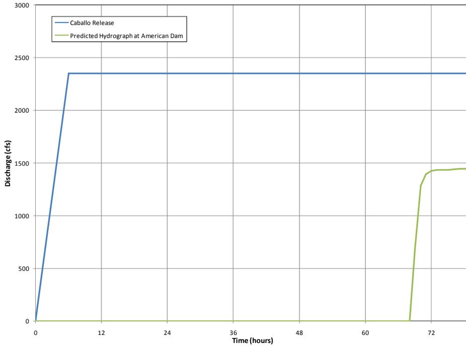
Figure 5.1. Modeled release hydrograph from Caballo Dam for the irrigation operational flow of 2,350 cfs and the predicted hydrograph at American Dam under restoration project conditions.
