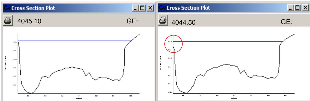
Figure 4.12. Before and after cross-section plot of river connection.
