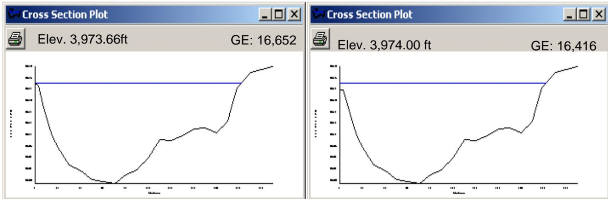
Figure 4.25. Baseline condition (left) and restored cross-section with lowered bank (right).
