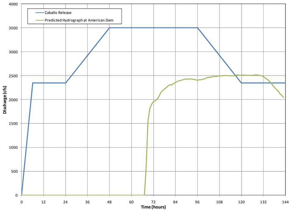
Figure 5.2. Modeled release hydrograph from Caballo Dam for the restoration flow of 3,500 cfs and the predicted hydrograph at American Dam under restoration project conditions.
