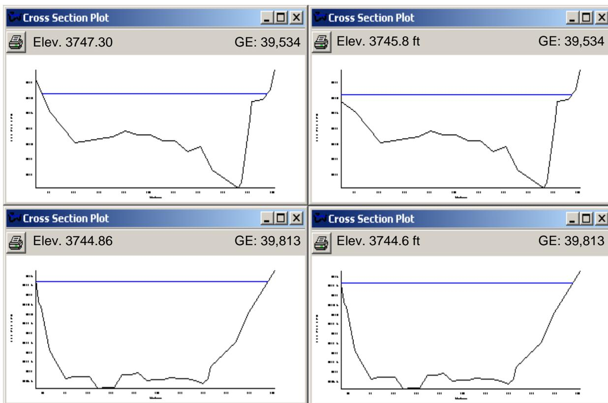
Figure 4.39. Baseline condition (left) and restored cross-section with lowered bank (right).
