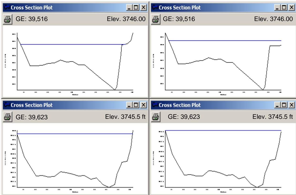
Figure 4.37. Baseline condition (left) and restored cross section with lowered bank (right).
