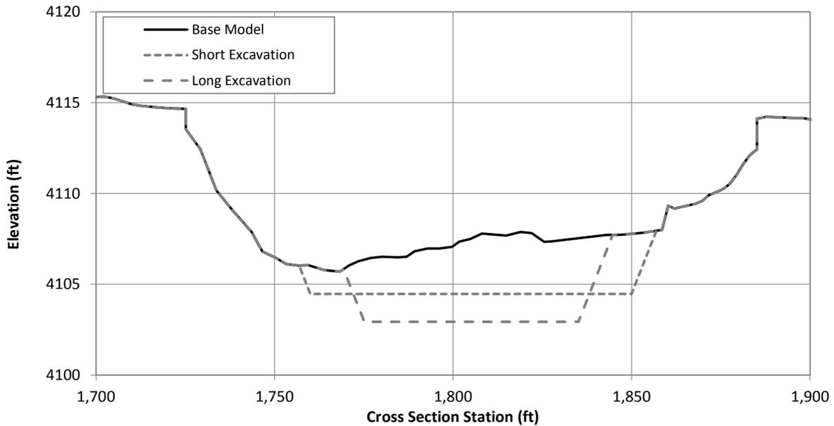
Figure G.1.5. Typical cross section at Problem Location 1 showing the existing (Base Model) channel geometry and excavated geometry under the short and long excavation scenarios (River Station 518772.4).
