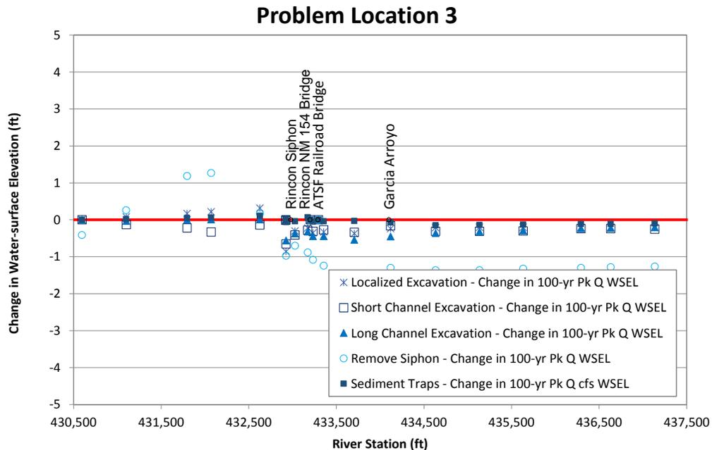
Figure N.12. Predicted change in long-term water-surface elevation at the 100-year peak flow relative to the base condition at Problem Location 3 for the alternatives that were evaluated with the steady-state hydraulic model compared to existing (base model) conditions.
