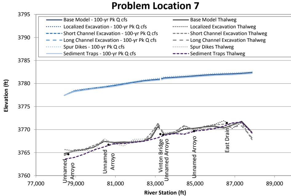
Figure N.27. Predicted water-surface profiles at the 100-year peak flow at Problem Location 7 representing long-term conditions based on hydraulic modeling with the predicted geometry at the end of the sediment-transport simulations of the base and alternative conditions.
