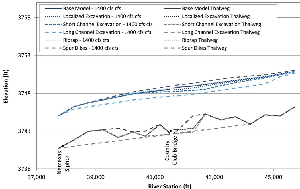
Figure L.57. Predicted water-surface profiles at 1,400 cfs at Problem Location 8 under existing (base model) conditions and for the alternatives that were evaluated with the steady-state hydraulic model.
