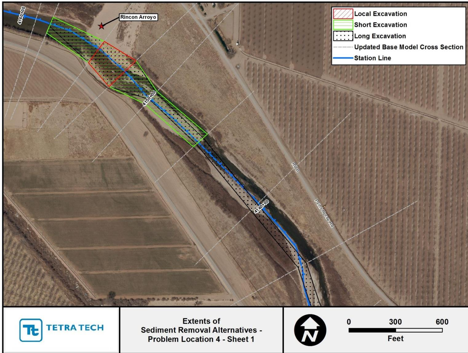
Figure G.2.9. Mapping showing extents of the localized, short and long sediment-removal alternatives at Problem Location 4 (Sheet 1).
