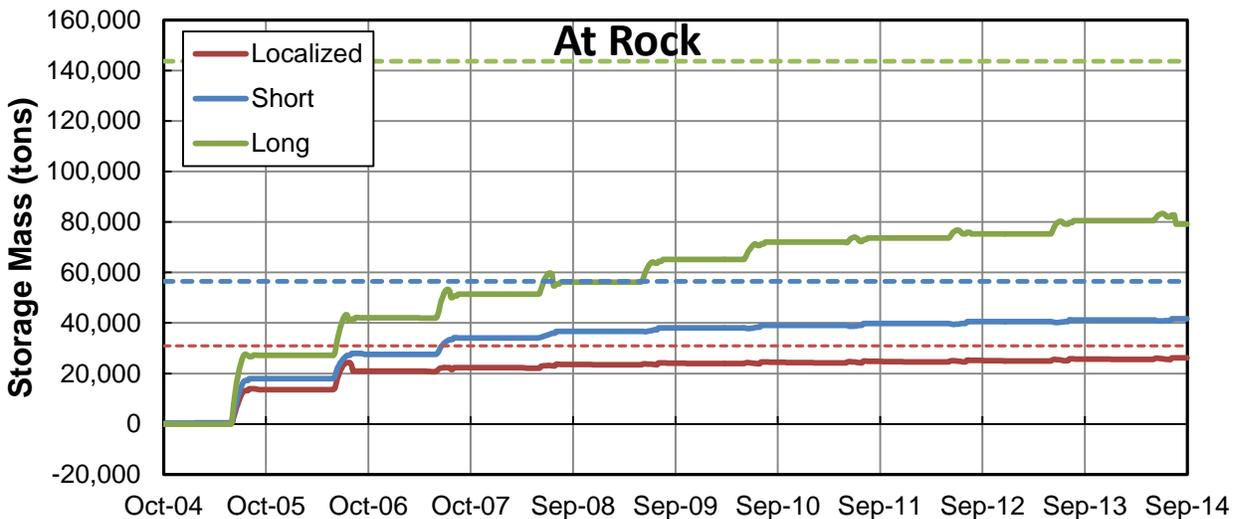
Figure M.2.28. Predicted cumulative mass of aggradation or degradation over time along the extents of the excavated reaches at Rock Canyon (Problem Location 5) from the sediment-transport simulations of the sediment-removal alternatives. The dashed lines represent the excavated mass for each type of excavation.
