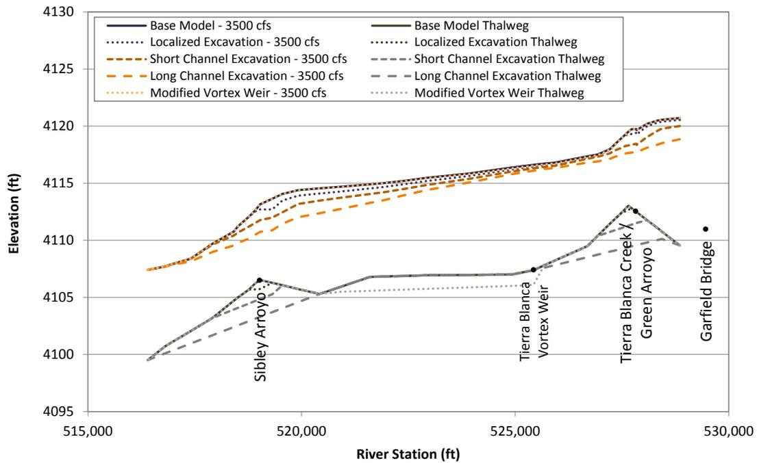
Figure L.5. Predicted water-surface profiles at 3,500 cfs at Problem Location 1 under existing (base model) conditions and for the alternatives that were evaluated with the steady-state hydraulic model.
