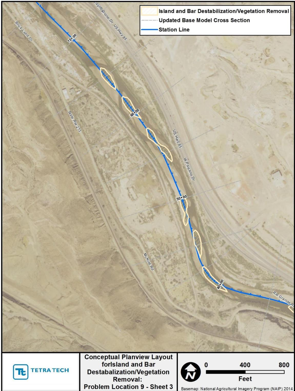
Figure J.14. Aerial photography showing extents of features treated with island/bar destabilization and vegetation removal at Problem Location 9 (Sheet 3).
