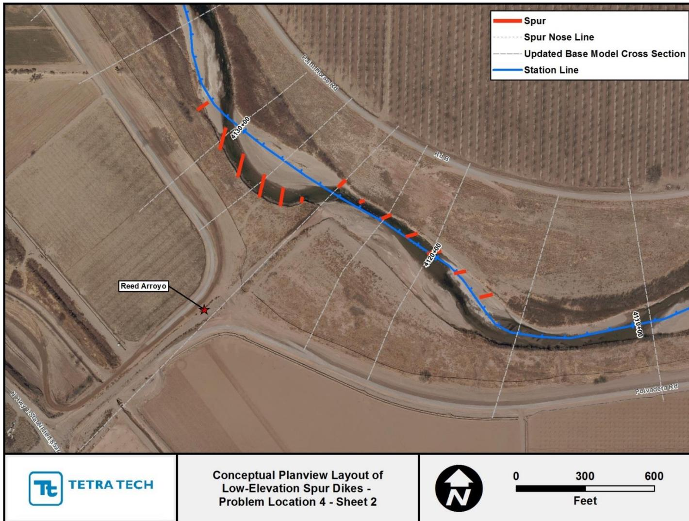
Figure I.2. Conceptual layout of low-elevation spur dikes at Problem Location 4 (Sheet 2).
