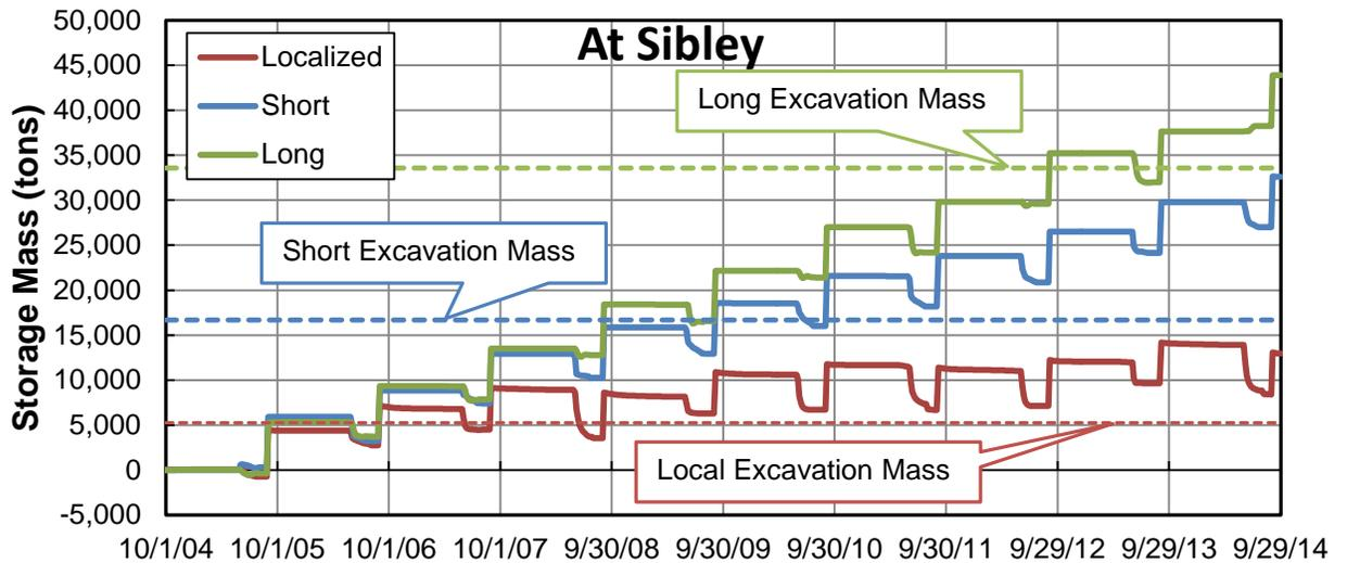
Figure M.2.20. Predicted cumulative mass of aggradation or degradation over time along the extents of the excavated reaches at Sibley Arroyo (Problem Location 1) from the sediment-transport simulations of the sediment-removal alternatives. The dashed lines represent the excavated mass for each type of excavation.
