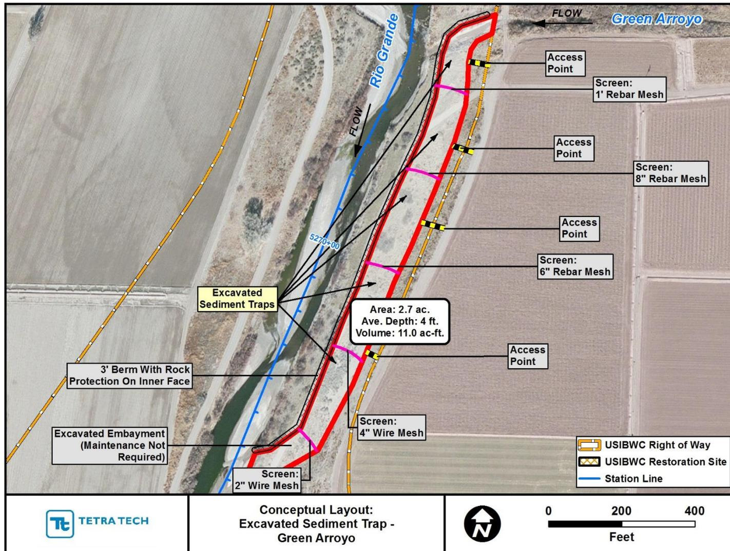
Figure H.2. Conceptual layout of sediment trap for Green Arroyo at Problem Location 1.
