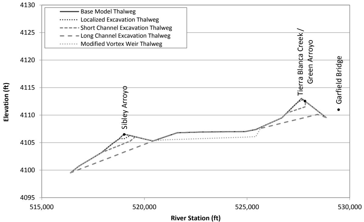
Figure G.1.1. Existing (Base Model) and excavation thalweg profiles at Problem Location 1.
