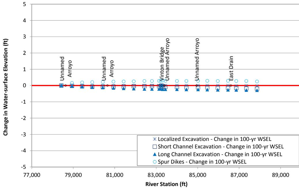
Figure L.56. Predicted change in water-surface elevation at the routed 100-year peak flow at Problem Location 7 for the alternatives that were evaluated with the steady-state hydraulic model compared to existing (base model) conditions.
