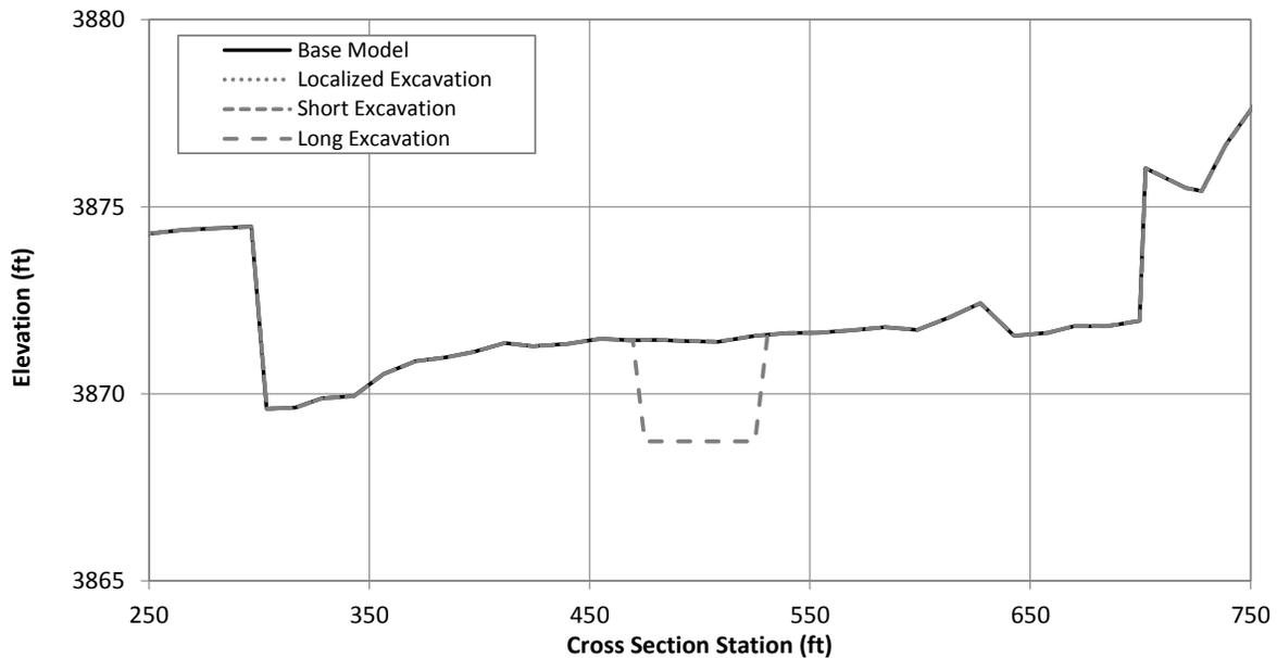
Figure G.1.26. Typical cross section at Problem Location 6 showing the existing (Base Model) channel geometry and excavated geometry under the localized, short and long excavation scenarios (River Station 215011.7).
