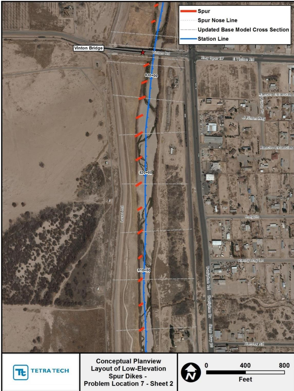
Figure I.7. Conceptual layout of low-elevation spur dikes at Problem Location 7 (Sheet 2).
