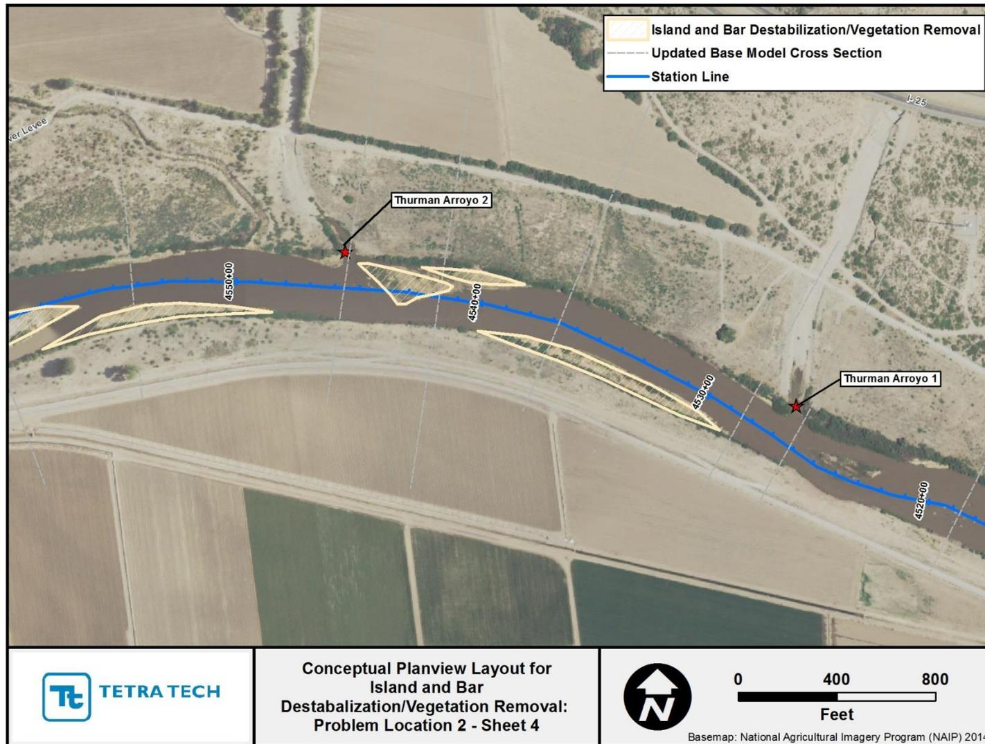
Figure J.4. Aerial photography showing extents of features treated with island/bar destabilization and vegetation removal at Problem Location 2 (Sheet 4).
