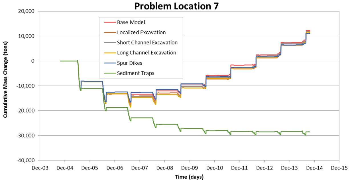
Figure M.2.7. Predicted cumulative mass of aggradation or degradation over time along the modeled reach at Problem Location 7 from the sediment-transport simulations of the base and alternative conditions.
