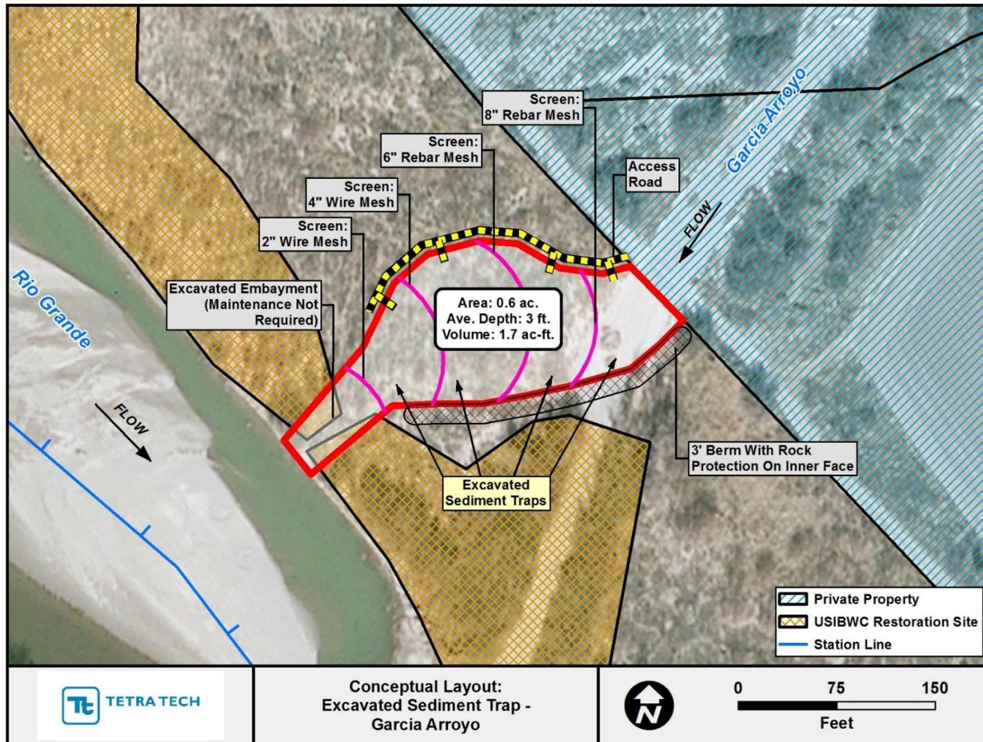
Figure H.7. Conceptual layout of sediment trap for Garcia Arroyo at Problem Location 3.
