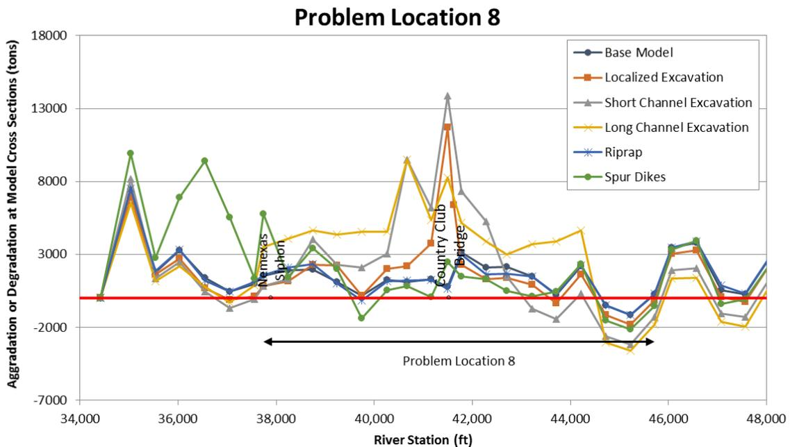
Figure M.1.8. Spatial profiles showing the predicted cumulative mass of aggradation or degradation at the end of the sediment-transport simulations for base alternative conditions at Problem Location 8.
