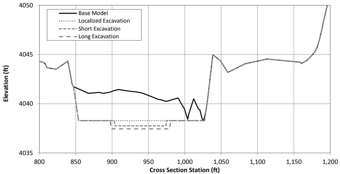
Figure G.1.12. Typical cross section at Problem Location 3 showing the existing (Base Model) channel geometry and excavated geometry under the localized, short and long excavation scenarios (River Station 434118.9).
