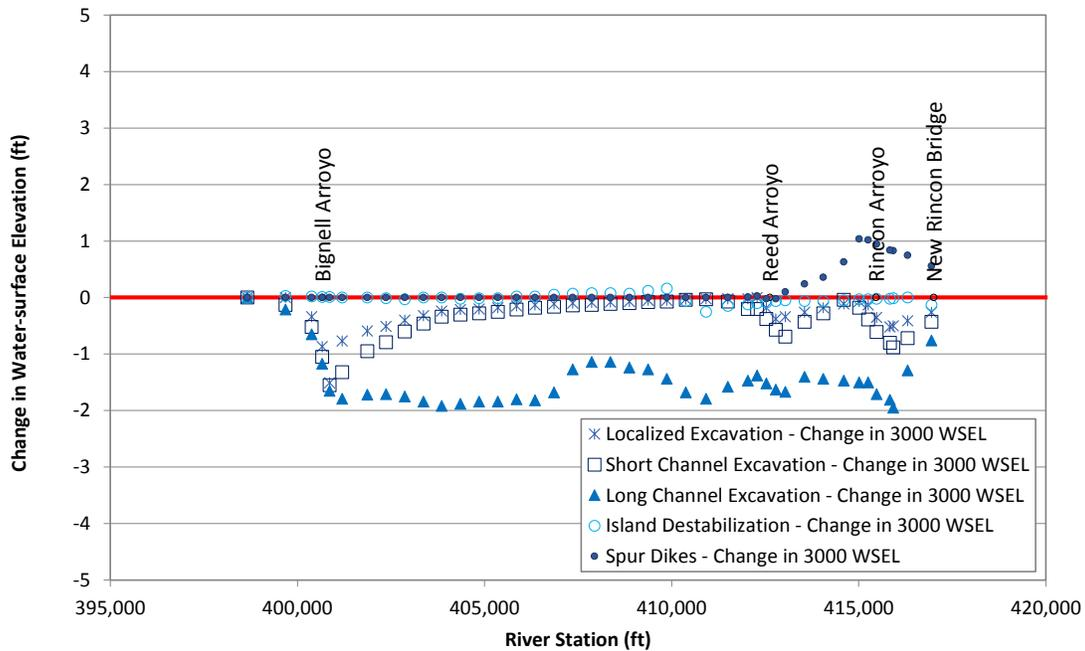
Figure L.28. Predicted change in water-surface elevation at 3,000 cfs at Problem Location 4 for the alternatives that were evaluated with the steady-state hydraulic model compared to existing (base model) conditions.
