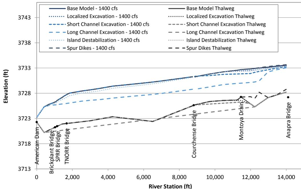
Figure L.65. Predicted water-surface profiles at 1,400 cfs at Problem Location 9 under existing (base model) conditions and for the alternatives that were evaluated with the steady-state hydraulic model.
