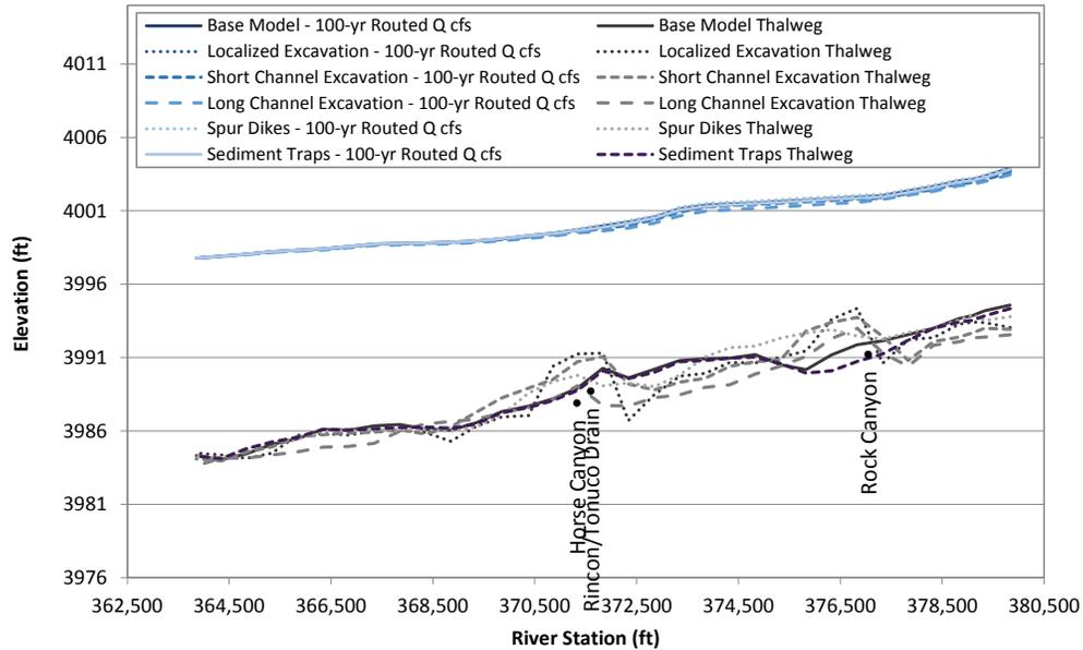
Figure N.19. Predicted water-surface profiles at the 100-year peak flow at Problem Location 5 representing long-term conditions based on hydraulic modeling with the predicted geometry at the end of the sediment-transport simulations of the base and alternative conditions.
