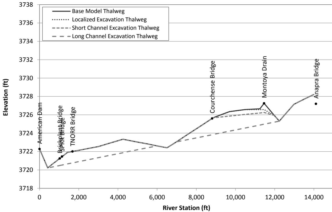
Figure G.1.37. Existing (Base Model) and excavation thalweg profiles at Problem Location 9.
