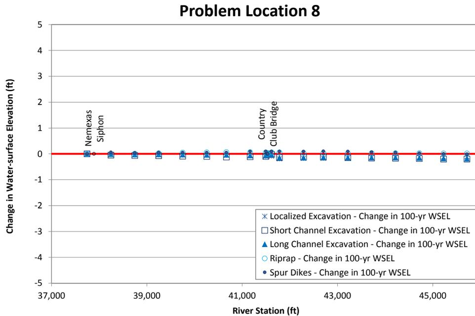
Figure N.32. Predicted change in long-term water-surface elevation at the 100-year peak flow relative to the base condition at Problem Location 8 for the alternatives that were evaluated with the steady-state hydraulic model compared to existing (base model) conditions.
