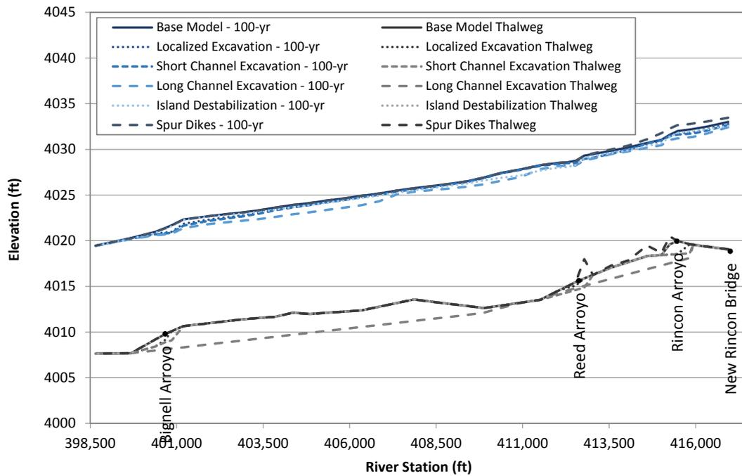
Figure L.31. Predicted water-surface profiles at the routed 100-year peak flow at Problem Location 4 under existing (base model) conditions and for the alternatives that were evaluated with the steady-state hydraulic model.
