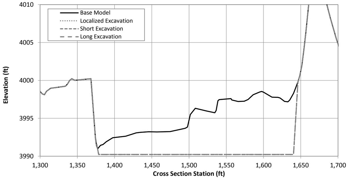
Figure G.1.21. Typical cross section at Problem Location 5 showing the existing (Base Model) channel geometry and excavated geometry under the localized, short and long excavation scenarios (River Station 376830.4).
