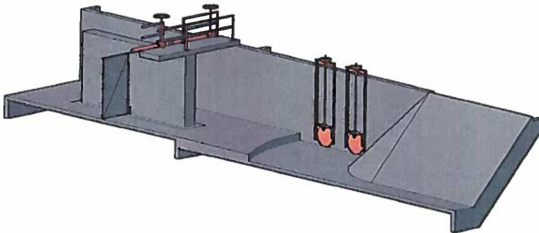
Figure 4. Section view of proposed Eastside Canal new first check
