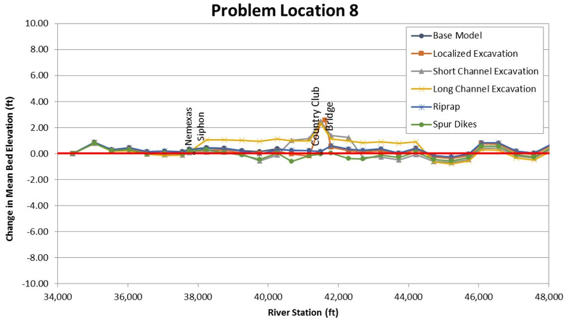
Figure M.1.17. Spatial profiles showing the predicted change in mean bed elevation at the end of the sediment-transport simulations for base alternative conditions at Problem Location 8.
