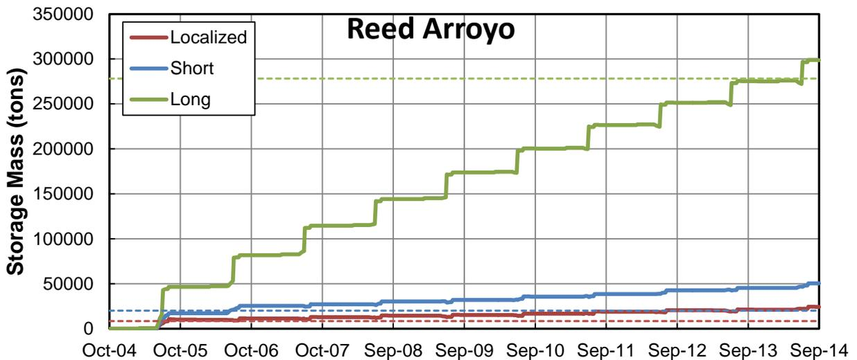
Figure M.2.26. Predicted cumulative mass of aggradation or degradation over time along the extents of the excavated reaches at Reed Arroyo (Problem Location 4) from the sediment-transport simulations of the sediment-removal alternatives. The dashed lines represent the excavated mass for each type of excavation.
