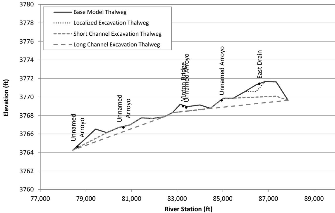
Figure G.1.29. Existing (Base Model) and excavation thalweg profiles at Problem Location 7.
