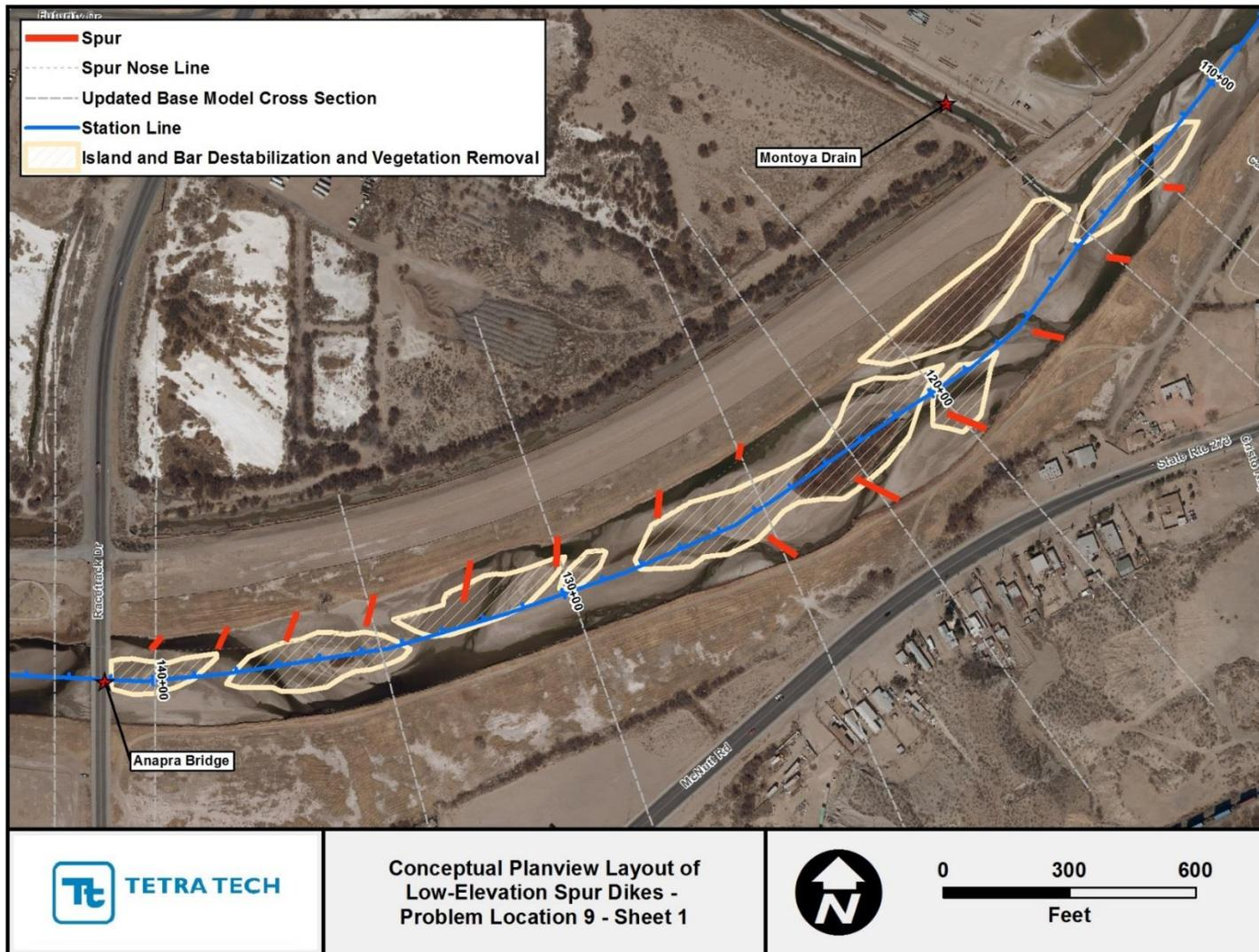
Figure I.11. Conceptual layout of low-elevation spur dikes at Problem Location 9.
