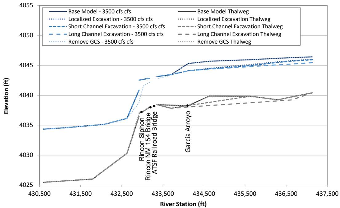
Figure L.21. Predicted water-surface profiles at 3,500 cfs at Problem Location 3 under existing (base model) conditions and for the alternatives that were evaluated with the steady-state hydraulic model.
