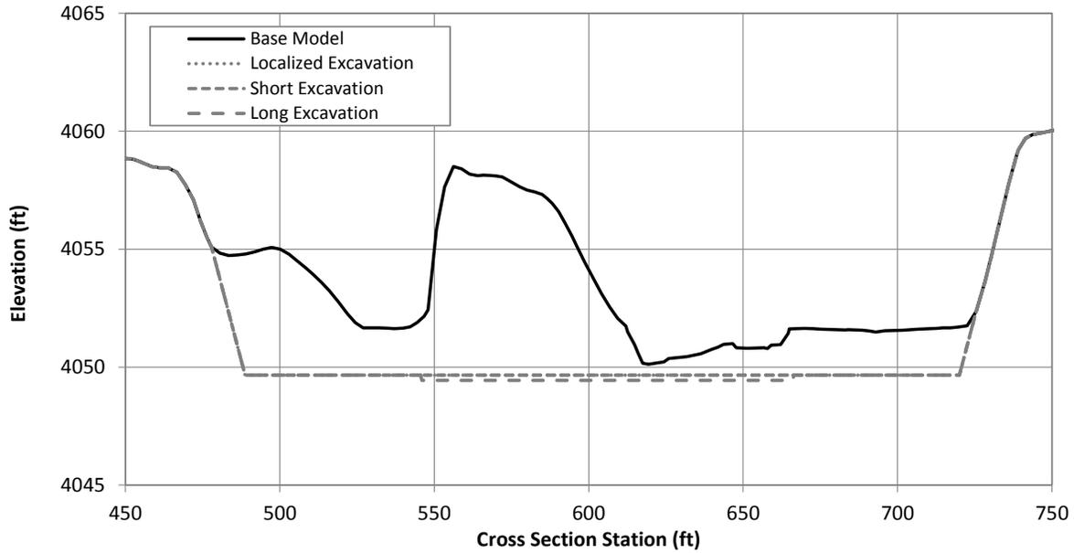
Figure G.1.7. Typical cross section at Problem Location 2 showing the existing (Base Model) channel geometry and excavated geometry under the localized, short and long excavation scenarios (River Station 454174.4).
