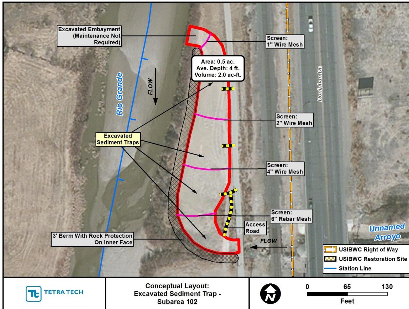
Figure H.11. Conceptual layout of sediment trap for the unnamed arroyo draining Subarea 102 at Problem Location 7.
