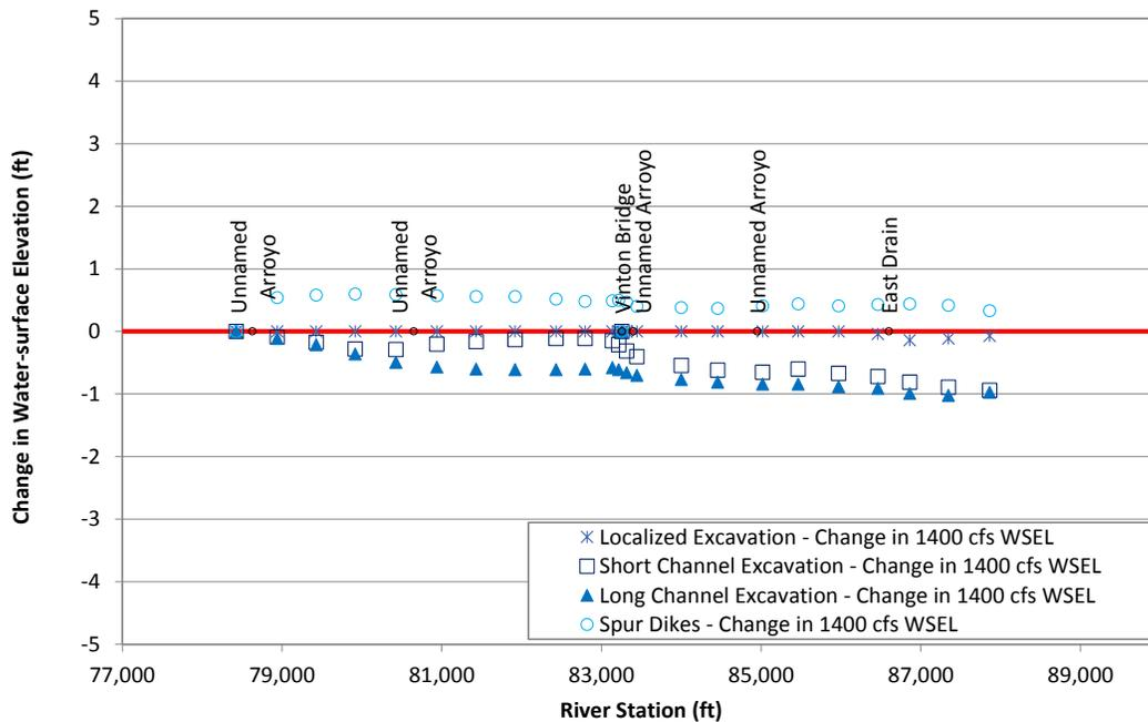
Figure L.50. Predicted change in water-surface elevation at 1,400 cfs at Problem Location 7 for the alternatives that were evaluated with the steady-state hydraulic model compared to existing (base model) conditions.
