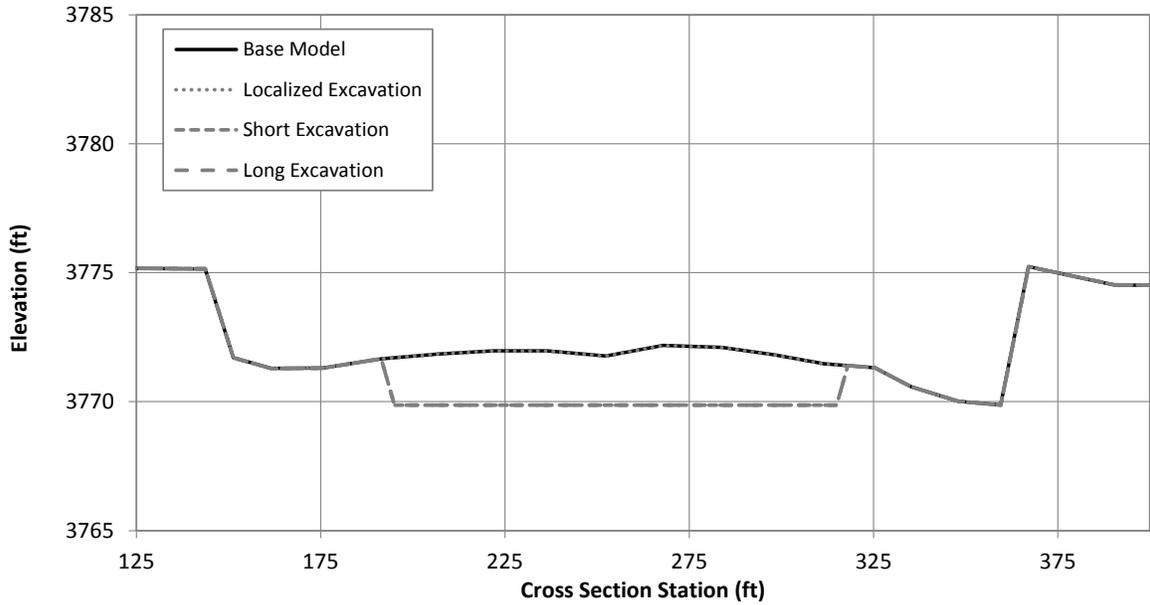
Figure G.1.31. Typical cross section at Problem Location 7 showing the existing (Base Model) channel geometry and excavated geometry under the localized, short and long excavation scenarios (River Station 85464.6).
