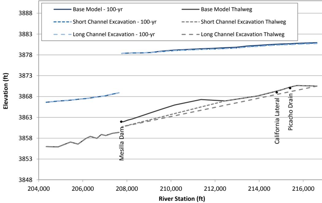
Figure L.47. Predicted water-surface profiles at the routed 100-year peak flow at Problem Location 6 under existing (base model) conditions and for the alternatives that were evaluated with the steady-state hydraulic model.
