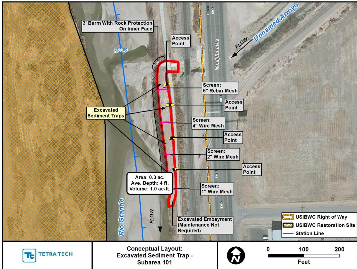
Figure H.10. Conceptual layout of sediment trap for the unnamed arroyo draining Subarea 101 at Problem Location 7.
