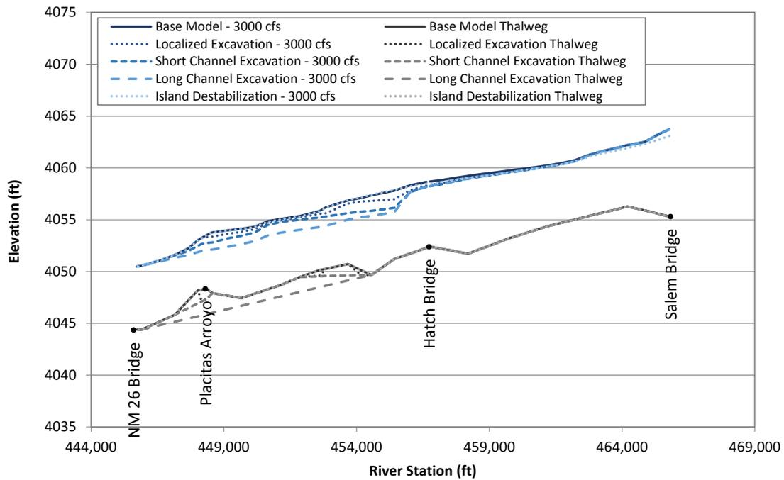
Figure L.11. Predicted water-surface profiles at 3,000 cfs at Problem Location 2 under existing (base model) conditions and for the alternatives that were evaluated with the steady-state hydraulic model.
