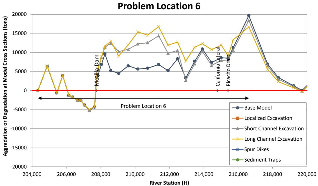
Figure M.1.6. Spatial profiles showing the predicted cumulative mass of aggradation or degradation at the end of the sediment-transport simulations for base alternative conditions at Problem Location 6.
