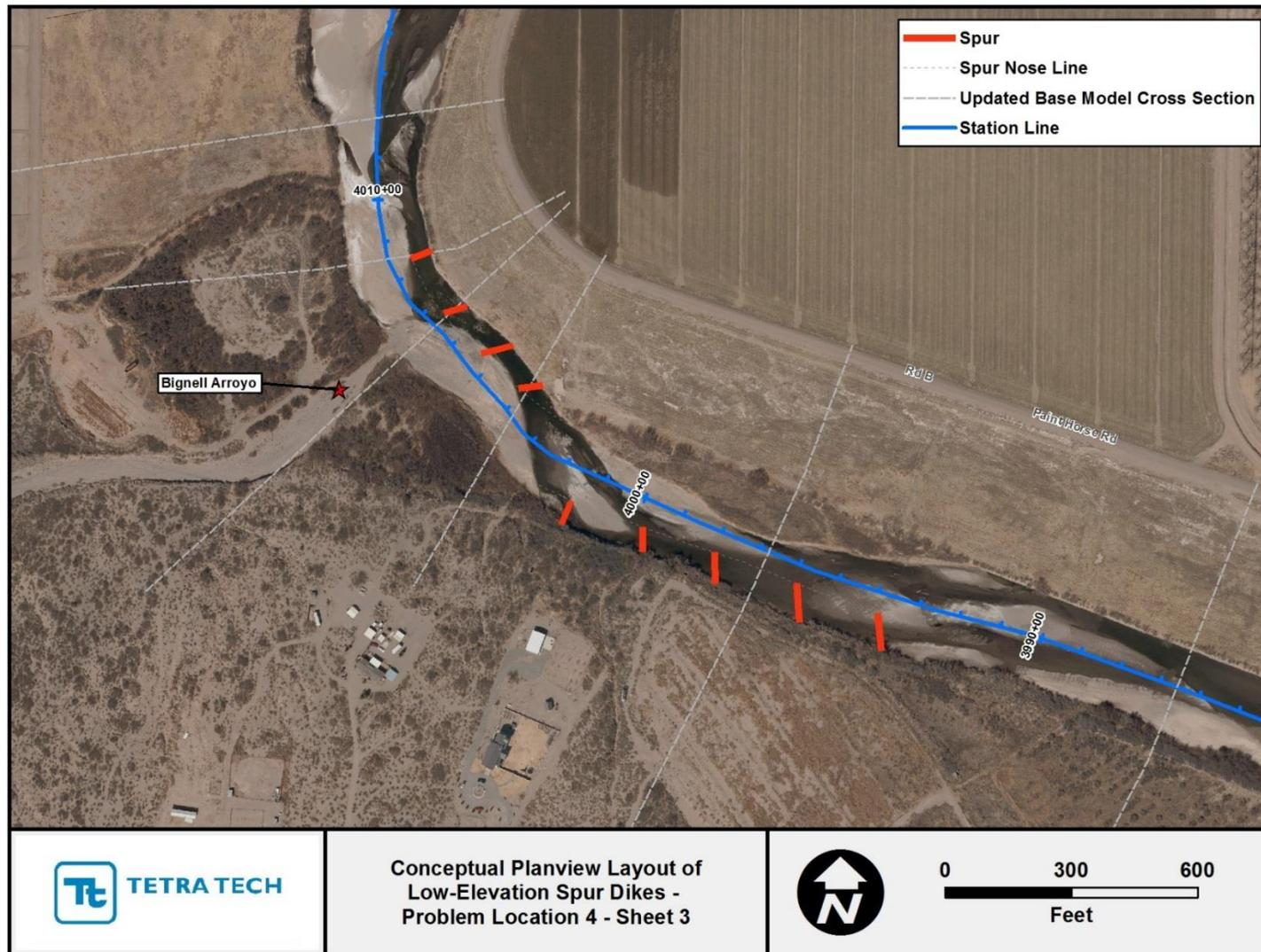
Figure I.3. Conceptual layout of low-elevation spur dikes at Problem Location 4 (Sheet 3).
