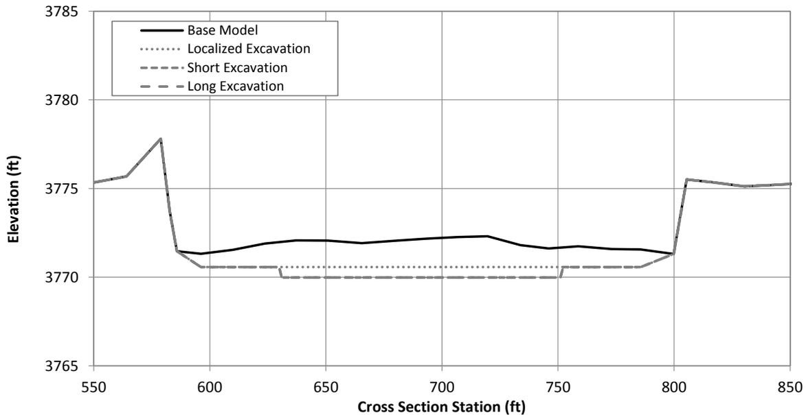
Figure G.1.30. Typical cross section at Problem Location 7 showing the existing (Base Model) channel geometry and excavated geometry under the localized, short and long excavation scenarios (River Station 86460).
