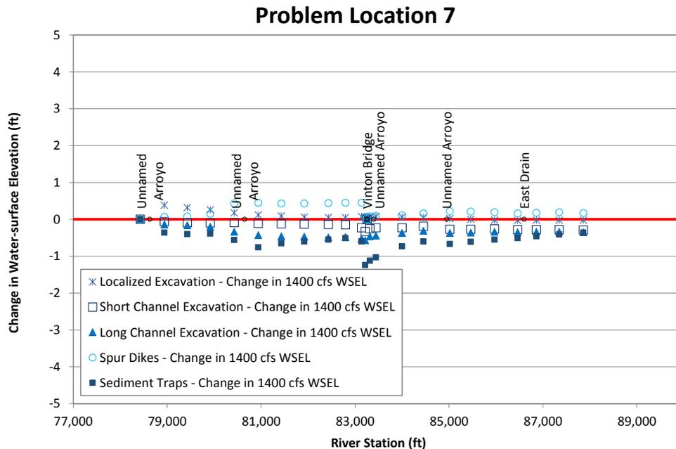
Figure N.26. Predicted change in long-term water-surface elevation at 1,400 cfs relative to the base condition at Problem Location 7 for the alternatives that were evaluated with the steady-state hydraulic model compared to existing (base model) conditions.
