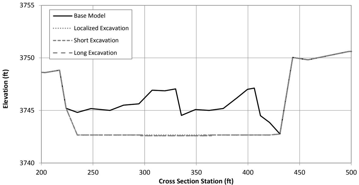
Figure G.1.35. Typical cross section at Problem Location 8 showing the existing (Base Model) channel geometry and excavated geometry under the localized, short and long excavation scenarios (River Station 41495.8).
