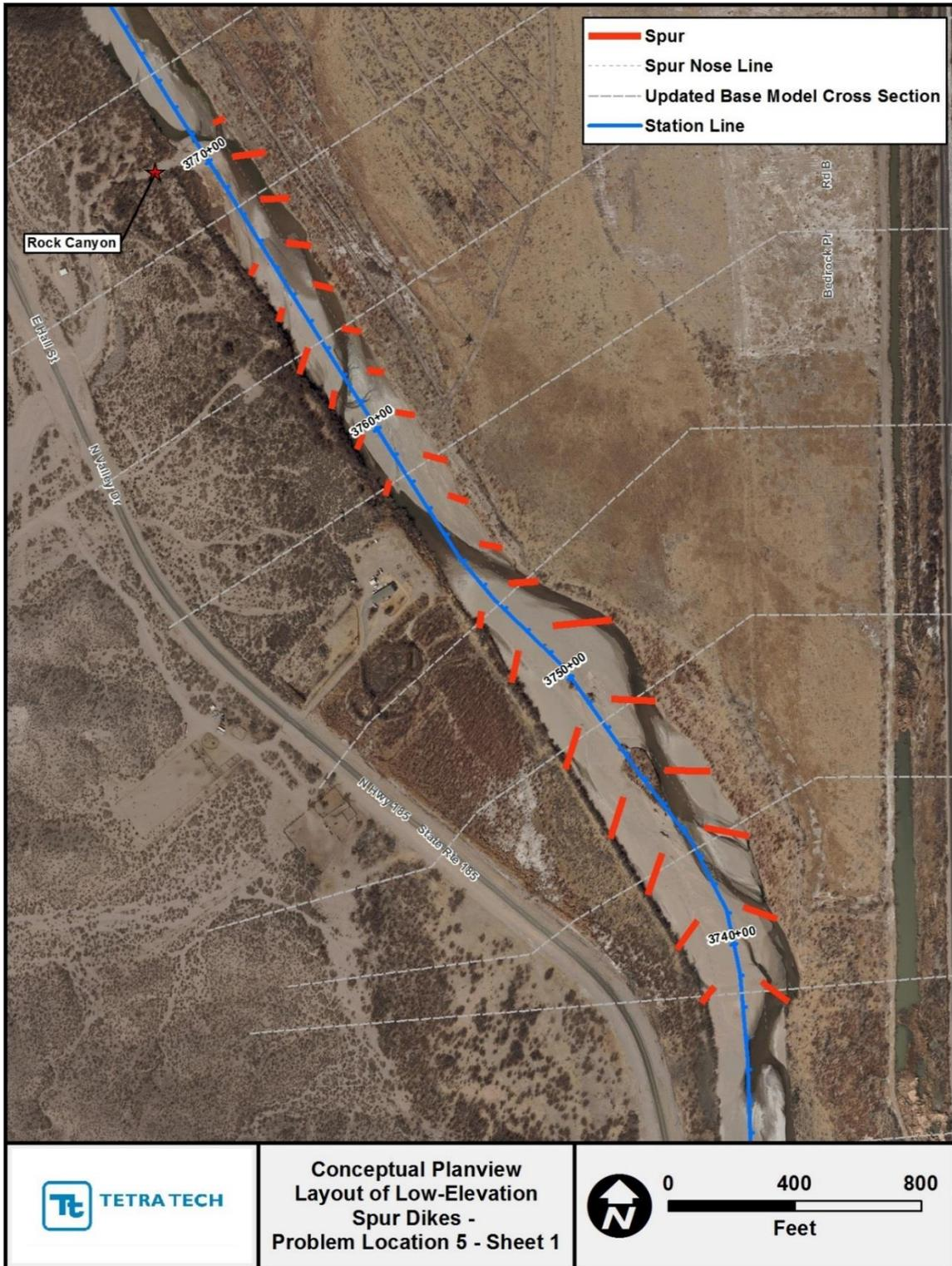
Figure I.4. Conceptual layout of low-elevation spur dikes at Problem Location 5 (Sheet 1; see also Figure 24 in the main report).
