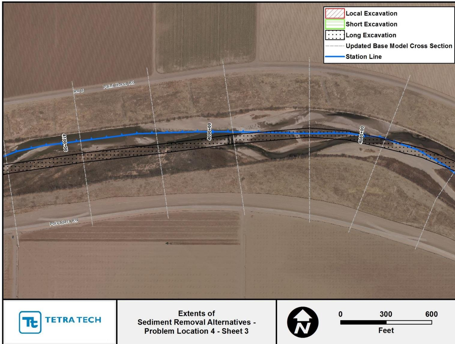
Figure G.2.11. Mapping showing extents of the localized, short and long sediment-removal alternatives at Problem Location 4 (Sheet 3).
