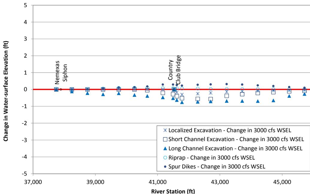
Figure L.60. Predicted change in water-surface elevation at 3,000 cfs at Problem Location 8 for the alternatives that were evaluated with the steady-state hydraulic model compared to existing (base model) conditions.
