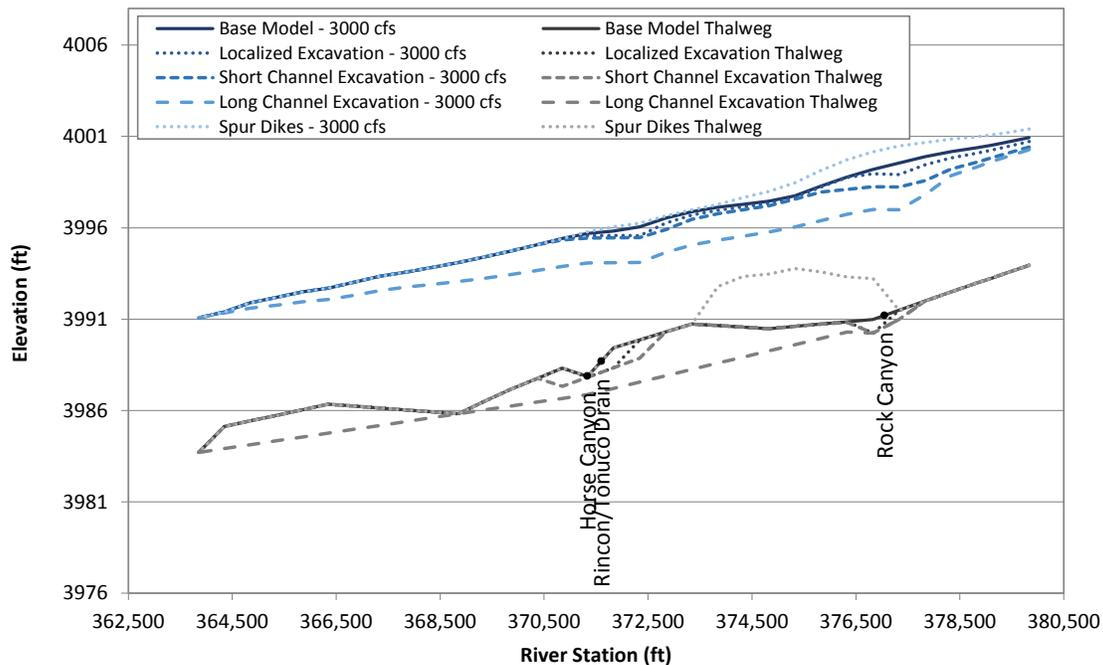
Figure L.35. Predicted water-surface profiles at 3,000 cfs at Problem Location 5 under existing (base model) conditions and for the alternatives that were evaluated with the steady-state hydraulic model.
