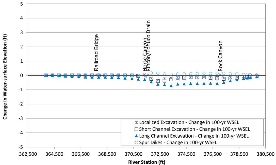
Figure L.40. Predicted change in water-surface elevation at the routed 100-year peak flow at Problem Location 5 for the alternatives that were evaluated with the steady-state hydraulic model compared to existing (base model) conditions.
