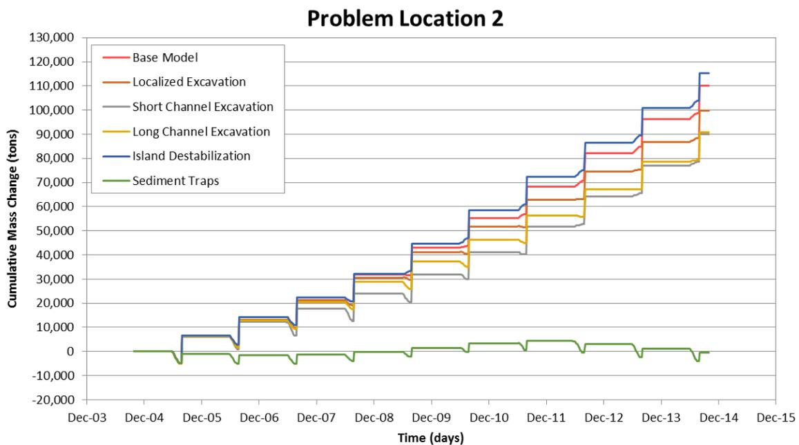
Figure M.2.2. Predicted cumulative mass of aggradation or degradation over time along the modeled reach at Problem Location 2 from the sediment-transport simulations of the base and alternative conditions.
