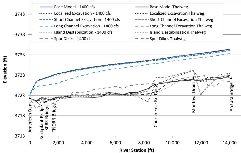
Figure N.33. Predicted water-surface profiles at 1,400 cfs at Problem Location 9 representing long-term conditions based on hydraulic modeling with the predicted geometry at the end of the sediment-transport simulations of the base and alternative conditions.
