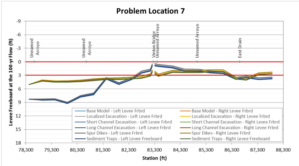
Figure O.5. Predicted levee freeboard during the 100-year flow at Problem Location 7 representing long-term conditions based on hydraulic modeling with the predicted geometry at the end of the sediment-transport simulations of the base and alternative conditions.
