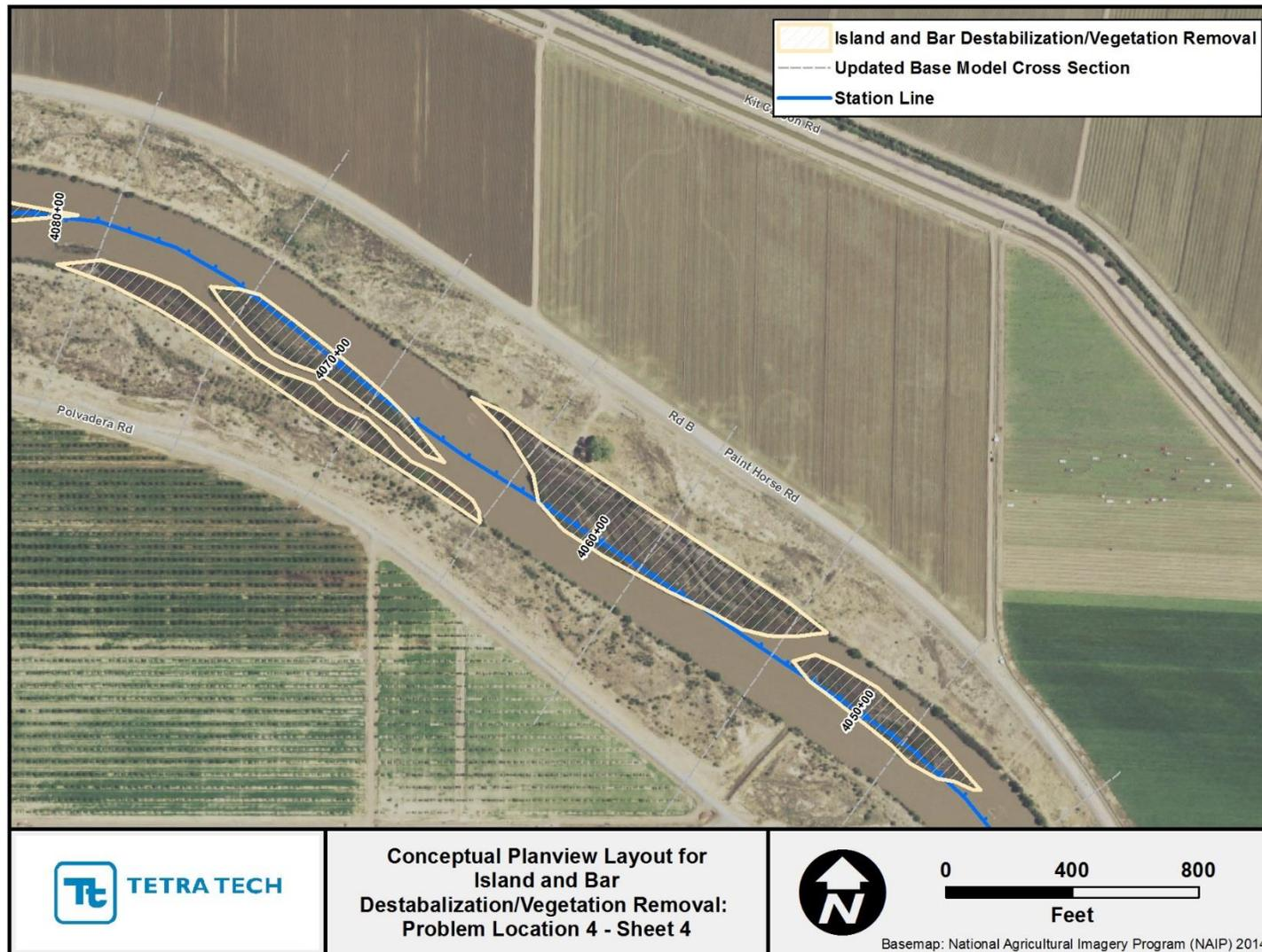
Figure J.9. Aerial photography showing extents of features treated with island/bar destabilization and vegetation removal at Problem Location 4 (Sheet 4).
