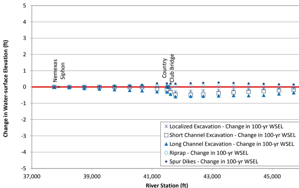
Figure L.64. Predicted change in water-surface elevation at the routed 100-year peak flow at Problem Location 8 for the alternatives that were evaluated with the steady-state hydraulic model compared to existing (base model) conditions.
