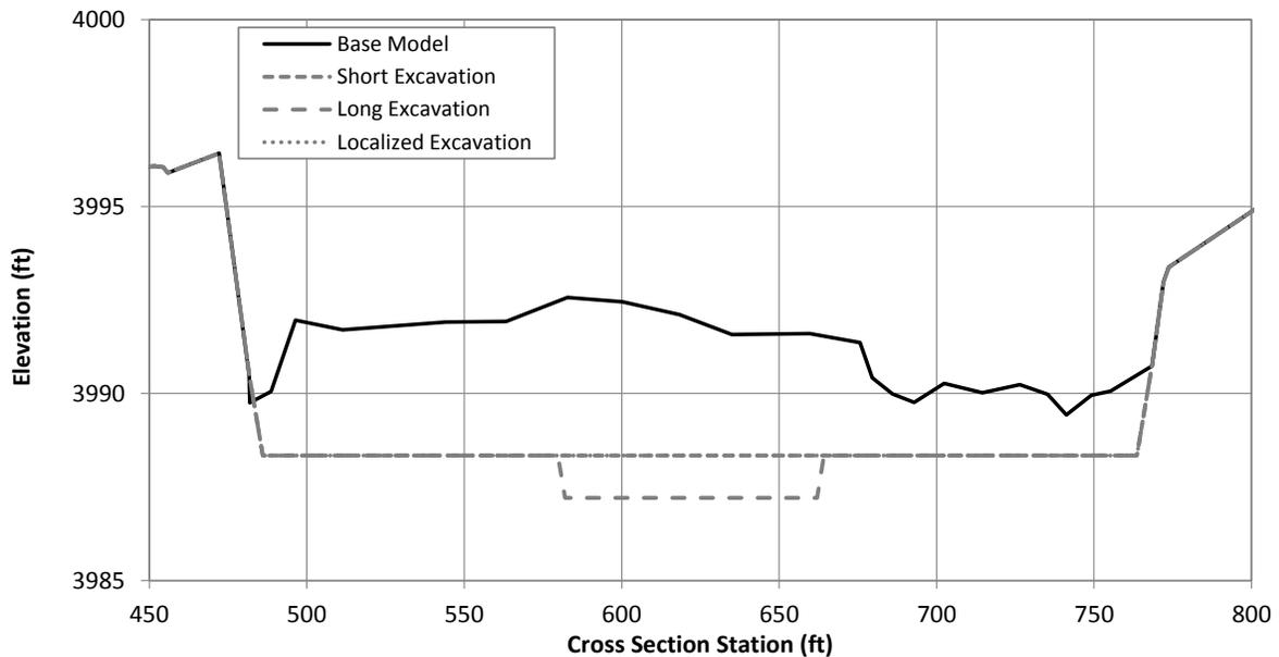
Figure G.1.24. Typical cross section at Problem Location 5 showing the existing (Base Model) channel geometry and excavated geometry under the localized, short and long excavation scenarios (River Station 371836.6).
