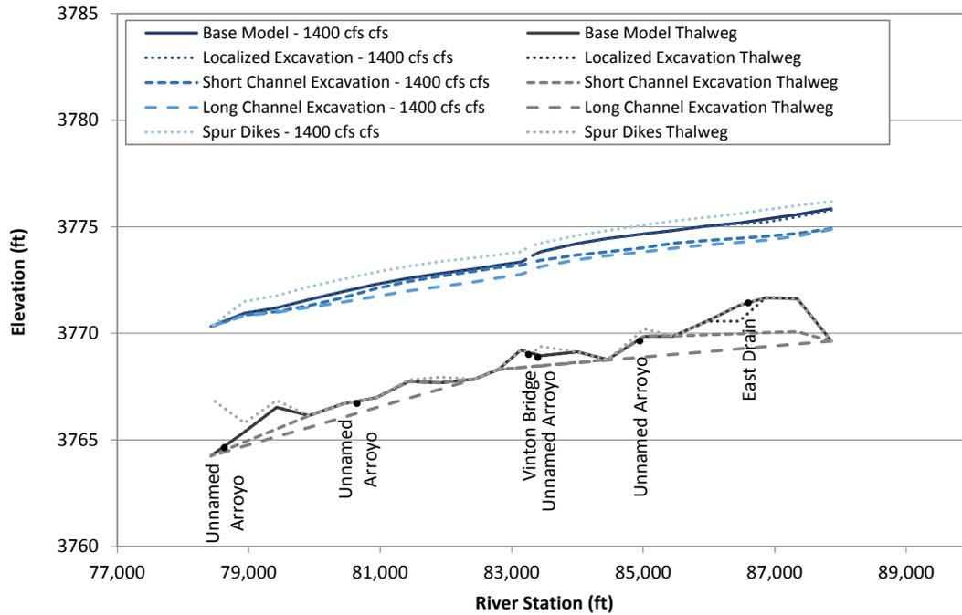
Figure L.49. Predicted water-surface profiles at 1,400 cfs at Problem Location 7 under existing (base model) conditions and for the alternatives that were evaluated with the steady-state hydraulic model.
