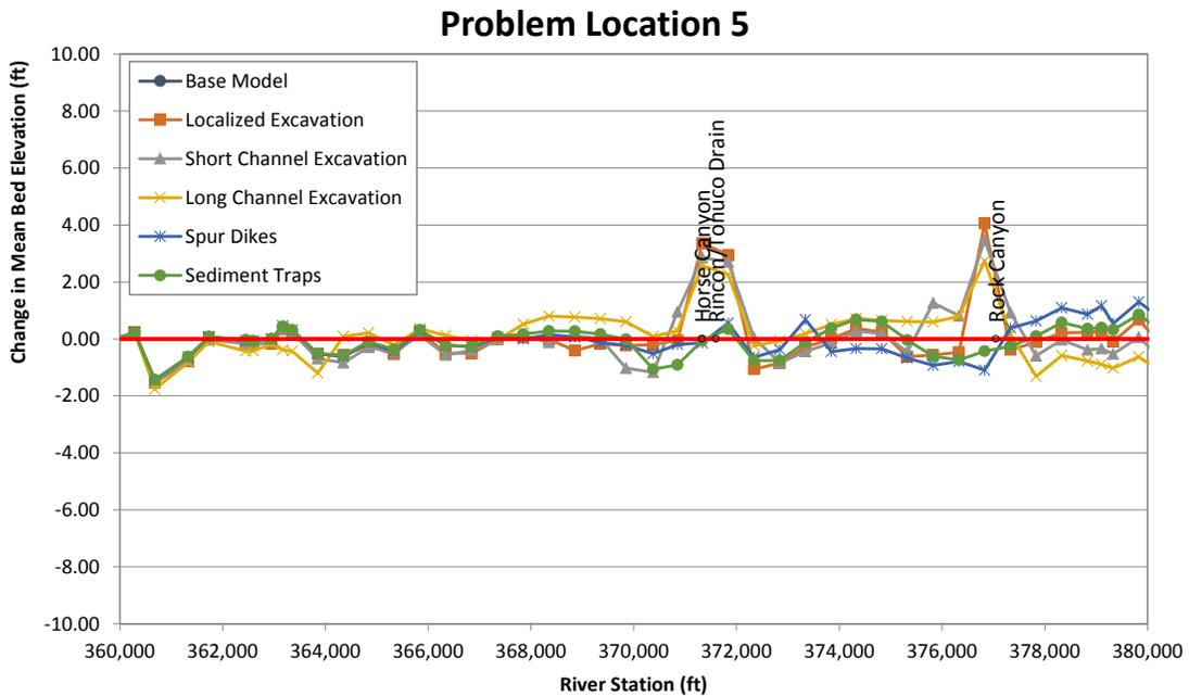
Figure M.1.14. Spatial profiles showing the predicted change in mean bed elevation at the end of the sediment-transport simulations for base alternative conditions at Problem Location 5.
