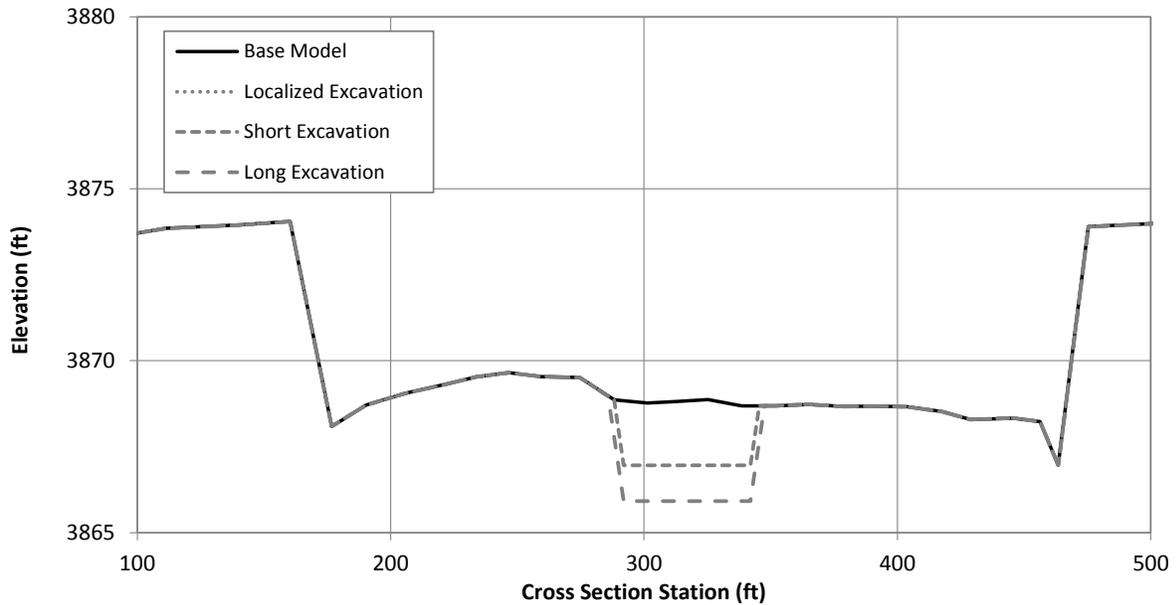
Figure G.1.27. Typical cross section at Problem Location 6 showing the existing (Base Model) channel geometry and excavated geometry under the localized, short and long excavation scenarios (River Station 212468.2).
