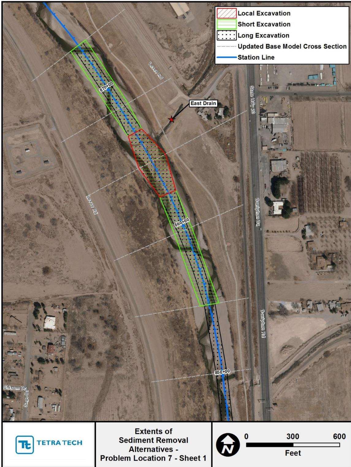
Figure G.2.24. Mapping showing extents of the localized, short and long sediment-removal alternatives at Problem Location 7 (Sheet 1).
