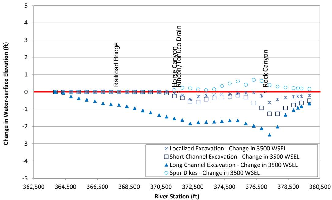
Figure L.38. Predicted change in water-surface elevation at 3,500 cfs at Problem Location 5 for the alternatives that were evaluated with the steady-state hydraulic model compared to existing (base model) conditions.
