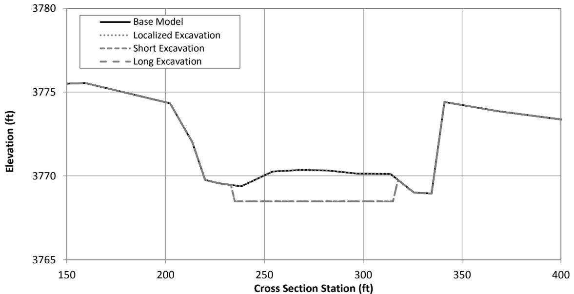
Figure G.1.32. Typical cross section at Problem Location 7 showing the existing (Base Model) channel geometry and excavated geometry under the localized, short and long excavation scenarios (River Station 83444.4).
