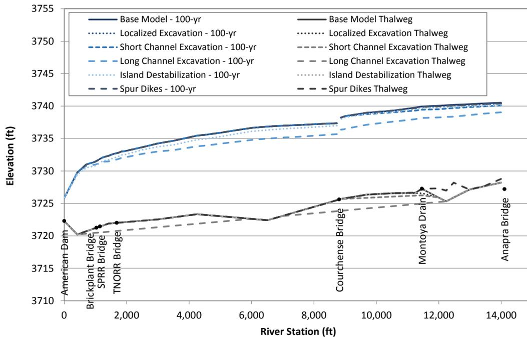
Figure L.71. Predicted water-surface profiles at the routed 100-year peak flow at Problem Location 9 under existing (base model) conditions and for the alternatives that were evaluated with the steady-state hydraulic model.
