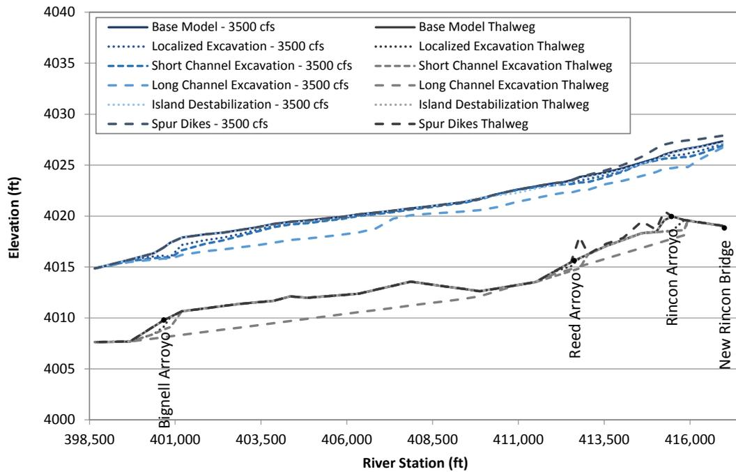
Figure L.29. Predicted water-surface profiles at 3,500 cfs at Problem Location 4 under existing (base model) conditions and for the alternatives that were evaluated with the steady-state hydraulic model.
