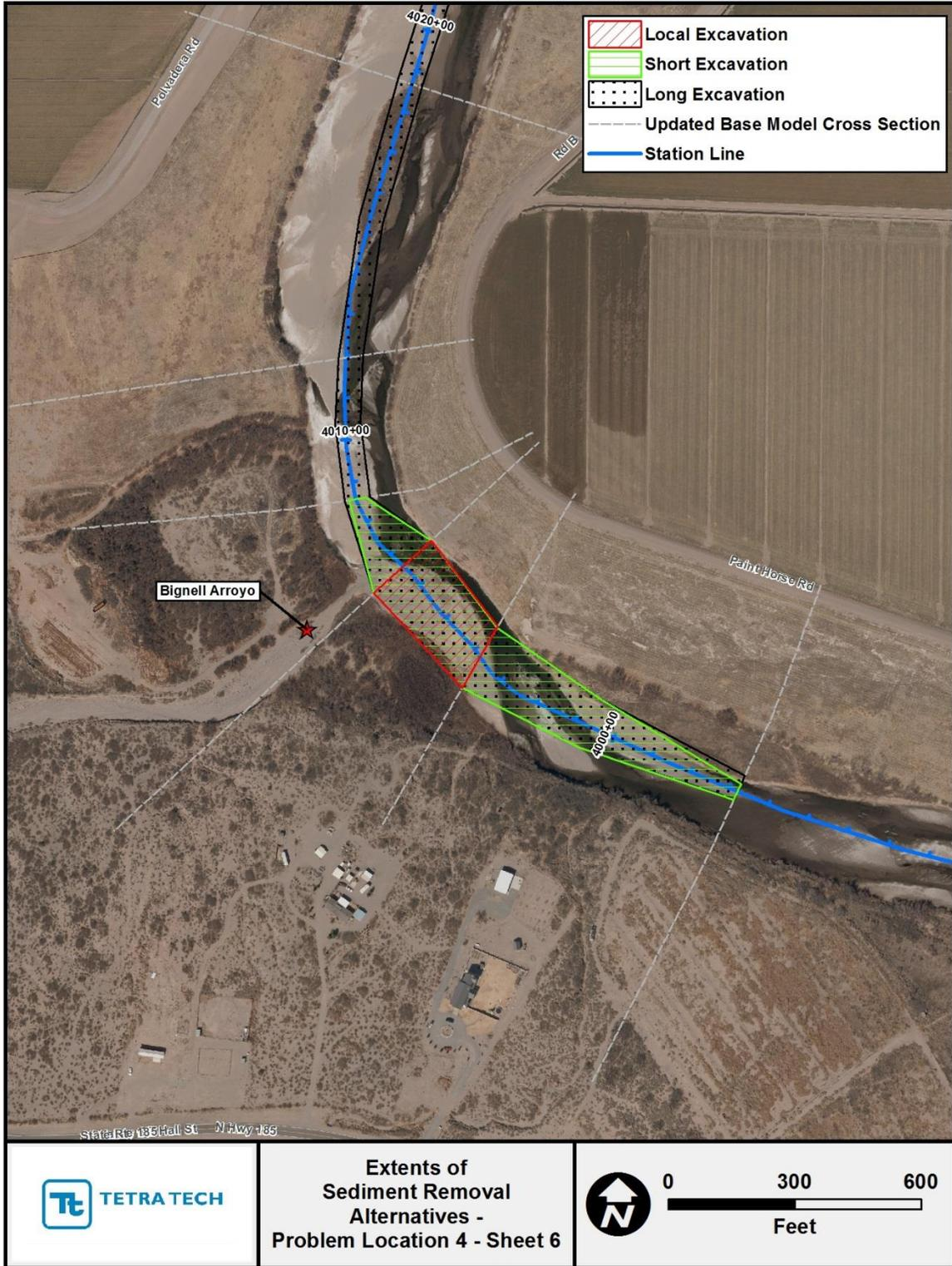
Figure G.2.14. Mapping showing extents of the localized, short and long sediment-removal alternatives at Problem Location 4 (Sheet 6).
