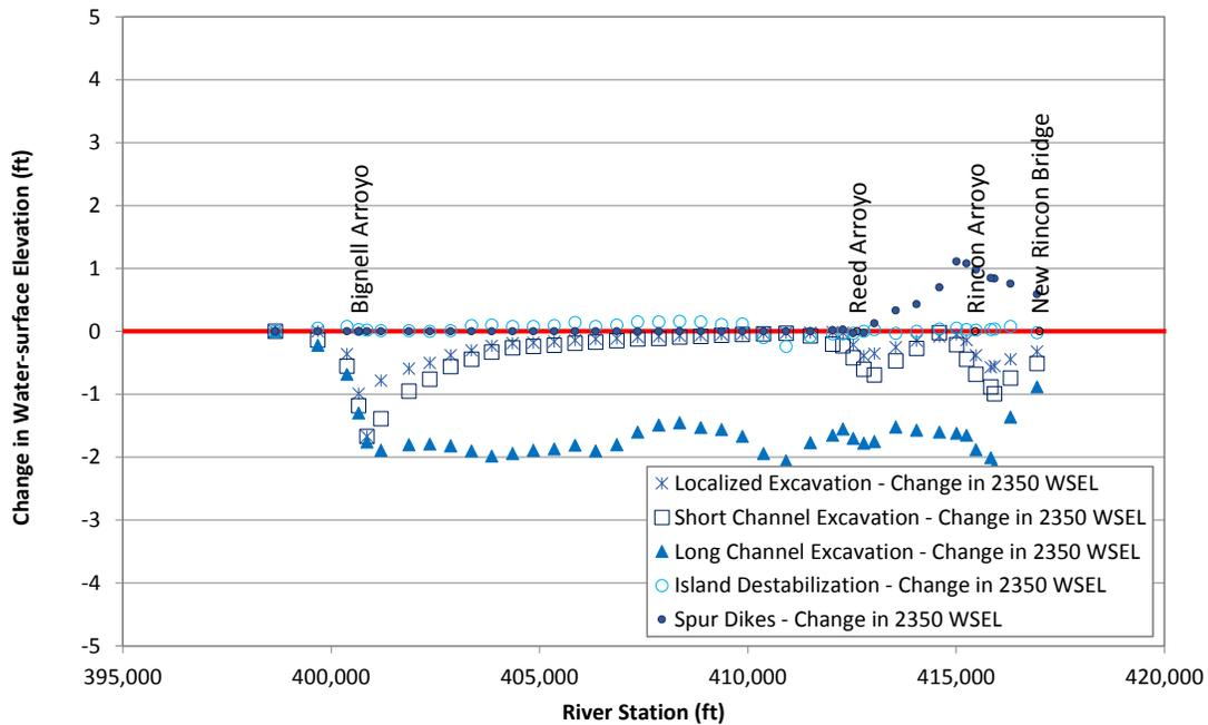
Figure L.26. Predicted change in water-surface elevation at 2,350 cfs at Problem Location 4 for the alternatives that were evaluated with the steady-state hydraulic model compared to existing (base model) conditions.
