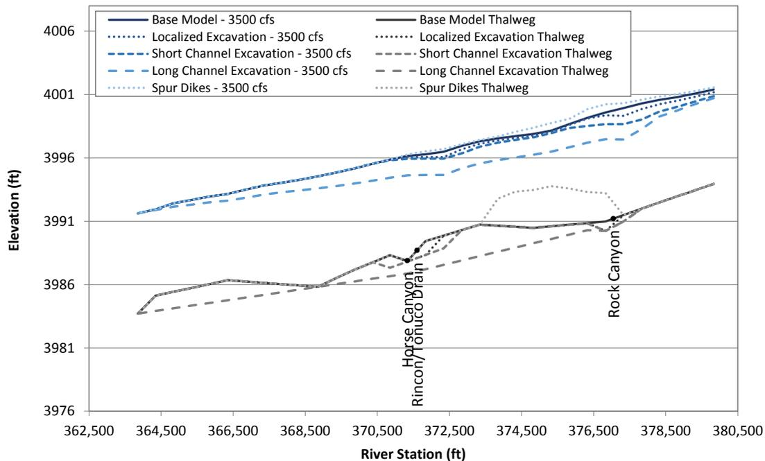
Figure L.37. Predicted water-surface profiles at 3,500 cfs at Problem Location 5 under existing (base model) conditions and for the alternatives that were evaluated with the steady-state hydraulic model.
