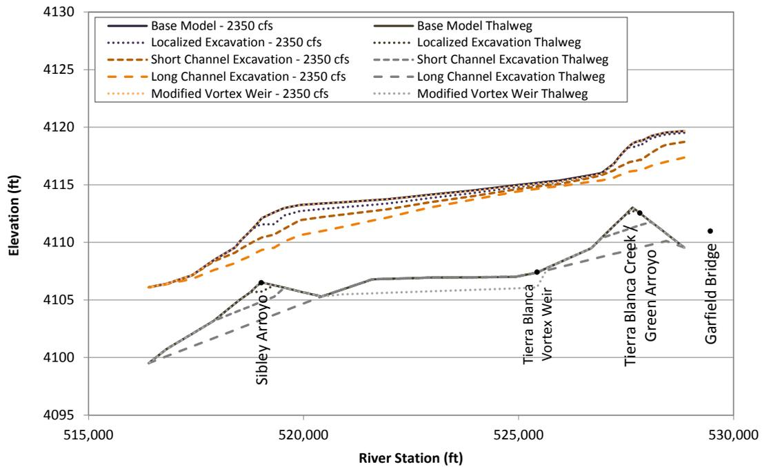
Figure L.1. Predicted water-surface profiles at 2,350 cfs at Problem Location 1 under existing (base model) conditions and for the alternatives that were evaluated with the steady-state hydraulic model.
