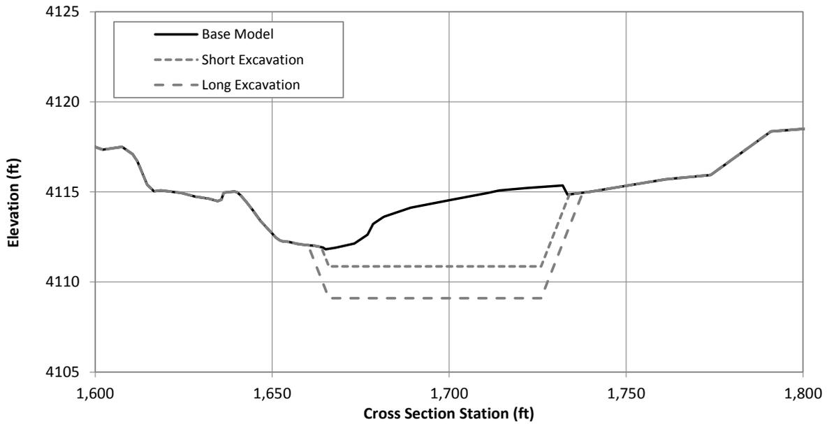
Figure G.1.3. Typical cross section at Problem Location 1 showing the existing (Base Model) channel geometry and excavated geometry under the short and long excavation scenarios (River Station 527320.4).
