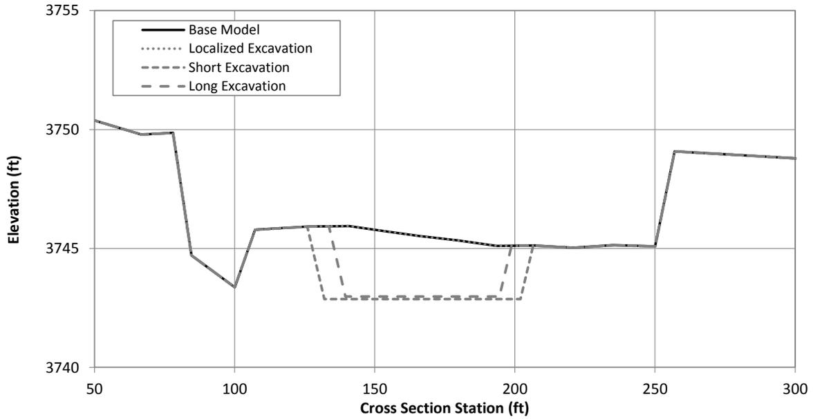
Figure G.1.34. Typical cross section at Problem Location 8 showing the existing (Base Model) channel geometry and excavated geometry under the localized, short and long excavation scenarios (River Station 42287.4).
