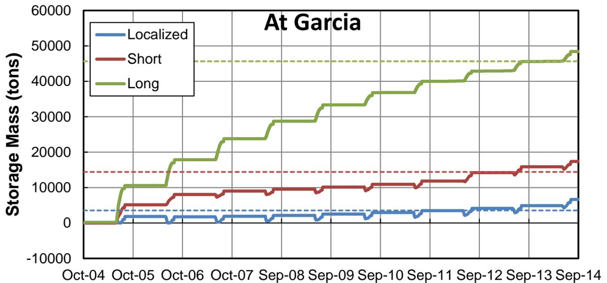
Figure M.2.24. Predicted cumulative mass of aggradation or degradation over time along the extents of the excavated reaches at Garcia Arroyo (Problem Location 3) from the sediment-transport simulations of the sediment-removal alternatives. The dashed lines represent the excavated mass for each type of excavation.
