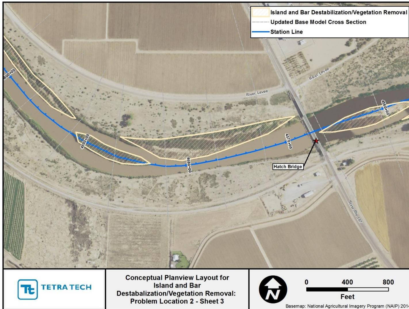
Figure J.3. Aerial photography showing extents of features treated with island/bar destabilization and vegetation removal at Problem Location 2 (Sheet 3).
