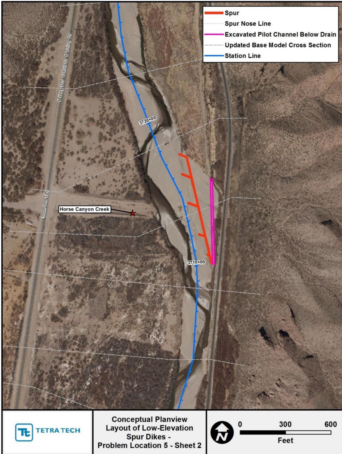
Figure I.5. Conceptual layout of low-elevation spur dikes at Problem Location 5 (Sheet 2; see also Figure 26 in the main report).
