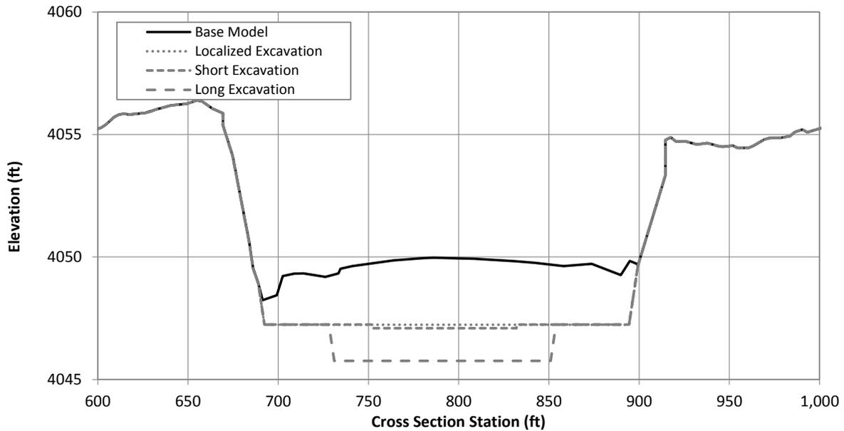
Figure G.1.9. Typical cross section at Problem Location 2 showing the existing (Base Model) channel geometry and excavated geometry under the localized, short and long excavation scenarios (River Station 448155.2).
