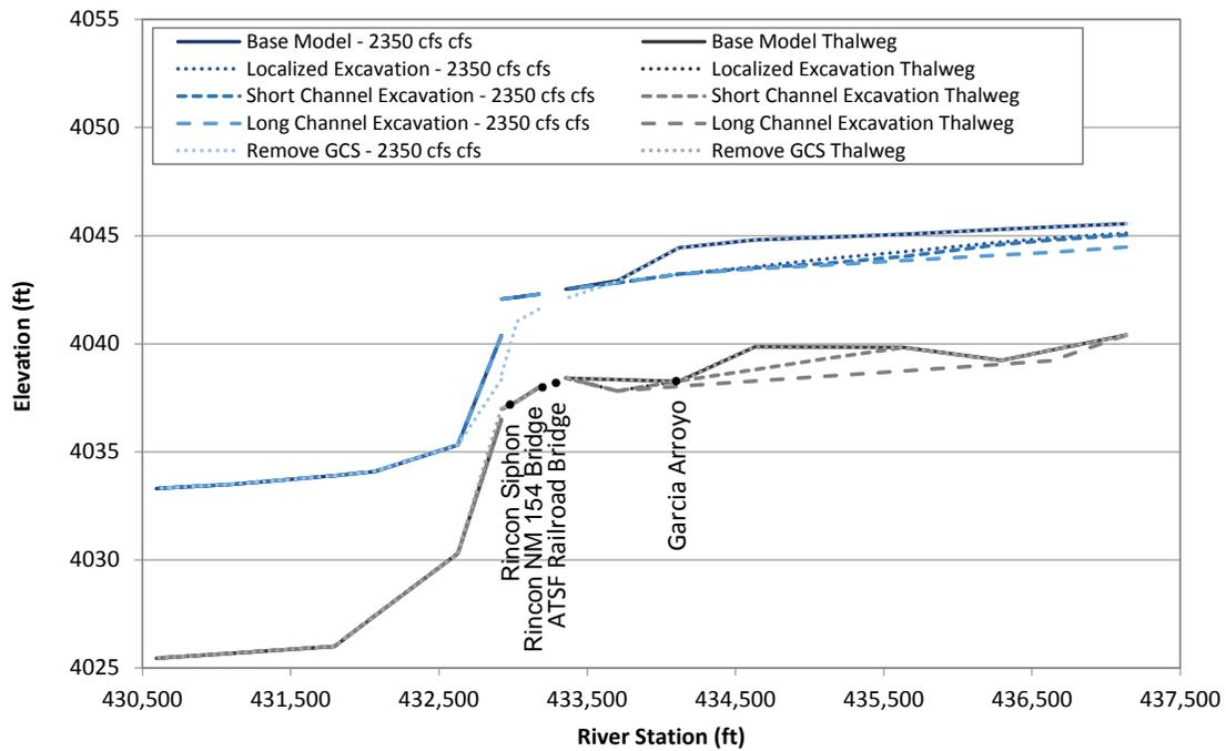
Figure L.17. Predicted water-surface profiles at 2,350 cfs at Problem Location 3 under existing (base model) conditions and for the alternatives that were evaluated with the steady-state hydraulic model.
