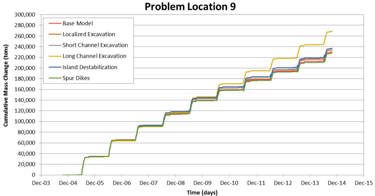
Figure M.2.9. Predicted cumulative mass of aggradation or degradation over time along the modeled reach at Problem Location 9 from the sediment-transport simulations of the base and alternative conditions.
