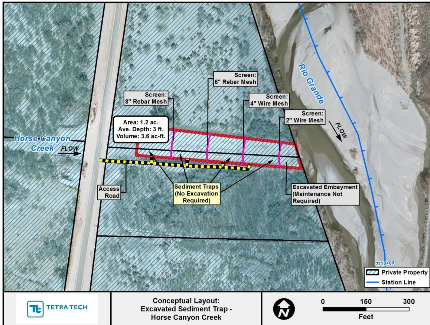
Figure H.9. Conceptual layout of sediment trap for Horse Canyon Creek at Problem Location 5.
