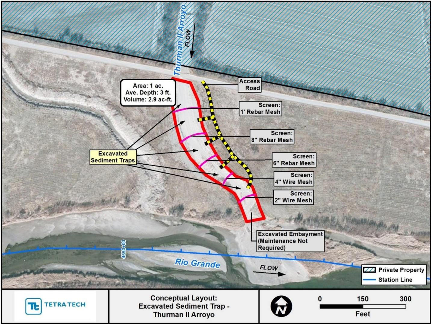
Figure H.4. Conceptual layout of sediment trap for Thurman II Arroyo at Problem Location 2.
