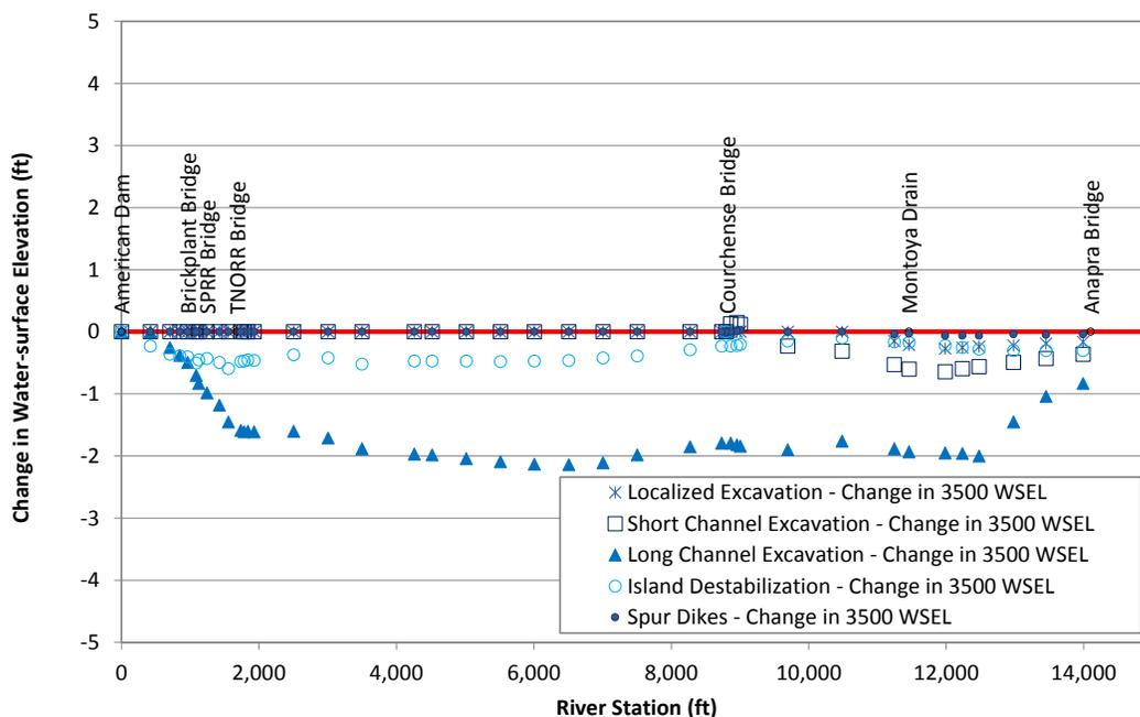
Figure L.70. Predicted change in water-surface elevation at 3,500 cfs at Problem Location 9 for the alternatives that were evaluated with the steady-state hydraulic model compared to existing (base model) conditions.
