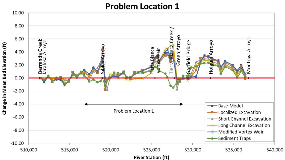
Figure M.1.10. Spatial profiles showing the predicted change in mean bed elevation at the end of the sediment-transport simulations for base alternative conditions at Problem Location 1.
