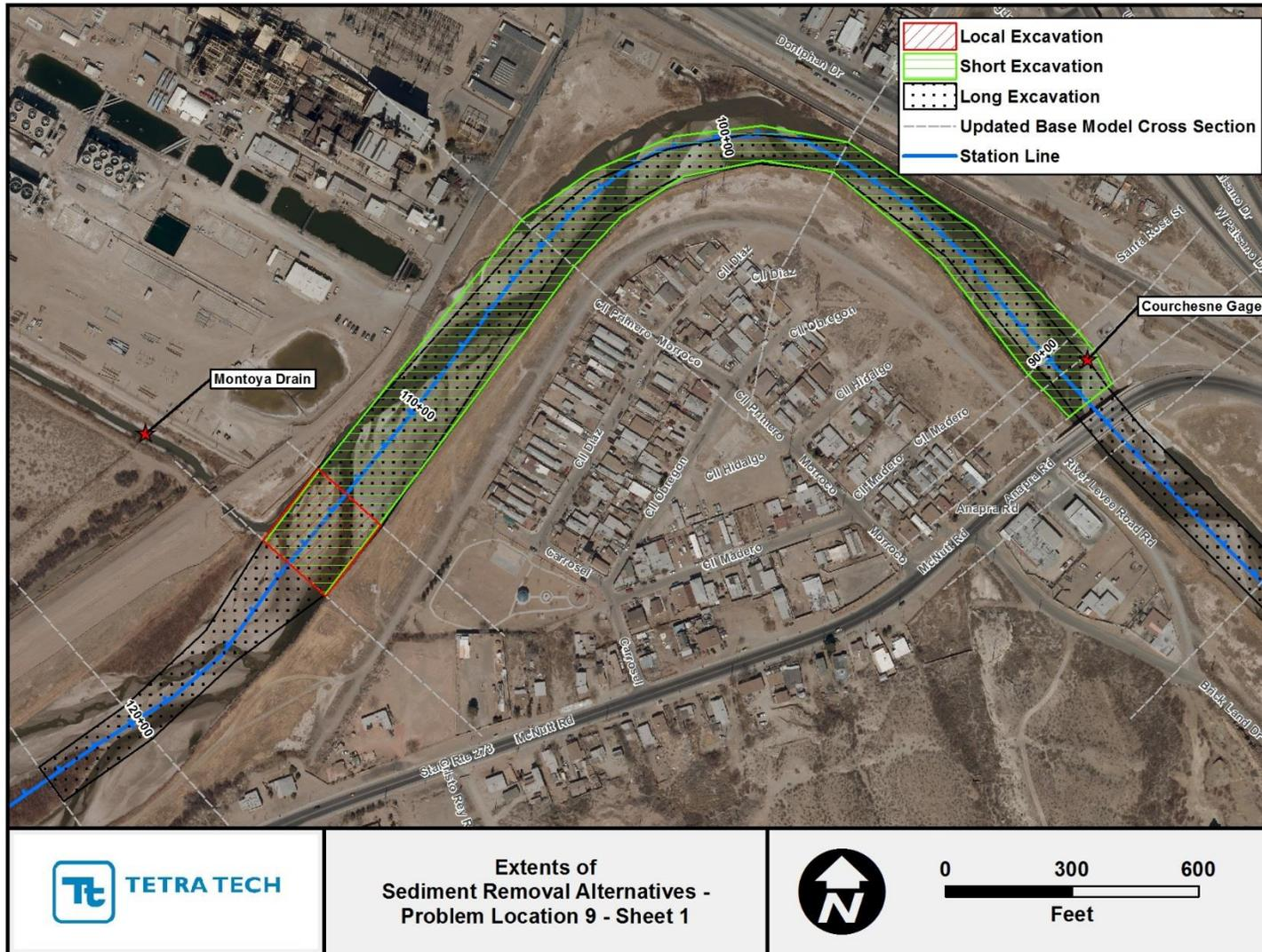
Figure G.2.31. Mapping showing extents of the localized, short and long sediment-removal alternatives at Problem Location 9 (Sheet 1).
