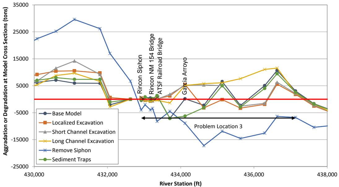
Figure M.1.3. Spatial profiles showing the predicted cumulative mass of aggradation or degradation at the end of the sediment-transport simulations for base alternative conditions at Problem Location 3.
