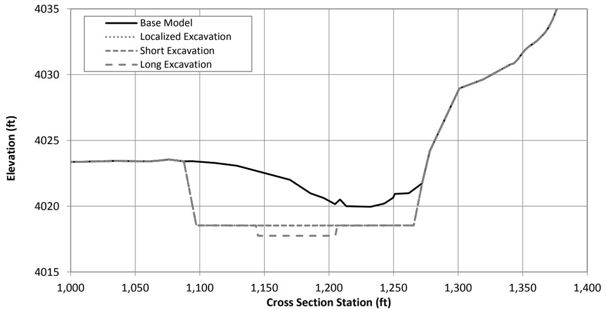
Figure G.1.16. Typical cross section at Problem Location 4 showing the existing (Base Model) channel geometry and excavated geometry under the localized, short and long excavation scenarios (River Station 415476.8).
