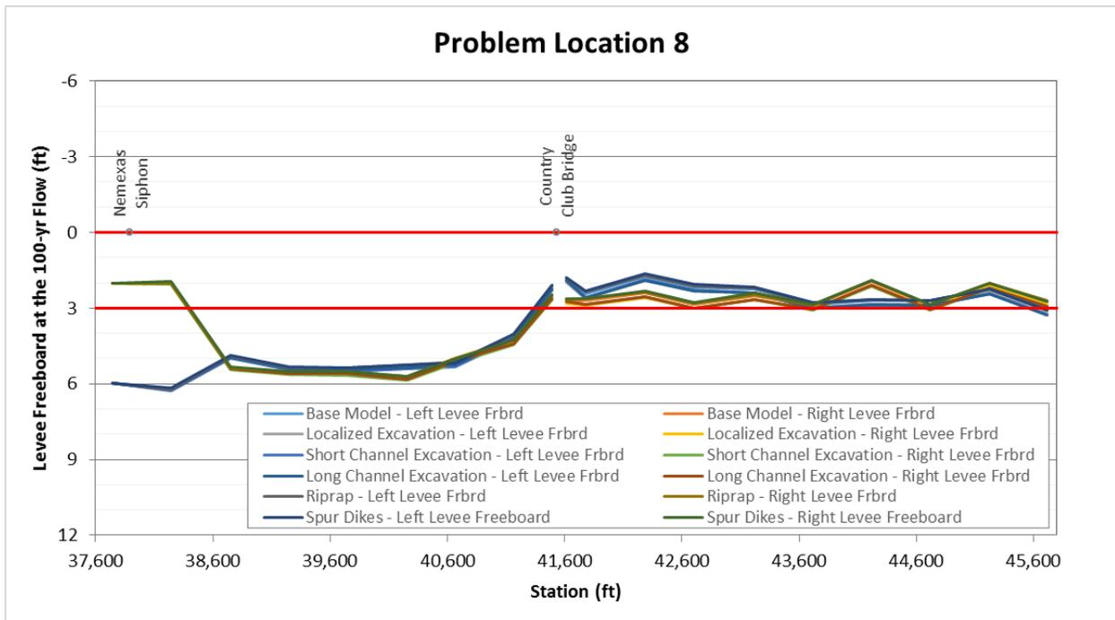
Figure O.6. Predicted levee freeboard during the 100-year flow at Problem Location 8 representing long-term conditions based on hydraulic modeling with the predicted geometry at the end of the sediment-transport simulations of the base and alternative conditions.
