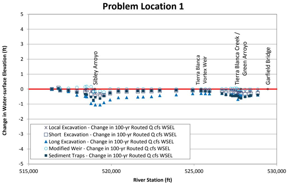
Figure N.4. Predicted change in long-term water-surface elevation at the 100-year peak flow relative to the base condition at Problem Location 1 for the alternatives that were evaluated with the steady-state hydraulic model compared to existing (base model) conditions.
