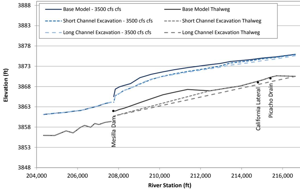
Figure L.45. Predicted water-surface profiles at 3,500 cfs at Problem Location 6 under existing (base model) conditions and for the alternatives that were evaluated with the steady-state hydraulic model.
