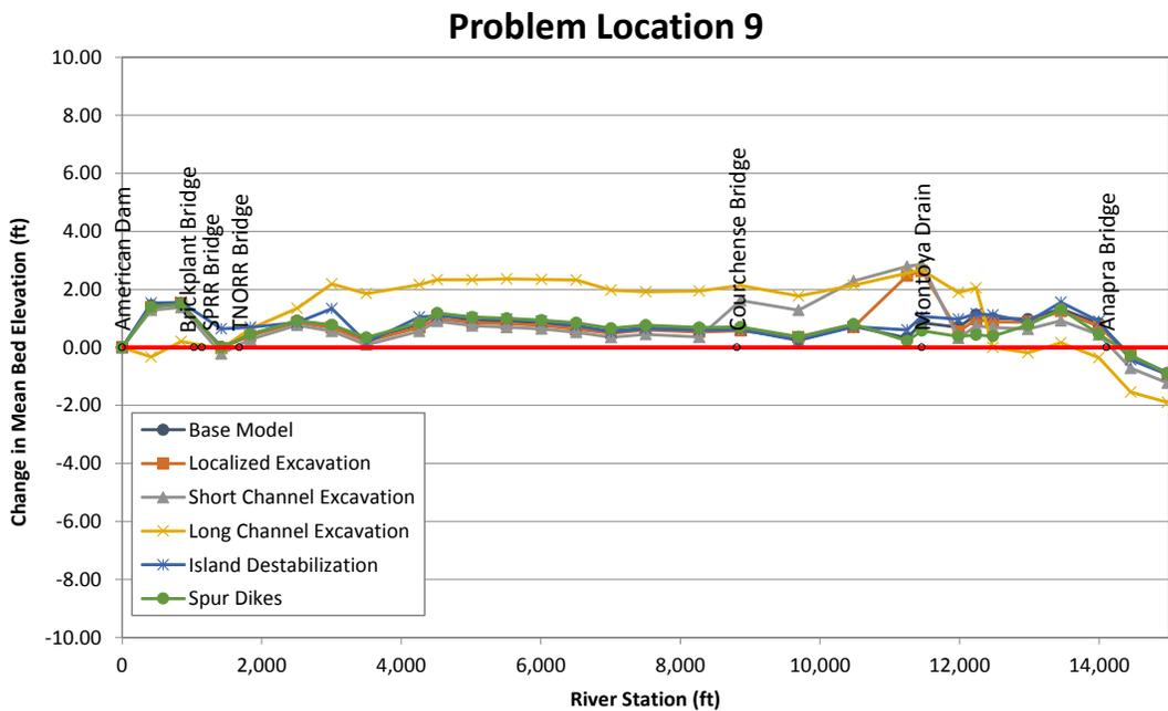
Figure M.1.18. Spatial profiles showing the predicted change in mean bed elevation at the end of the sediment-transport simulations for base alternative conditions at Problem Location 9.
