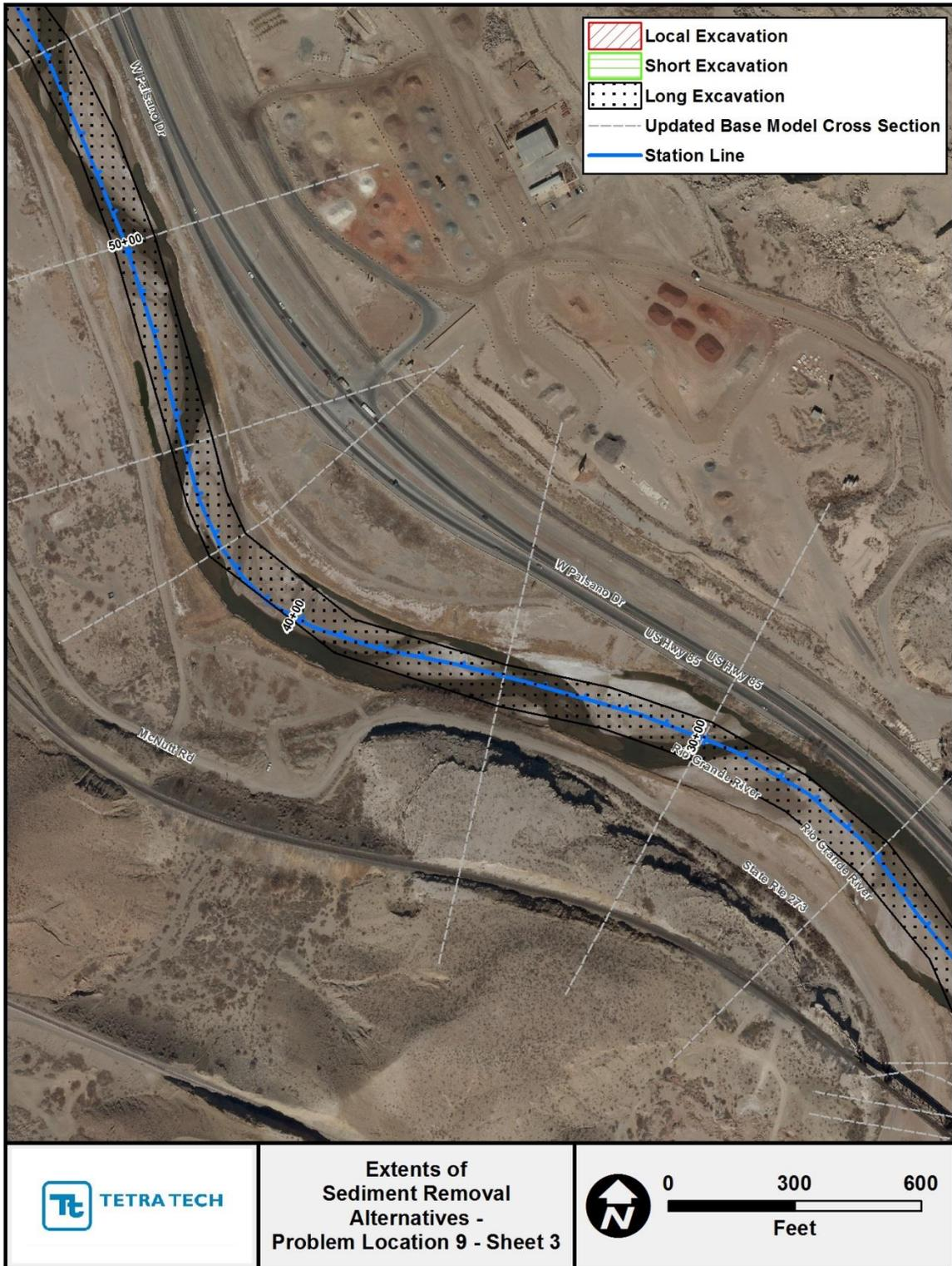
Figure G.2.33. Mapping showing extents of the localized, short and long sediment-removal alternatives at Problem Location 9 (Sheet 3).
