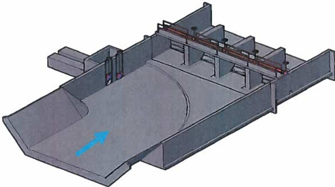
Figure 1. 3D view of proposed design for new Westside first check structure and sluiceway
