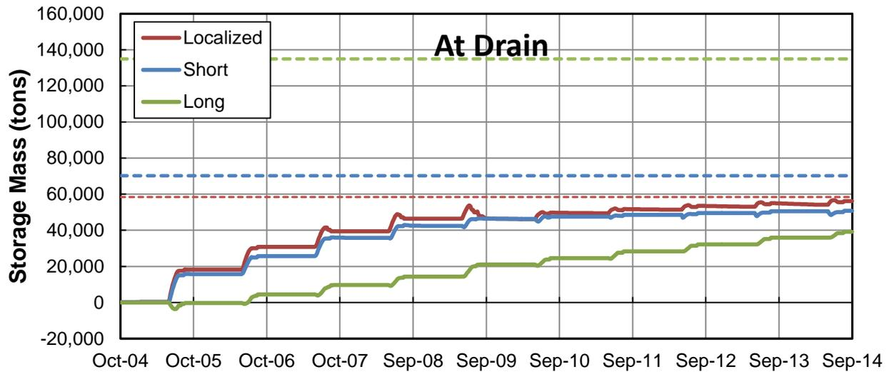
Figure M.2.29. Predicted cumulative mass of aggradation or degradation over time along the extents of the excavated reaches at the Rincon/Tonuco Drain (Problem Location 5) from the sediment-transport simulations of the sediment-removal alternatives. The dashed lines represent the excavated mass for each type of excavation.
