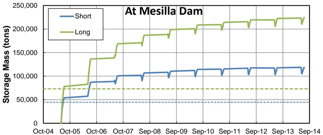
Figure M.2.30. Predicted cumulative mass of aggradation or degradation over time along the extents of the excavated reaches at Mesilla Dam (Problem Location 6) from the sediment-transport simulations of the sediment-removal alternatives. The dashed lines represent the excavated mass for each type of excavation.
