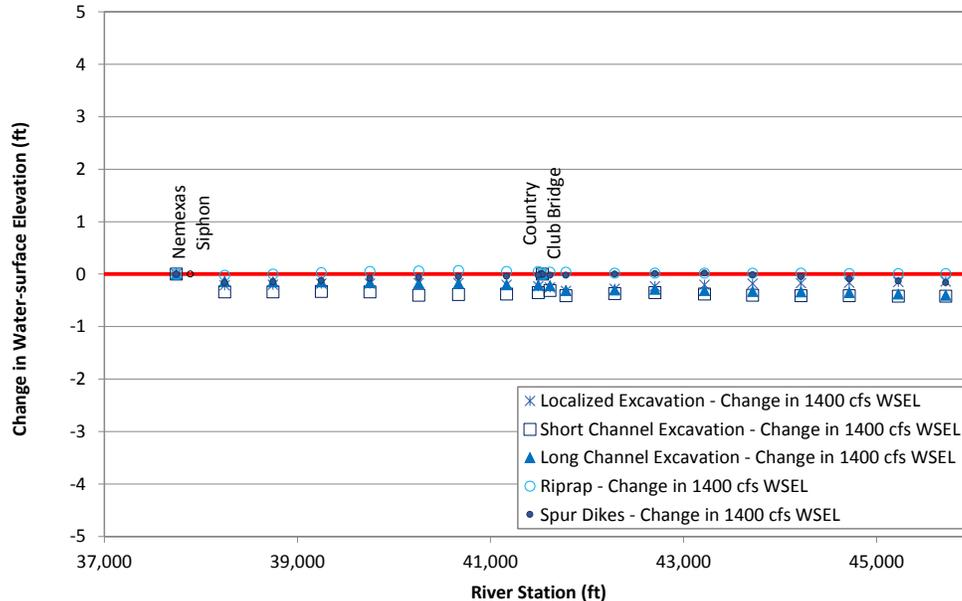
Figure N.30. Predicted change in long-term water-surface elevation at 1,400 cfs relative to the base condition at Problem Location 8 for the alternatives that were evaluated with the steady-state hydraulic model compared to existing (base model) conditions.
