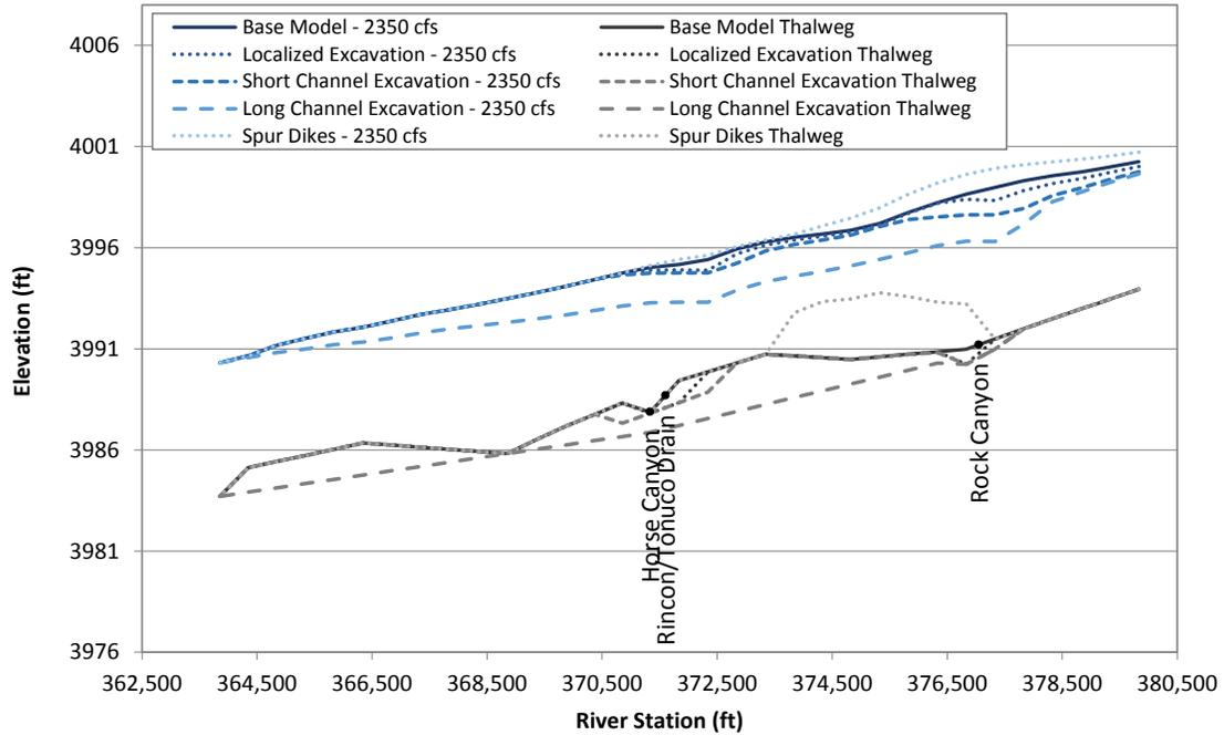
Figure L.33. Predicted water-surface profiles at 2,350 cfs at Problem Location 5 under existing (base model) conditions and for the alternatives that were evaluated with the steady-state hydraulic model.
