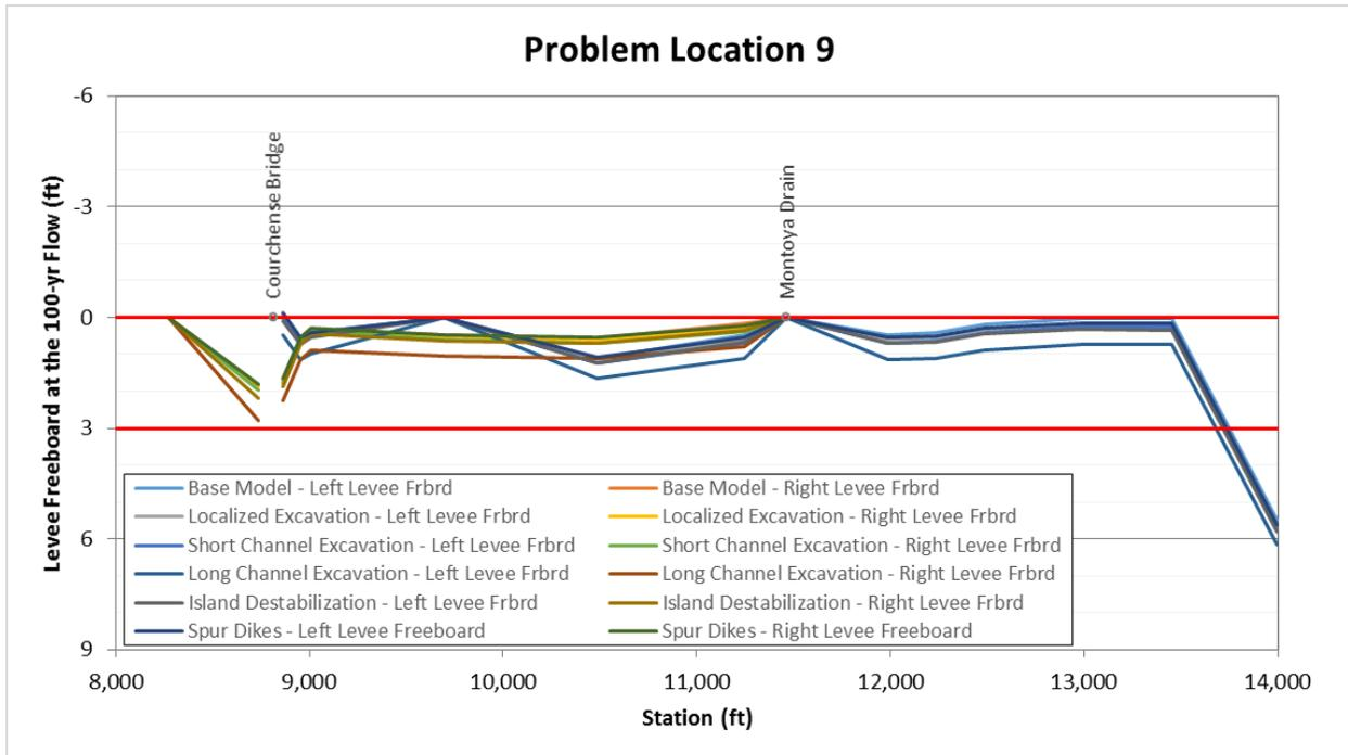
Figure O.7. Predicted levee freeboard during the 100-year flow at Problem Location 9 representing long-term conditions based on hydraulic modeling with the predicted geometry at the end of the sediment-transport simulations of the base and alternative conditions.
