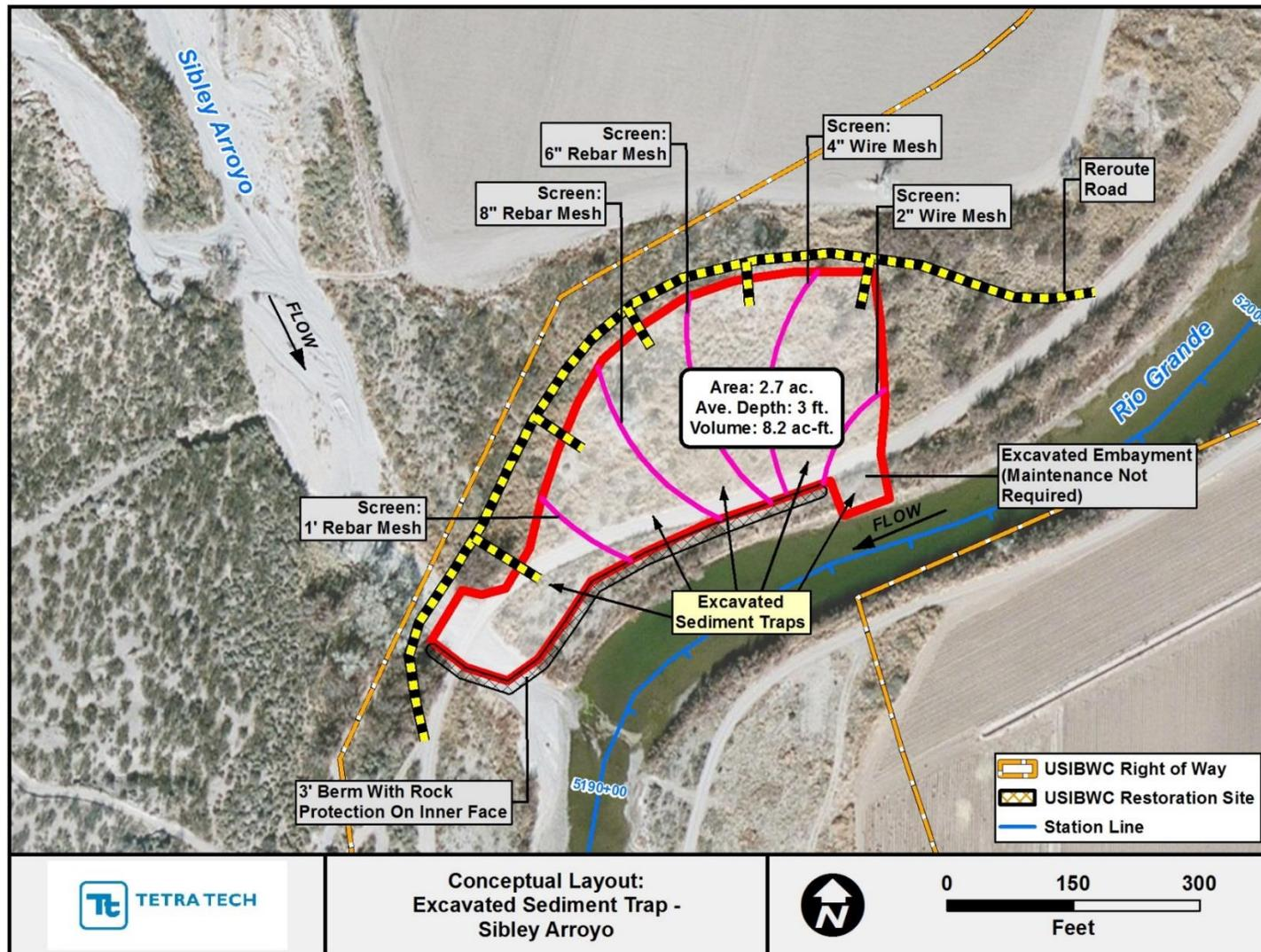
Figure H.3. Conceptual layout of sediment trap for Sibley Arroyo at Problem Location 1.
