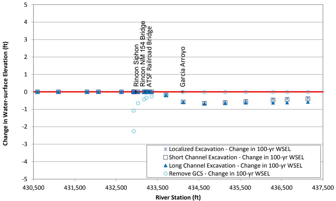
Figure L.24. Predicted change in water-surface elevation at the routed 100-year peak flow at Problem Location 3 for the alternatives that were evaluated with the steady-state hydraulic model compared to existing (base model) conditions.
