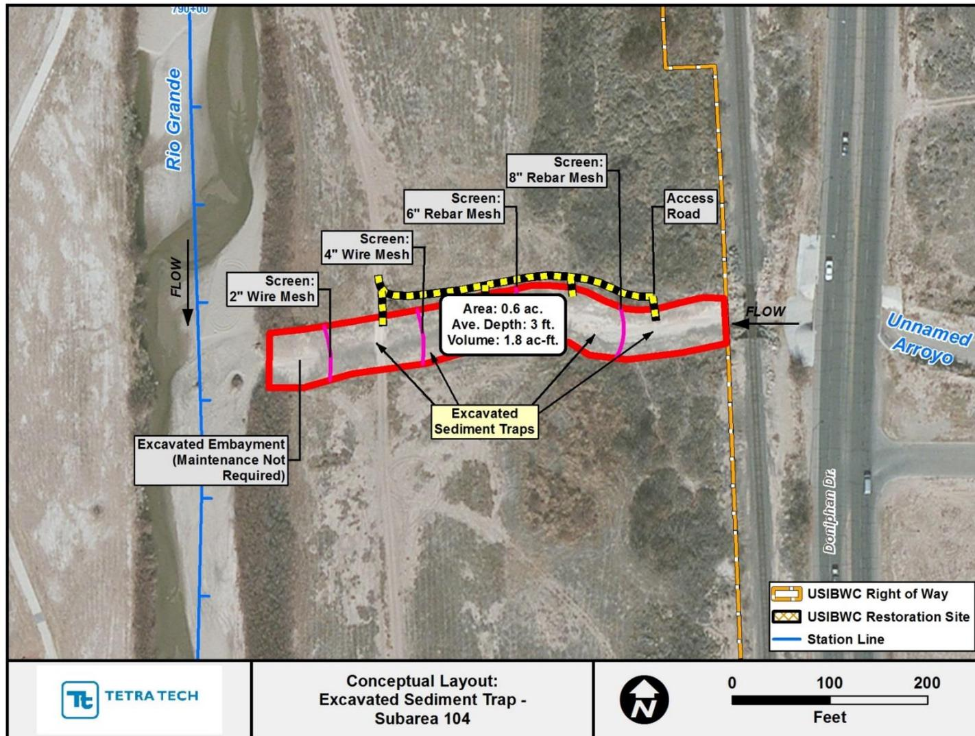
Figure H.13. Conceptual layout of sediment trap for the unnamed arroyo draining Subarea 104 at Problem Location 7.
