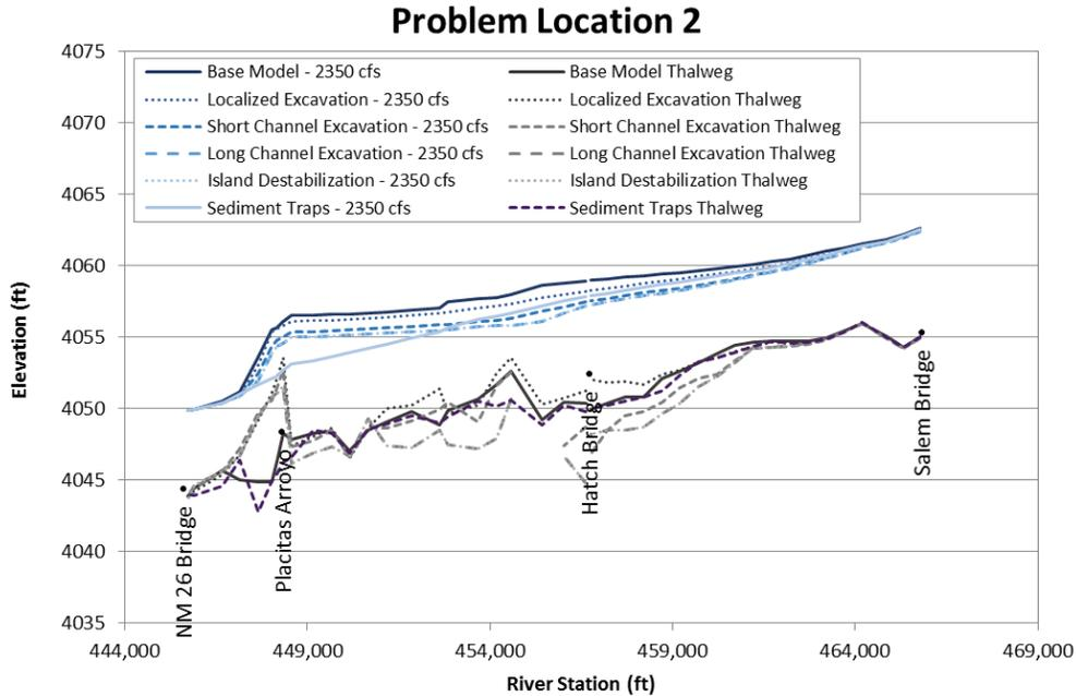
Figure N.5. Predicted water-surface profiles at 2,350 cfs at Problem Location 2 representing long-term conditions based on hydraulic modeling with the predicted geometry at the end of the sediment-transport simulations of the base and alternative conditions.
