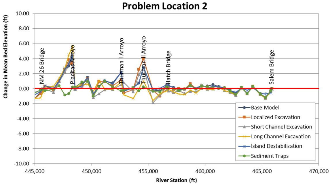
Figure M.1.11. Spatial profiles showing the predicted change in mean bed elevation at the end of the sediment-transport simulations for base alternative conditions at Problem Location 2.
