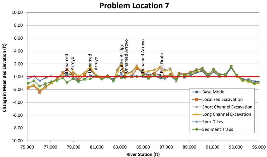
Figure M.1.16. Spatial profiles showing the predicted change in mean bed elevation at the end of the sediment-transport simulations for base alternative conditions at Problem Location 7.
