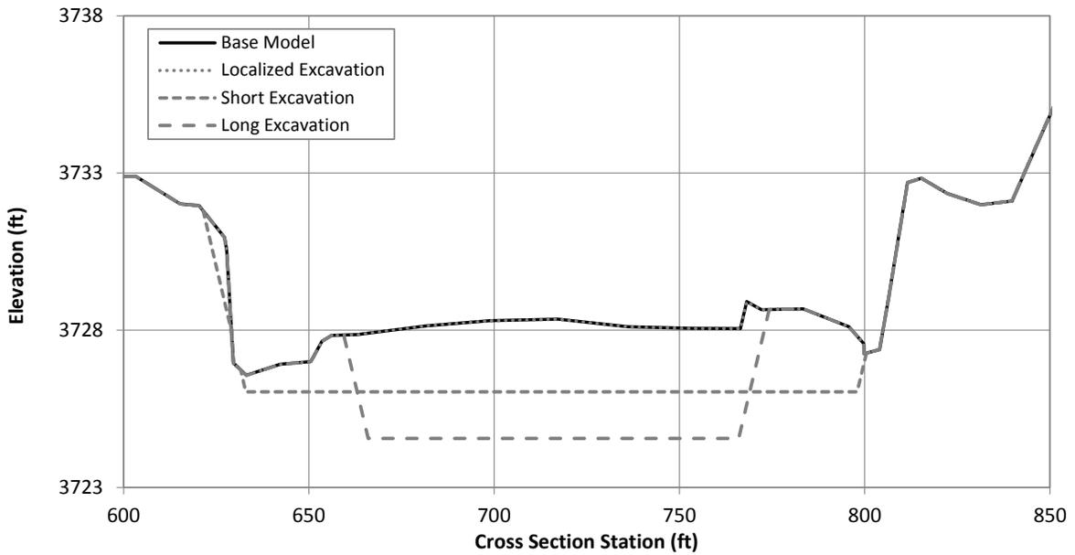
Figure G.1.39. Typical cross section at Problem Location 9 showing the existing (Base Model) channel geometry and excavated geometry under the localized, short and long excavation scenarios (River Station 10483.52).
