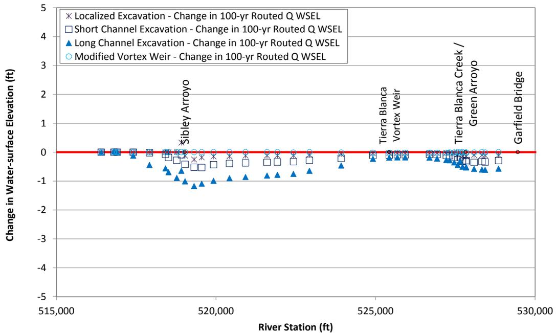
Figure L.8. Predicted change in water-surface elevation at the routed 100-year peak flow at Problem Location 1 for the alternatives that were evaluated with the steady-state hydraulic model compared to existing (base model) conditions.
