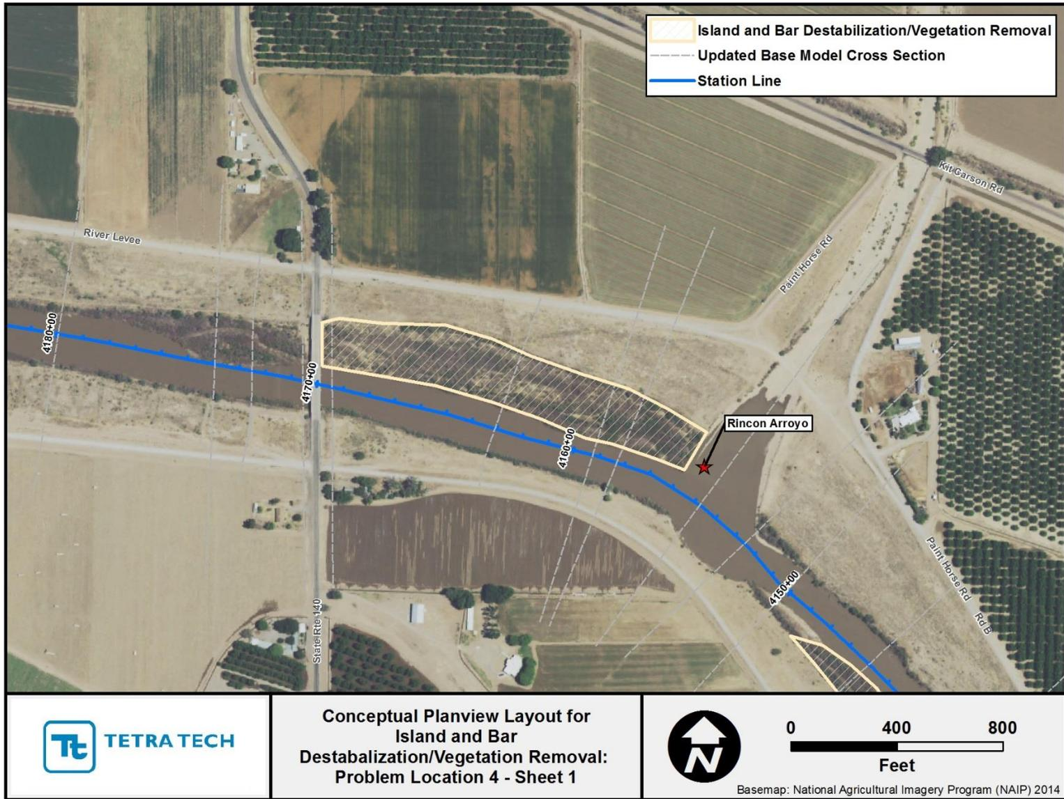
Figure J.6. Aerial photography showing extents of features treated with island/bar destabilization and vegetation removal at Problem Location 4 (Sheet 1).
