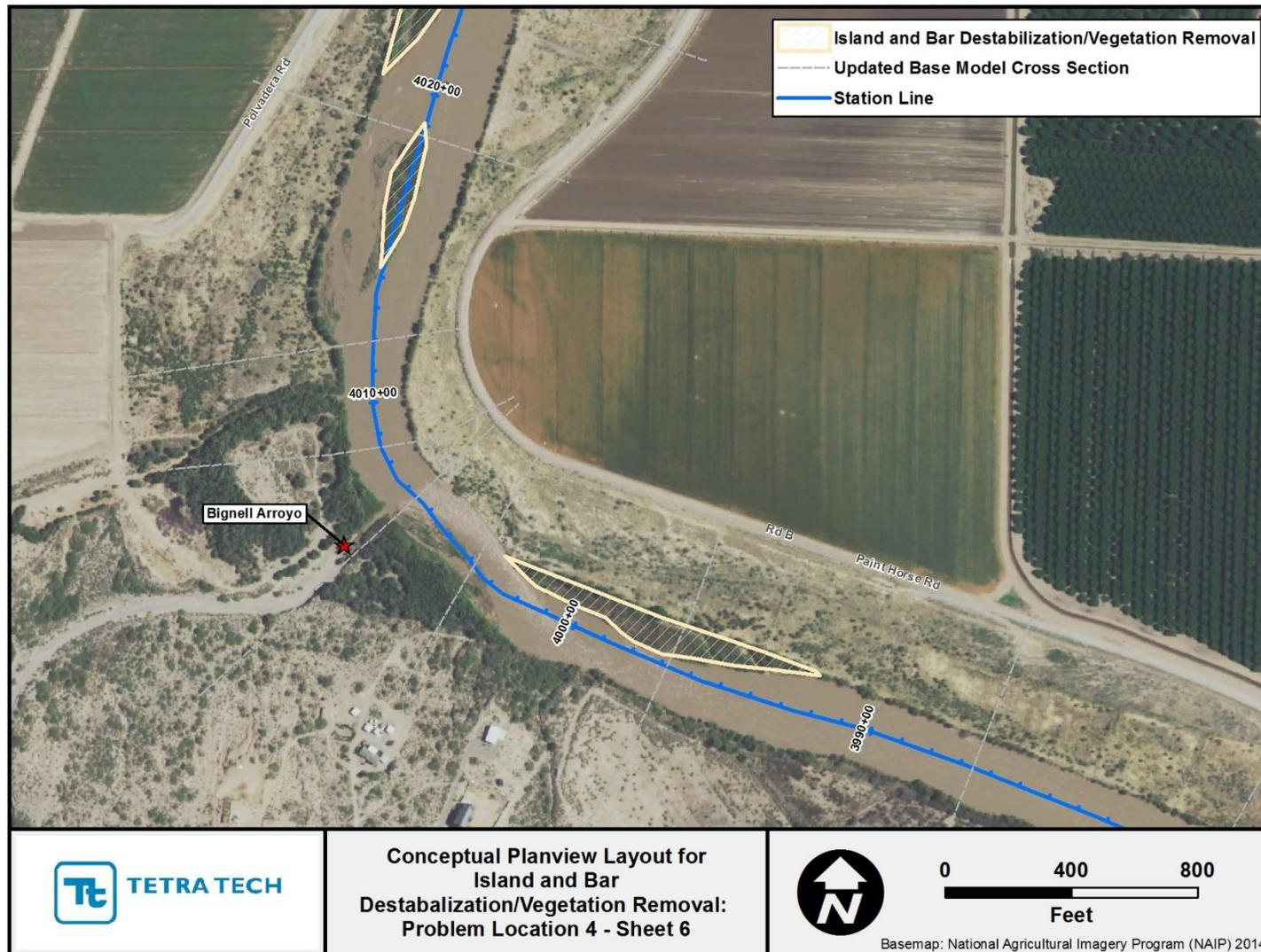
Figure J.11. Aerial photography showing extents of features treated with island/bar destabilization and vegetation removal at Problem Location 4 (Sheet 6).
