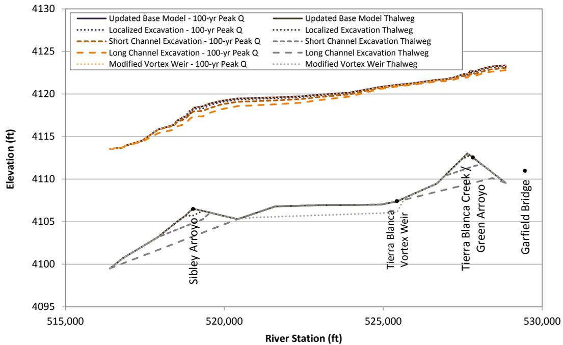
Figure L.7. Predicted water-surface profiles at the routed 100-year peak flow at Problem Location 1 under existing (base model) conditions and for the alternatives that were evaluated with the steady-state hydraulic model.
