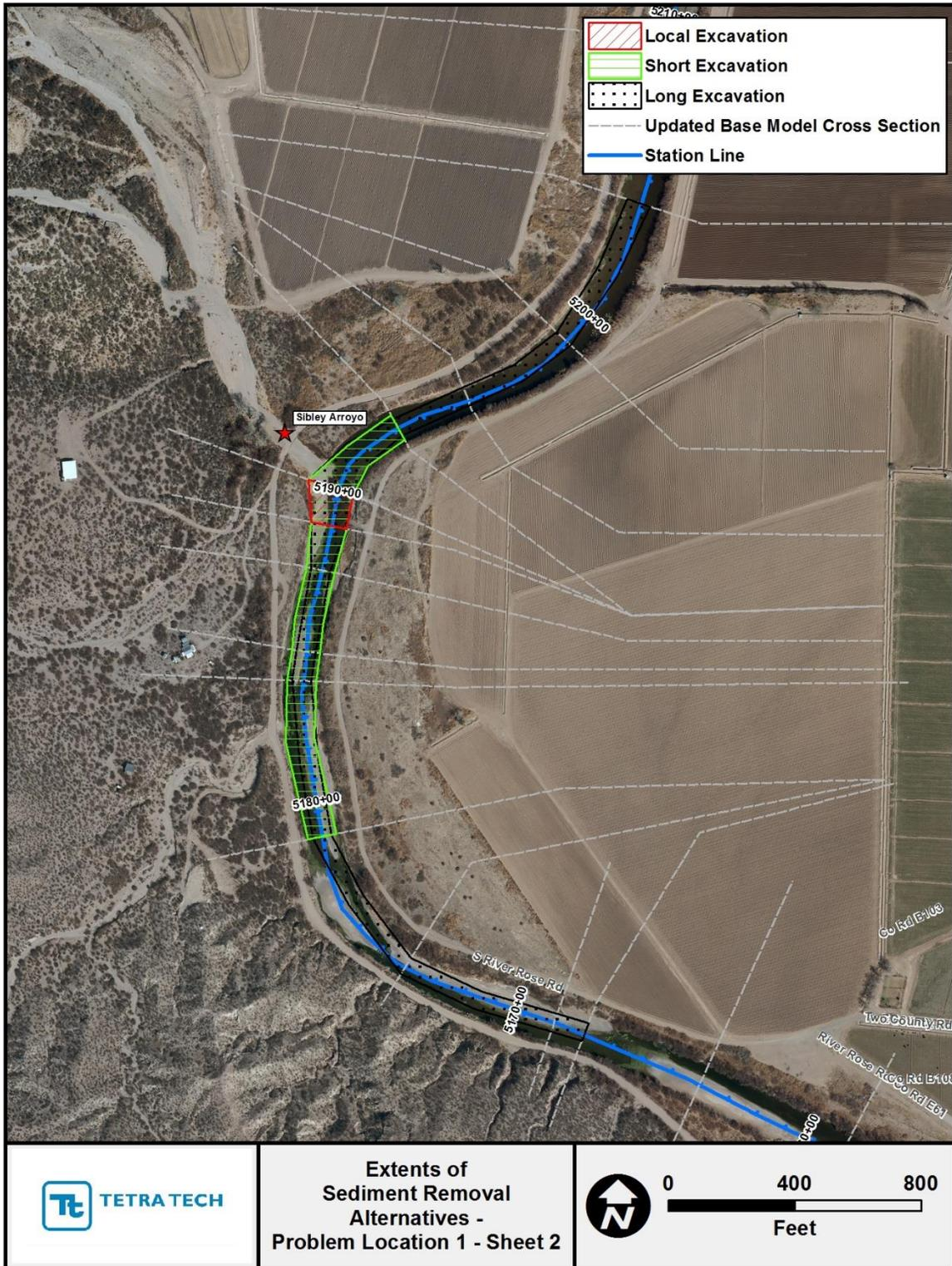
Figure G.2.2. Mapping showing extents of the localized, short and long sediment-removal alternatives at Problem Location 1 (Sheet 2).
