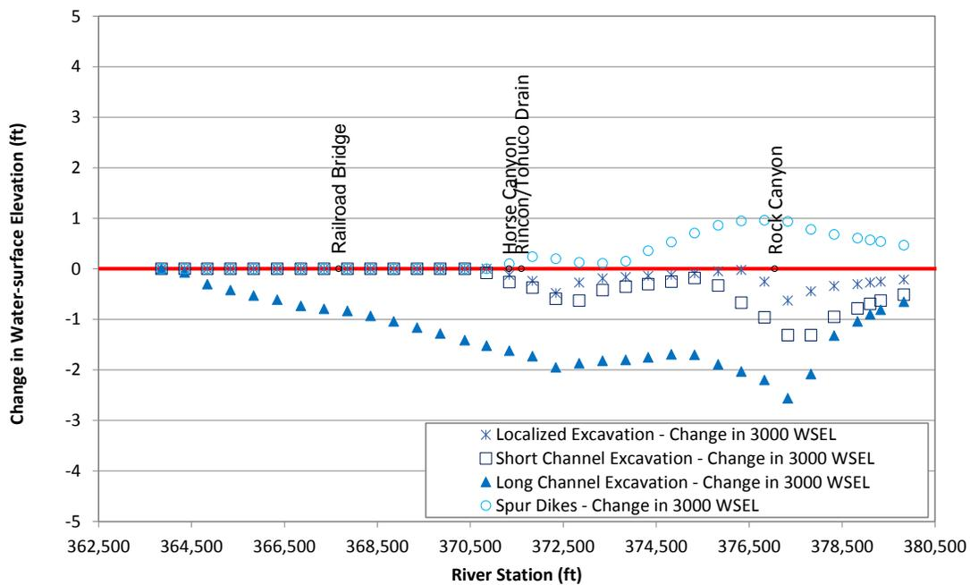
Figure L.36. Predicted change in water-surface elevation at 3,000 cfs at Problem Location 5 for the alternatives that were evaluated with the steady-state hydraulic model compared to existing (base model) conditions.
