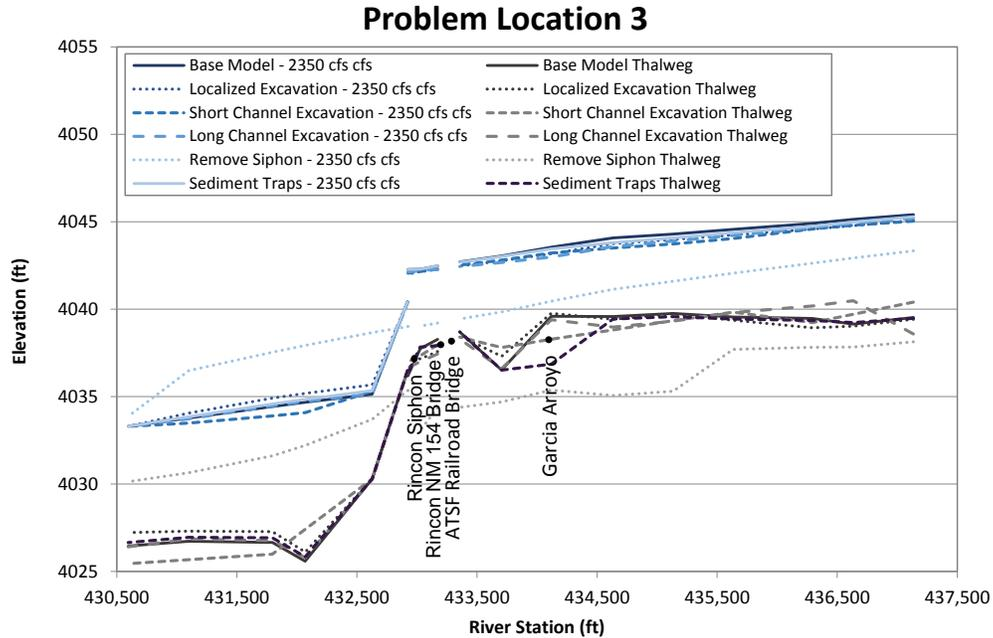
Figure N.9. Predicted water-surface profiles at 2,350 cfs at Problem Location 3 representing long-term conditions based on hydraulic modeling with the predicted geometry at the end of the sediment-transport simulations of the base and alternative conditions.
