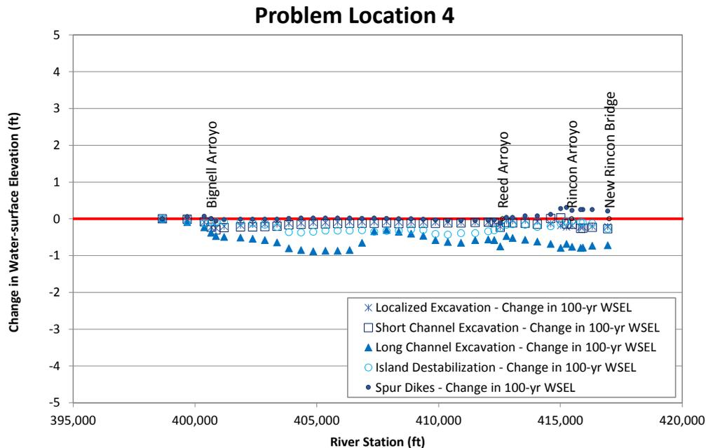
Figure N.16. Predicted change in long-term water-surface elevation at the 100-year peak flow relative to the base condition at Problem Location 4 for the alternatives that were evaluated with the steady-state hydraulic model compared to existing (base model) conditions.
