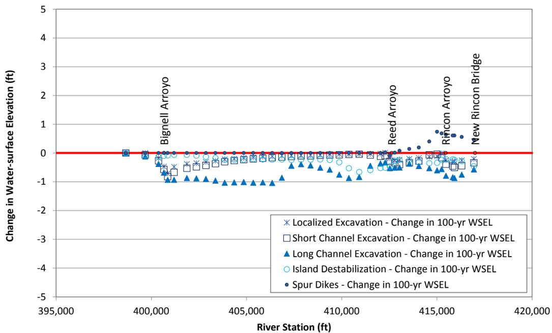
Figure L.32. Predicted change in water-surface elevation at the routed 100-year peak flow at Problem Location 4 for the alternatives that were evaluated with the steady-state hydraulic model compared to existing (base model) conditions.
