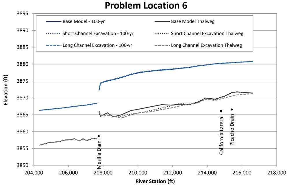
Figure N.23. Predicted water-surface profiles at the 100-year peak flow at Problem Location 6 representing long-term conditions based on hydraulic modeling with the predicted geometry at the end of the sediment-transport simulations of the base and alternative conditions.
