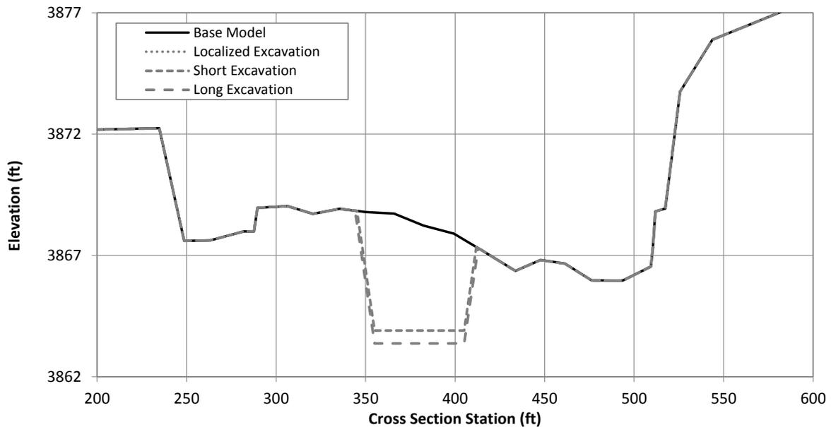
Figure G.1.28. Typical cross section at Problem Location 6 showing the existing (Base Model) channel geometry and excavated geometry under the localized, short and long excavation scenarios (River Station 210162.5).
