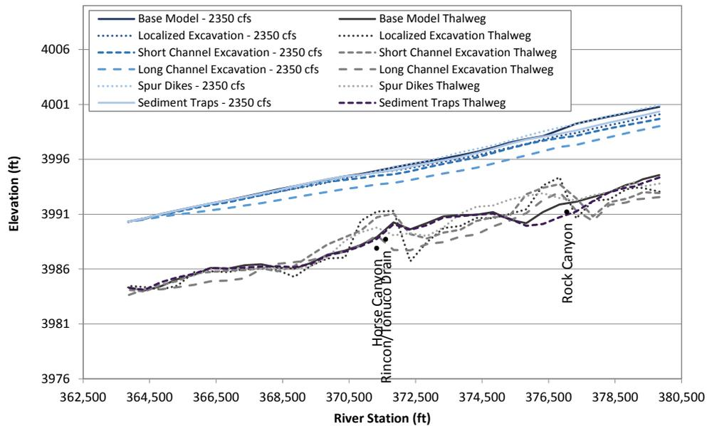
Figure N.17. Predicted water-surface profiles at 2,350 cfs at Problem Location 5 representing long-term conditions based on hydraulic modeling with the predicted geometry at the end of the sediment-transport simulations of the base and alternative conditions.
