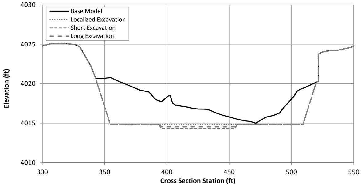
Figure G.1.17. Typical cross section at Problem Location 4 showing the existing (Base Model) channel geometry and excavated geometry under the localized, short and long excavation scenarios (River Station 412284.1).
