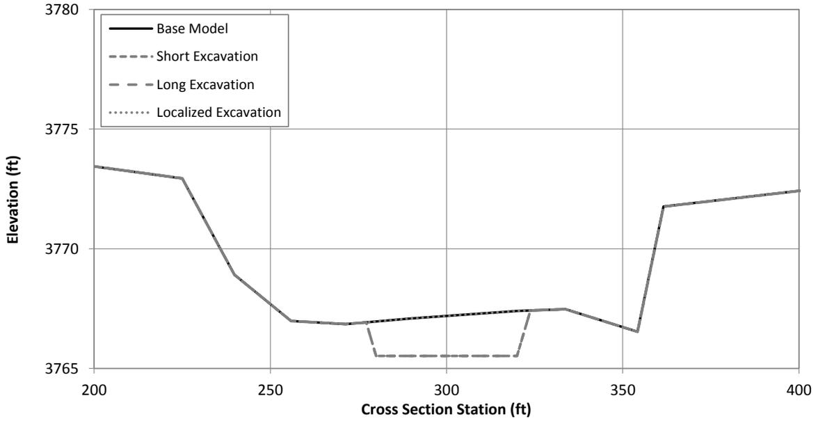
Figure G.1.32. Typical cross section at Problem Location 7 showing the existing (Base Model) channel geometry and excavated geometry under the localized, short and long excavation scenarios (River Station 79425.6).
