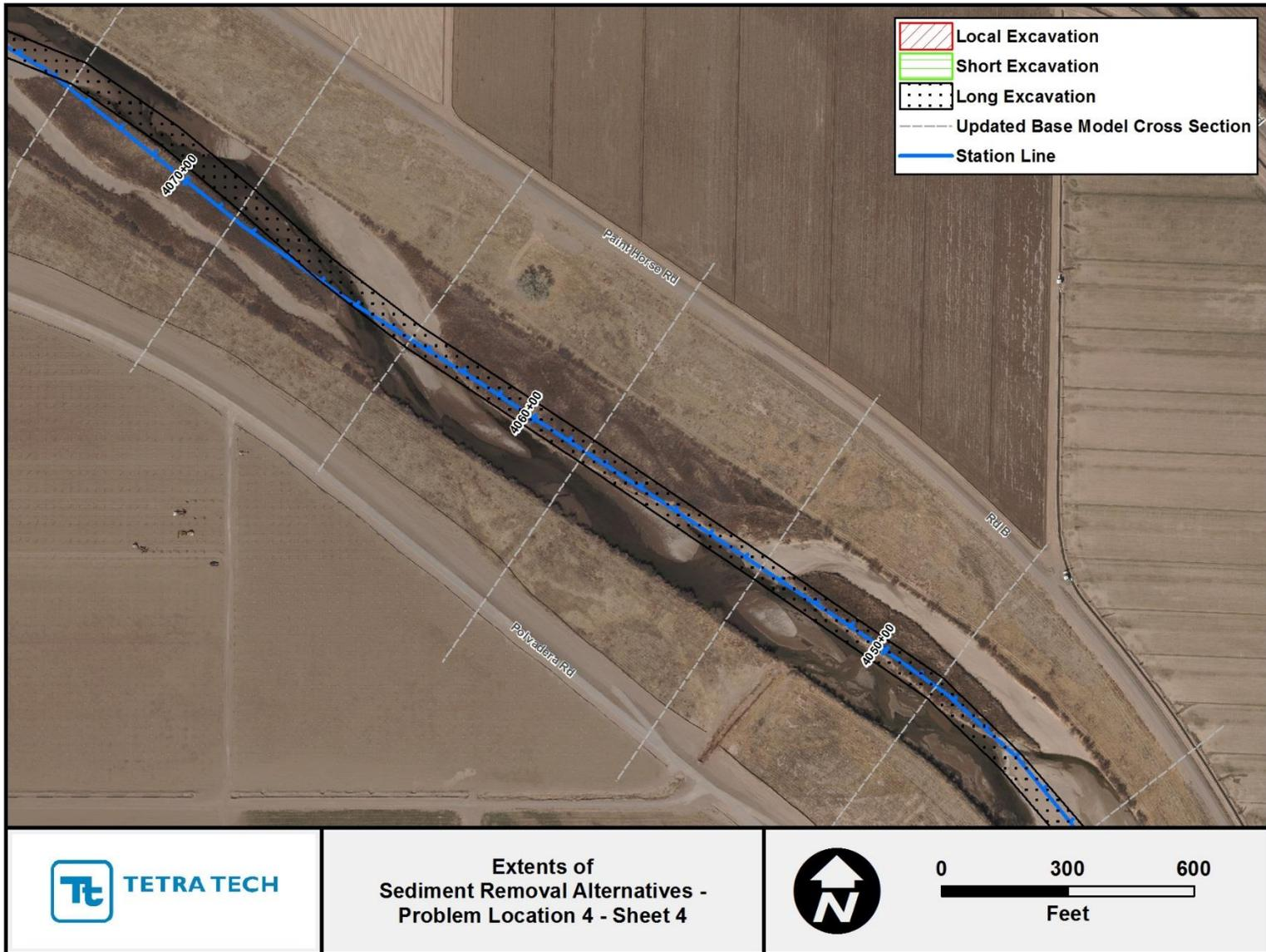
Figure G.2.12. Mapping showing extents of the localized, short and long sediment-removal alternatives at Problem Location 4 (Sheet 4).
