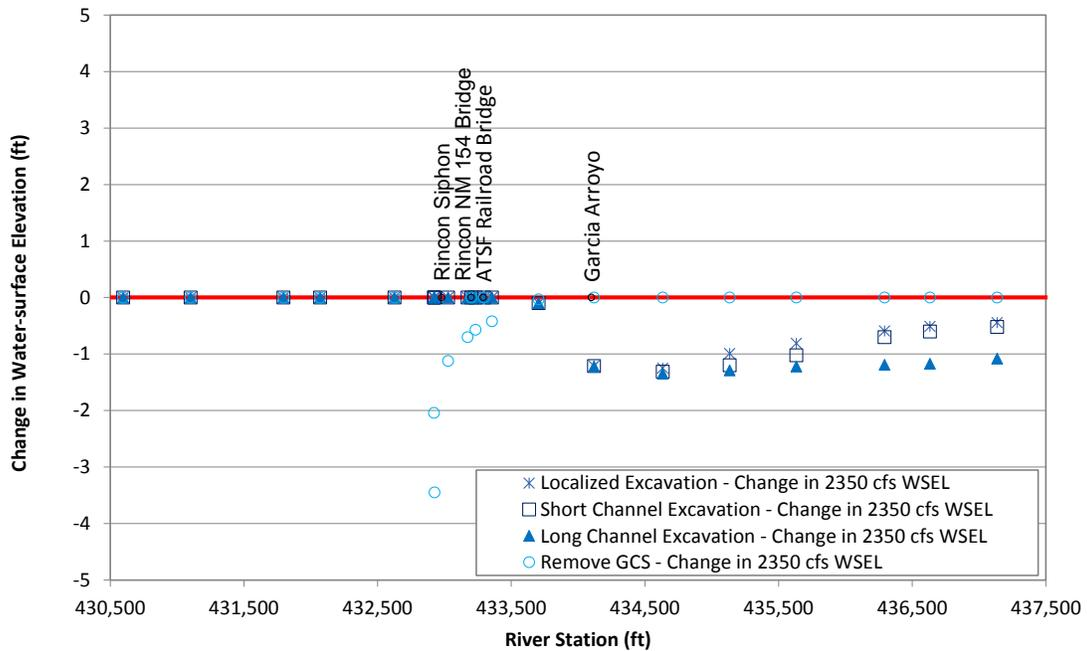
Figure L.18. Predicted change in water-surface elevation at 2,350 cfs at Problem Location 3 for the alternatives that were evaluated with the steady-state hydraulic model compared to existing (base model) conditions.
