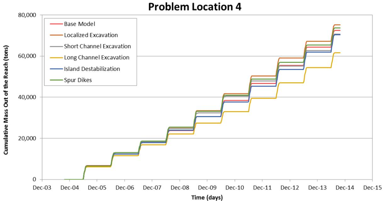
Figure M.2.13. Predicted cumulative mass delivered from the downstream of the model reach at Problem Location 4 from the sediment-transport simulations of the base and alternative conditions.
