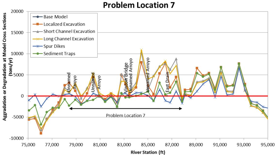
Figure M.1.7. Spatial profiles showing the predicted cumulative mass of aggradation or degradation at the end of the sediment-transport simulations for base alternative conditions at Problem Location 7.
