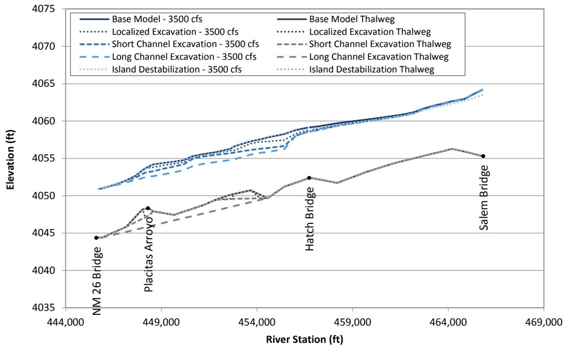
Figure L.13. Predicted water-surface profiles at 3,500 cfs at Problem Location 2 under existing (base model) conditions and for the alternatives that were evaluated with the steady-state hydraulic model.
