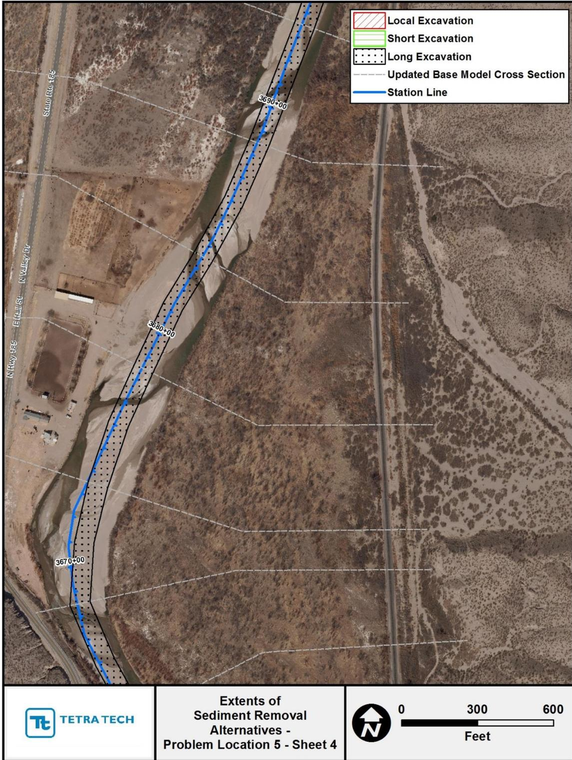
Figure G.2.18. Mapping showing extents of the localized, short and long sediment-removal alternatives at Problem Location 5 (Sheet 4).
