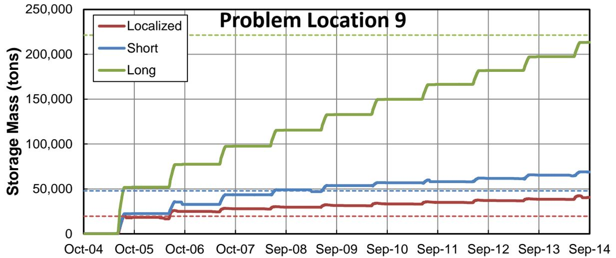
Figure M.2.35. Predicted cumulative mass of aggradation or degradation over time along the extents of the excavated reaches at Problem Location 9 from the sediment-transport simulations of the sediment-removal alternatives. The dashed lines represent the excavated mass for each type of excavation.
