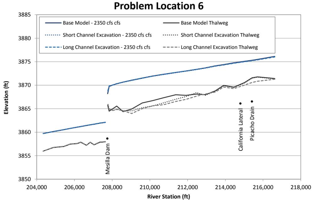
Figure N.21. Predicted water-surface profiles at 2,350 cfs at Problem Location 6 representing long-term conditions based on hydraulic modeling with the predicted geometry at the end of the sediment-transport simulations of the base and alternative conditions.
