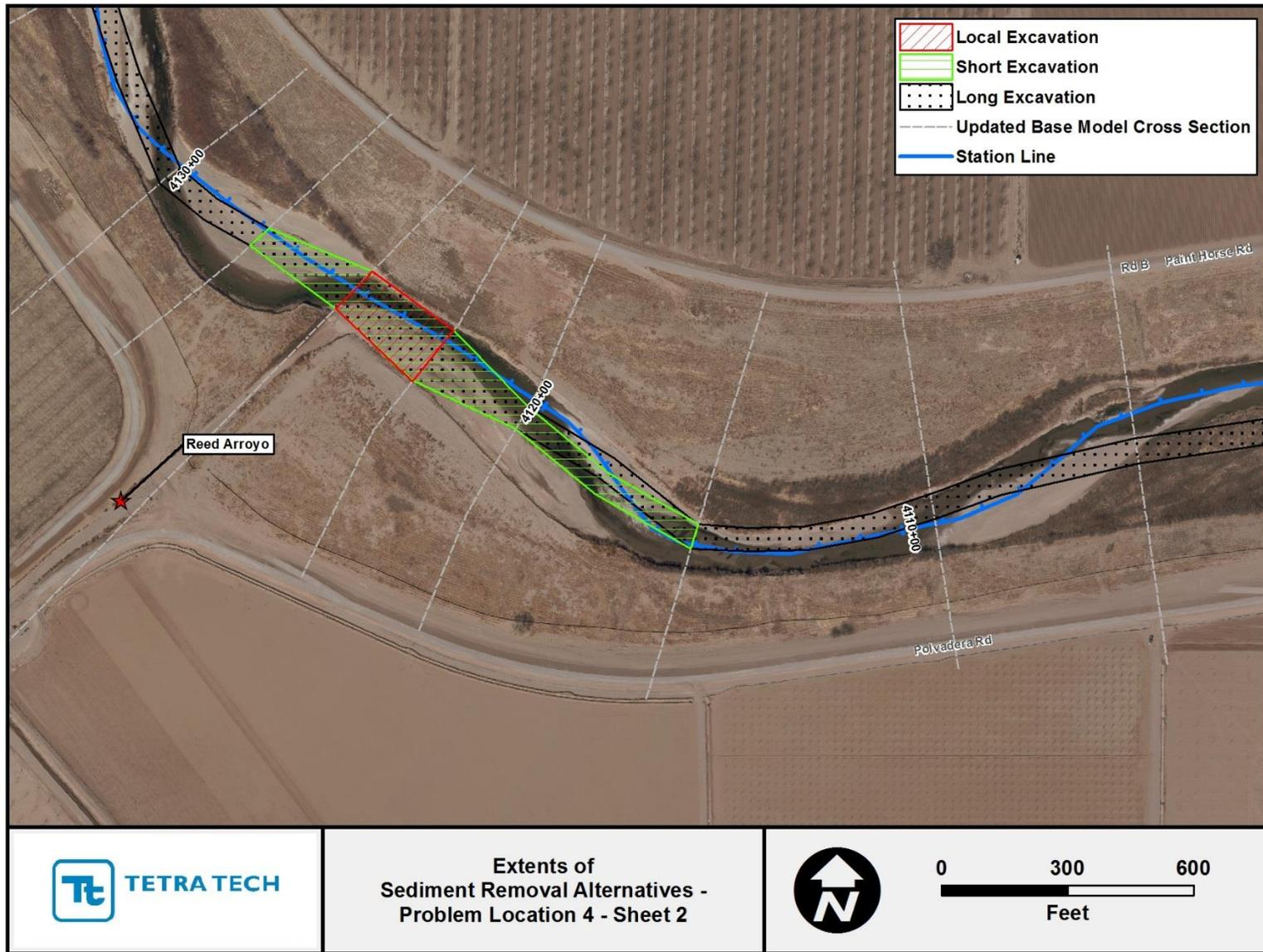
Figure G.2.10. Mapping showing extents of the localized, short and long sediment-removal alternatives at Problem Location 4 (Sheet 2).
