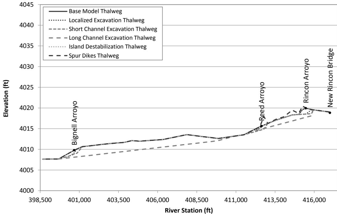
Figure G.1.15. Existing (Base Model) and excavation thalweg profiles at Problem Location 4.
