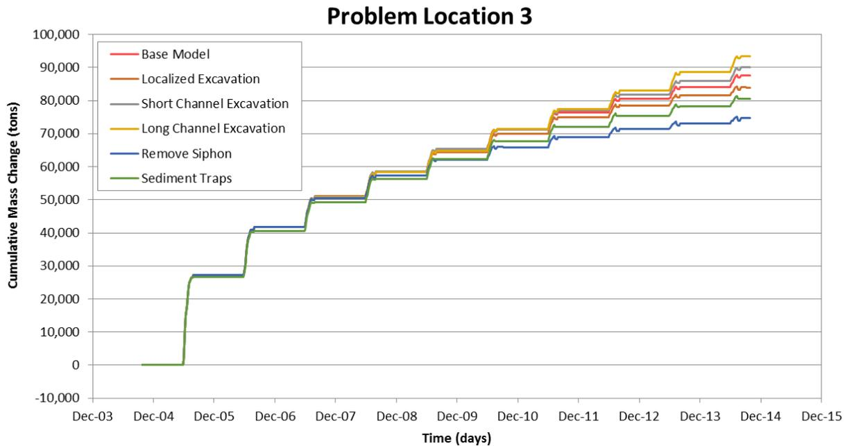
Figure M.2.3. Predicted cumulative mass of aggradation or degradation over time along the modeled reach at Problem Location 3 from the sediment-transport simulations of the base and alternative conditions.
