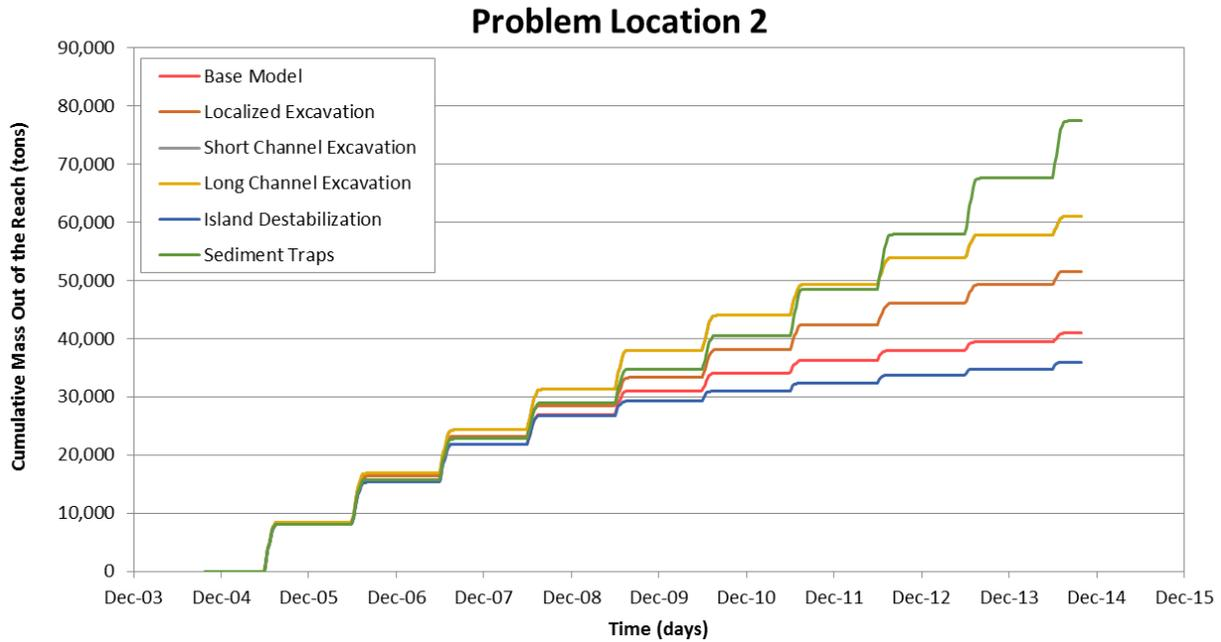
Figure M.2.11. Predicted cumulative mass delivered from the downstream of the model reach at Problem Location 2 from the sediment-transport simulations of the base and alternative conditions.
