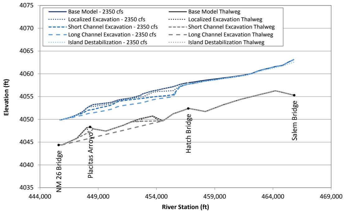
Figure L.9. Predicted water-surface profiles at 2,350 cfs at Problem Location 2 under existing (base model) conditions and for the alternatives that were evaluated with the steady-state hydraulic model.
