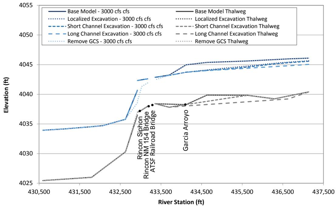
Figure L.19. Predicted water-surface profiles at 3,000 cfs at Problem Location 3 under existing (base model) conditions and for the alternatives that were evaluated with the steady-state hydraulic model.
