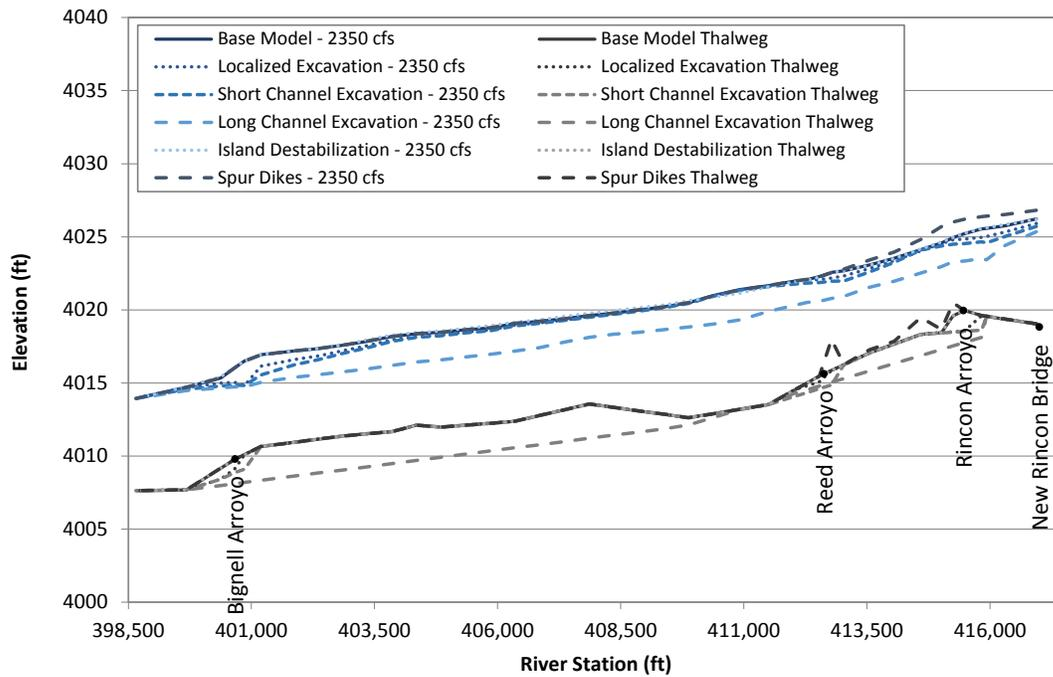
Figure L.25. Predicted water-surface profiles at 2,350 cfs at Problem Location 4 under existing (base model) conditions and for the alternatives that were evaluated with the steady-state hydraulic model.
