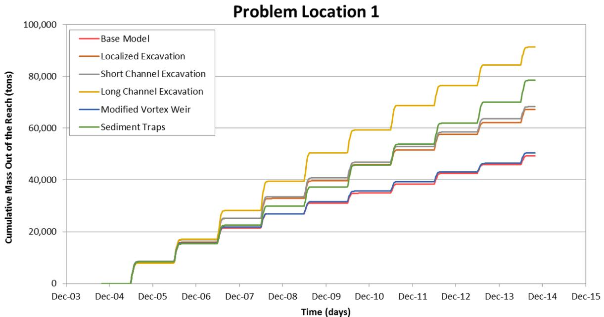
Figure M.2.10. Predicted cumulative mass delivered from the downstream of the model reach at Problem Location 1 from the sediment-transport simulations of the base and alternative conditions.
