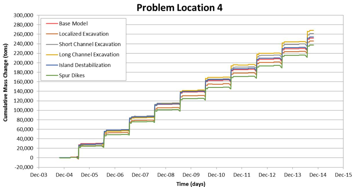
Figure M.2.4. Predicted cumulative mass of aggradation or degradation over time along the modeled reach at Problem Location 4 from the sediment-transport simulations of the base and alternative conditions.
