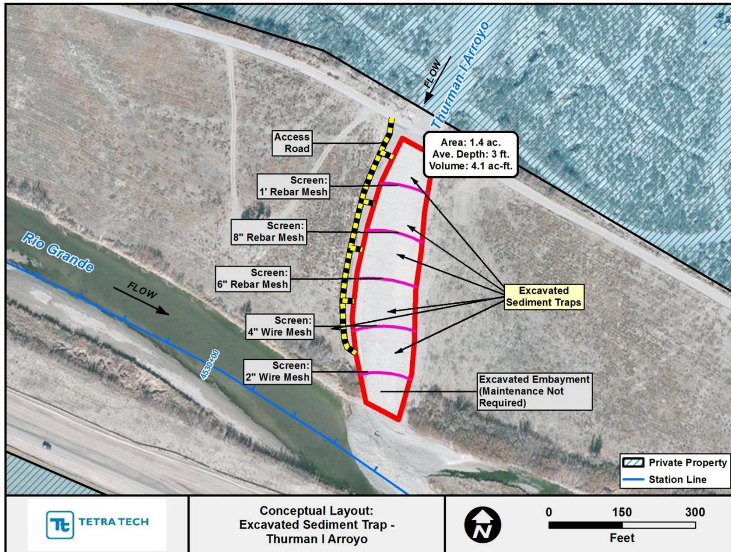
Figure H.5. Conceptual layout of sediment trap for Thurman I Arroyo at Problem Location 2.
