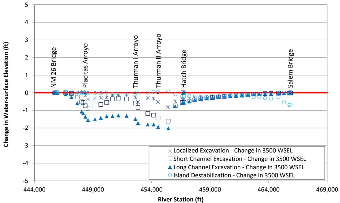
Figure L.14. Predicted change in water-surface elevation at 3,500 cfs at Problem Location 2 for the alternatives that were evaluated with the steady-state hydraulic model compared to existing (base model) conditions.
