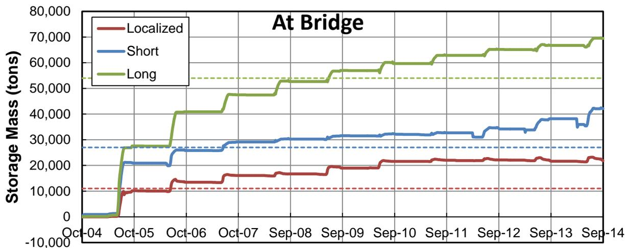
Figure M.2.34. Predicted cumulative mass of aggradation or degradation over time along the extents of the excavated reaches at Country Club Bridge (Problem Location 8) from the sediment-transport simulations of the sediment-removal alternatives. The dashed lines represent the excavated mass for each type of excavation.
