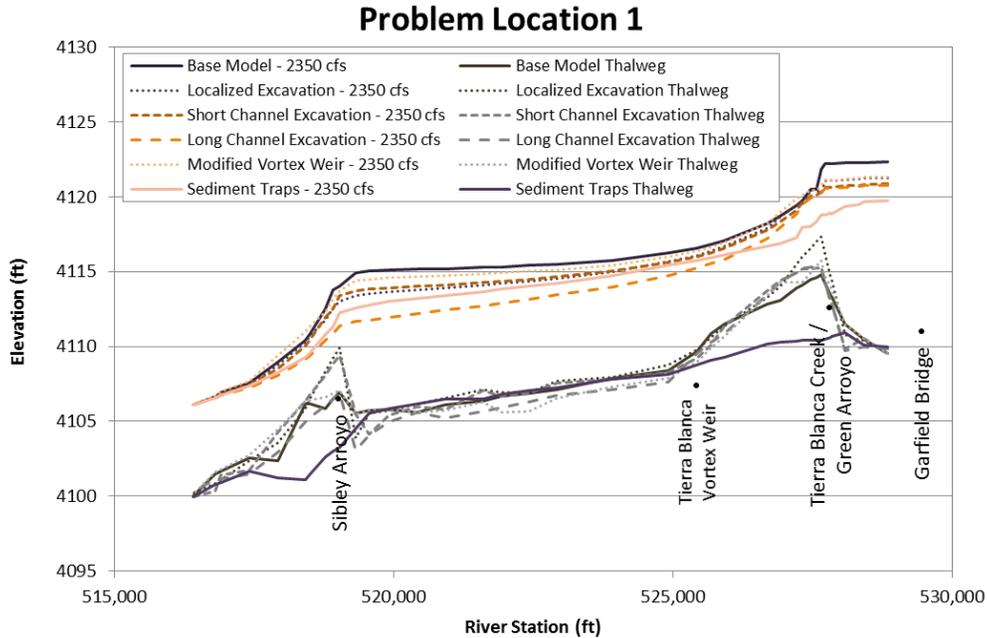
Figure N.1. Predicted water-surface profiles at 2,350 cfs at Problem Location 1 representing long-term conditions based on hydraulic modeling with the predicted geometry at the end of the sediment-transport simulations of the base and alternative conditions.
