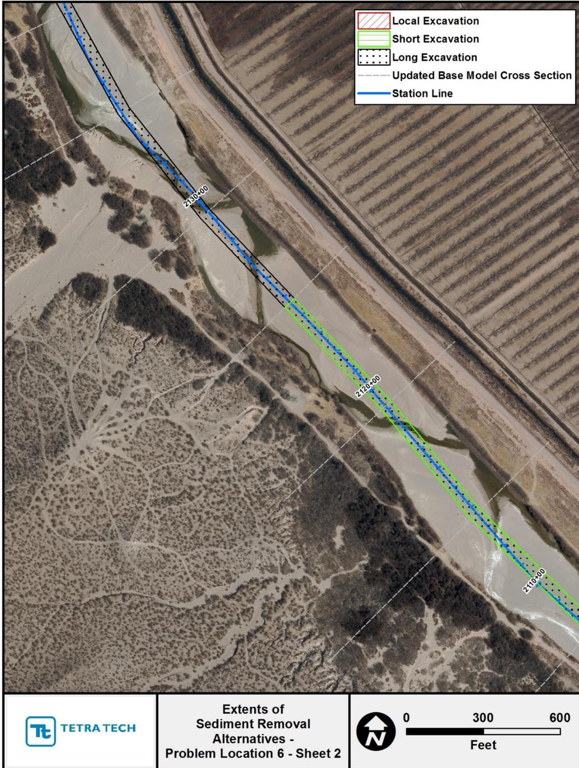
Figure G.2.21. Mapping showing extents of the localized, short and long sediment-removal alternatives at Problem Location 6 (Sheet 2).
