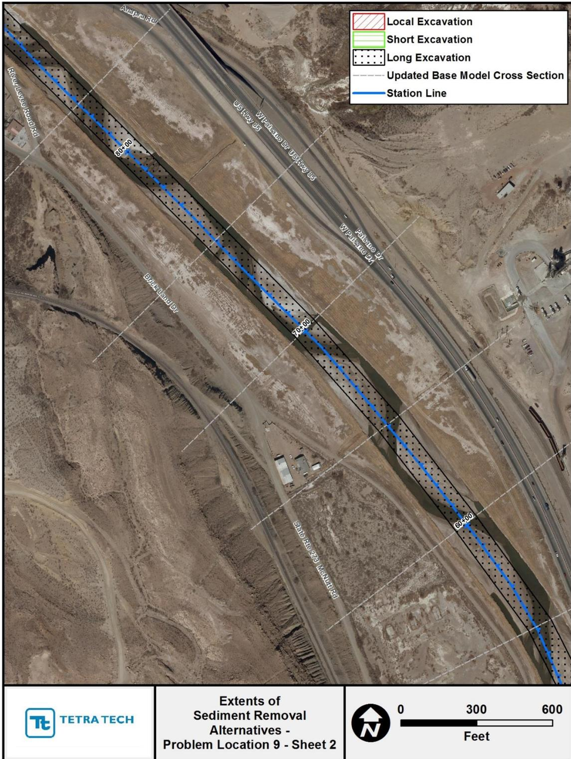
Figure G.2.32. Mapping showing extents of the localized, short and long sediment-removal alternatives at Problem Location 9 (Sheet 2).
