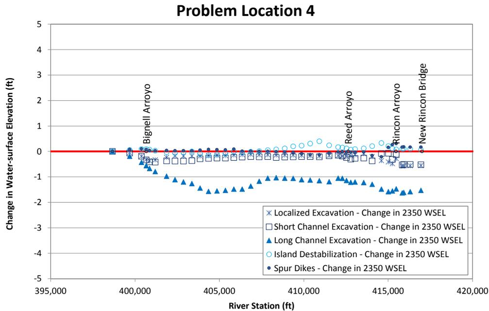
Figure N.14. Predicted change in long-term water-surface elevation at 2,350 cfs relative to the base condition at Problem Location 4 for the alternatives that were evaluated with the steady-state hydraulic model compared to existing (base model) conditions.
