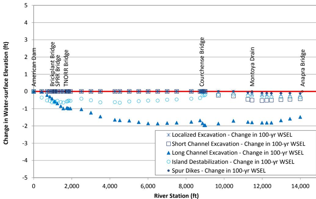
Figure L.72. Predicted change in water-surface elevation at the routed 100-year peak flow at Problem Location 9 for the alternatives that were evaluated with the steady-state hydraulic model compared to existing (base model) conditions.
