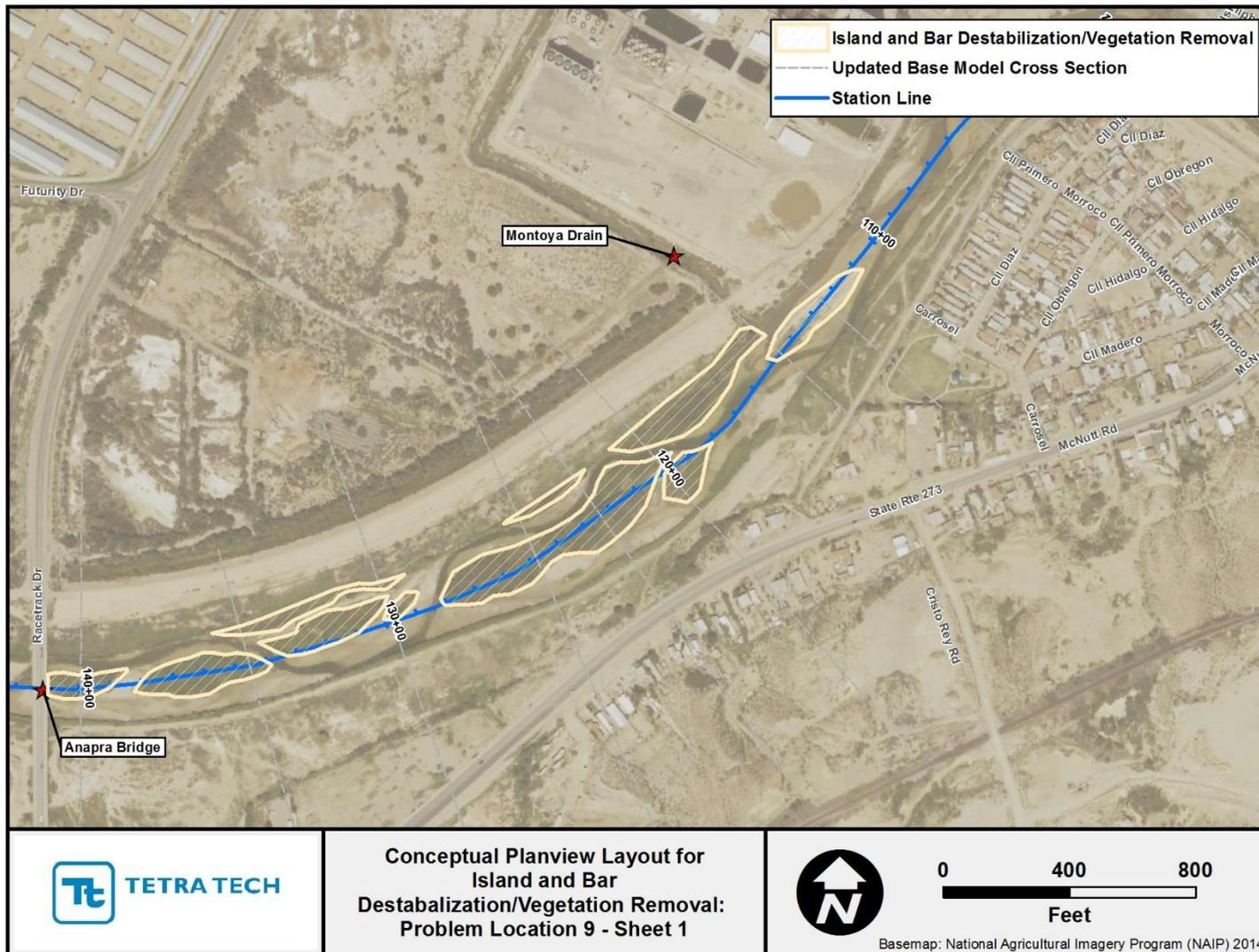
Figure J.12. Aerial photography showing extents of features treated with island/bar destabilization and vegetation removal at Problem Location 9 (Sheet 1).
