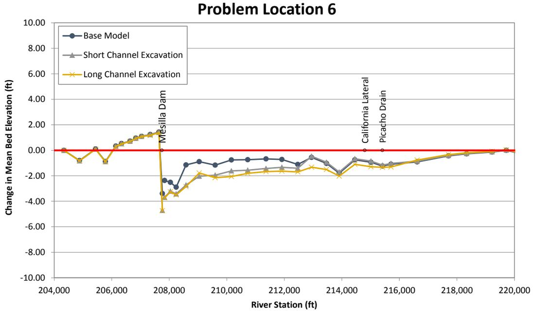
Figure M.1.15. Spatial profiles showing the predicted change in mean bed elevation at the end of the sediment-transport simulations for base alternative conditions at Problem Location 6.
