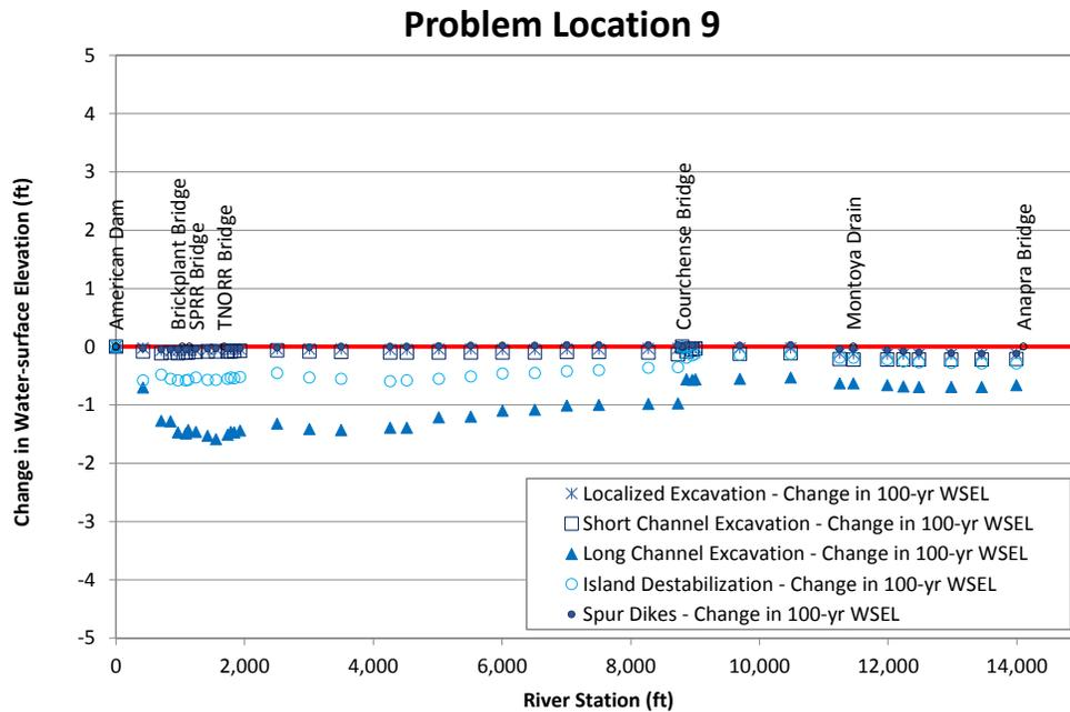
Figure N.36. Predicted change in long-term water-surface elevation at the 100-year peak flow relative to the base condition at Problem Location 9 for the alternatives that were evaluated with the steady-state hydraulic model compared to existing (base model) conditions.
