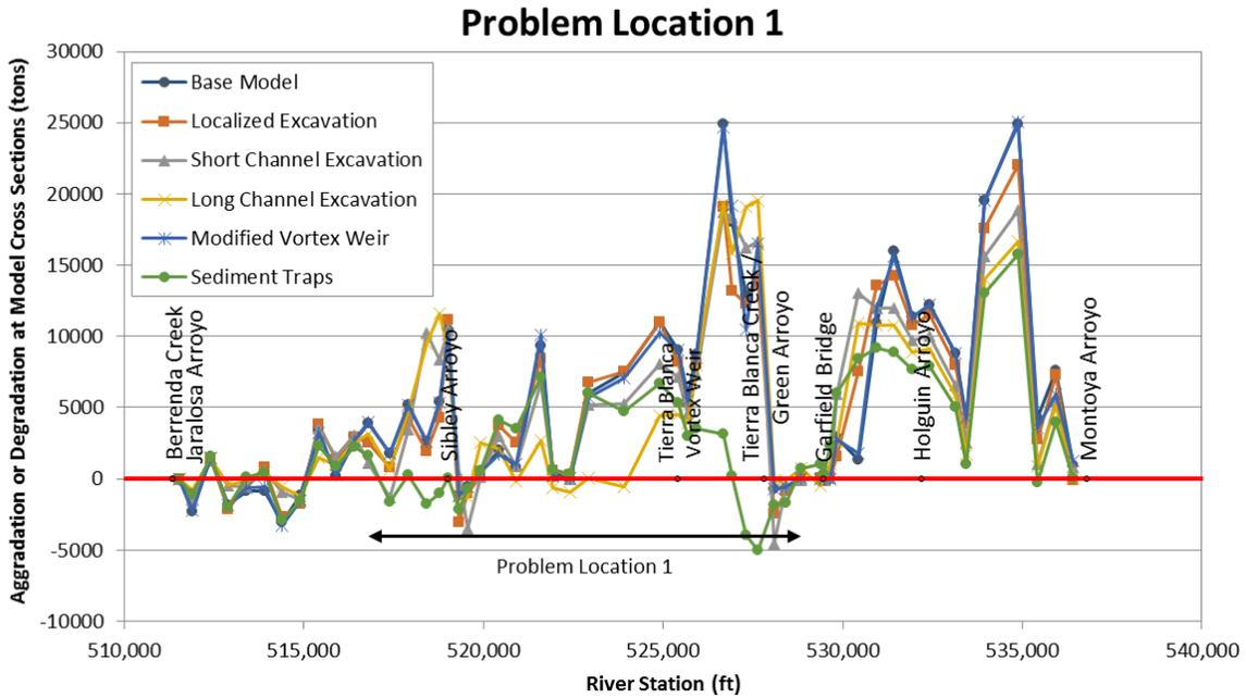
Figure M.1.1. Spatial profiles showing the predicted cumulative mass of aggradation or degradation at the end of the sediment-transport simulations for base alternative conditions at Problem Location 1.
