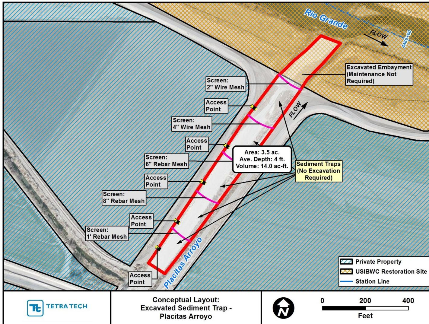
Figure H.6. Conceptual layout of sediment trap for Placitas Arroyo at Problem Location 2.
