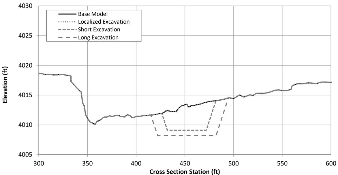
Figure G.1.18. Typical cross section at Problem Location 4 showing the existing (Base Model) channel geometry and excavated geometry under the localized, short and long excavation scenarios (River Station 400857.9).
