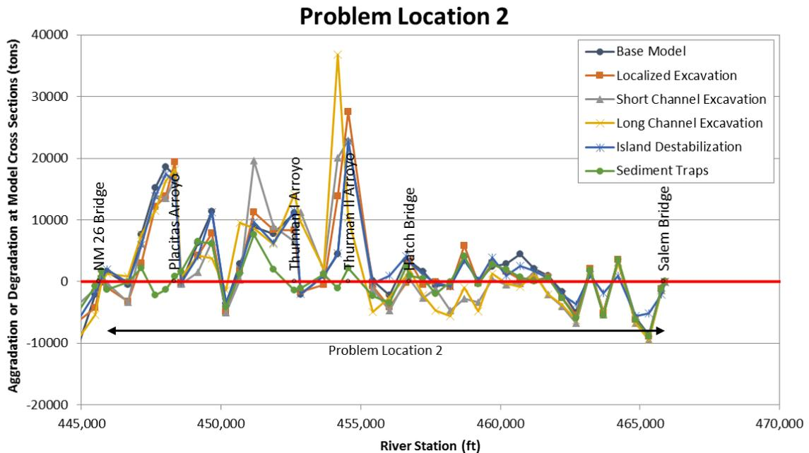
Figure M.1.2. Spatial profiles showing the predicted cumulative mass of aggradation or degradation at the end of the sediment-transport simulations for base alternative conditions at Problem Location 2.
