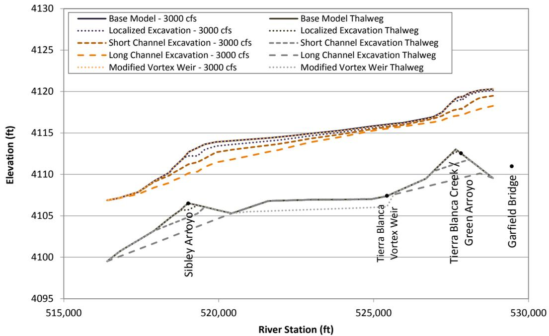
Figure L.3. Predicted water-surface profiles at 3,000 cfs at Problem Location 1 under existing (base model) conditions and for the alternatives that were evaluated with the steady-state hydraulic model.
