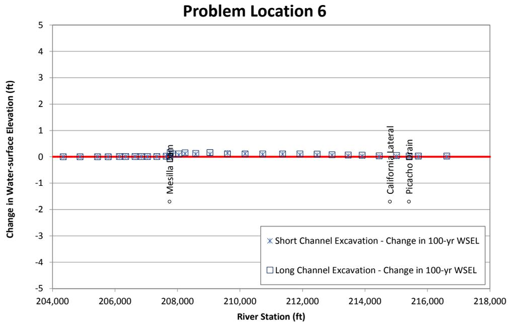
Figure N.24. Predicted change in long-term water-surface elevation at the 100-year peak flow relative to the base condition at Problem Location 6 for the alternatives that were evaluated with the steady-state hydraulic model compared to existing (base model) conditions.
