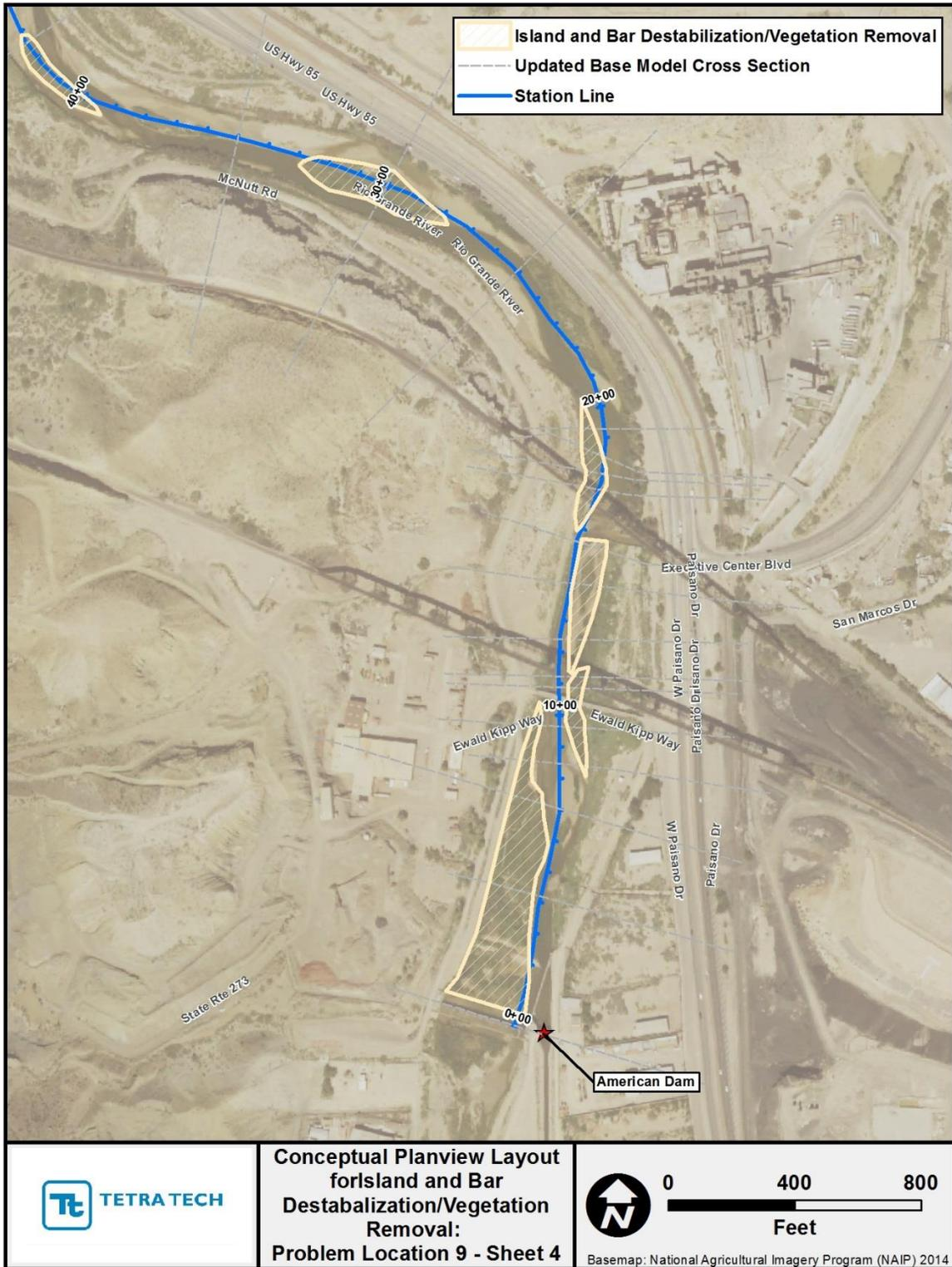
Figure J.15. Aerial photography showing extents of features treated with island/bar destabilization and vegetation removal at Problem Location 9 (Sheet 4).
