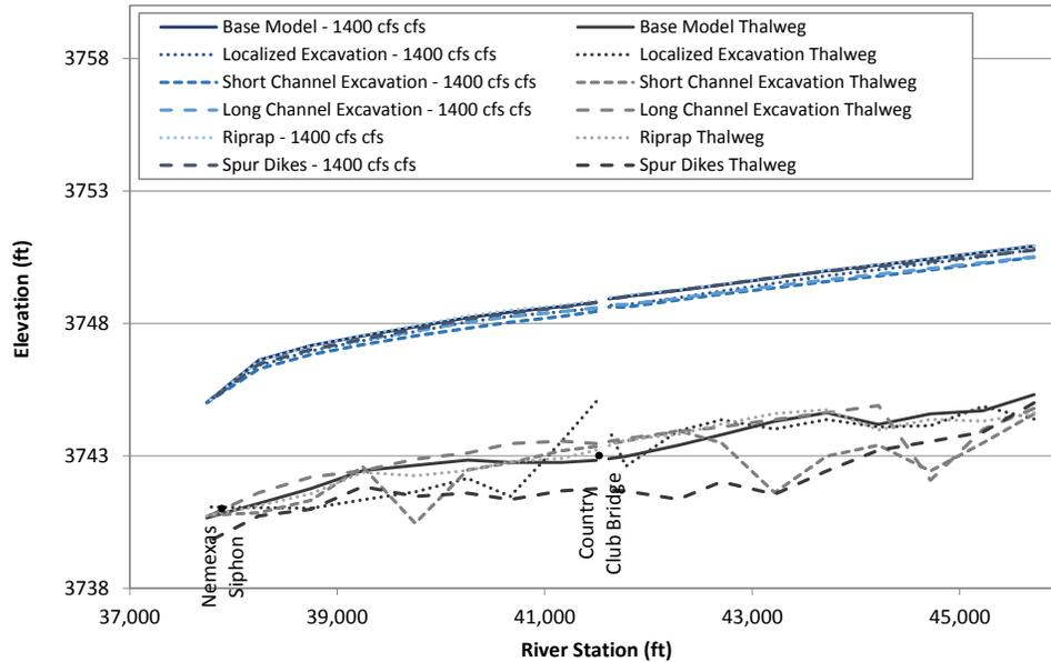
Figure N.29. Predicted water-surface profiles at 1,400 cfs at Problem Location 8 representing long-term conditions based on hydraulic modeling with the predicted geometry at the end of the sediment-transport simulations of the base and alternative conditions.
