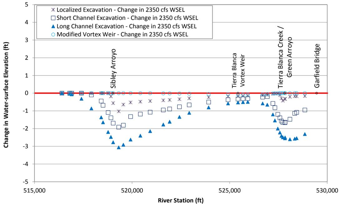
Figure L.2. Predicted change in water-surface elevation at 2,350 cfs at Problem Location 1 for the alternatives that were evaluated with the steady-state hydraulic model compared to existing (base model) conditions.
