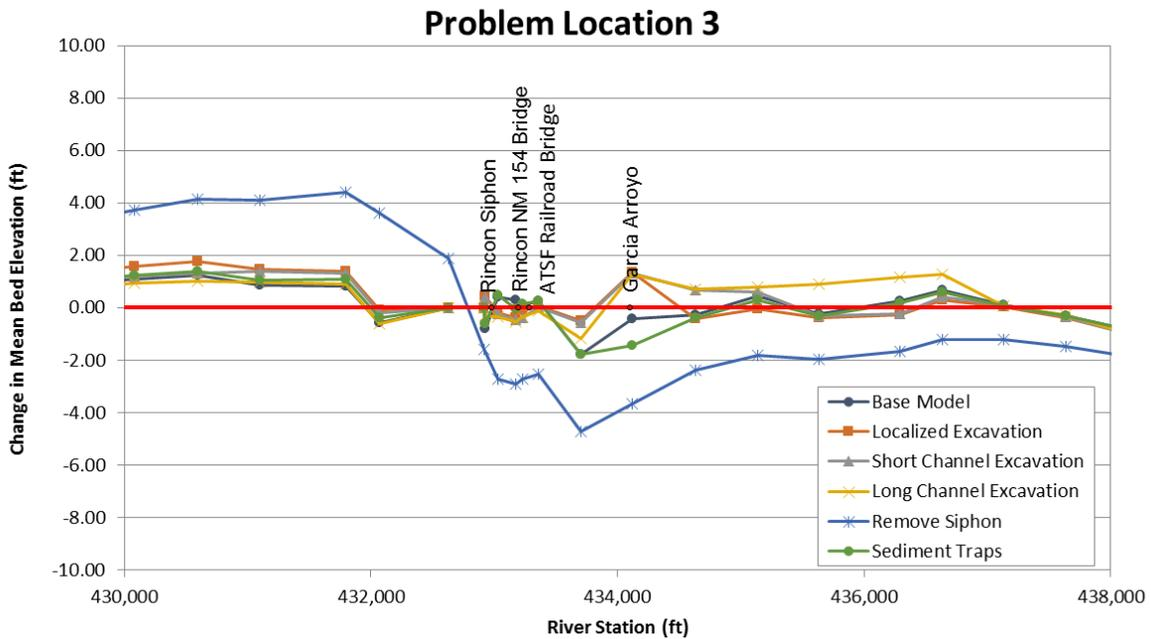
Figure M.1.12. Spatial profiles showing the predicted change in mean bed elevation at the end of the sediment-transport simulations for base alternative conditions at Problem Location 3.
