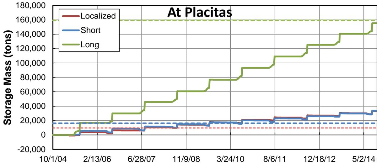
Figure M.2.23. Predicted cumulative mass of aggradation or degradation over time along the extents of the excavated reaches at Placitas Arroyo (Problem Location 2) from the sediment-transport simulations of the sediment-removal alternatives. The dashed lines represent the excavated mass for each type of excavation.
