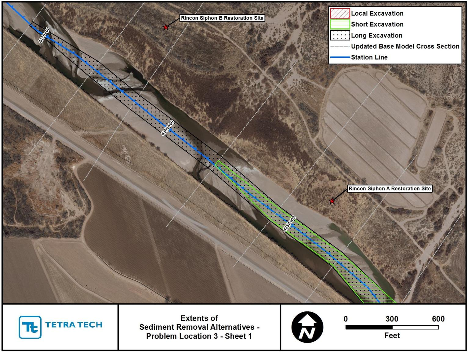
Figure G.2.7. Mapping showing extents of the localized, short and long sediment-removal alternatives at Problem Location 3 (Sheet 1).
