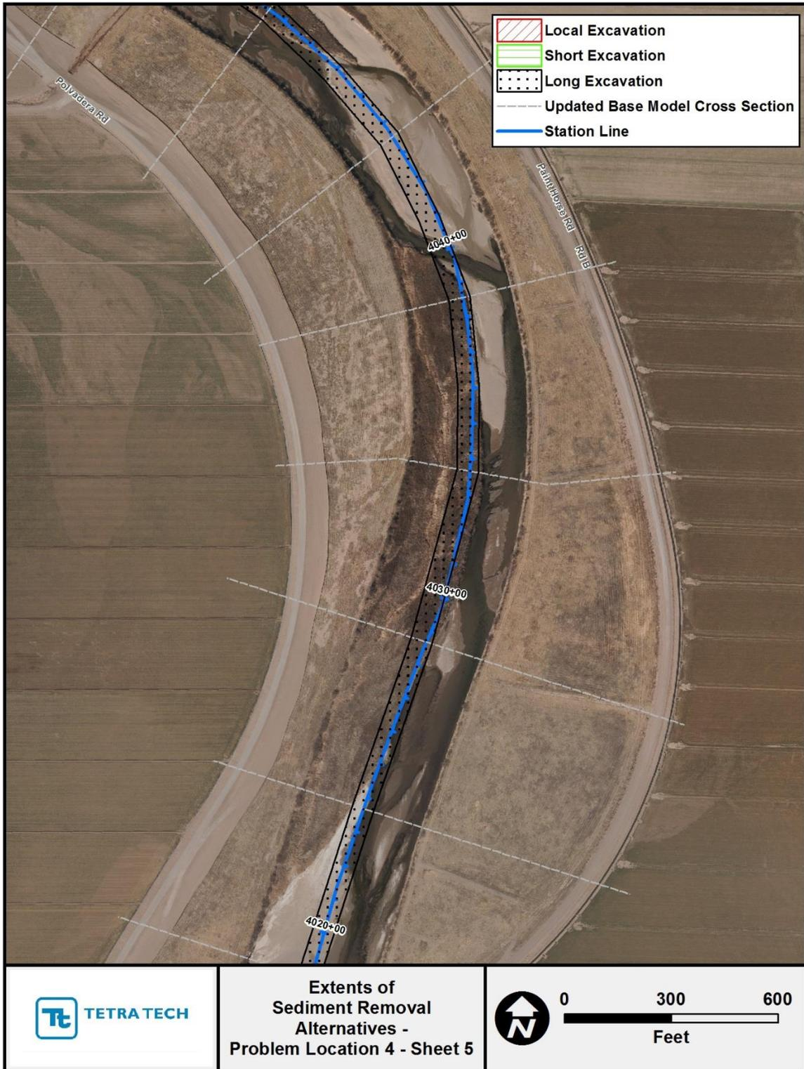
Figure G.2.13. Mapping showing extents of the localized, short and long sediment-removal alternatives at Problem Location 4 (Sheet 5).
