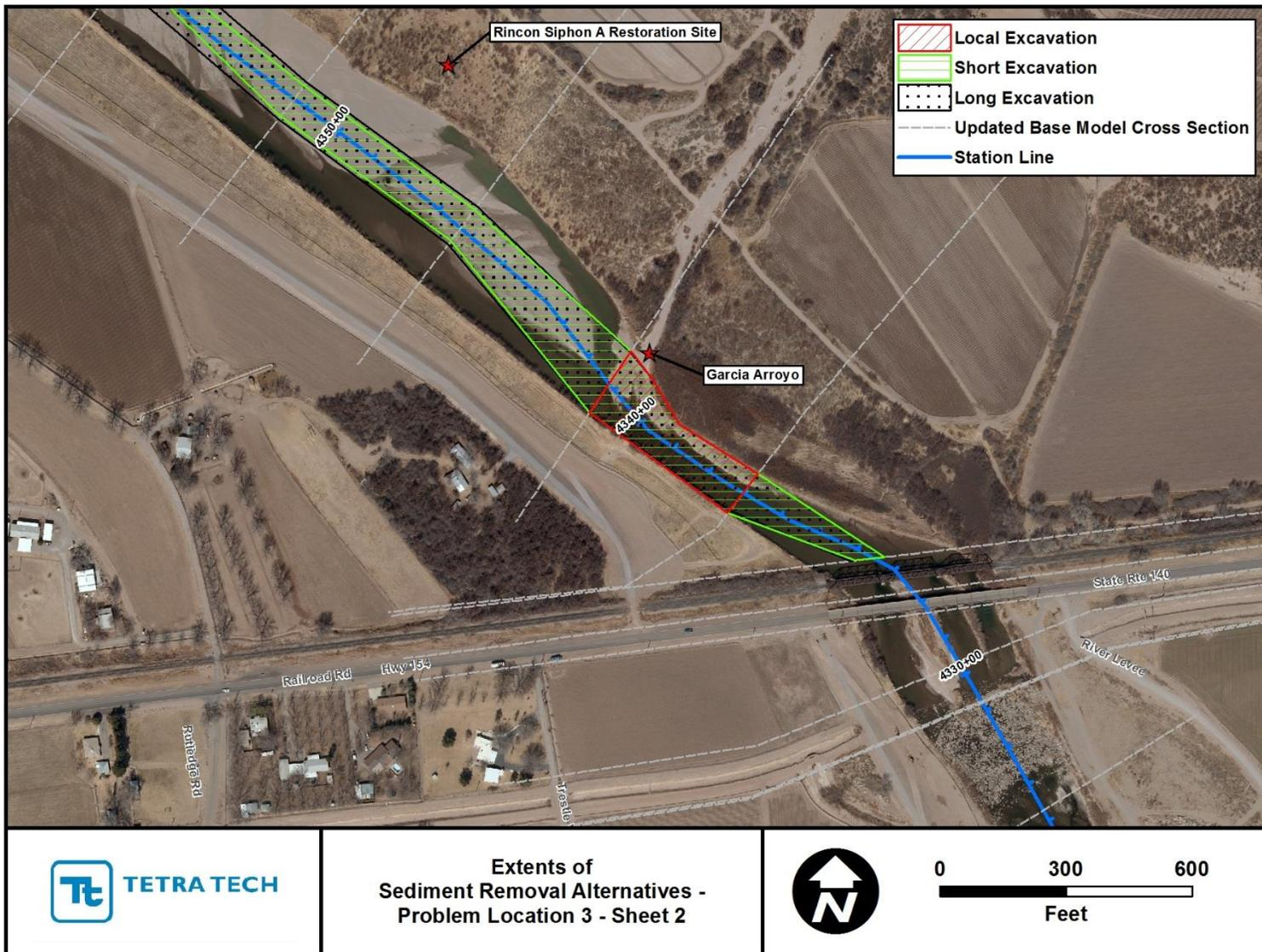
Figure G.2.8. Mapping showing extents of the localized, short and long sediment-removal alternatives at Problem Location 3 (Sheet 2).
