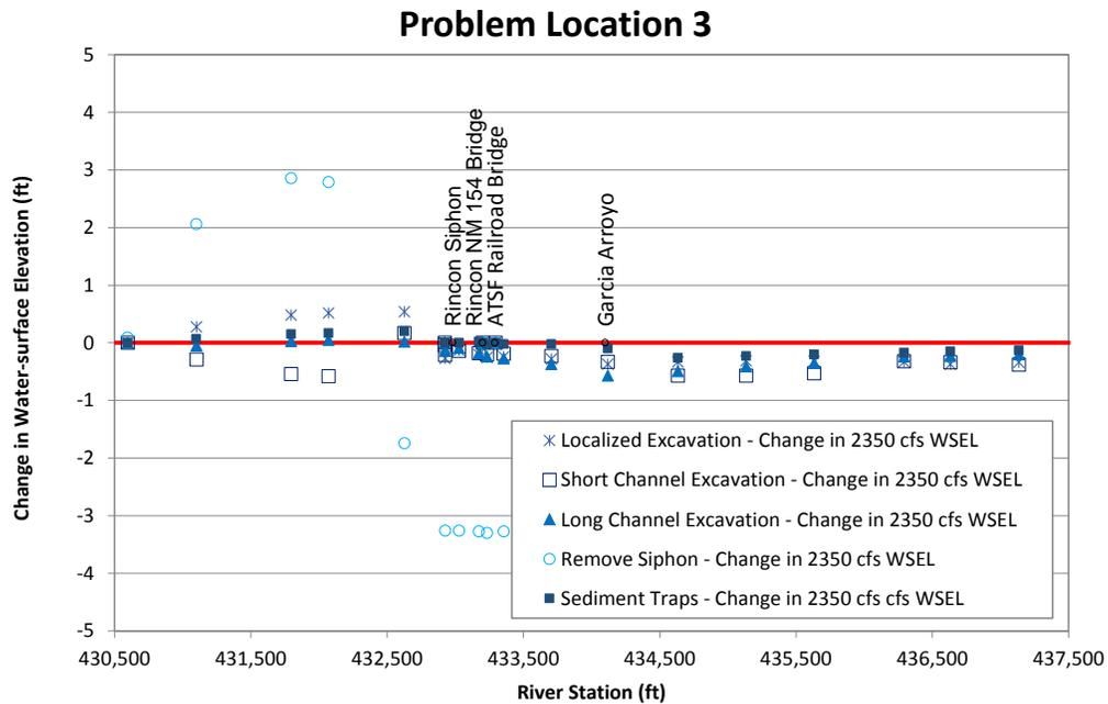
Figure N.10. Predicted change in long-term water-surface elevation at 2,350 cfs relative to the base condition at Problem Location 3 for the alternatives that were evaluated with the steady-state hydraulic model compared to existing (base model) conditions.
