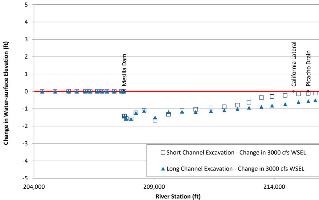
Figure L.44. Predicted change in water-surface elevation at 3,000 cfs at Problem Location 6 for the alternatives that were evaluated with the steady-state hydraulic model compared to existing (base model) conditions.
