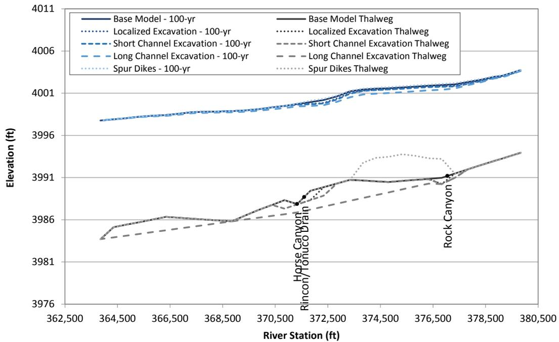
Figure L.39. Predicted water-surface profiles at the routed 100-year peak flow at Problem Location 5 under existing (base model) conditions and for the alternatives that were evaluated with the steady-state hydraulic model.
