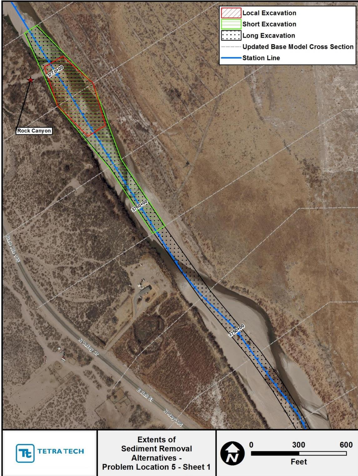
Figure G.2.15. Mapping showing extents of the localized, short and long sediment-removal alternatives at Problem Location 5 (Sheet 1).
