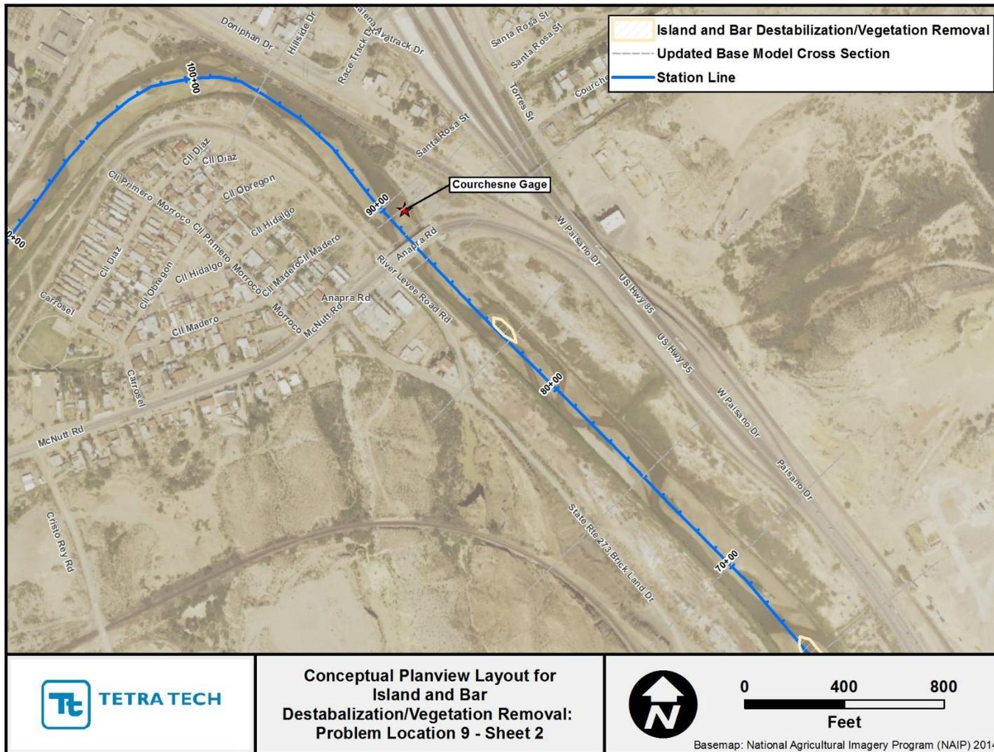
Figure J.13. Aerial photography showing extents of features treated with island/bar destabilization and vegetation removal at Problem Location 9 (Sheet 2).
