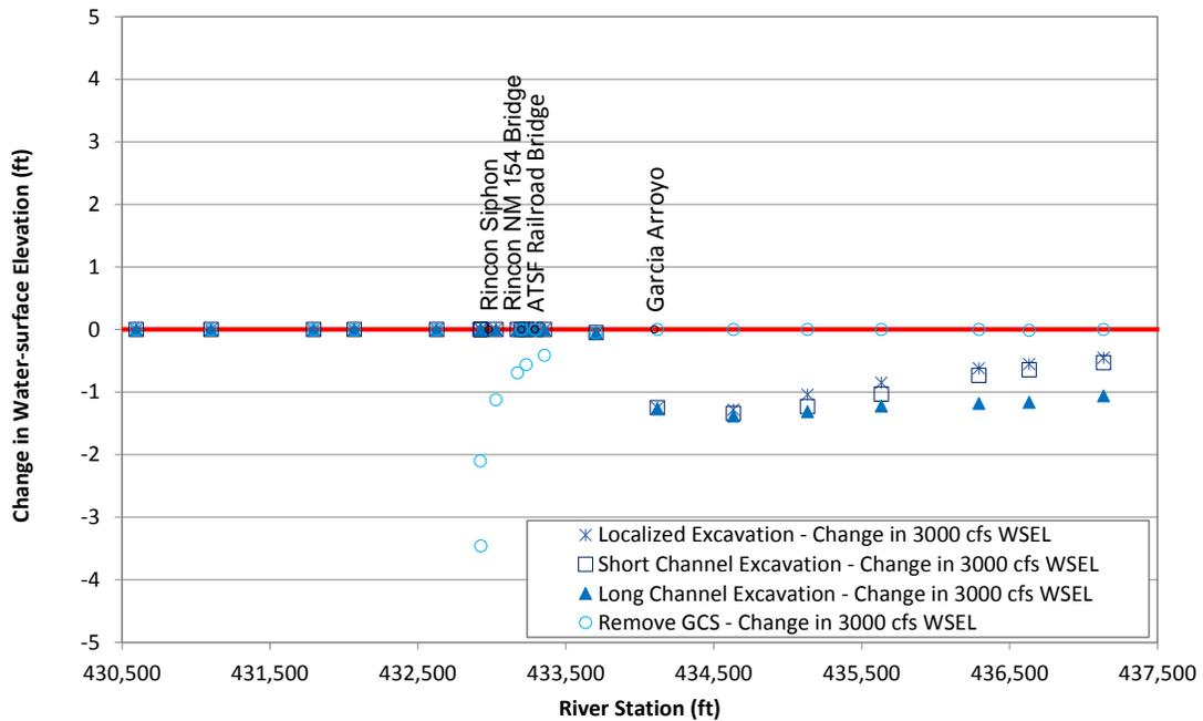
Figure L.20. Predicted change in water-surface elevation at 3,000 cfs at Problem Location 3 for the alternatives that were evaluated with the steady-state hydraulic model compared to existing (base model) conditions.
