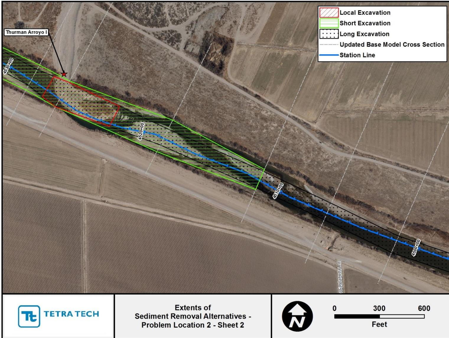
Figure G.2.4. Mapping showing extents of the localized, short and long sediment-removal alternatives at Problem Location 2 (Sheet 2).
