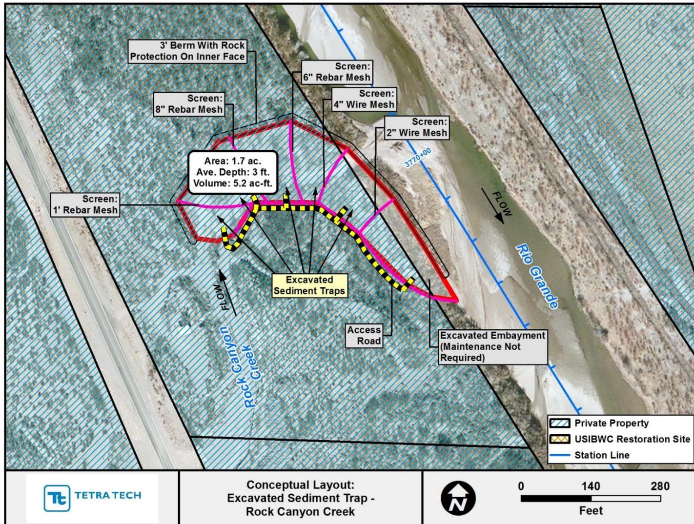
Figure H.8. Conceptual layout of sediment trap for Rock Canyon at Problem Location 5 (see also Figure 23 in the main report).
