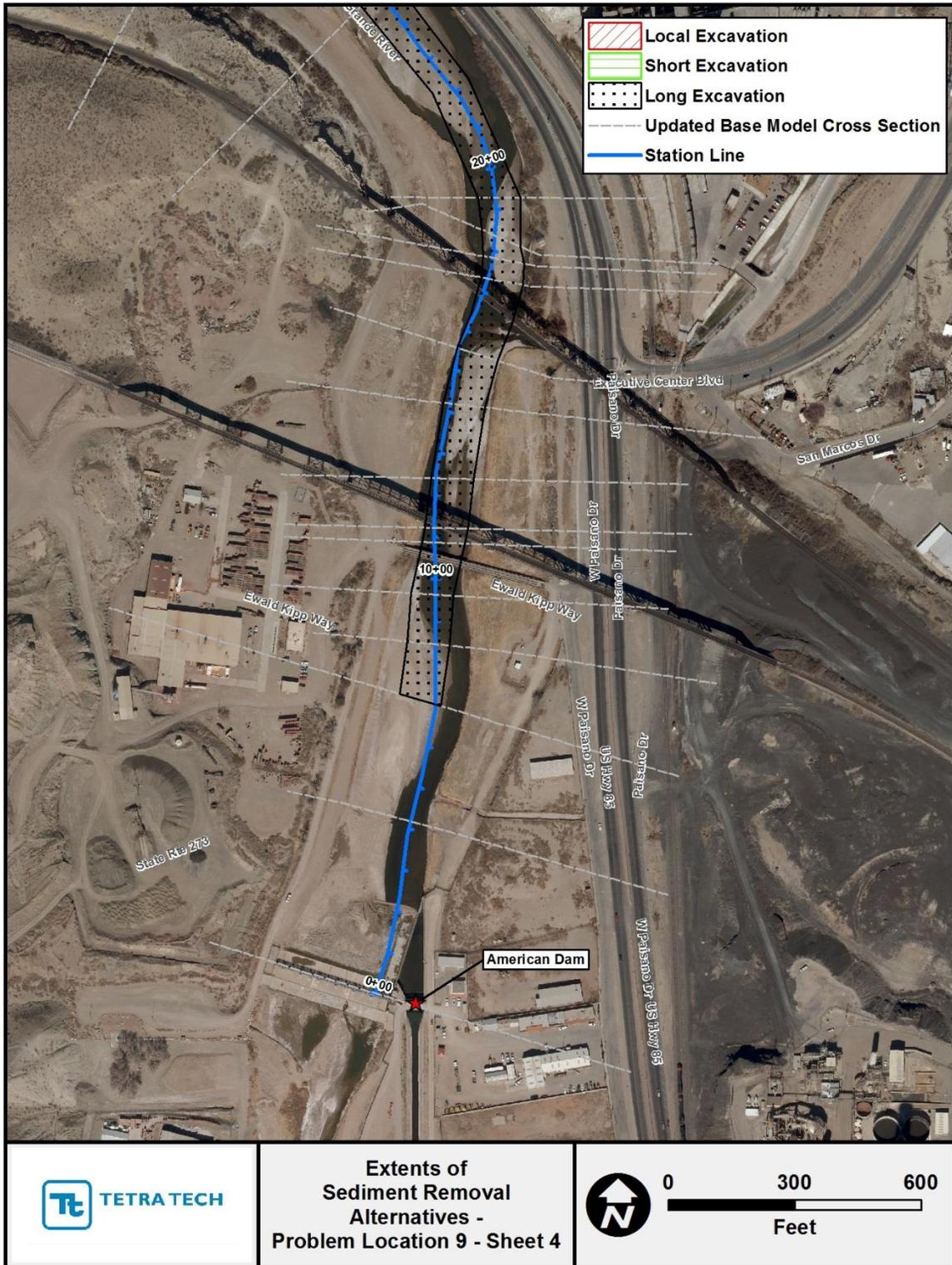
Figure G.2.34. Mapping showing extents of the localized, short and long sediment-removal alternatives at Problem Location 9 (Sheet 4).
