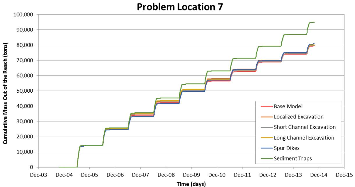
Figure M.2.16. Predicted cumulative mass delivered from the downstream of the model reach at Problem Location 7 from the sediment-transport simulations of the base and alternative conditions.
