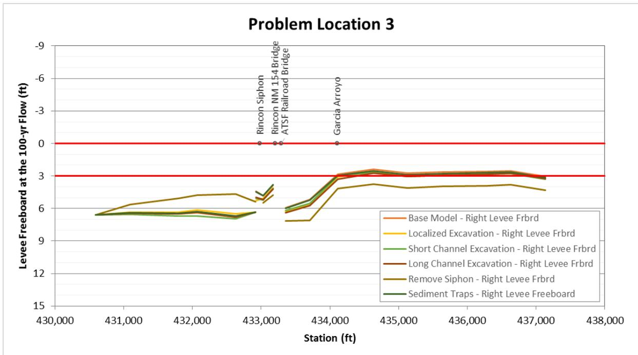
Figure O.2. Predicted levee freeboard during the 100-year flow at Problem Location 3 representing long-term conditions based on hydraulic modeling with the predicted geometry at the end of the sediment-transport simulations of the base and alternative conditions.
