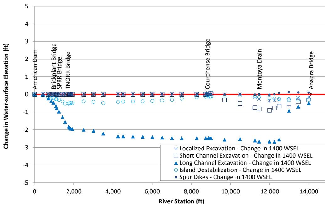
Figure L.66. Predicted change in water-surface elevation at 1,400 cfs at Problem Location 9 for the alternatives that were evaluated with the steady-state hydraulic model compared to existing (base model) conditions.
