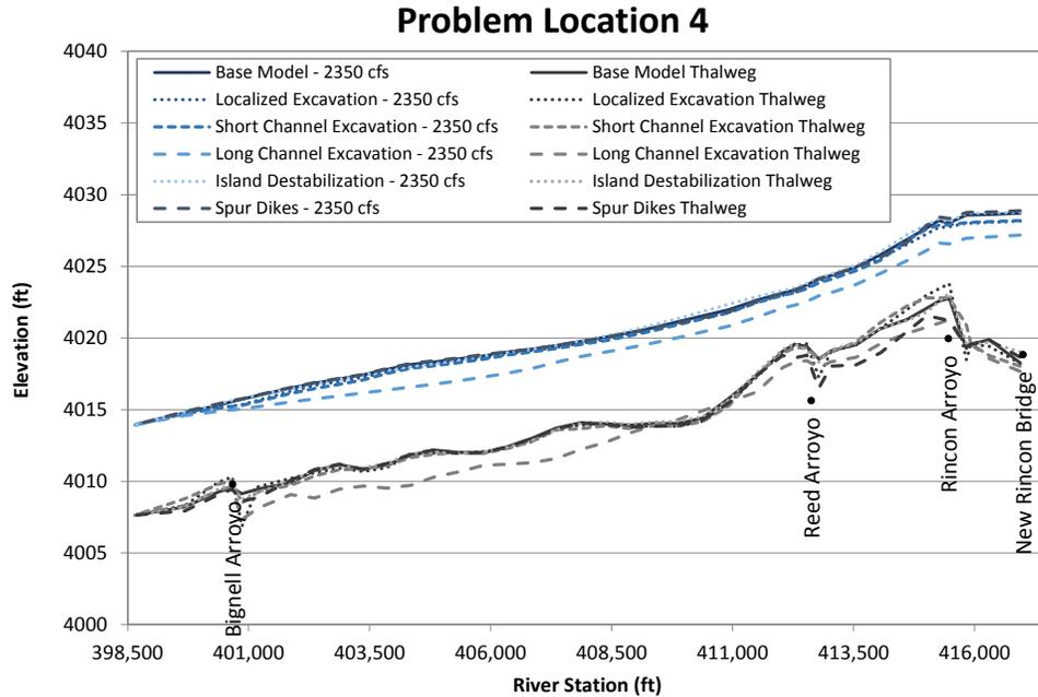
Figure N.13. Predicted water-surface profiles at 2,350 cfs at Problem Location 4 representing long-term conditions based on hydraulic modeling with the predicted geometry at the end of the sediment-transport simulations of the base and alternative conditions.
