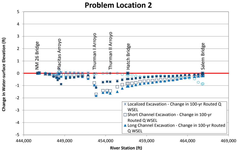
Figure N.8. Predicted change in long-term water-surface elevation at the 100-year peak flow relative to the base condition at Problem Location 2 for the alternatives that were evaluated with the steady-state hydraulic model compared to existing (base model) conditions.
