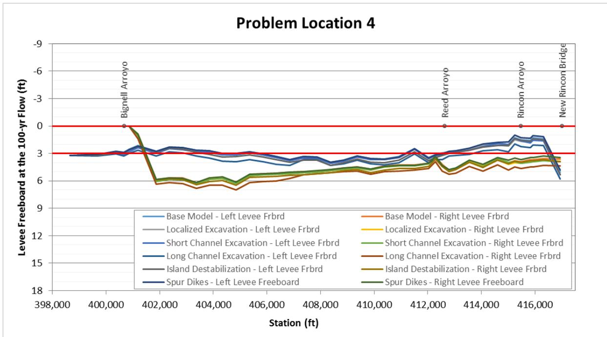
Figure O.3. Predicted levee freeboard during the 100-year flow at Problem Location 4 representing long-term conditions based on hydraulic modeling with the predicted geometry at the end of the sediment-transport simulations of the base and alternative conditions.
