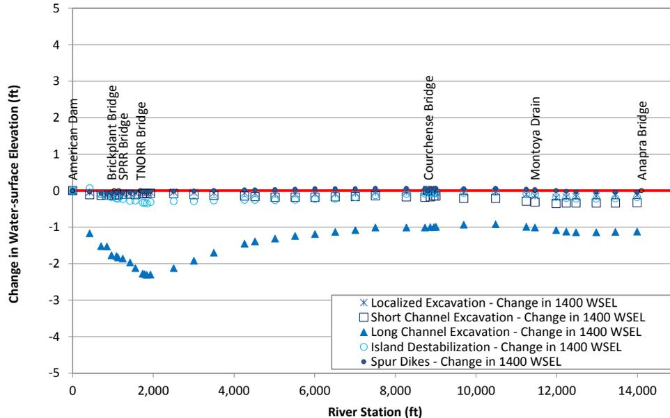
Figure N.34. Predicted change in long-term water-surface elevation at 1,400 cfs relative to the base condition at Problem Location 9 for the alternatives that were evaluated with the steady-state hydraulic model compared to existing (base model) conditions.
