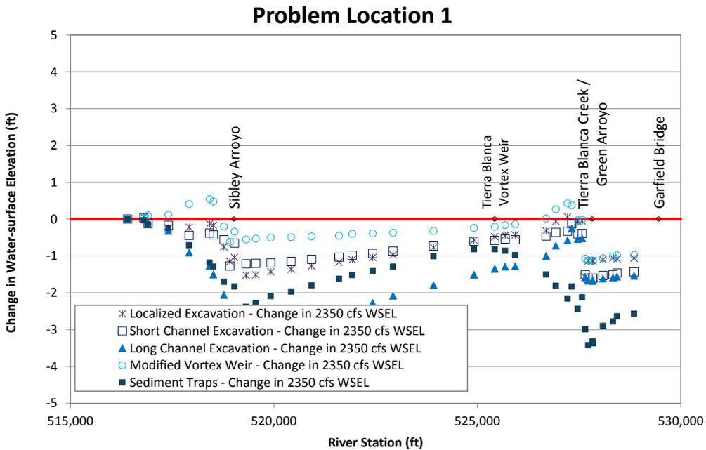
Figure N.2. Predicted change in long-term water-surface elevation at 2,350 cfs relative to the base condition at Problem Location 1 for the alternatives that were evaluated with the steady-state hydraulic model compared to existing (base model) conditions.
