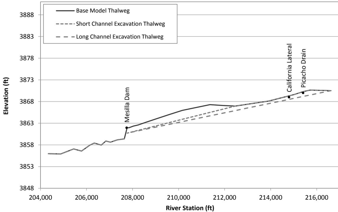
Figure G.1.25. Existing (Base Model) and excavation thalweg profiles at Problem Location 6.
