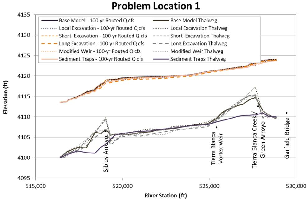
Figure N.3. Predicted water-surface profiles at the 100-year peak flow at Problem Location 1 representing long-term conditions based on hydraulic modeling with the predicted geometry at the end of the sediment-transport simulations of the base and alternative conditions.
