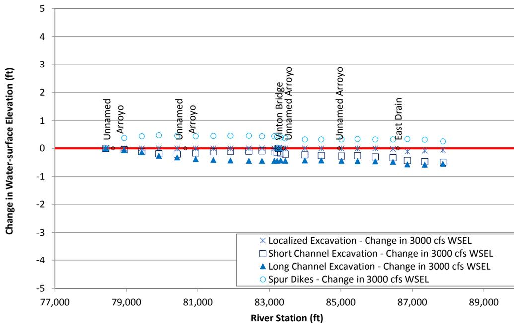
Figure L.52. Predicted change in water-surface elevation at 3,000 cfs at Problem Location 7 for the alternatives that were evaluated with the steady-state hydraulic model compared to existing (base model) conditions.
