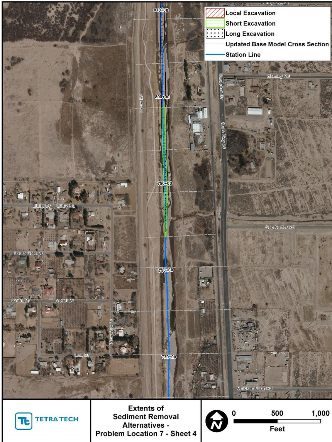
Figure G.2.27. Mapping showing extents of the localized, short and long sediment-removal alternatives at Problem Location 7 (Sheet 4).
