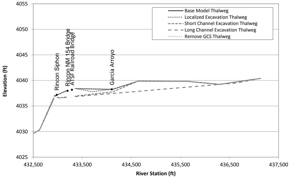
Figure G.1.11. Existing (Base Model) and excavation thalweg profiles at Problem Location 3.
