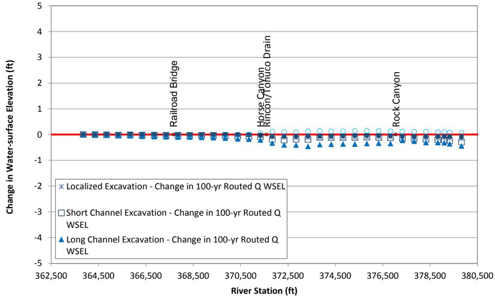
Figure N.20. Predicted change in long-term water-surface elevation at the 100-year peak flow relative to the base condition at Problem Location 5 for the alternatives that were evaluated with the steady-state hydraulic model compared to existing (base model) conditions.
