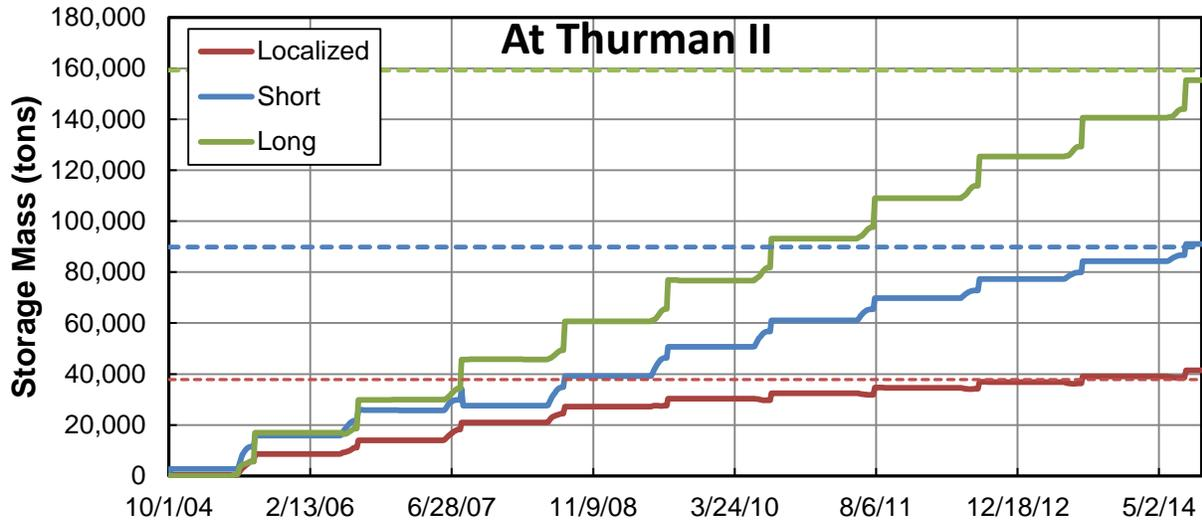
Figure M.2.21. Predicted cumulative mass of aggradation or degradation over time along the extents of the excavated reaches at Thurman II Arroyo (Problem Location 2) from the sediment-transport simulations of the sediment-removal alternatives. The dashed lines represent the excavated mass for each type of excavation.
