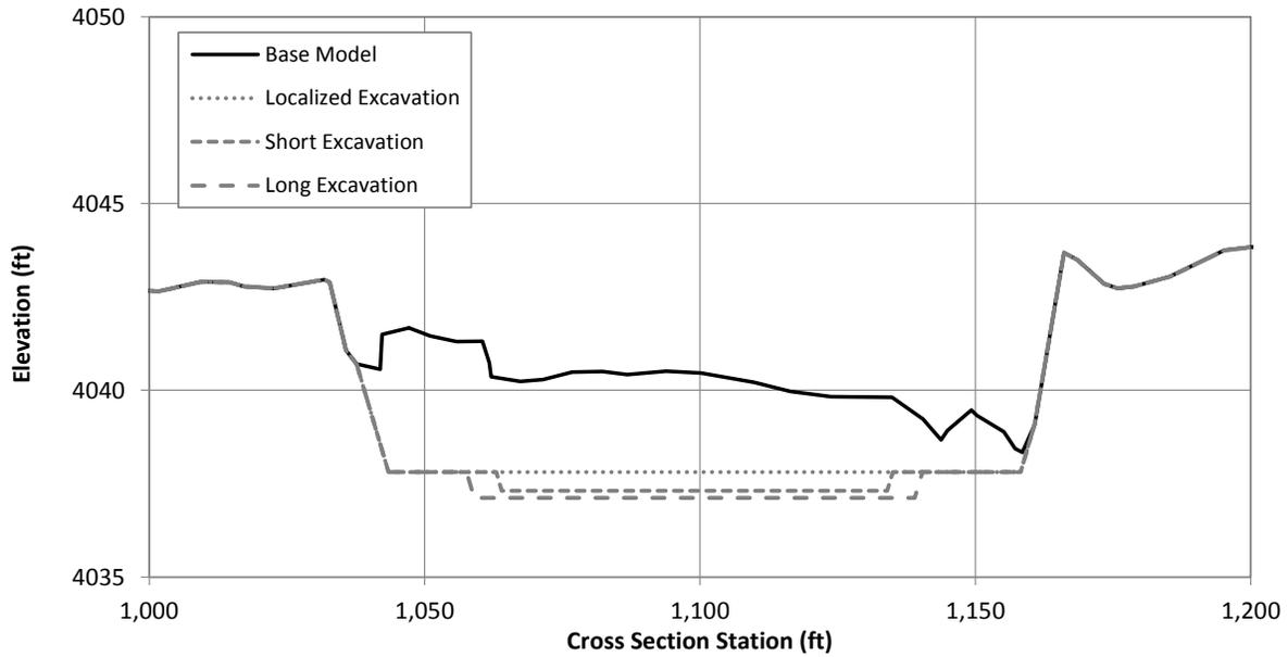
Figure G.1.13. Typical cross section at Problem Location 3 showing the existing (Base Model) channel geometry and excavated geometry under the localized, short and long excavation scenarios (River Station 433704.5).
