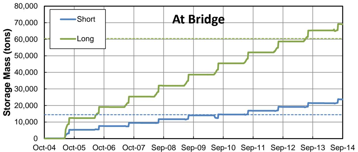
Figure M.2.32. Predicted cumulative mass of aggradation or degradation over time along the extents of the excavated reaches at Vinton Bridge (Problem Location 7) from the sediment-transport simulations of the sediment-removal alternatives. The dashed lines represent the excavated mass for each type of excavation.
