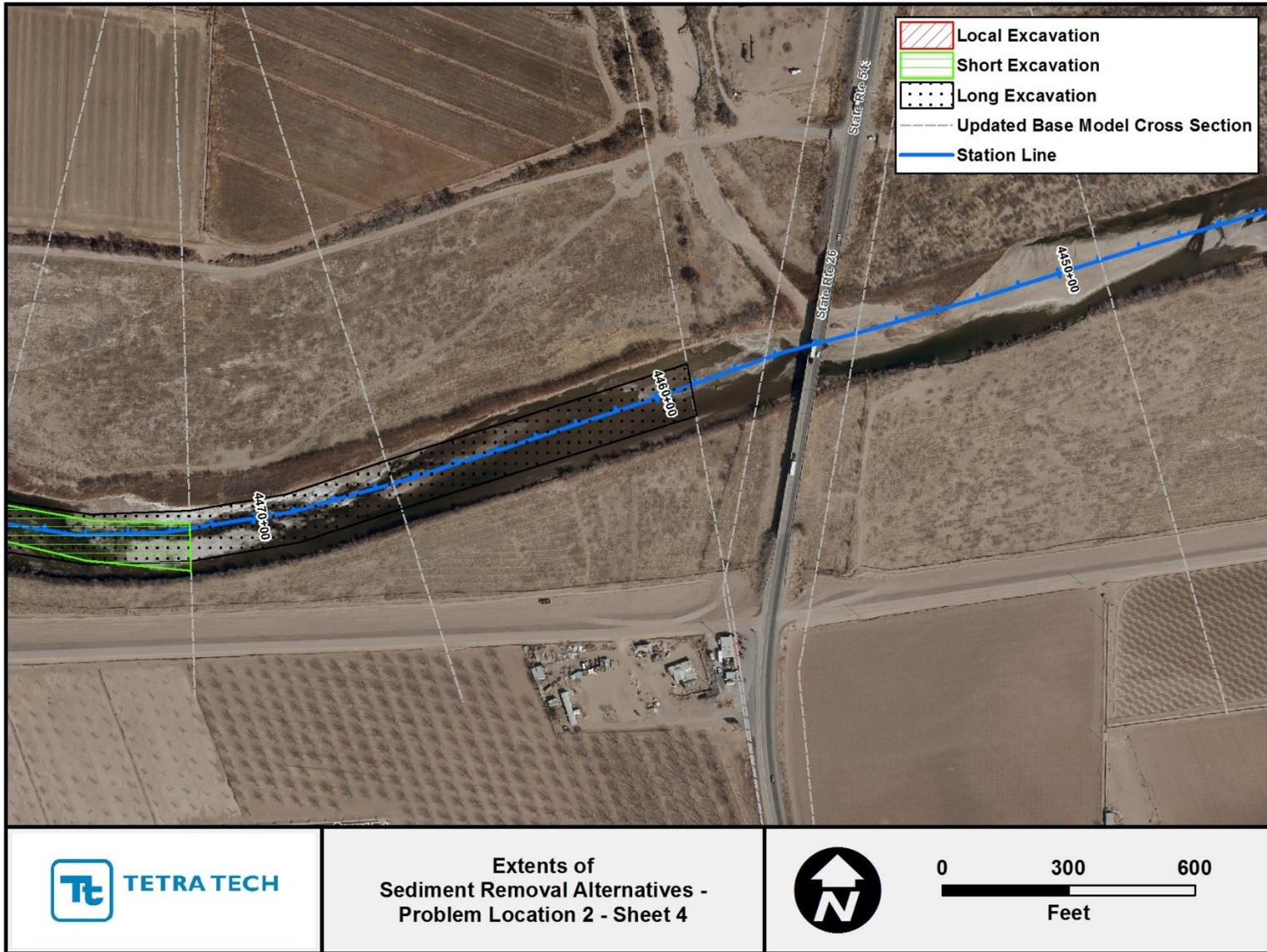
Figure G.2.6. Mapping showing extents of the localized, short and long sediment-removal alternatives at Problem Location 2 (Sheet 4).
