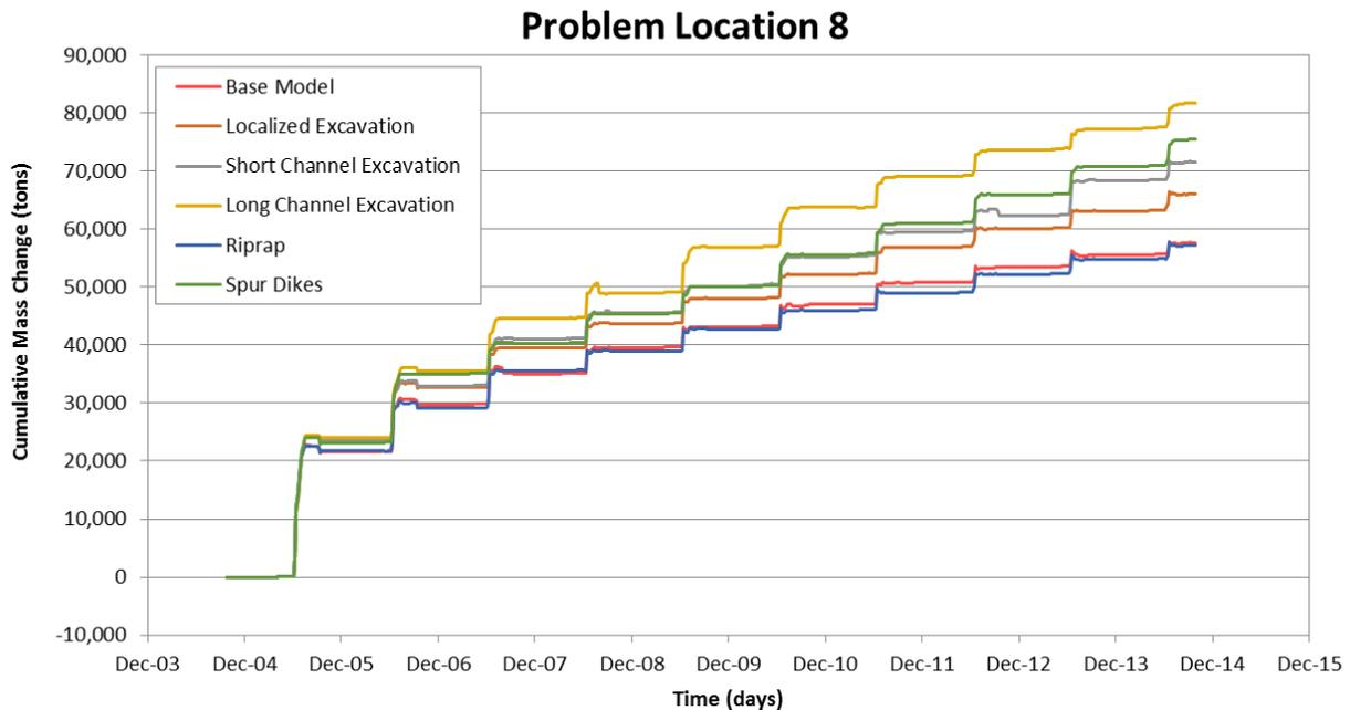
Figure M.2.8. Predicted cumulative mass of aggradation or degradation over time along the modeled reach at Problem Location 8 from the sediment-transport simulations of the base and alternative conditions.
