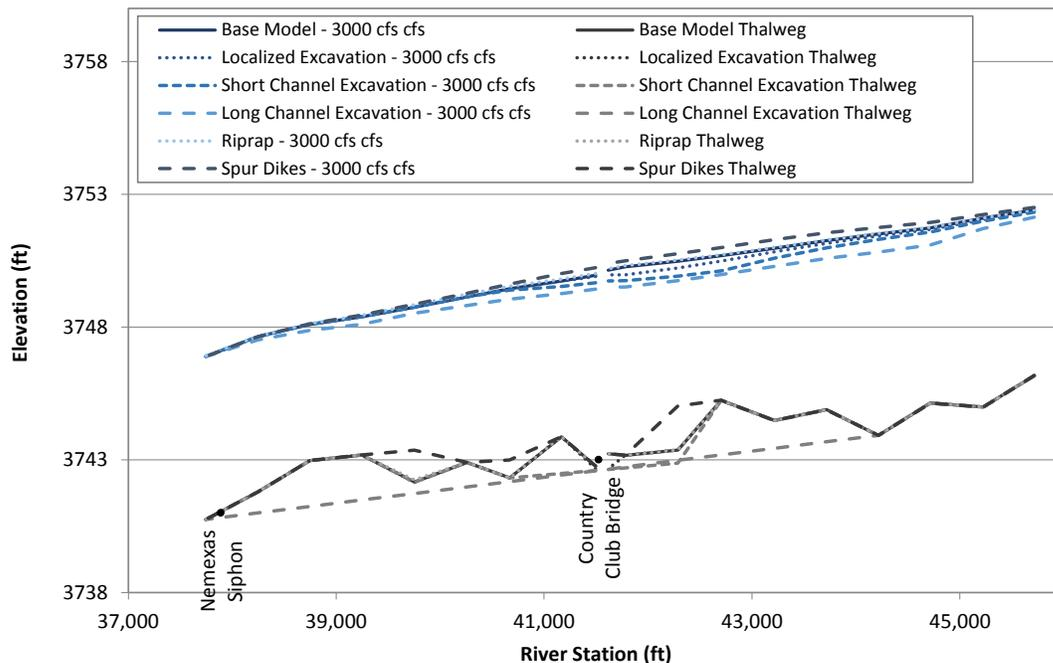
Figure L.59. Predicted water-surface profiles at 3,000 cfs at Problem Location 8 under existing (base model) conditions and for the alternatives that were evaluated with the steady-state hydraulic model.
