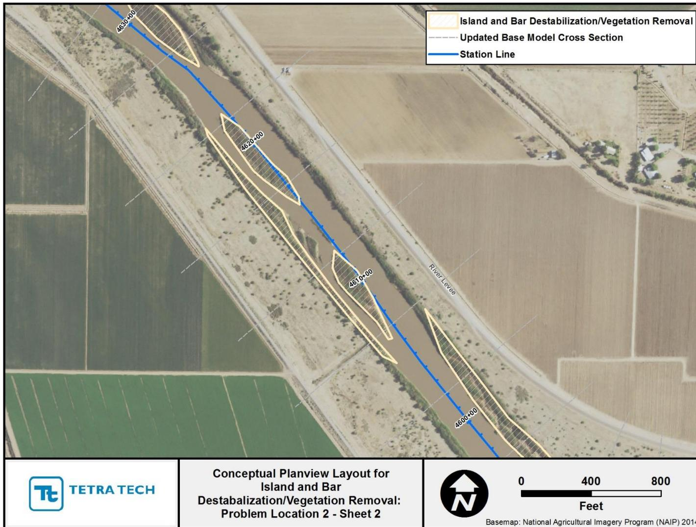
Figure J.2. Aerial photography showing extents of features treated with island/bar destabilization and vegetation removal at Problem Location 2 (Sheet 2).
