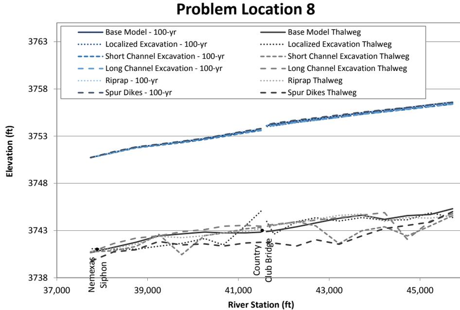
Figure N.31. Predicted water-surface profiles at the 100-year peak flow at Problem Location 8 representing long-term conditions based on hydraulic modeling with the predicted geometry at the end of the sediment-transport simulations of the base and alternative conditions.
