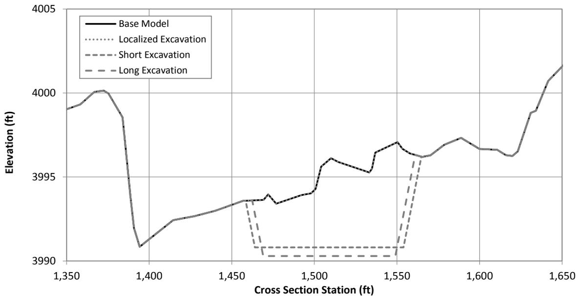
Figure G.1.22. Typical cross section at Problem Location 5 showing the existing (Base Model) channel geometry and excavated geometry under the localized, short and long excavation scenarios (River Station 376330).
