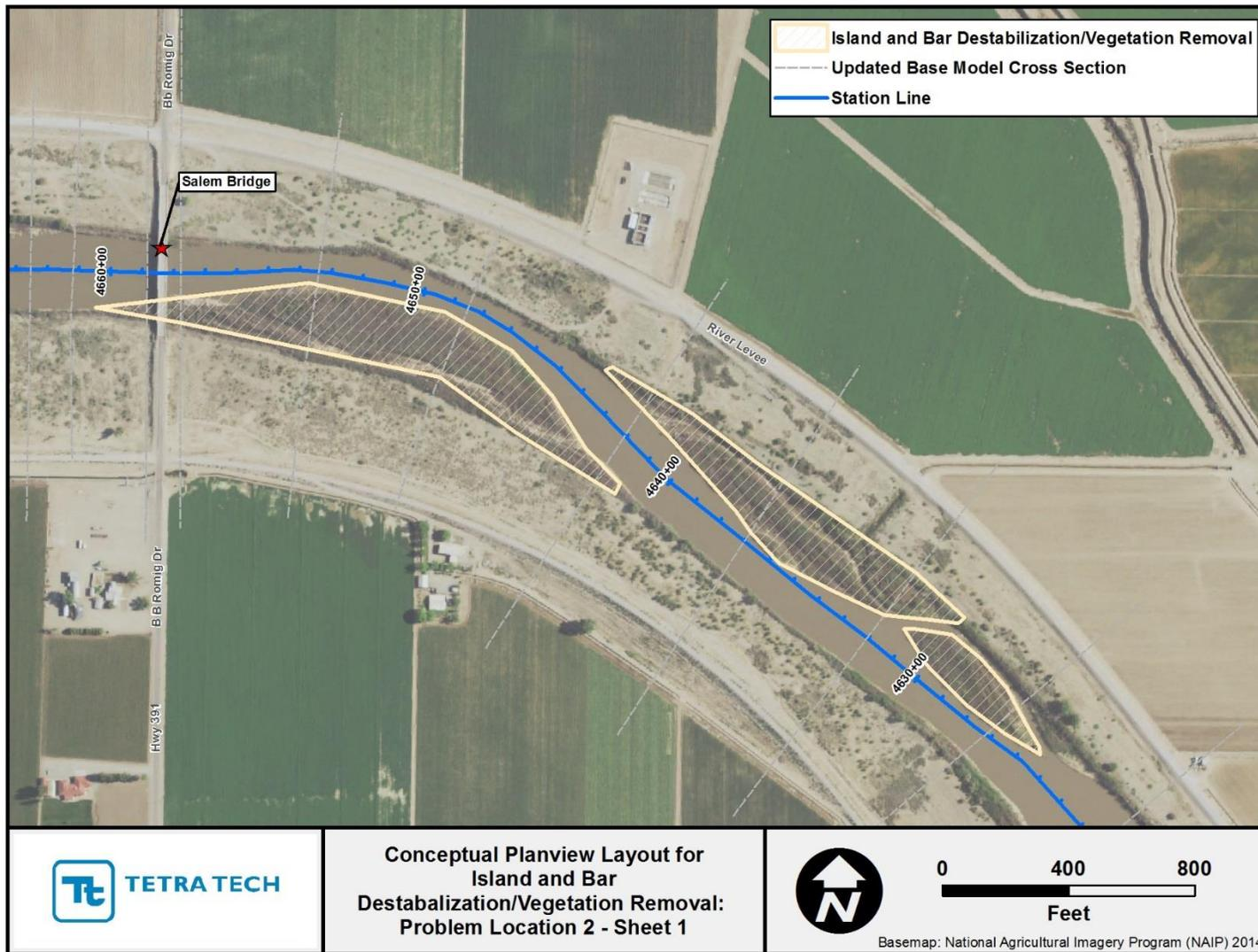
Figure J.1. Aerial photography showing extents of features treated with island/bar destabilization and vegetation removal at Problem Location 2 (Sheet 1).
