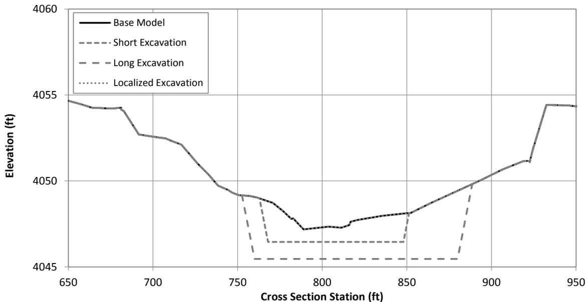
Figure G.1.10. Typical cross section at Problem Location 2 showing the existing (Base Model) channel geometry and excavated geometry under the localized, short and long excavation scenarios (River Station 447654.5).
