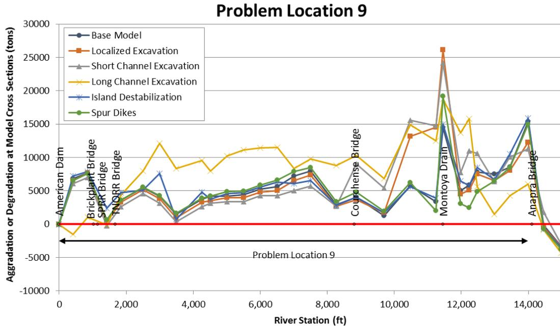
Figure M.1.9. Spatial profiles showing the predicted cumulative mass of aggradation or degradation at the end of the sediment-transport simulations for base alternative conditions at Problem Location 9.
