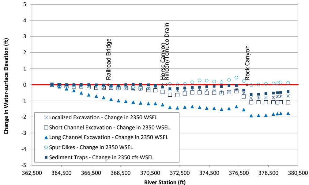
Figure N.18. Predicted change in long-term water-surface elevation at 2,350 cfs relative to the base condition at Problem Location 5 for the alternatives that were evaluated with the steady-state hydraulic model compared to existing (base model) conditions.
