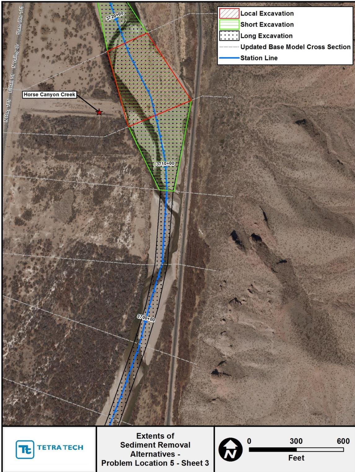
Figure G.2.17. Mapping showing extents of the localized, short and long sediment-removal alternatives at Problem Location 5 (Sheet 3).
