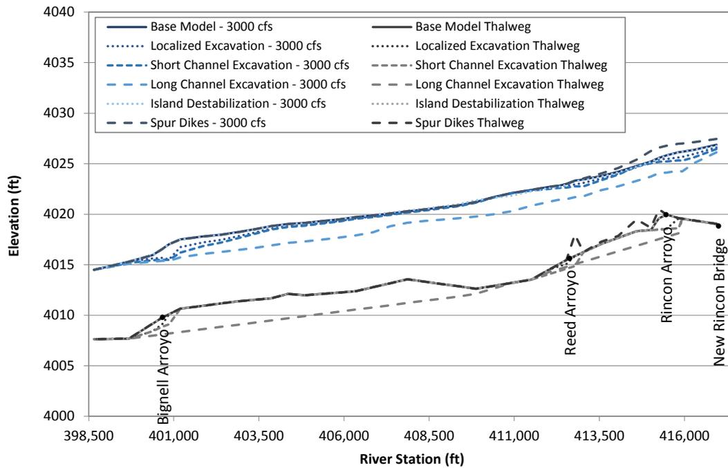
Figure L.27. Predicted water-surface profiles at 3,000 cfs at Problem Location 4 under existing (base model) conditions and for the alternatives that were evaluated with the steady-state hydraulic model.
