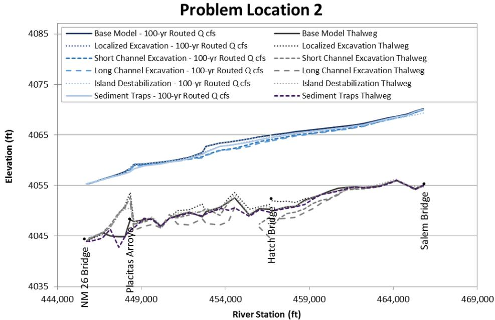
Figure N.7. Predicted water-surface profiles at the 100-year peak flow at Problem Location 2 representing long-term conditions based on hydraulic modeling with the predicted geometry at the end of the sediment-transport simulations of the base and alternative conditions.
