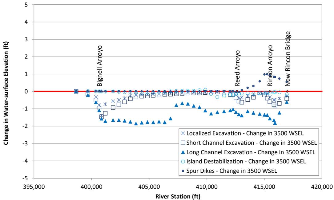
Figure L.30. Predicted change in water-surface elevation at 3,500 cfs at Problem Location 4 for the alternatives that were evaluated with the steady-state hydraulic model compared to existing (base model) conditions.
