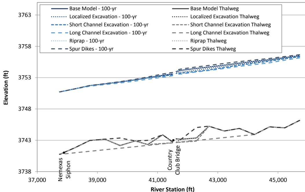
Figure L.63. Predicted water-surface profiles at the routed 100-year peak flow at Problem Location 8 under existing (base model) conditions and for the alternatives that were evaluated with the steady-state hydraulic model.
