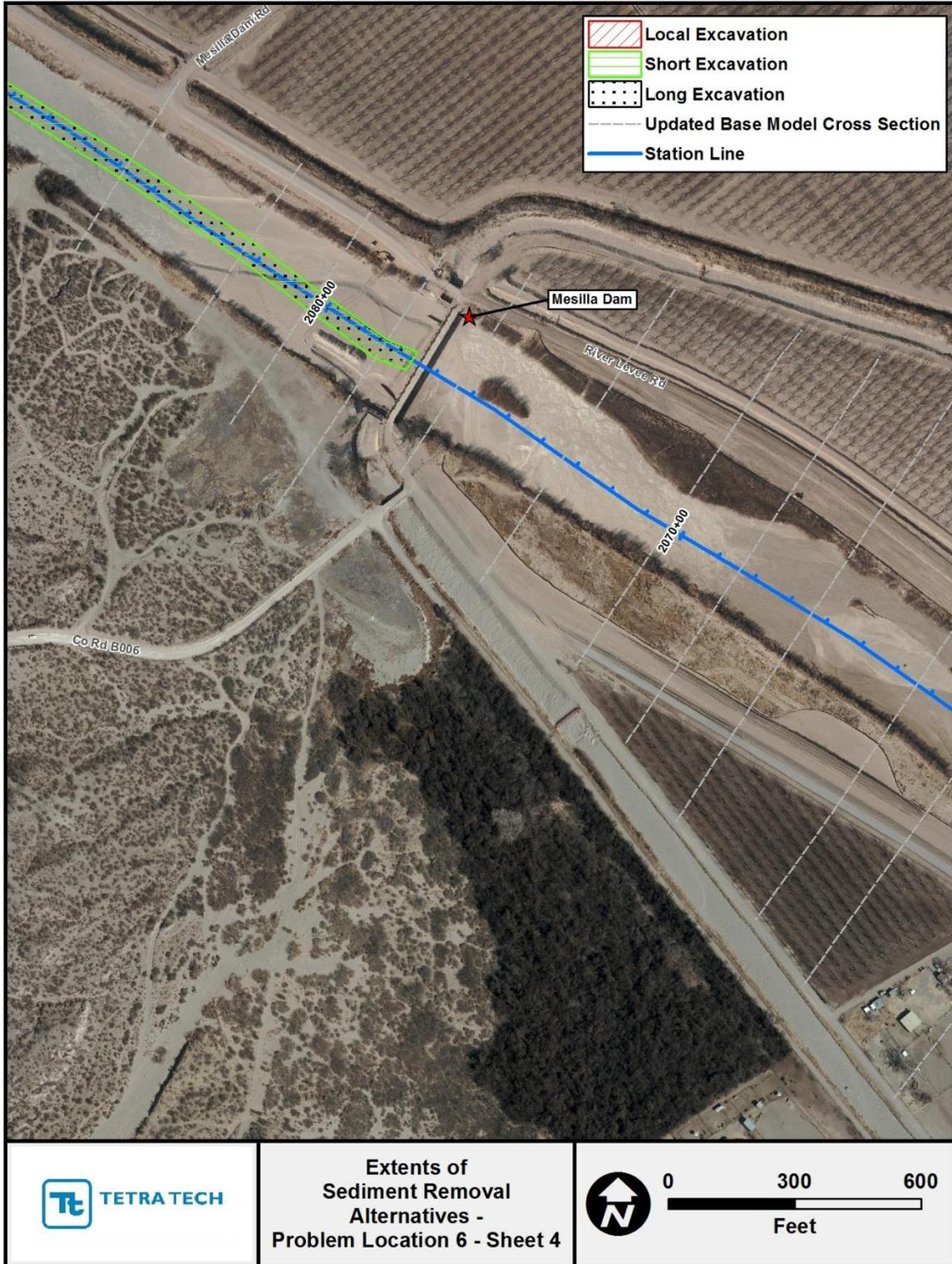
Figure G.2.23. Mapping showing extents of the localized, short and long sediment-removal alternatives at Problem Location 6 (Sheet 4).
