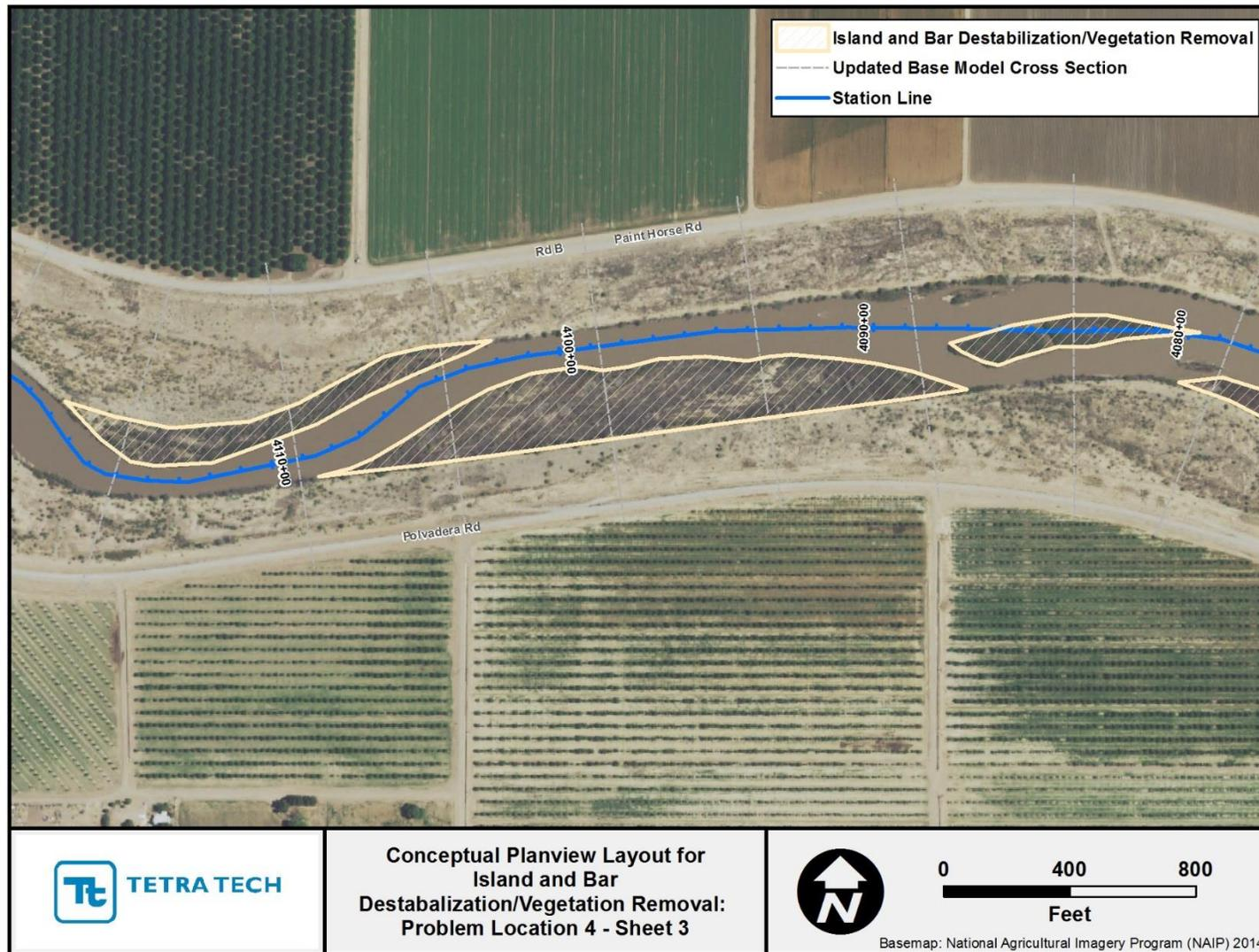
Figure J.8. Aerial photography showing extents of features treated with island/bar destabilization and vegetation removal at Problem Location 4 (Sheet 3).
