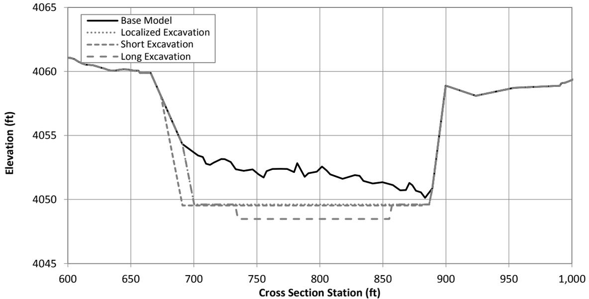
Figure G.1.8. Typical cross section at Problem Location 2 showing the existing (Base Model) channel geometry and excavated geometry under the localized, short and long excavation scenarios (River Station 452614.1).
