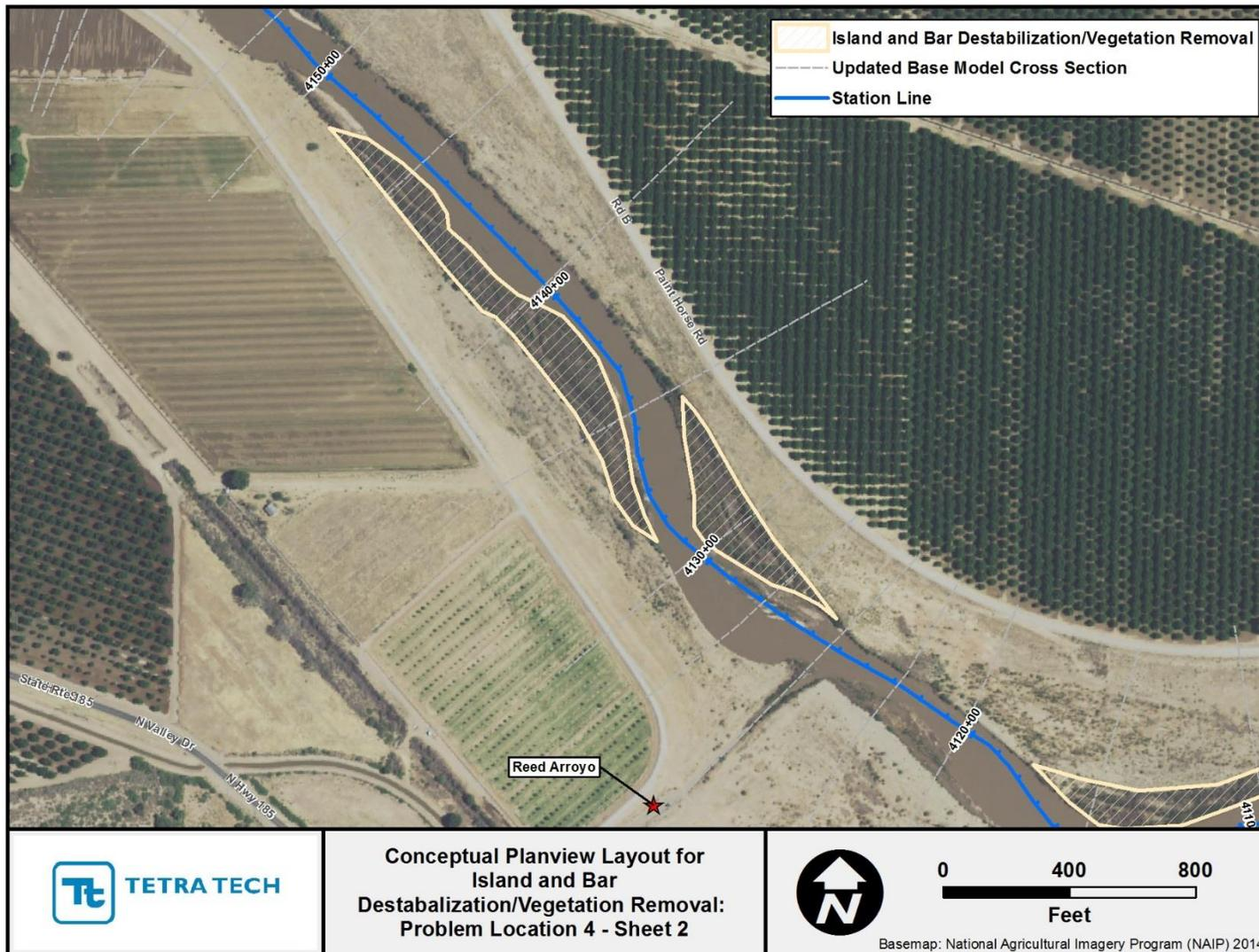
Figure J.7. Aerial photography showing extents of features treated with island/bar destabilization and vegetation removal at Problem Location 4 (Sheet 2).
