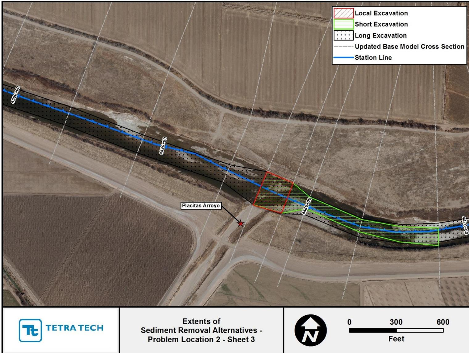
Figure G.2.5. Mapping showing extents of the localized, short and long sediment-removal alternatives at Problem Location 2 (Sheet 3).
