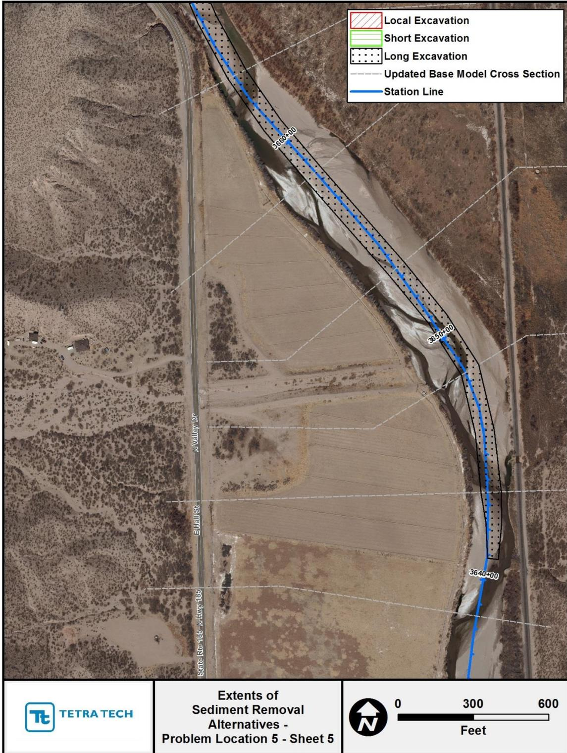
Figure G.2.19. Mapping showing extents of the localized, short and long sediment-removal alternatives at Problem Location 5 (Sheet 5).
