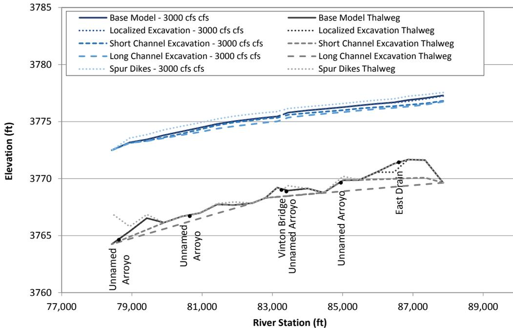
Figure L.51. Predicted water-surface profiles at 3,000 cfs at Problem Location 7 under existing (base model) conditions and for the alternatives that were evaluated with the steady-state hydraulic model.
