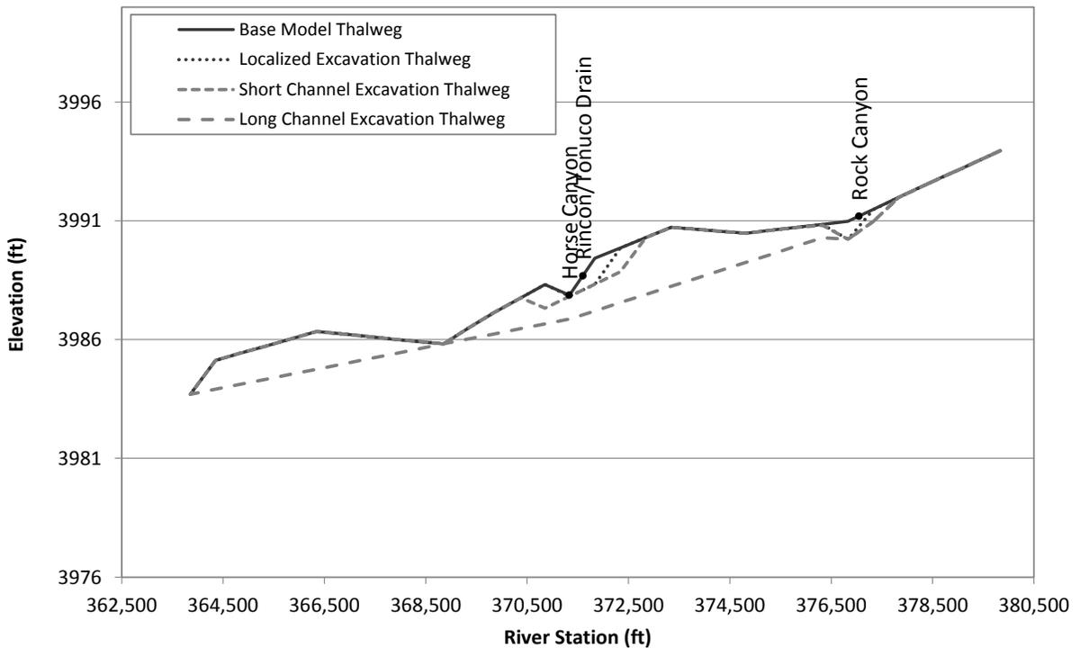
Figure G.1.20. Existing (Base Model) and excavation thalweg profiles at Problem Location 5.
