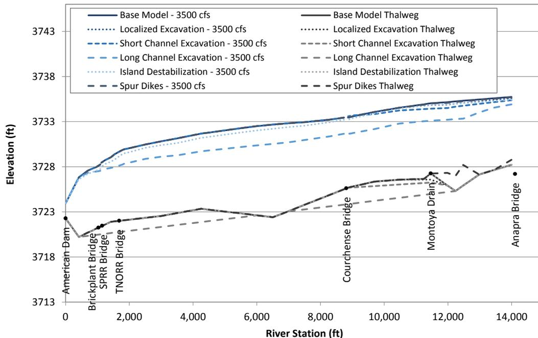
Figure L.69. Predicted water-surface profiles at 3,500 cfs at Problem Location 9 under existing (base model) conditions and for the alternatives that were evaluated with the steady-state hydraulic model.
