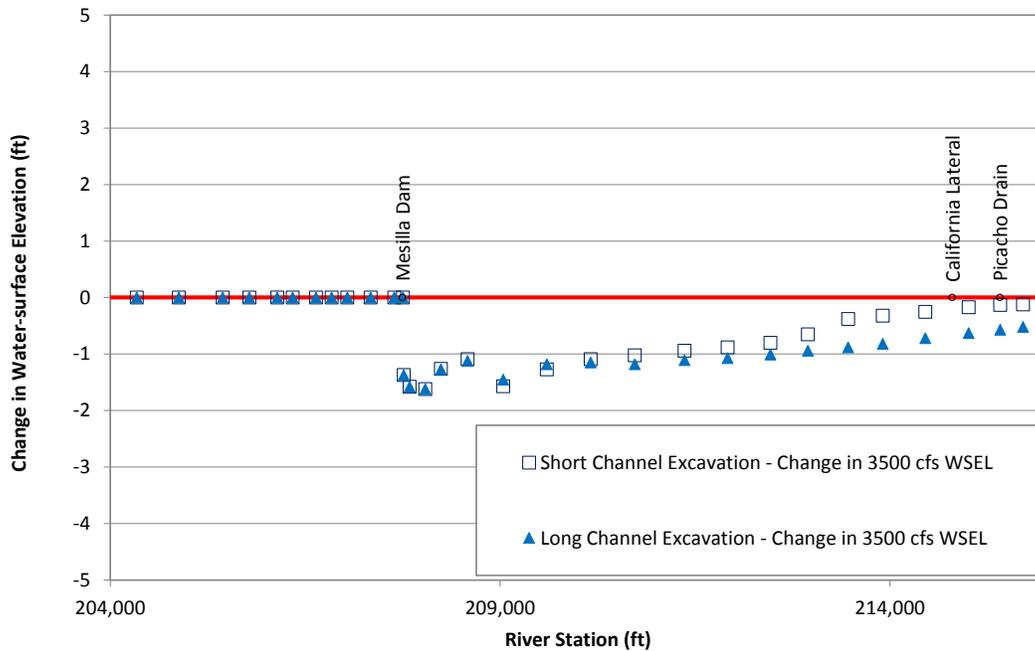
Figure L.46. Predicted change in water-surface elevation at 3,500 cfs at Problem Location 6 for the alternatives that were evaluated with the steady-state hydraulic model compared to existing (base model) conditions.
