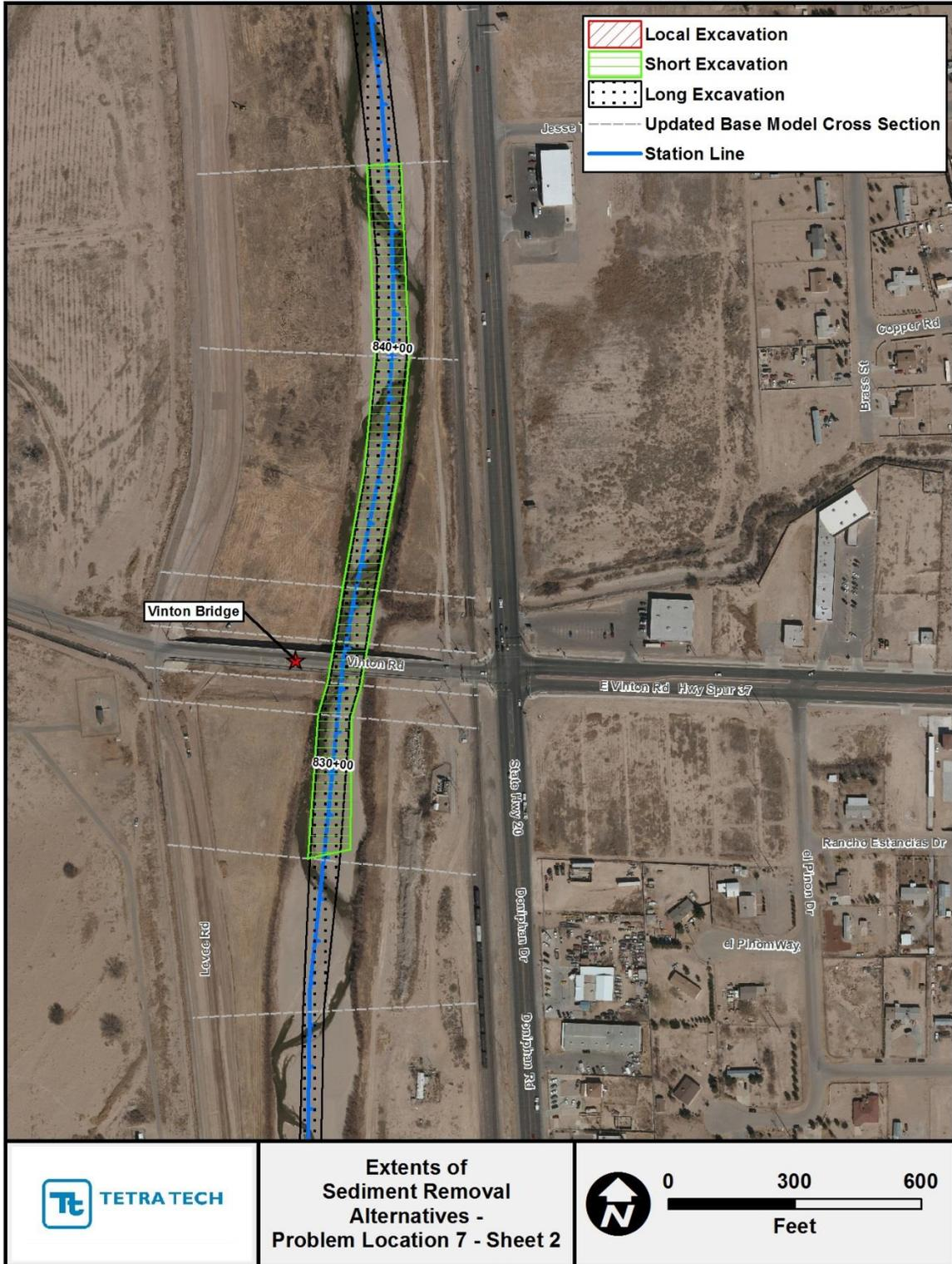
Figure G.2.25. Mapping showing extents of the localized, short and long sediment-removal alternatives at Problem Location 7 (Sheet 2).
