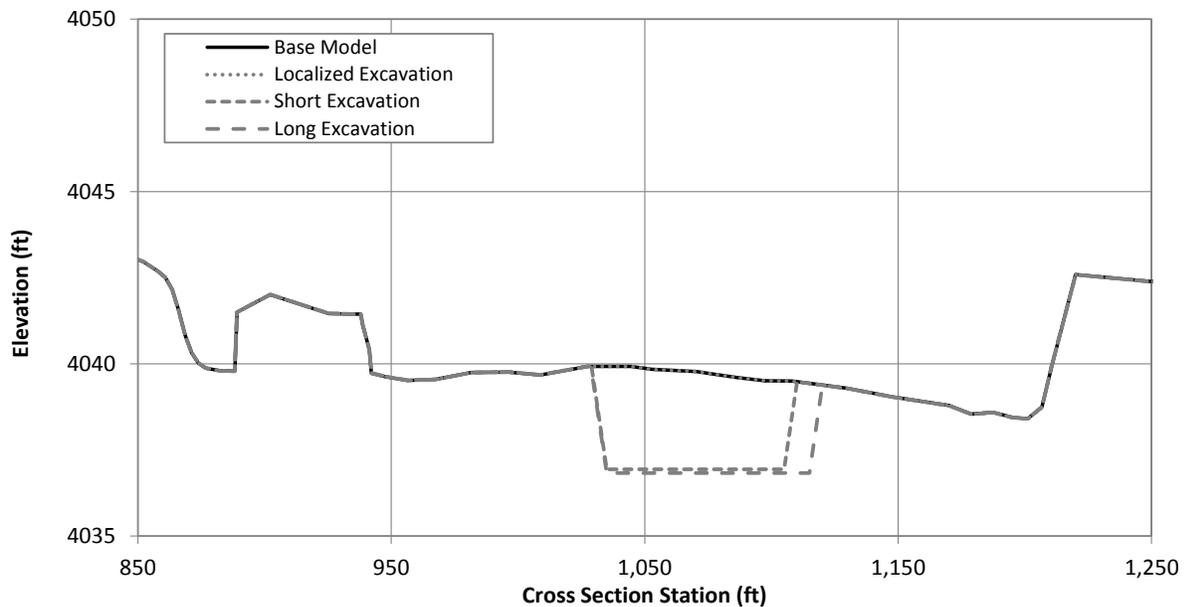
Figure G.1.14. Typical cross section at Problem Location 3 showing the existing (Base Model) channel geometry and excavated geometry under the localized, short and long excavation scenarios (River Station 433356.2).
