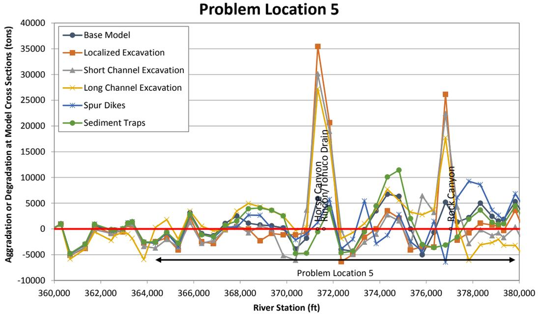
Figure M.1.5. Spatial profiles showing the predicted cumulative mass of aggradation or degradation at the end of the sediment-transport simulations for base alternative conditions at Problem Location 5.
