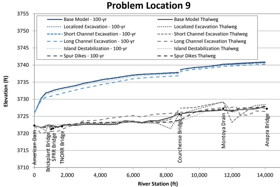
Figure N.35. Predicted water-surface profiles at the 100-year peak flow at Problem Location 9 representing long-term conditions based on hydraulic modeling with the predicted geometry at the end of the sediment-transport simulations of the base and alternative conditions.
