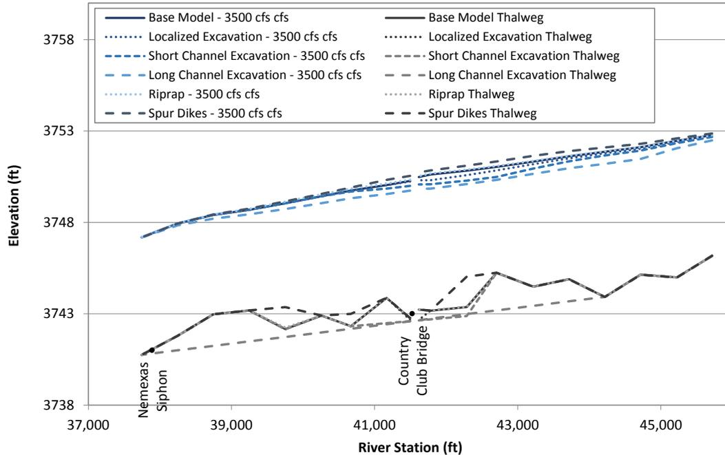
Figure L.61. Predicted water-surface profiles at 3,500 cfs at Problem Location 8 under existing (base model) conditions and for the alternatives that were evaluated with the steady-state hydraulic model.
