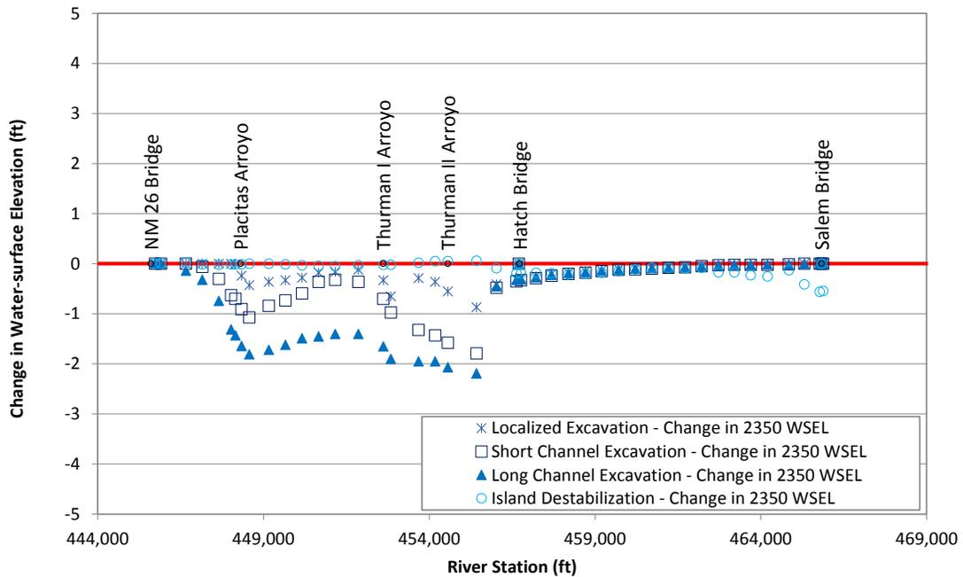
Figure L.10. Predicted change in water-surface elevation at 2,350 cfs at Problem Location 2 for the alternatives that were evaluated with the steady-state hydraulic model compared to existing (base model) conditions.
