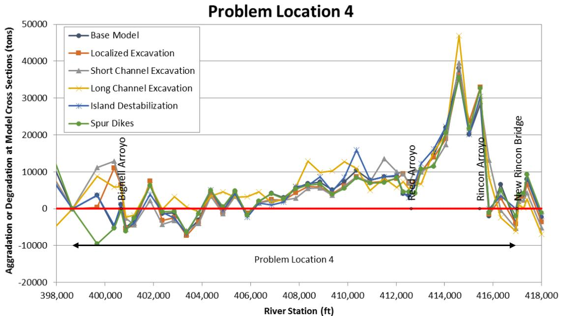
Figure M.1.4. Spatial profiles showing the predicted cumulative mass of aggradation or degradation at the end of the sediment-transport simulations for base alternative conditions at Problem Location 4.
