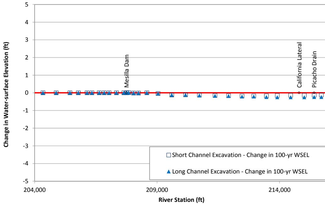
Figure L.48. Predicted change in water-surface elevation at the routed 100-year peak flow at Problem Location 6 for the alternatives that were evaluated with the steady-state hydraulic model compared to existing (base model) conditions.
