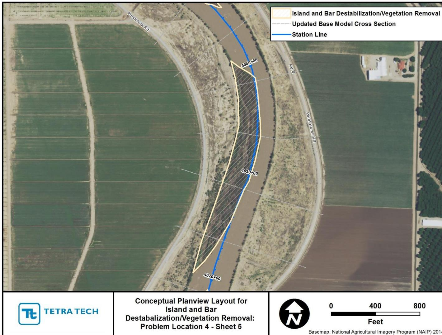
Figure J.10. Aerial photography showing extents of features treated with island/bar destabilization and vegetation removal at Problem Location 4 (Sheet 5).
