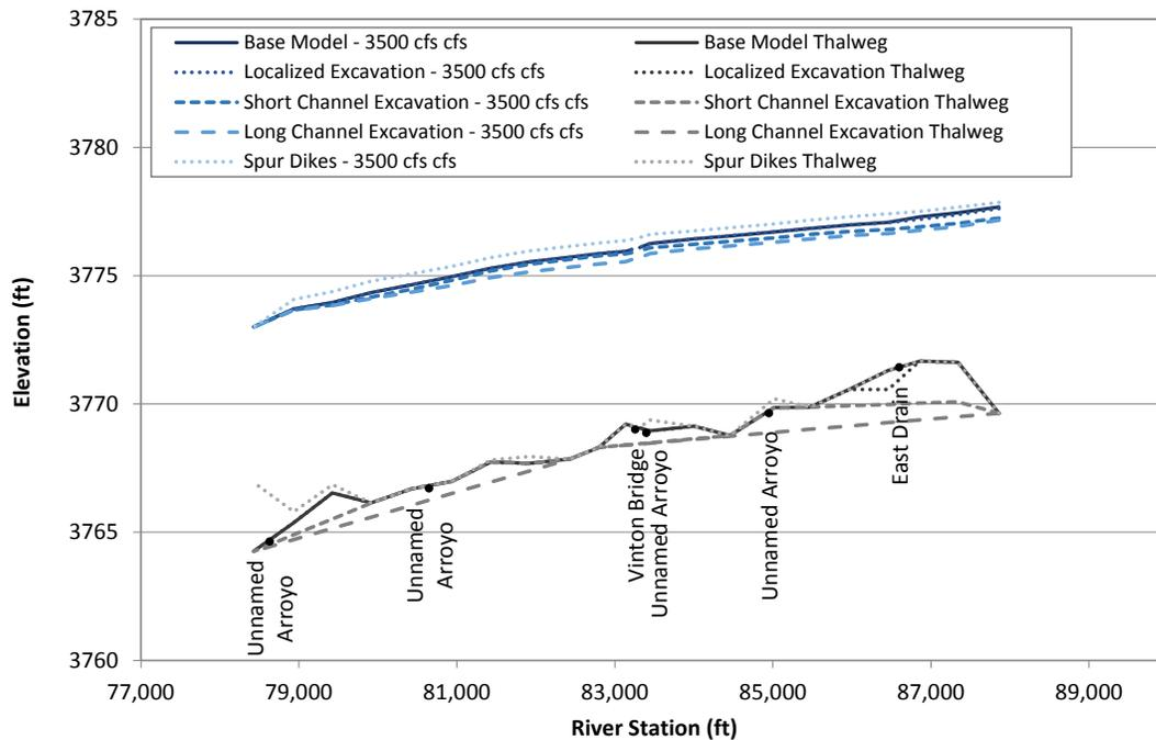
Figure L.53. Predicted water-surface profiles at 3,500 cfs at Problem Location 7 under existing (base model) conditions and for the alternatives that were evaluated with the steady-state hydraulic model.
