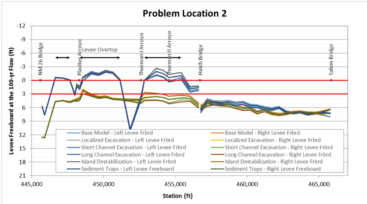
Figure O.1. Predicted levee freeboard during the 100-year flow at Problem Location 2 representing long-term conditions based on hydraulic modeling with the predicted geometry at the end of the sediment-transport simulations of the base and alternative conditions.
