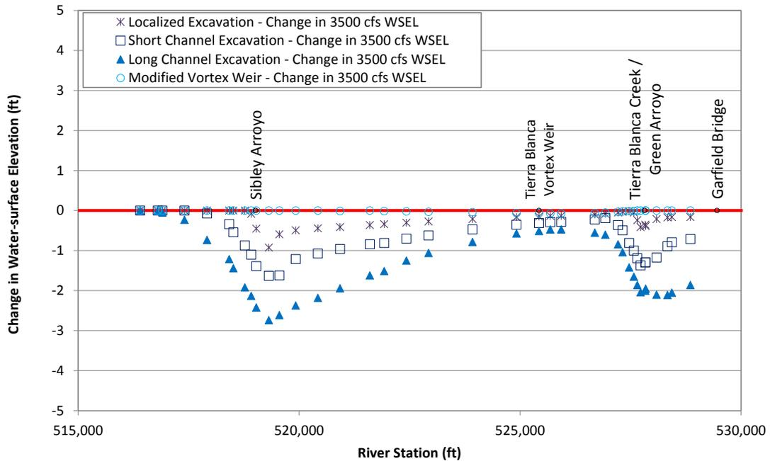
Figure L.6. Predicted change in water-surface elevation at 3,500 cfs at Problem Location 1 for the alternatives that were evaluated with the steady-state hydraulic model compared to existing (base model) conditions.
