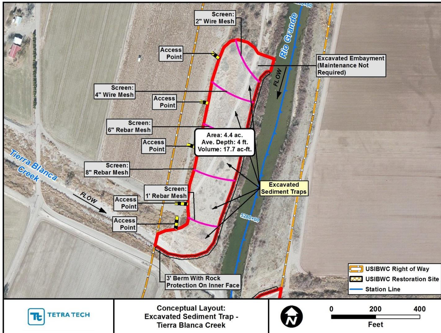
Figure H.1. Conceptual layout of sediment trap for Tierra Blanca Creek at Problem Location 1.
