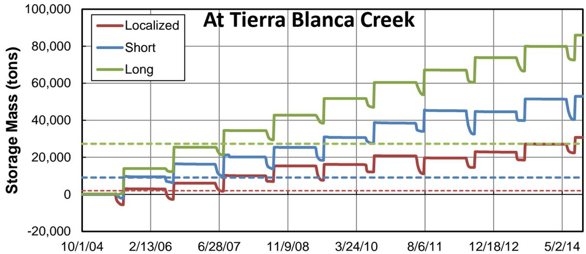
Figure M.2.19. Predicted cumulative mass of aggradation or degradation over time along the extents of the excavated reaches at Tierra Blanca Creek (Problem Location 1) from the sediment-transport simulations of the sediment-removal alternatives. The dashed lines represent the excavated mass for each type of excavation.
