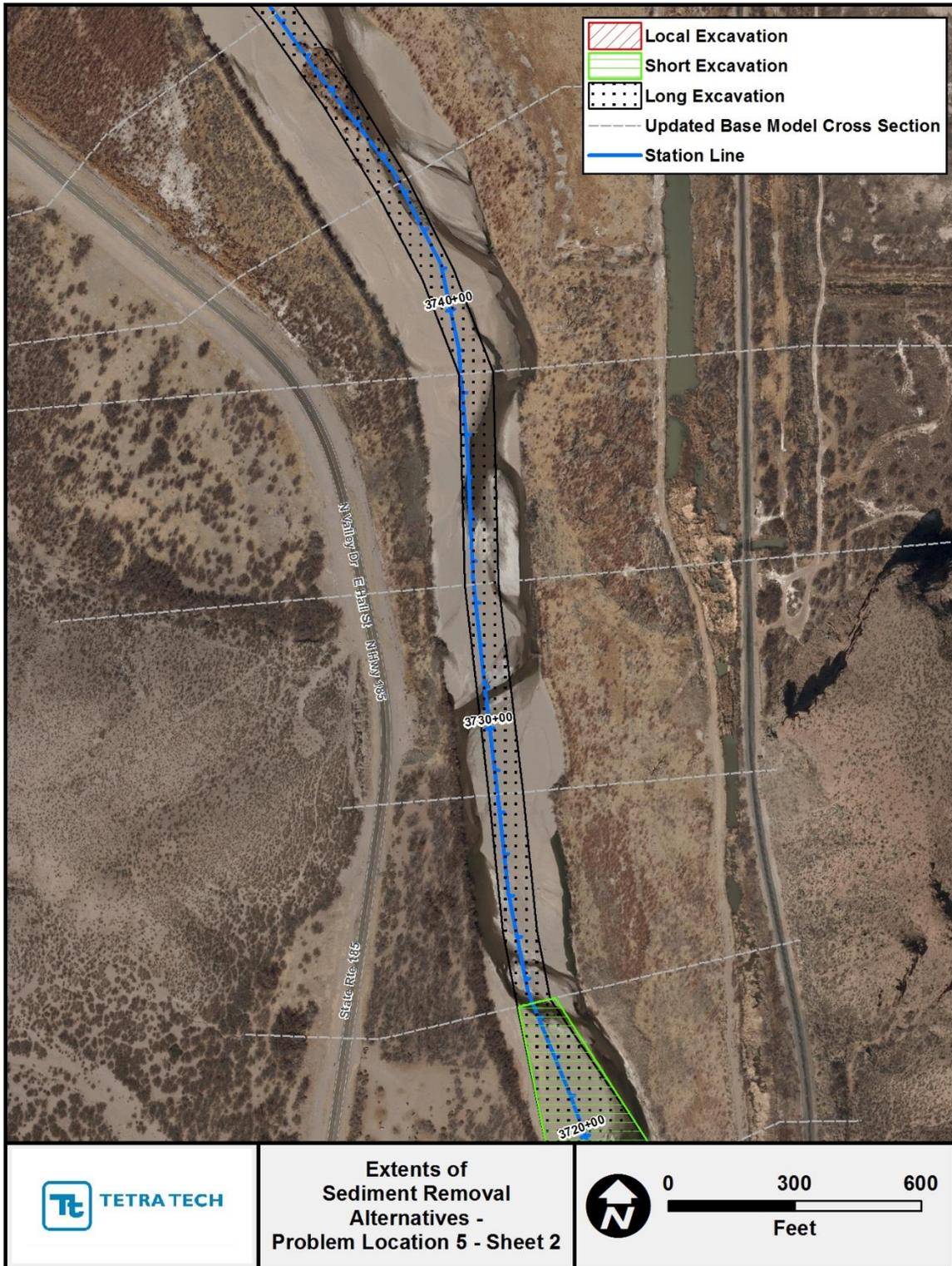
Figure G.2.16. Mapping showing extents of the localized, short and long sediment-removal alternatives at Problem Location 5 (Sheet 2).
