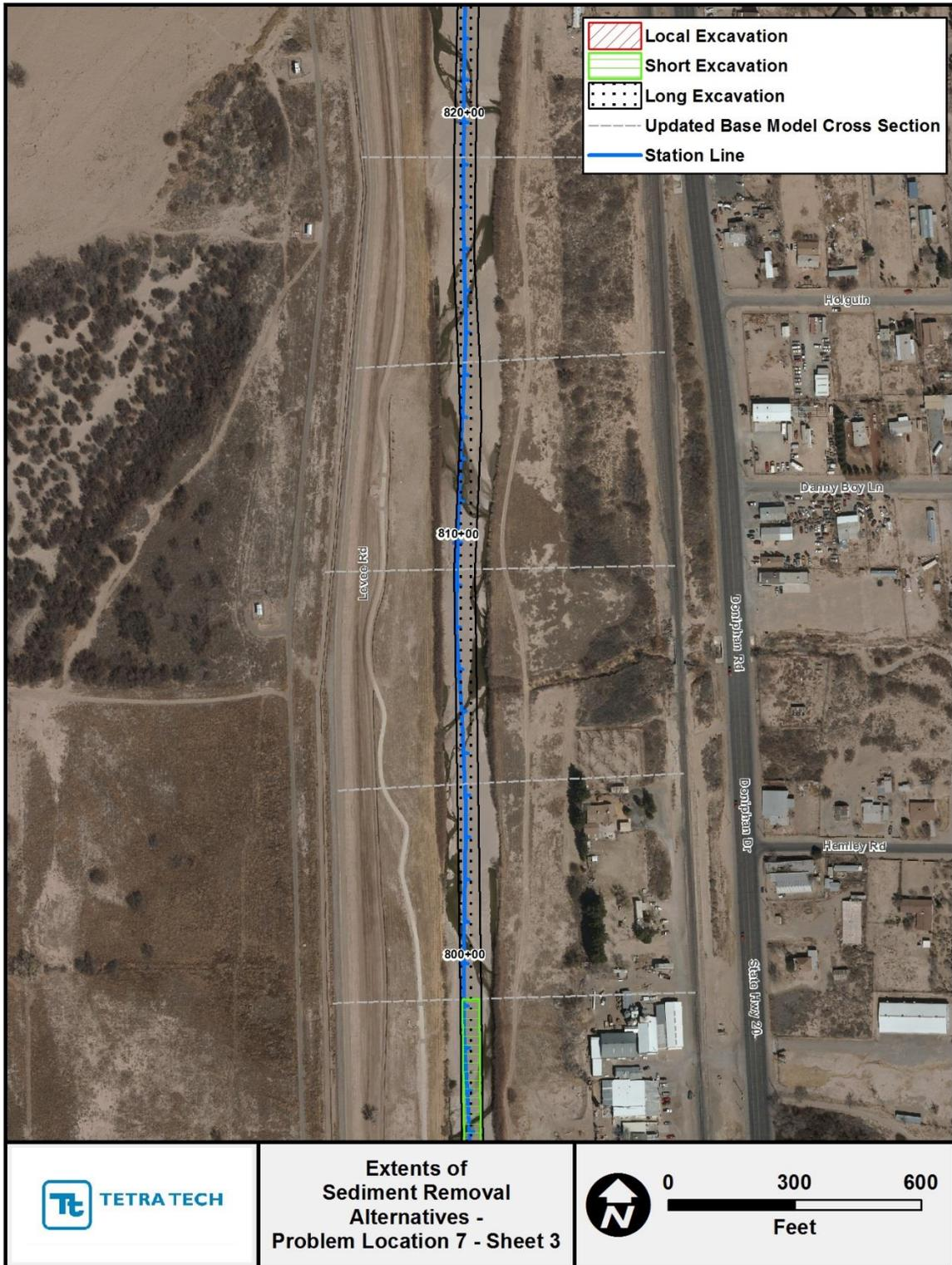
Figure G.2.26. Mapping showing extents of the localized, short and long sediment-removal alternatives at Problem Location 7 (Sheet 3).
