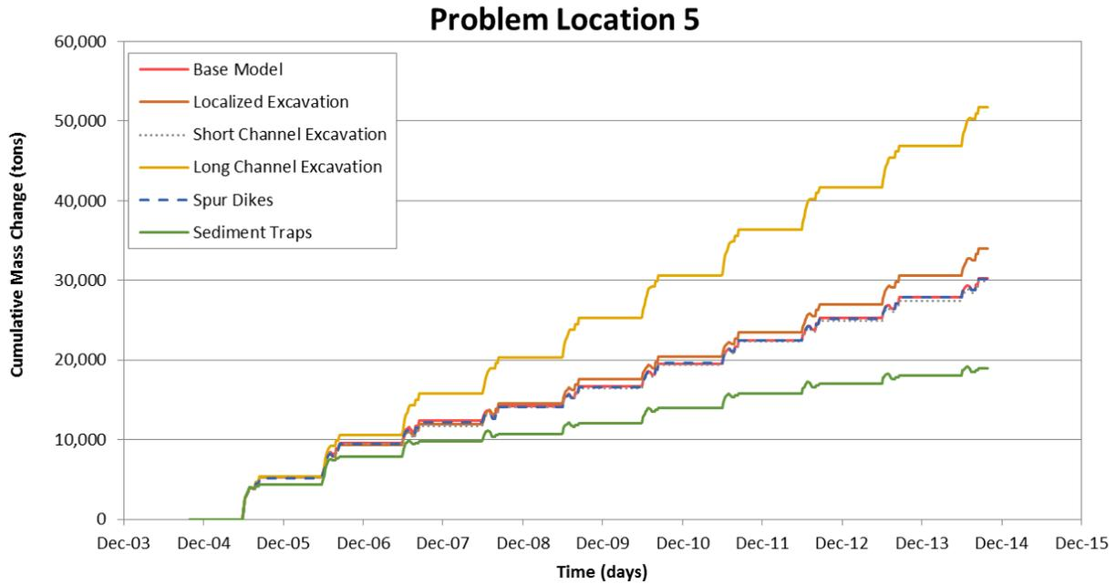
Figure M.2.5. Predicted cumulative mass of aggradation or degradation over time along the modeled reach at Problem Location 5 from the sediment-transport simulations of the base and alternative conditions.
