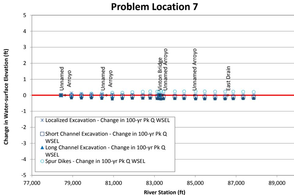
Figure N.28. Predicted change in long-term water-surface elevation at the 100-year peak flow relative to the base condition at Problem Location 7 for the alternatives that were evaluated with the steady-state hydraulic model compared to existing (base model) conditions.
