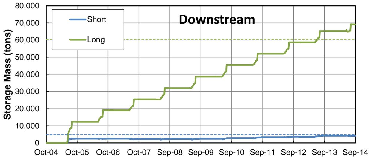
Figure M.2.33. Predicted cumulative mass of aggradation or degradation over time along the extents of the excavated reaches at the Subarea 103 (U/S) Arroyo (Problem Location 7) from the sediment-transport simulations of the sediment-removal alternatives. The dashed lines represent the excavated mass for each type of excavation.
