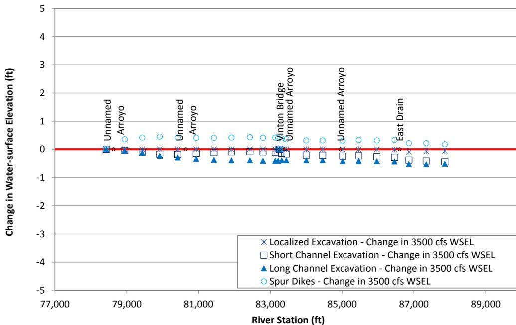
Figure L.54. Predicted change in water-surface elevation at 3,500 cfs at Problem Location 7 for the alternatives that were evaluated with the steady-state hydraulic model compared to existing (base model) conditions.
