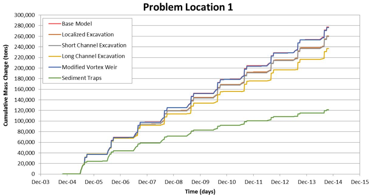
Figure M.2.1. Predicted cumulative mass of aggradation or degradation over time along the modeled reach at Problem Location 1 from the sediment-transport simulations of the base and alternative conditions.
