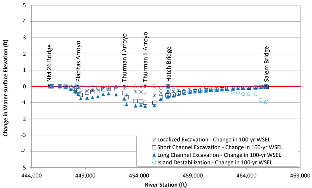
Figure L.16. Predicted change in water-surface elevation at the routed 100-year peak flow at Problem Location 2 for the alternatives that were evaluated with the steady-state hydraulic model compared to existing (base model) conditions.
