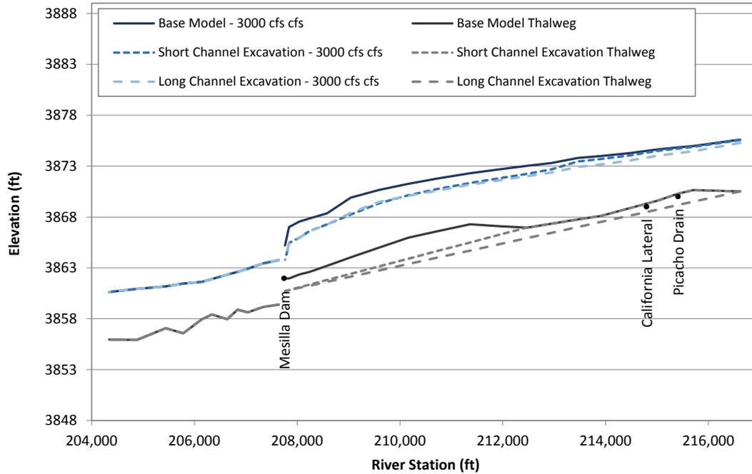
Figure L.43. Predicted water-surface profiles at 3,000 cfs at Problem Location 6 under existing (base model) conditions and for the alternatives that were evaluated with the steady-state hydraulic model.
