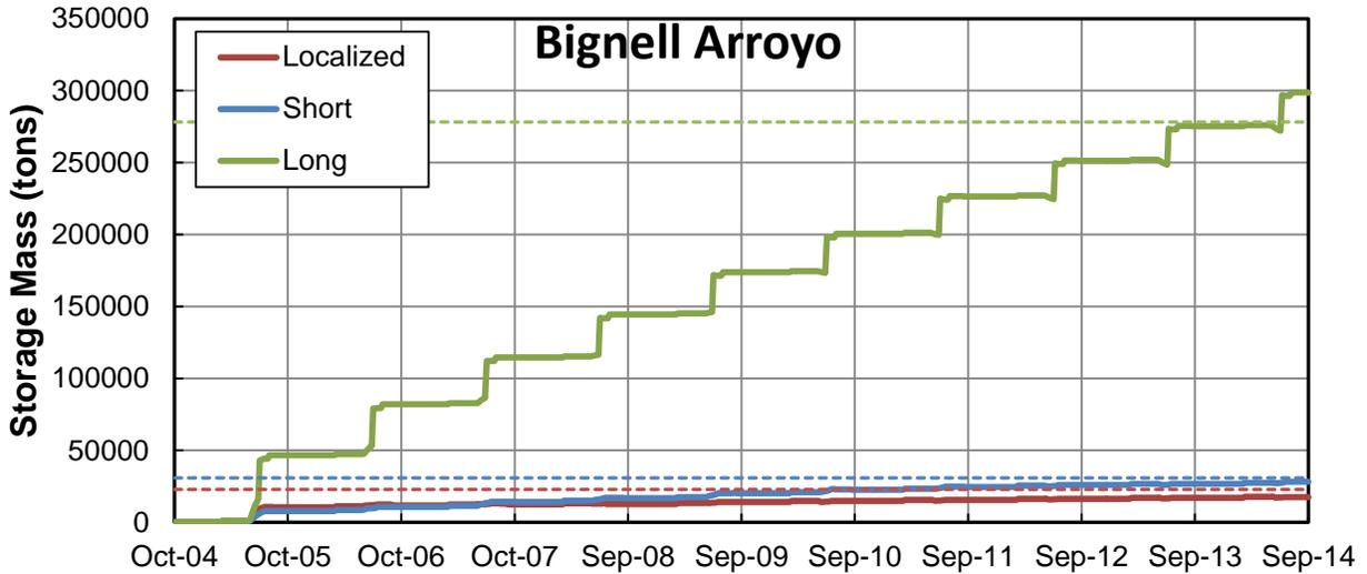
Figure M.2.27. Predicted cumulative mass of aggradation or degradation over time along the extents of the excavated reaches at Bignell Arroyo (Problem Location 4) from the sediment-transport simulations of the sediment-removal alternatives. The dashed lines represent the excavated mass for each type of excavation.
