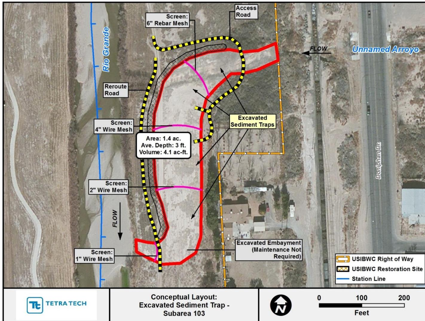
Figure H.12. Conceptual layout of sediment trap for the unnamed arroyo draining Subarea 103 at Problem Location 7.
