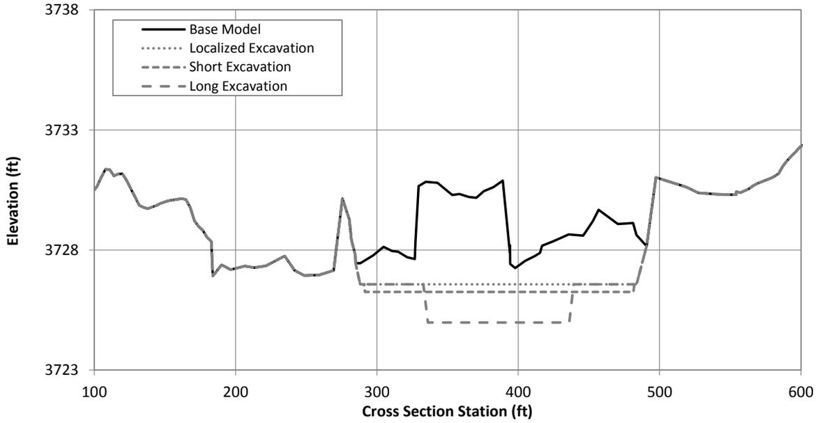
Figure G.1.38. Typical cross section at Problem Location 9 showing the existing (Base Model) channel geometry and excavated geometry under the localized, short and long excavation scenarios (River Station 11460.1).
