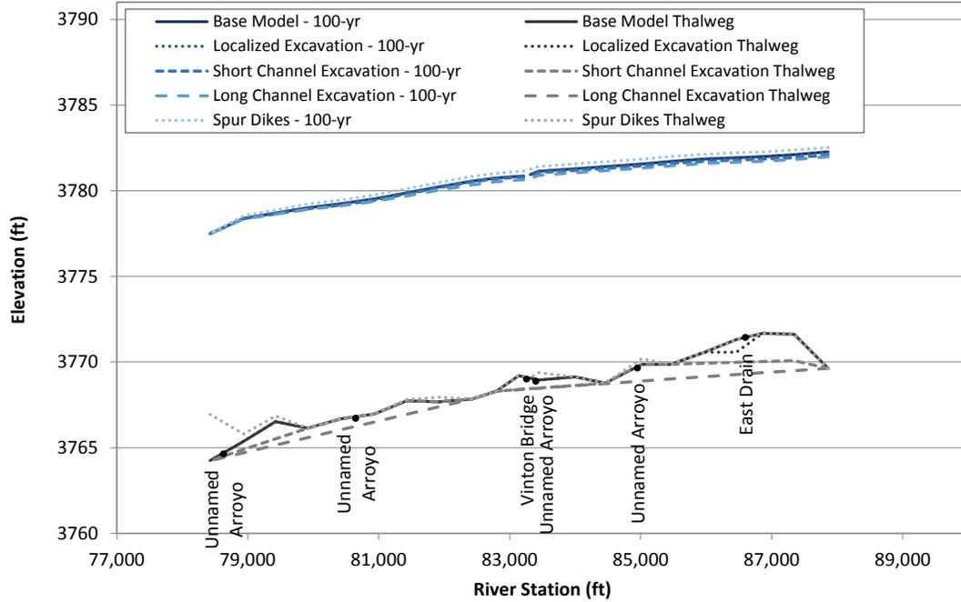
Figure L.55. Predicted water-surface profiles at the routed 100-year peak flow at Problem Location 7 under existing (base model) conditions and for the alternatives that were evaluated with the steady-state hydraulic model.
