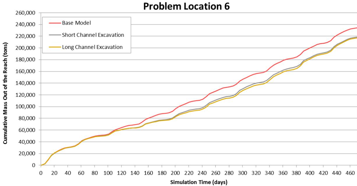
Figure M.2.15. Predicted cumulative mass delivered from the downstream of the model reach at Problem Location 6 from the sediment-transport simulations of the base and alternative conditions.
