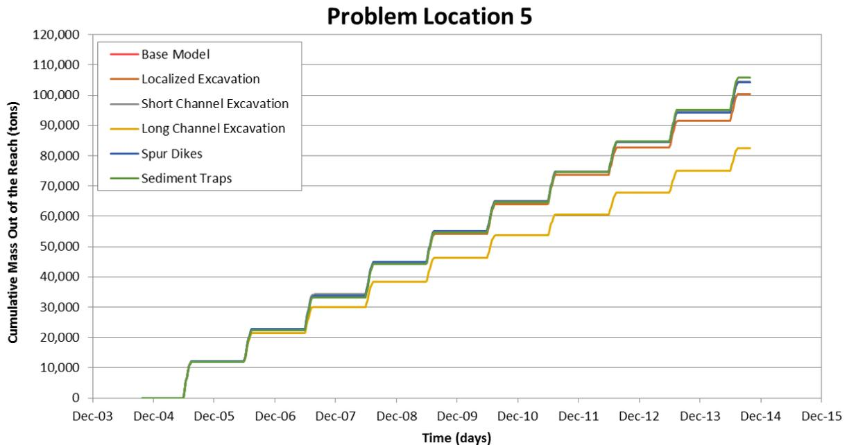
Figure M.2.14. Predicted cumulative mass delivered from the downstream of the model reach at Problem Location 5 from the sediment-transport simulations of the base and alternative conditions.
