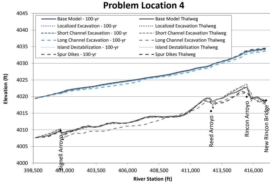
Figure N.15. Predicted water-surface profiles at the 100-year peak flow at Problem Location 4 representing long-term conditions based on hydraulic modeling with the predicted geometry at the end of the sediment-transport simulations of the base and alternative conditions.
