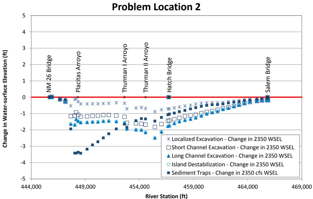
Figure N.6. Predicted change in long-term water-surface elevation at 2,350 cfs relative to the base condition at Problem Location 2 for the alternatives that were evaluated with the steady-state hydraulic model compared to existing (base model) conditions.
