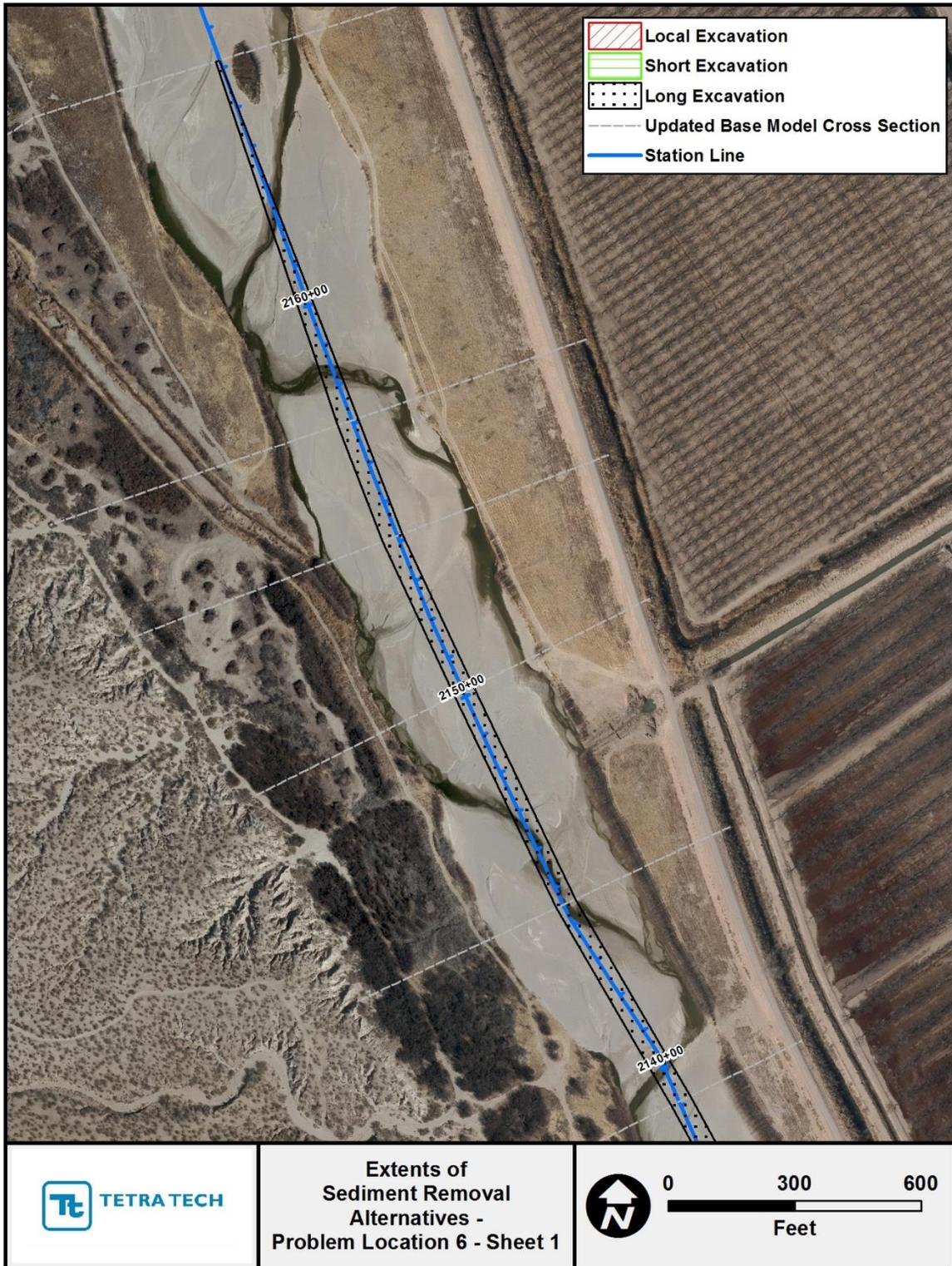
Figure G.2.20. Mapping showing extents of the localized, short and long sediment-removal alternatives at Problem Location 6 (Sheet 1).
