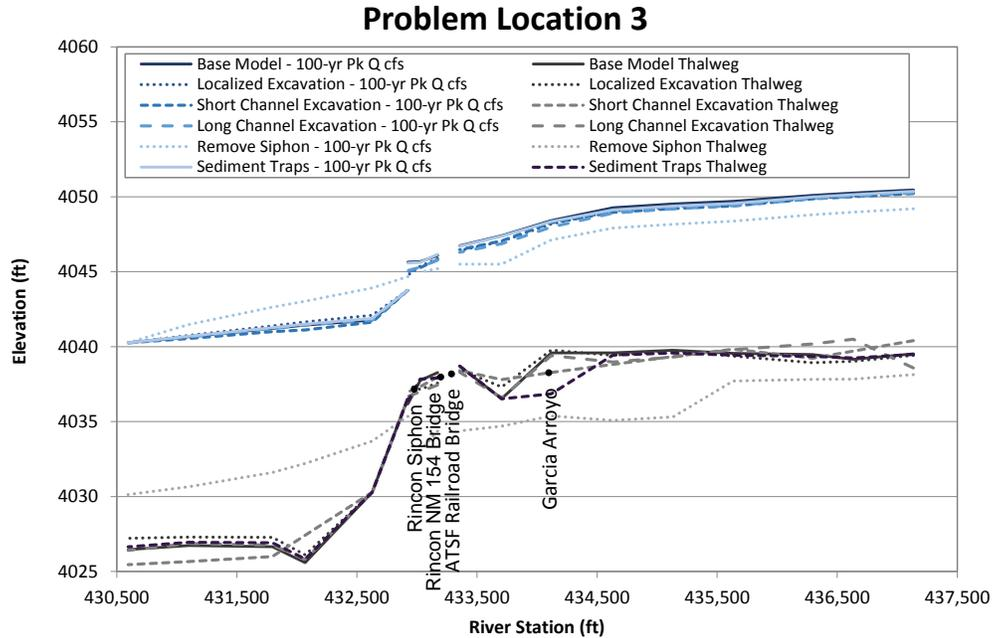
Figure N.11. Predicted water-surface profiles at the 100-year peak flow at Problem Location 3 representing long-term conditions based on hydraulic modeling with the predicted geometry at the end of the sediment-transport simulations of the base and alternative conditions.
