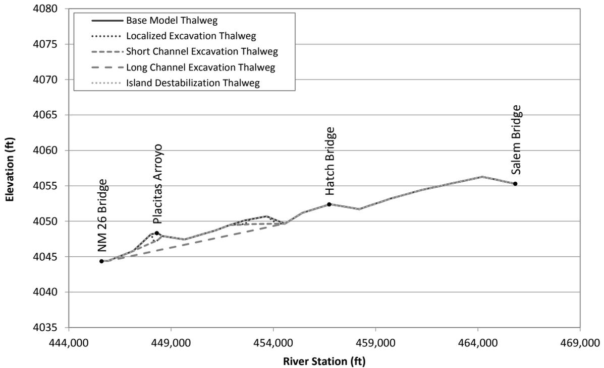
Figure G.1.6. Existing (Base Model) and excavation thalweg profiles at Problem Location 2.
