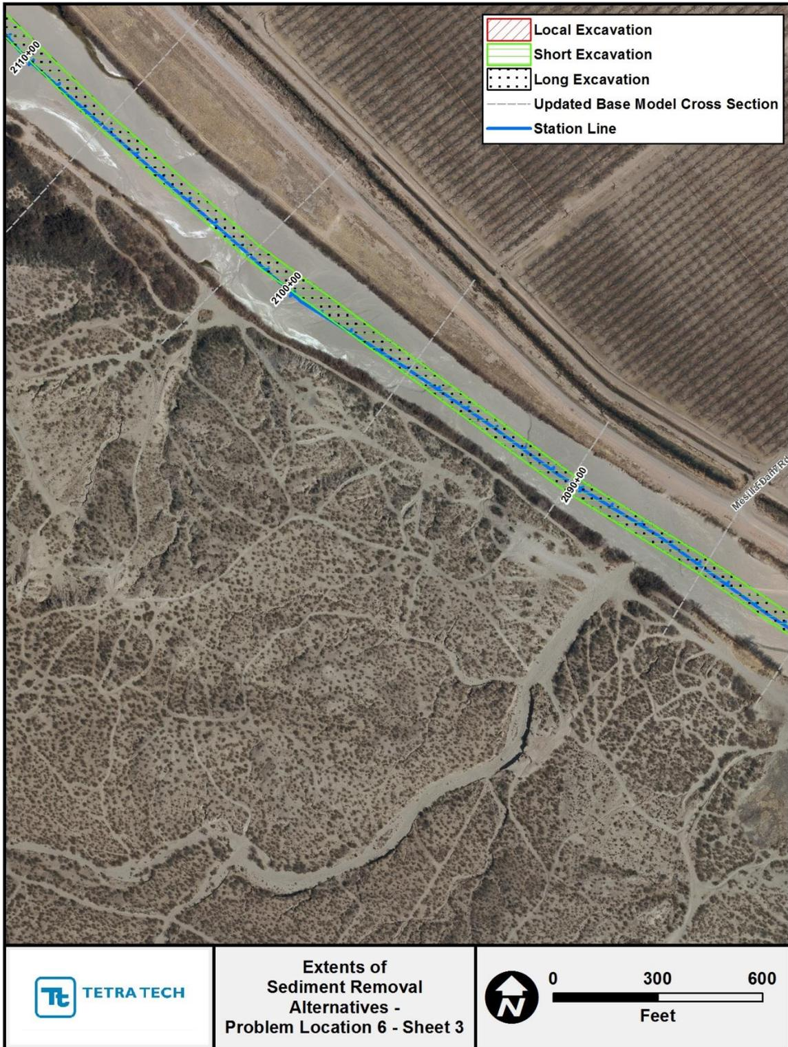
Figure G.2.22. Mapping showing extents of the localized, short and long sediment-removal alternatives at Problem Location 6 (Sheet 3).
