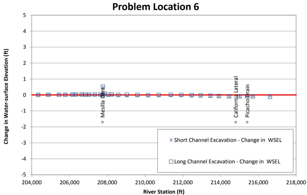
Figure N.22. Predicted change in long-term water-surface elevation at 2,350 cfs relative to the base condition at Problem Location 6 for the alternatives that were evaluated with the steady-state hydraulic model compared to existing (base model) conditions.
