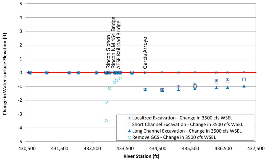
Figure L.22. Predicted change in water-surface elevation at 3,500 cfs at Problem Location 3 for the alternatives that were evaluated with the steady-state hydraulic model compared to existing (base model) conditions.
