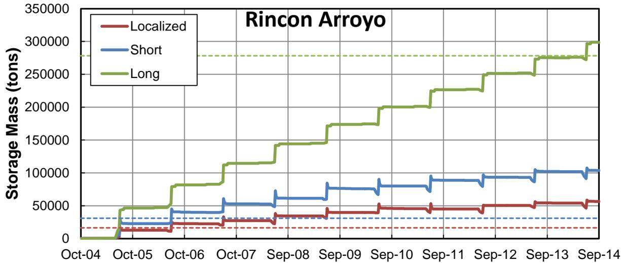
Figure M.2.25. Predicted cumulative mass of aggradation or degradation over time along the extents of the excavated reaches at Rincon Arroyo (Problem Location 4) from the sediment-transport simulations of the sediment-removal alternatives. The dashed lines represent the excavated mass for each type of excavation.
