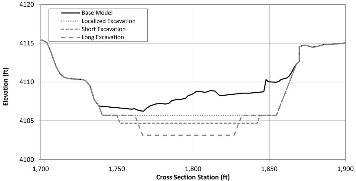
Figure G.1.4. Typical cross section at Problem Location 1 showing the existing (Base Model) channel geometry and excavated geometry under the localized, short and long excavation scenarios (River Station 518915).
