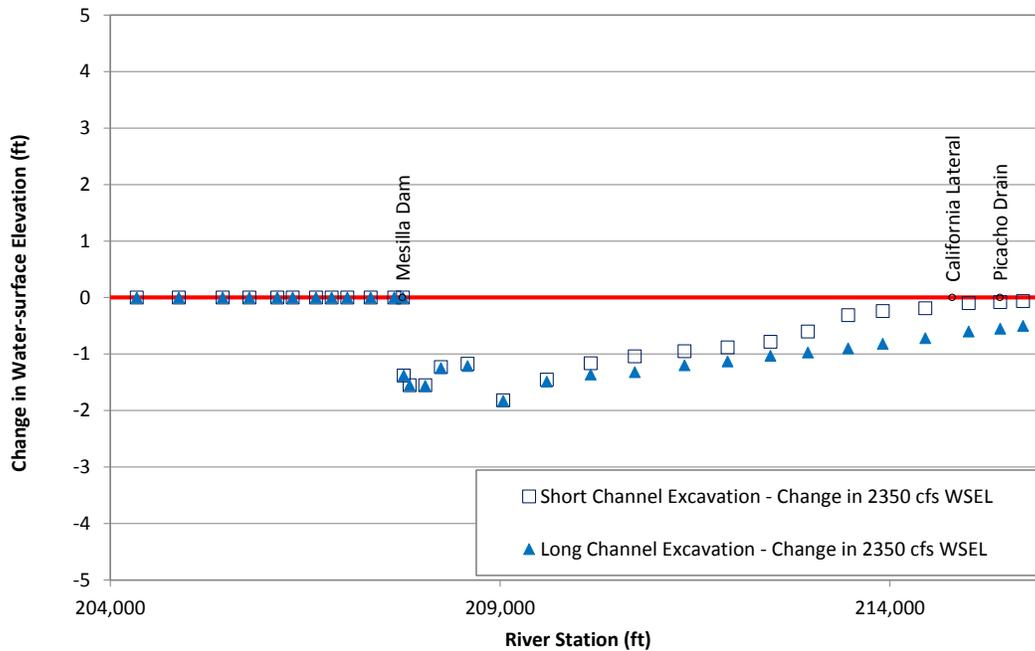
Figure L.42. Predicted change in water-surface elevation at 2,350 cfs at Problem Location 6 for the alternatives that were evaluated with the steady-state hydraulic model compared to existing (base model) conditions.
