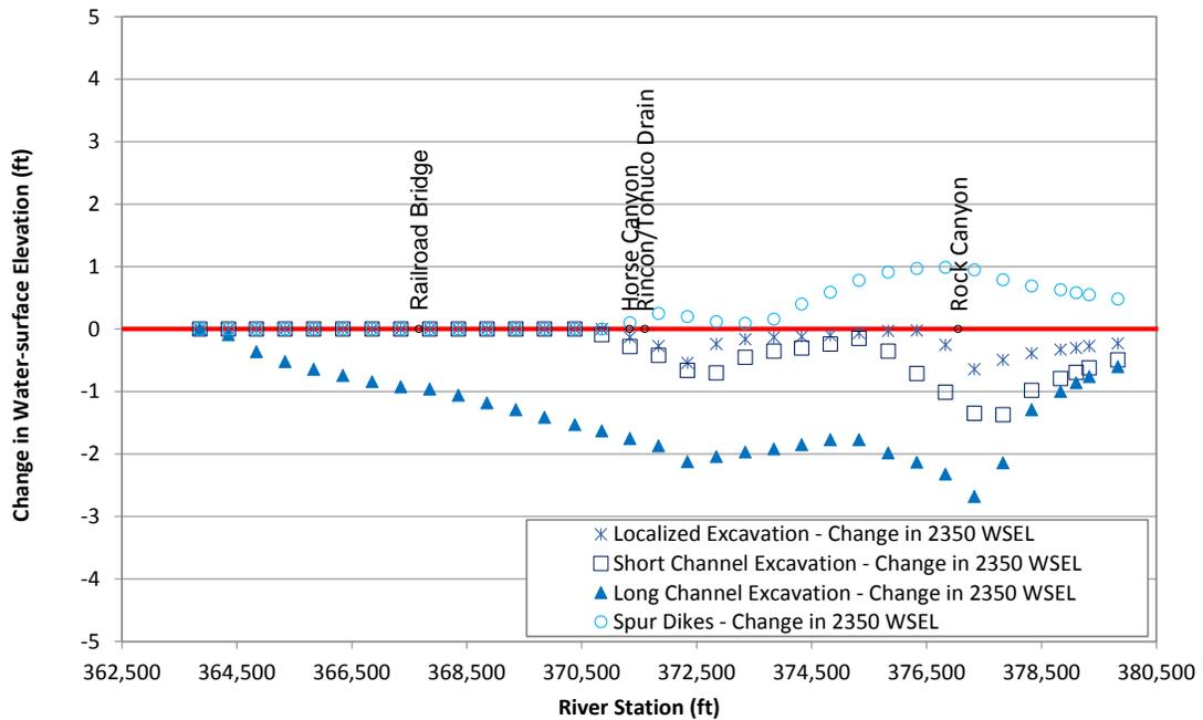
Figure L.34. Predicted change in water-surface elevation at 2,350 cfs at Problem Location 5 for the alternatives that were evaluated with the steady-state hydraulic model compared to existing (base model) conditions.
