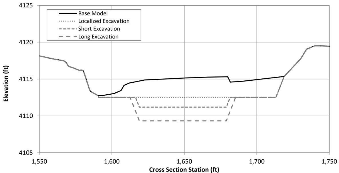
Figure G.1.2. Typical cross section at Problem Location 1 showing the existing (Base Model) channel geometry and excavated geometries under the localized, short and long excavation scenarios (River Station 527574.7).
