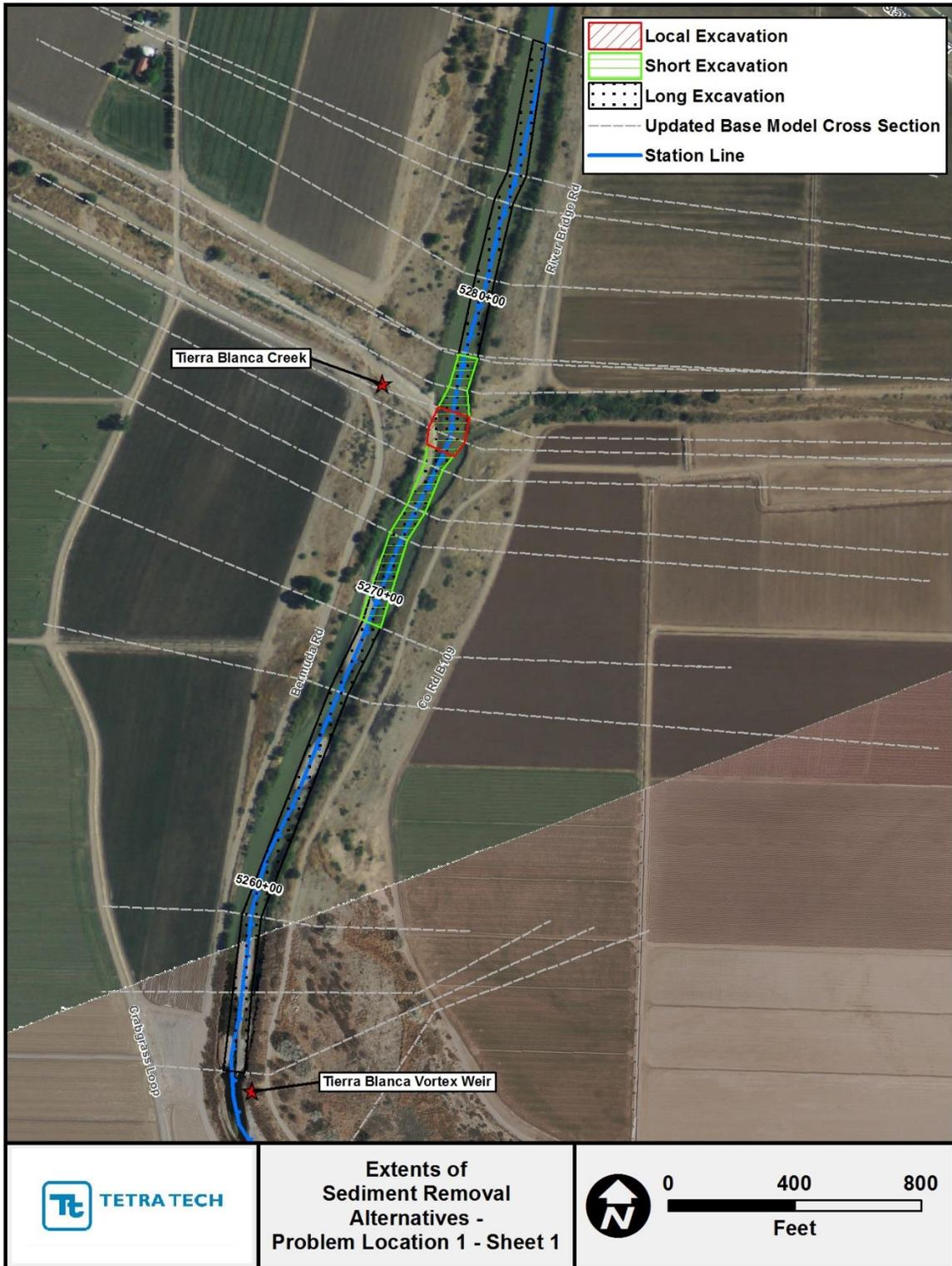
Figure G.2.1. Mapping showing extents of the localized, short and long sediment-removal alternatives at Problem Location 1 (Sheet 1).
