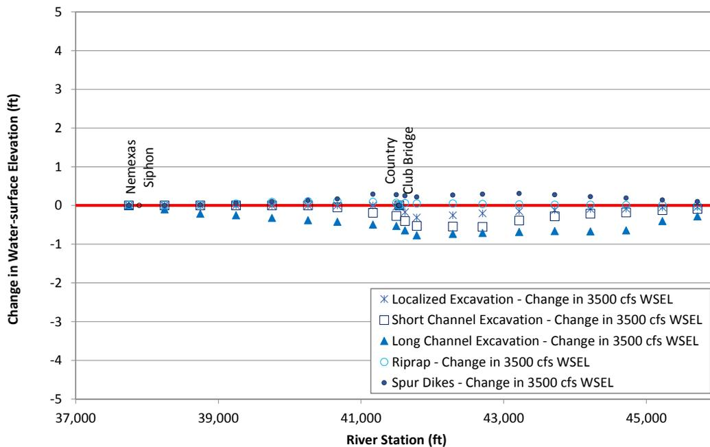
Figure L.62. Predicted change in water-surface elevation at 3,500 cfs at Problem Location 8 for the alternatives that were evaluated with the steady-state hydraulic model compared to existing (base model) conditions.
