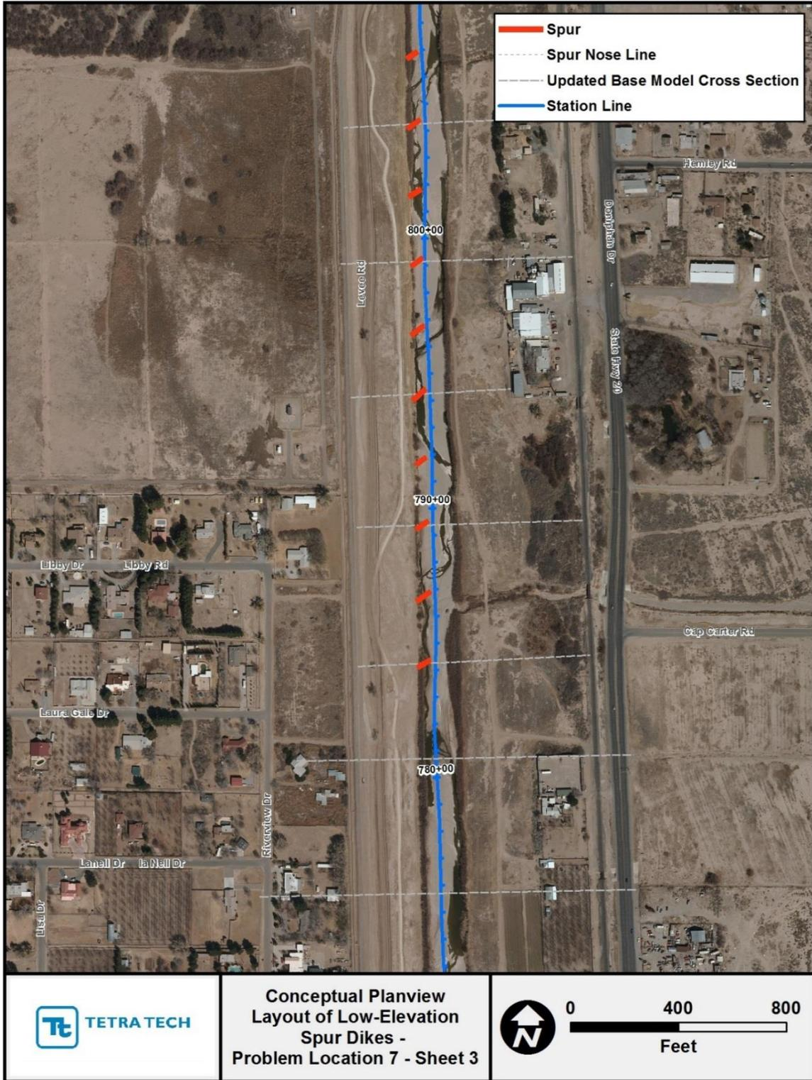
Figure I.8. Conceptual layout of low-elevation spur dikes at Problem Location 7 (Sheet 3).
