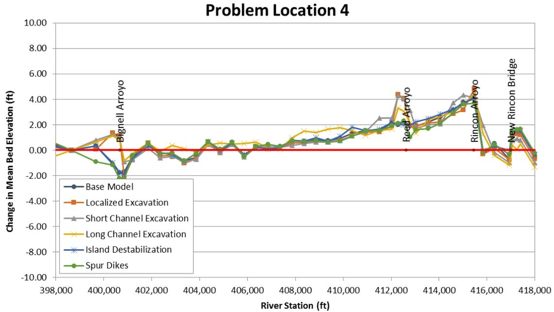
Figure M.1.13. Spatial profiles showing the predicted change in mean bed elevation at the end of the sediment-transport simulations for base alternative conditions at Problem Location 4.
