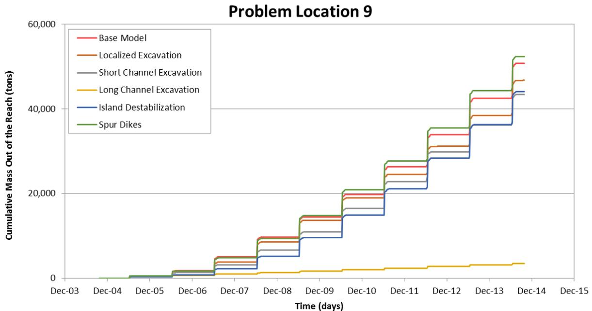
Figure M.2.18. Predicted cumulative mass delivered from the downstream of the model reach at Problem Location 9 from the sediment-transport simulations of the base and alternative conditions.
