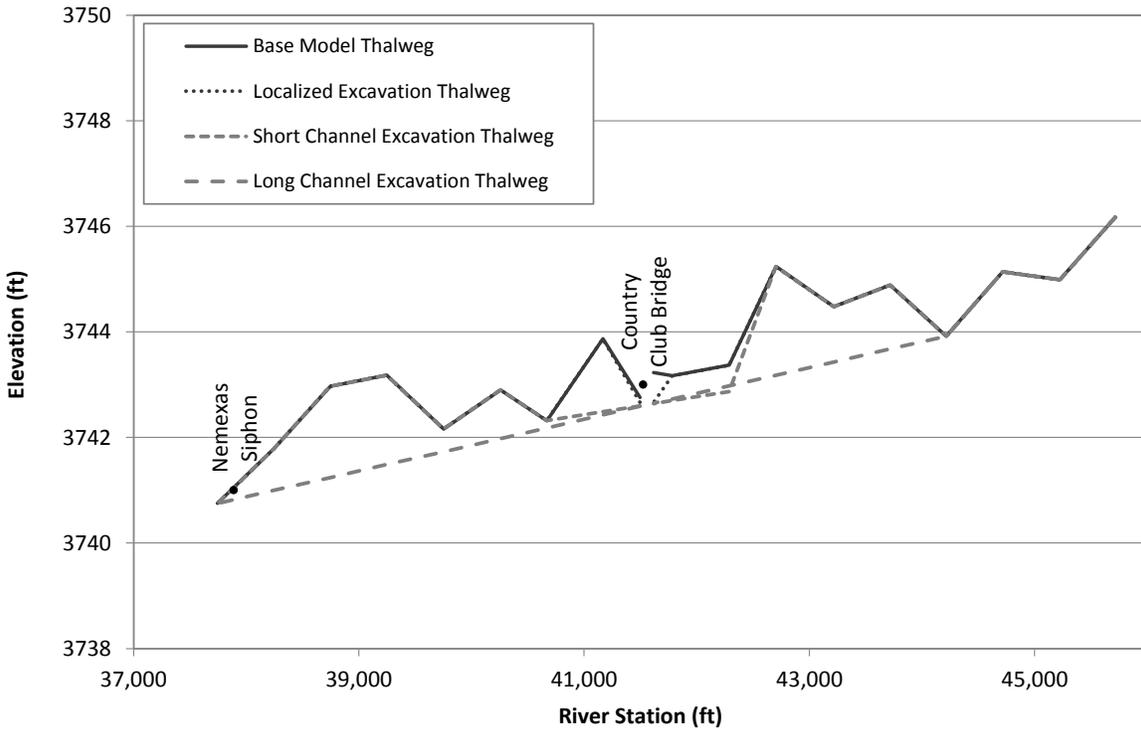
Figure G.1.33. Existing (Base Model) and excavation thalweg profiles at Problem Location 8.
