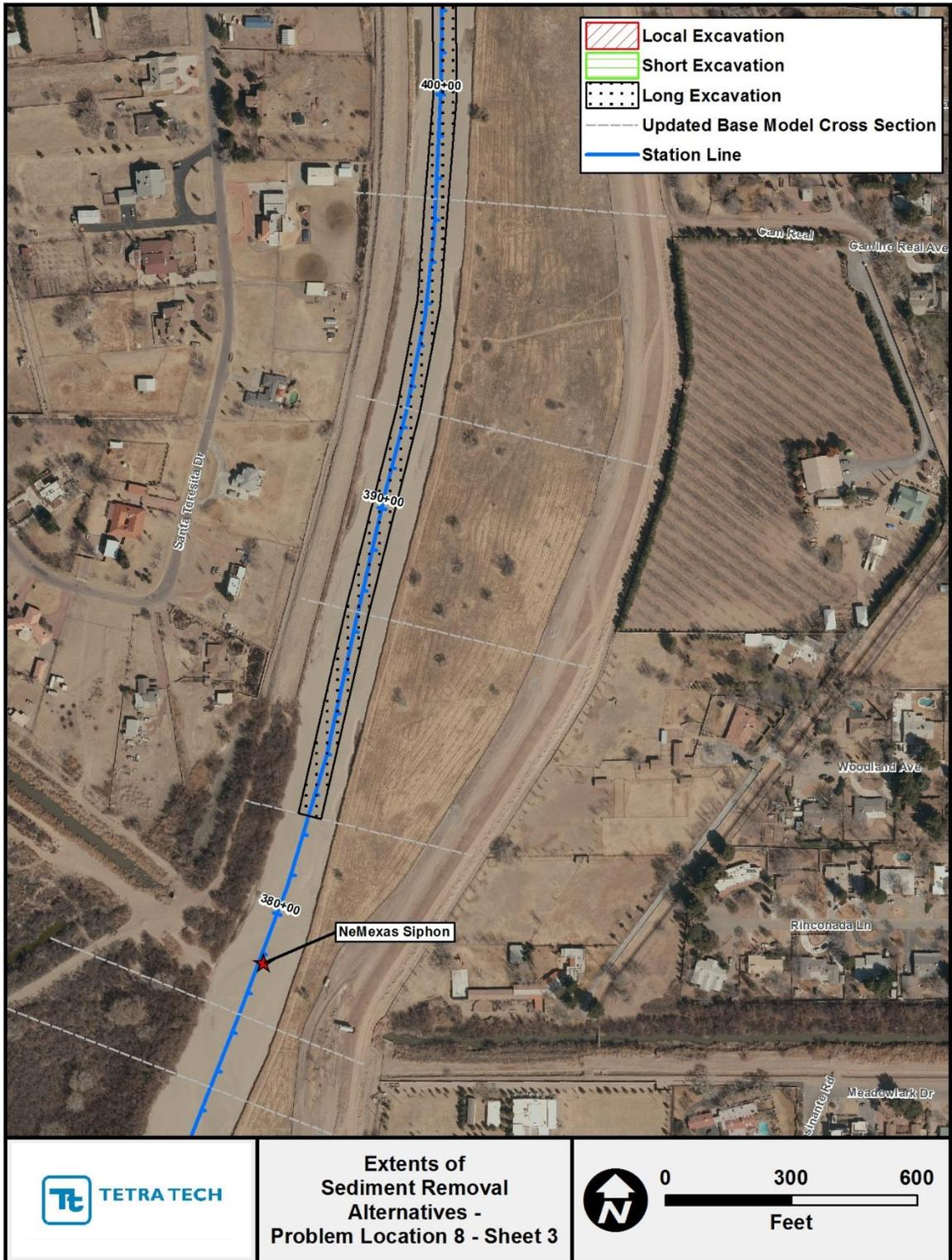
Figure G.2.30. Mapping showing extents of the localized, short and long sediment-removal alternatives at Problem Location 8 (Sheet 3).
