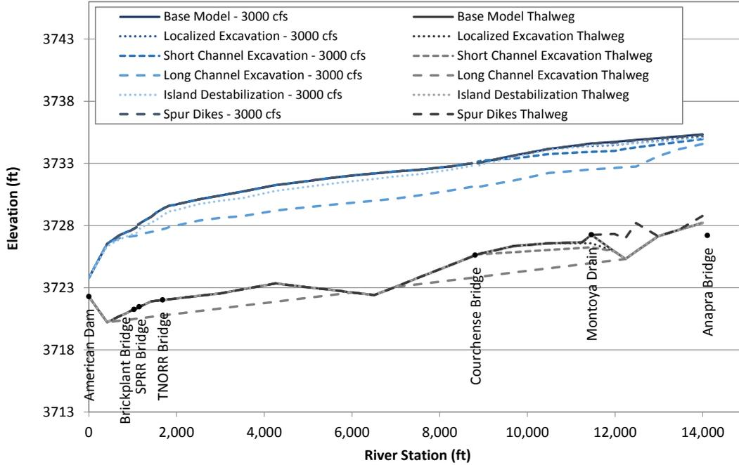
Figure L.67. Predicted water-surface profiles at 3,000 cfs at Problem Location 9 under existing (base model) conditions and for the alternatives that were evaluated with the steady-state hydraulic model.
