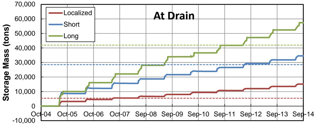
Figure M.2.31. Predicted cumulative mass of aggradation or degradation over time along the extents of the excavated reaches at the East Drain (Problem Location 7) from the sediment-transport simulations of the sediment-removal alternatives. The dashed lines represent the excavated mass for each type of excavation.
