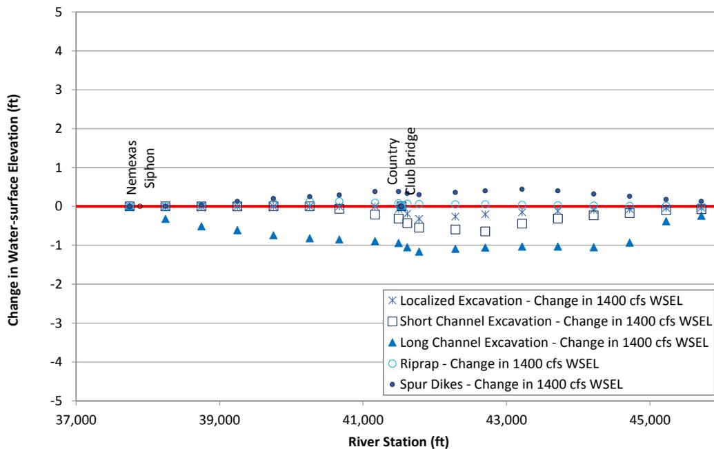
Figure L.58. Predicted change in water-surface elevation at 1,400 cfs at Problem Location 8 for the alternatives that were evaluated with the steady-state hydraulic model compared to existing (base model) conditions.
