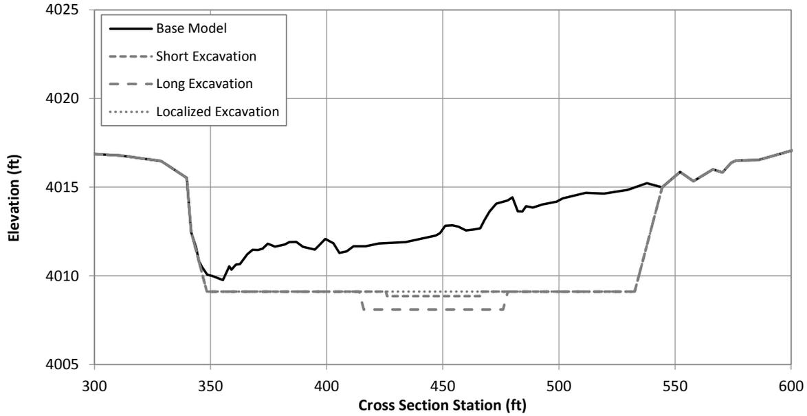
Figure G.1.19. Typical cross section at Problem Location 4 showing the existing (Base Model) channel geometry and excavated geometry under the localized, short and long excavation scenarios (River Station 400659.3).
