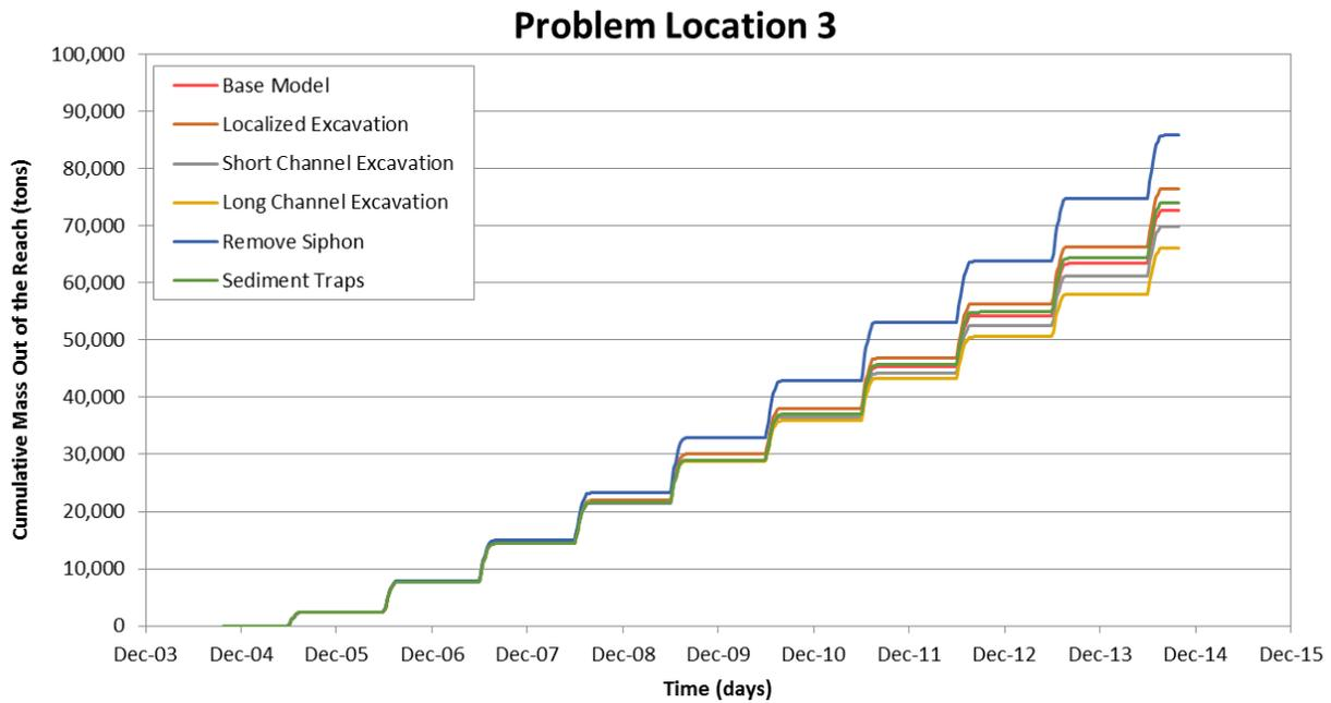
Figure M.2.12. Predicted cumulative mass delivered from the downstream of the model reach at Problem Location 3 from the sediment-transport simulations of the base and alternative conditions.
