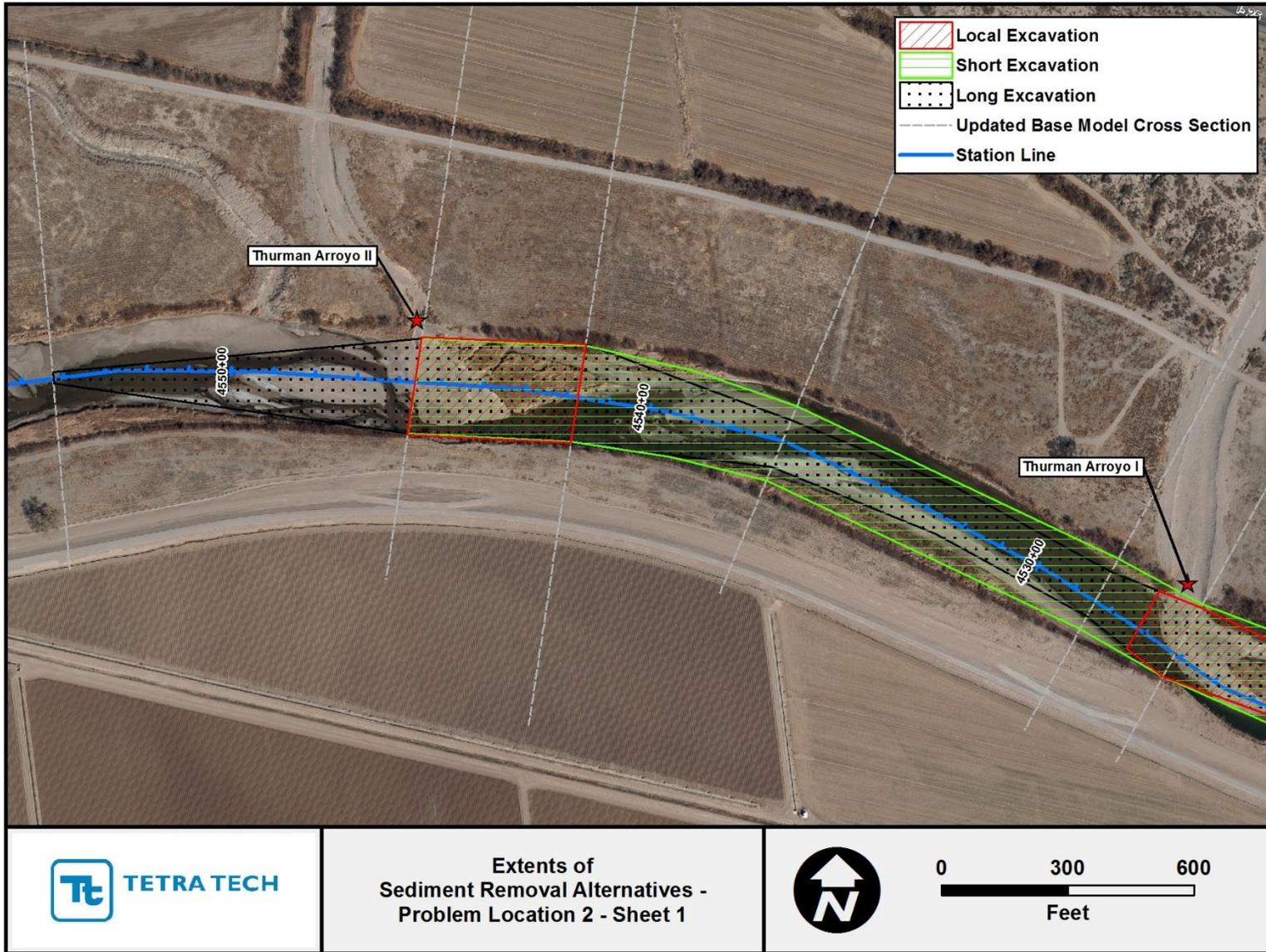
Figure G.2.3. Mapping showing extents of the localized, short and long sediment-removal alternatives at Problem Location 2 (Sheet 1).
