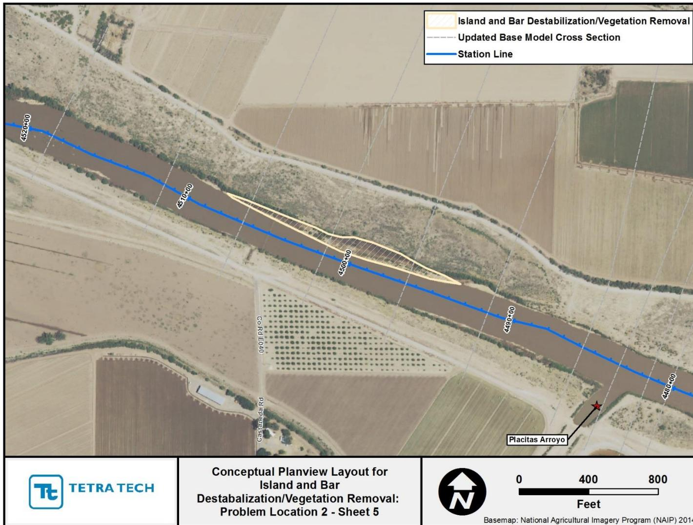
Figure J.5. Aerial photography showing extents of features treated with island/bar destabilization and vegetation removal at Problem Location 2 (Sheet 5).
