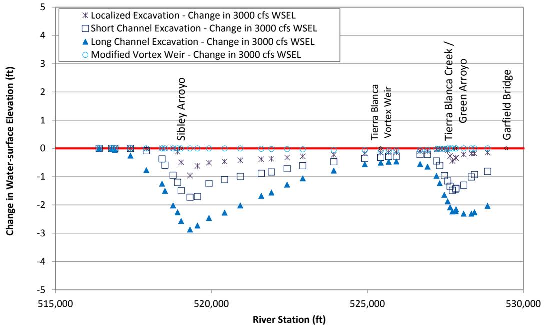
Figure L.4. Predicted change in water-surface elevation at 3,000 cfs at Problem Location 1 for the alternatives that were evaluated with the steady-state hydraulic model compared to existing (base model) conditions.
