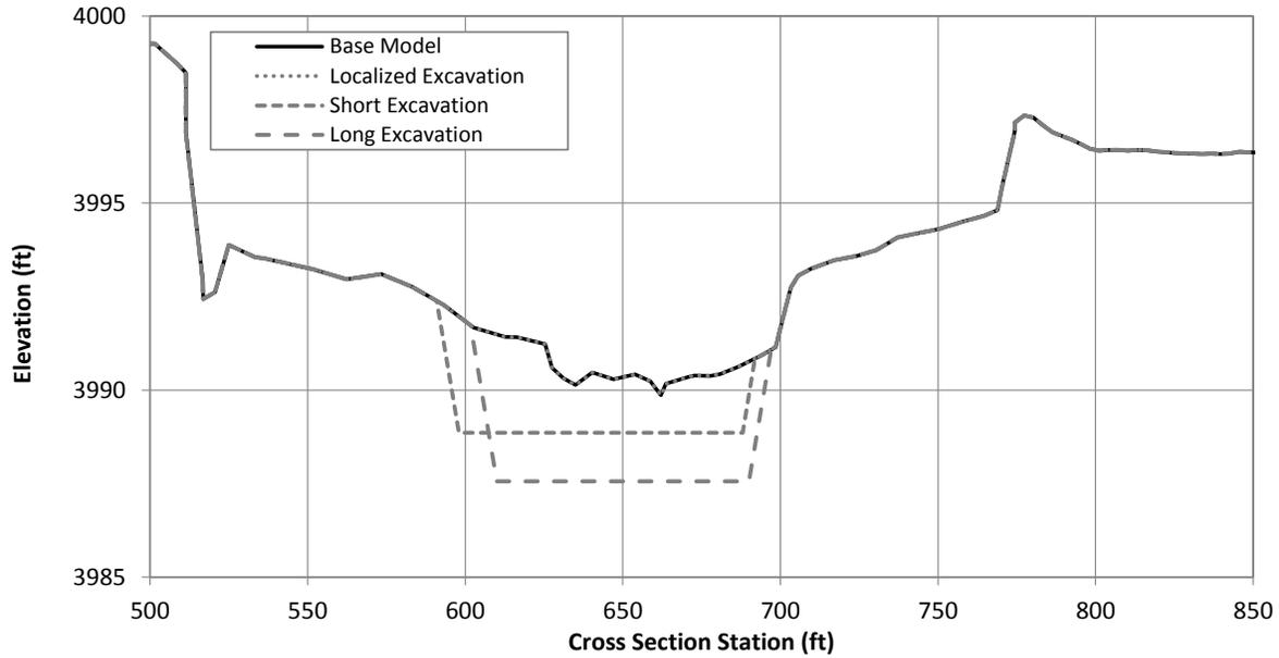
Figure G.1.23. Typical cross section at Problem Location 5 showing the existing (Base Model) channel geometry and excavated geometry under the localized, short and long excavation scenarios (River Station 372339.6).
