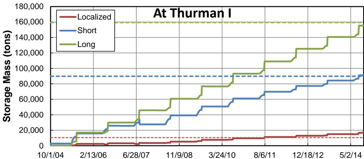
Figure M.2.22. Predicted cumulative mass of aggradation or degradation over time along the extents of the excavated reaches at Thurman I Arroyo (Problem Location 2) from the sediment-transport simulations of the sediment-removal alternatives. The dashed lines represent the excavated mass for each type of excavation.
