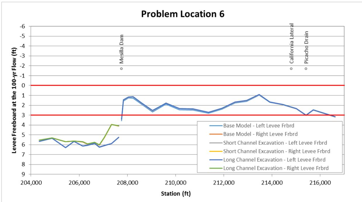
Figure O.4. Predicted levee freeboard during the 100-year flow at Problem Location 6 representing long-term conditions based on hydraulic modeling with the predicted geometry at the end of the sediment-transport simulations of the base and alternative conditions.
