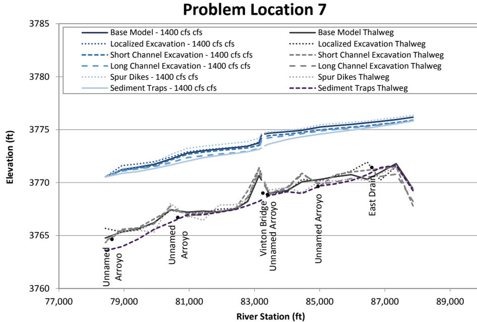
Figure N.25. Predicted water-surface profiles at 1,400 cfs at Problem Location 7 representing long-term conditions based on hydraulic modeling with the predicted geometry at the end of the sediment-transport simulations of the base and alternative conditions.
