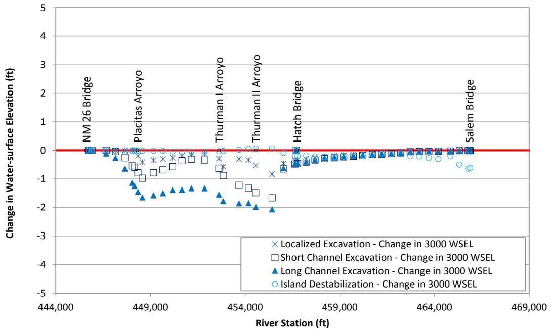
Figure L.12. Predicted change in water-surface elevation at 3,000 cfs at Problem Location 2 for the alternatives that were evaluated with the steady-state hydraulic model compared to existing (base model) conditions.
