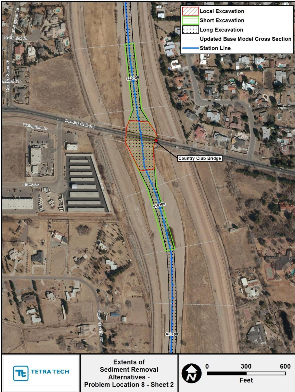
Figure G.2.29. Mapping showing extents of the localized, short and long sediment-removal alternatives at Problem Location 8 (Sheet 2).
