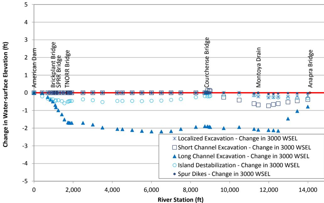
Figure L.68. Predicted change in water-surface elevation at 3,000 cfs at Problem Location 9 for the alternatives that were evaluated with the steady-state hydraulic model compared to existing (base model) conditions.
