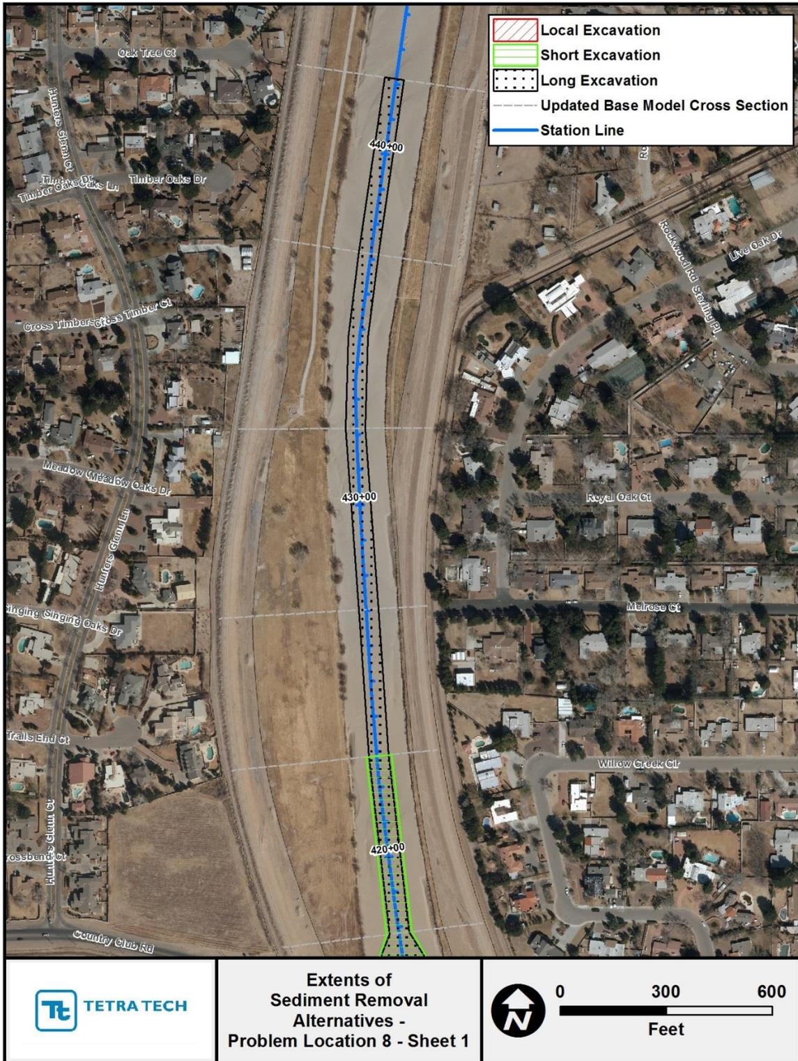
Figure G.2.28. Mapping showing extents of the localized, short and long sediment-removal alternatives at Problem Location 8 (Sheet 1).
