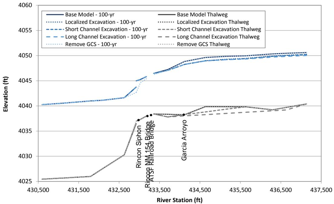
Figure L.23. Predicted water-surface profiles at the routed 100-year peak flow at Problem Location 3 under existing (base model) conditions and for the alternatives that were evaluated with the steady-state hydraulic model.
