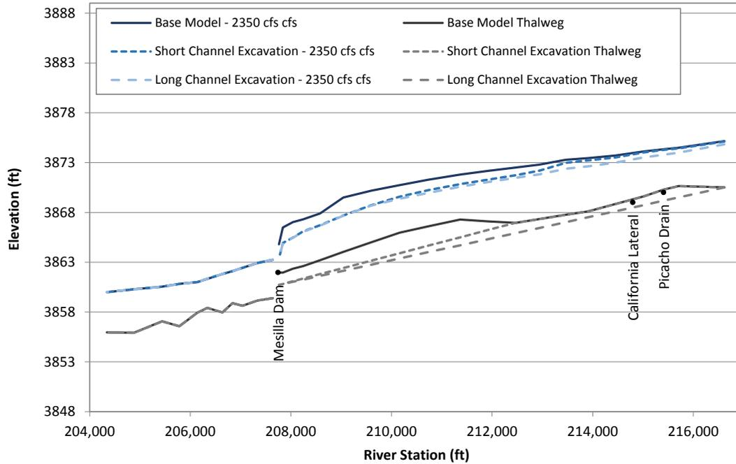
Figure L.41. Predicted water-surface profiles at 2,350 cfs at Problem Location 6 under existing (base model) conditions and for the alternatives that were evaluated with the steady-state hydraulic model.
