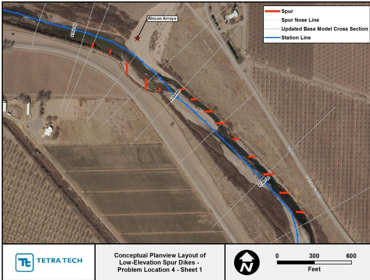
Figure I.1. Conceptual layout of low-elevation spur dikes at Problem Location 4 (Sheet 1).
