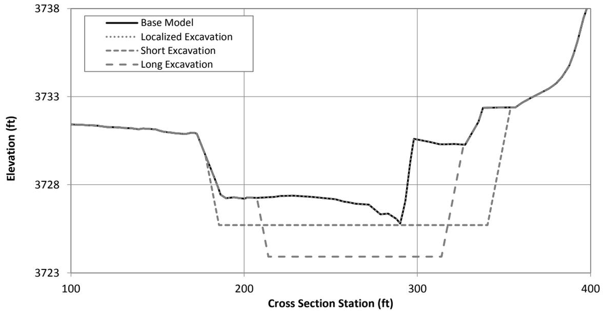
Figure G.1.40. Typical cross section at Problem Location 9 showing the existing (Base Model) channel geometry and excavated geometry under the localized, short and long excavation scenarios (River Station 9006.36).
