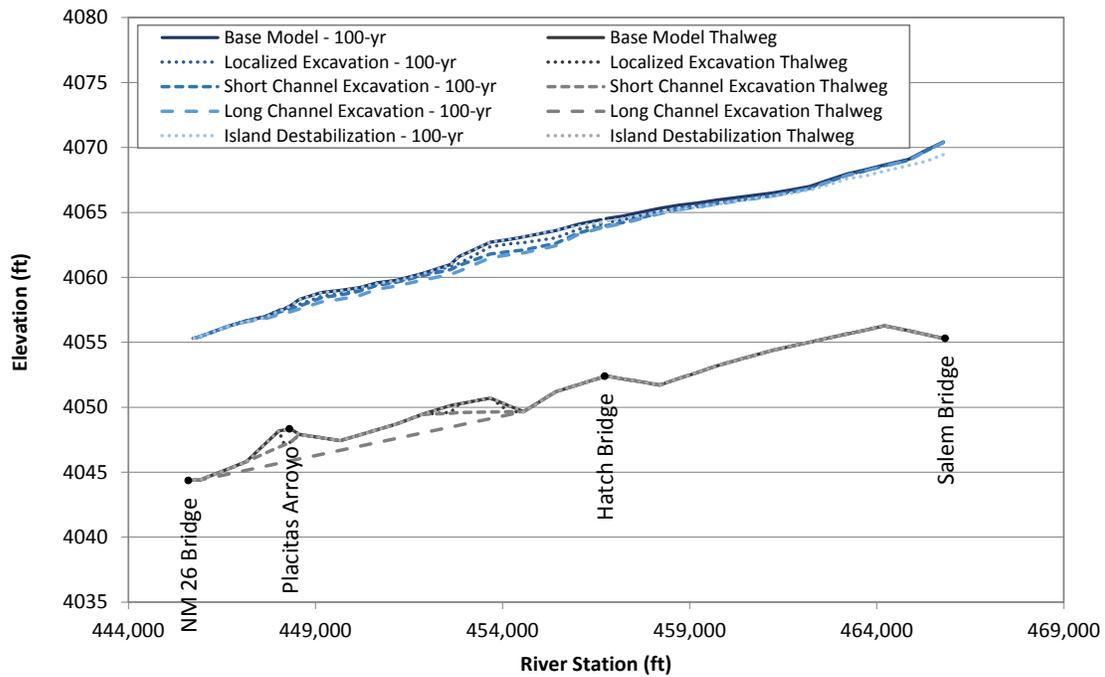
Figure L.15. Predicted water-surface profiles at the routed 100-year peak flow at Problem Location 2 under existing (base model) conditions and for the alternatives that were evaluated with the steady-state hydraulic model.
