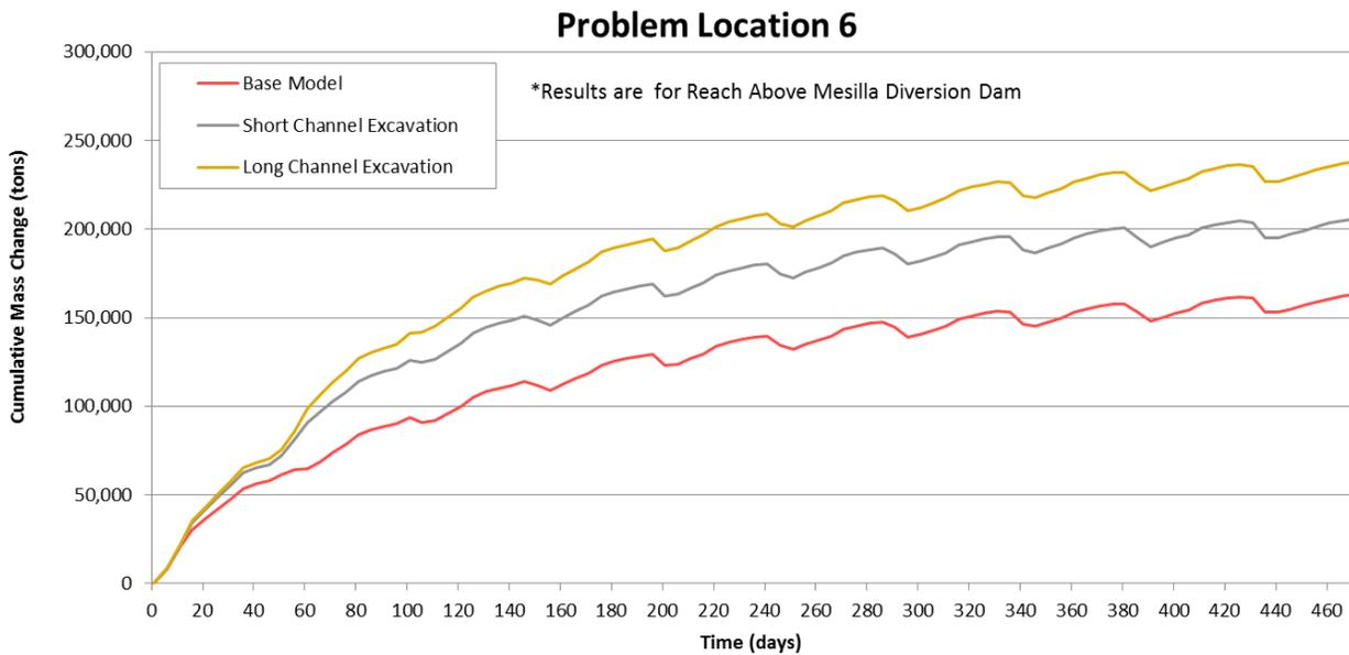
Figure M.2.6. Predicted cumulative mass of aggradation or degradation over time along the modeled reach at Problem Location 6 from the sediment-transport simulations of the base and alternative conditions.
