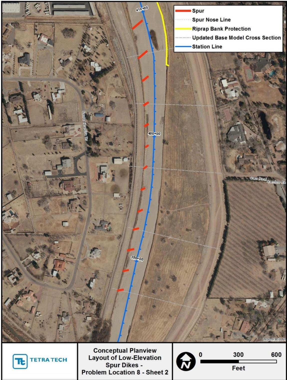
Figure I.10. Conceptual layout of low-elevation spur dikes at Problem Location 8 (Sheet 2).
