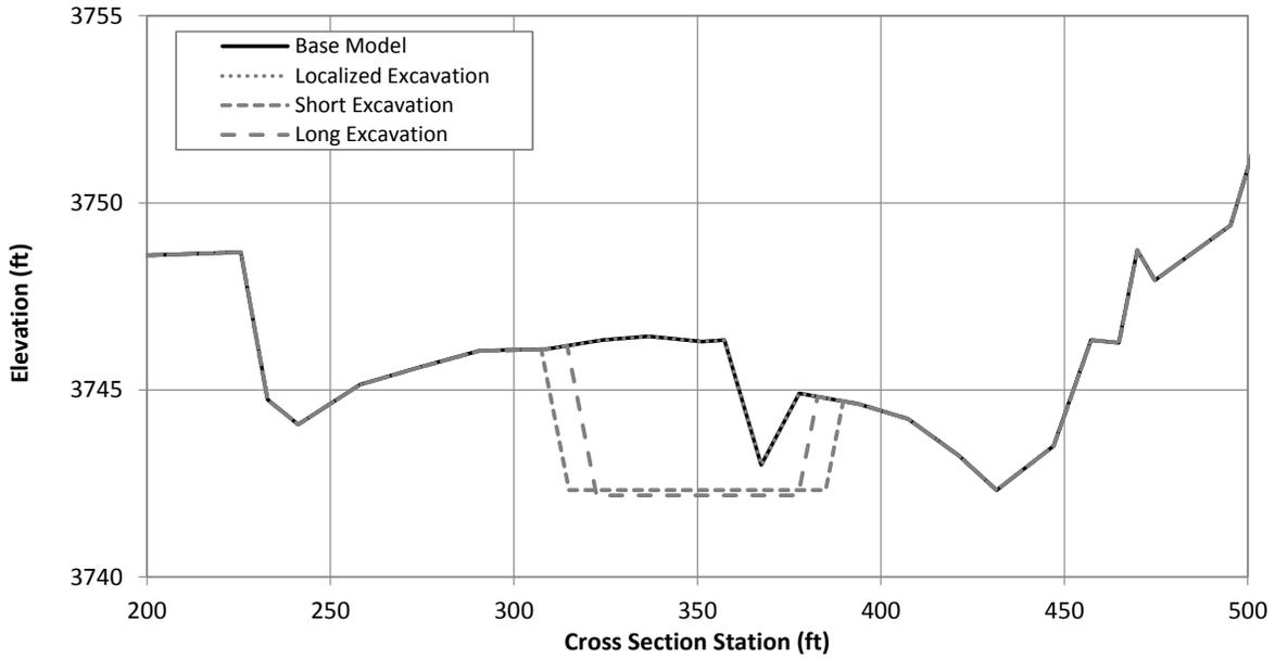
Figure G.1.36. Typical cross section at Problem Location 8 showing the existing (Base Model) channel geometry and excavated geometry under the localized, short and long excavation scenarios (River Station 40669.1).
