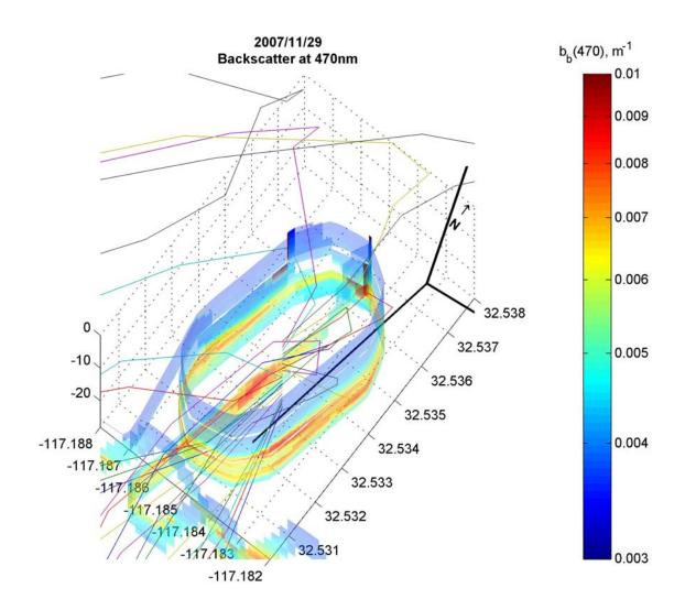
Near-field backscatter measurements at 470nm show good correspondence between elevated values (>0.006 m<sup>-1</sup>) and the estimated plume trajectory indicating elevated turbidity associated with the effluent.
