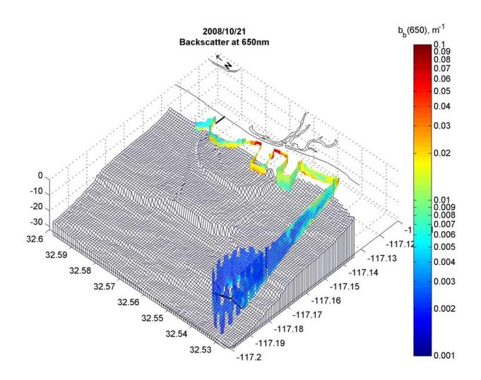
Backscatter measurements at 650 nm shows elevated values (>0.02 m<sup>-1</sup>) near the Tijuana River mouth indicating exchange with the estuary during periods of no flow.
