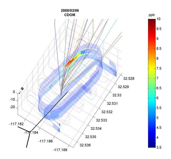
Near-field CDOM measurements shows good correspondence between elevated values (> 7 ppb) and the estimated plume trajectory.
