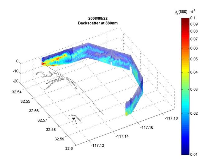
Backscatter measurements at 650 nm shows elevated values (>0.02 m<sup>-1</sup>) near the seafloor and just below the thermocline. Possible sources of elevated backscatter include sediment resuspension and phytoplankton.
