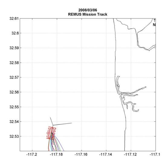
REMUS Mission track (red) and estimated SBOO plume trajectory (colored lines) based on near-realtime velocity profiles measured by the SBOO buoy.
