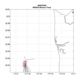
Figure A.4 REMUS Mission Tracks Southern Wye SBOO REMUS vehicle mission track (red) centered over the lower third of the southern wye of the SBOO (shown in black) for sampling conducted on March 6, 2008. Colored lines indicate the estimated plume trajectory based on SBOO buoy velocity profiles.
