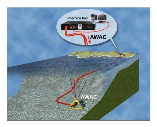
**Figure 13.** A concept drawing of the acoustic current meter / directional wave gauge that will be deployed from the Imperial Beach pier.
