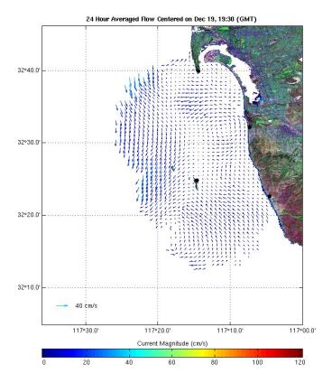
Figure 15. An example coverage map of observed surface currents. The radar locations are shown as black dots. This counter-clockwise eddy was observed on several occasions and can persist for anywhere between one and five days. One important feature of this eddy is the localized northward flow that brings water from the Tijuana Estuary to South Bay beaches. Ongoing studies will help determine the mechanisms that give rise to this eddy formation and provide a predictive capability to the region.
