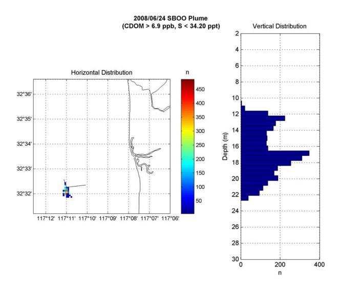
Horizontal and vertical plume distributions based on thresholding by the plumes' signature CDOM and salinity values. The number of samples satisfying the threshold criteria for a given horizontal or vertical bin is given by 'n'.
