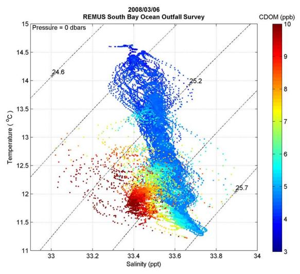
Temperature-Salinity (TS) diagram showing the distribution of watermasses by density (diagonal grid, units of kg/m<sup>3</sup> – 1000) and CDOM concentration. The outfall plume is distinguished as a fresher (lower salinity) watermass with high CDOM concentrations (> 6 ppb).
