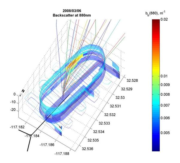
Near-field backscatter measurements at 880 nm shows good correspondence between elevated values (>0.01 m<sup>-1</sup>) and the estimated plume trajectory indicating elevated turbidity associated with the effluent.
