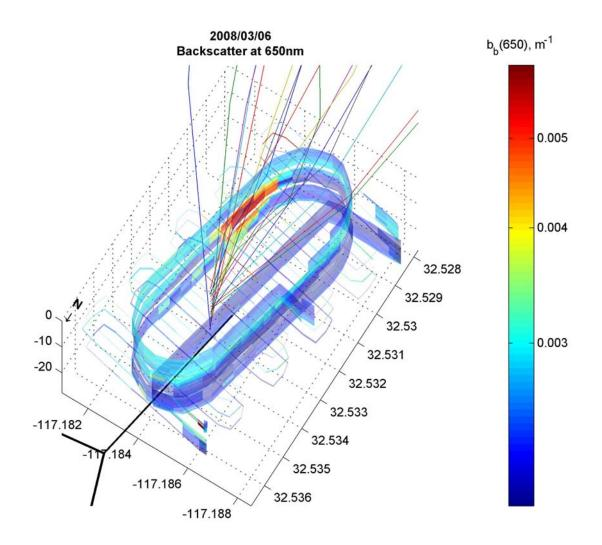
Near-field backscatter measurements at 650 nm shows good correspondence between elevated values (>0.004 m<sup>-1</sup>) and the estimated plume trajectory indicating elevated turbidity associated with the effluent.
