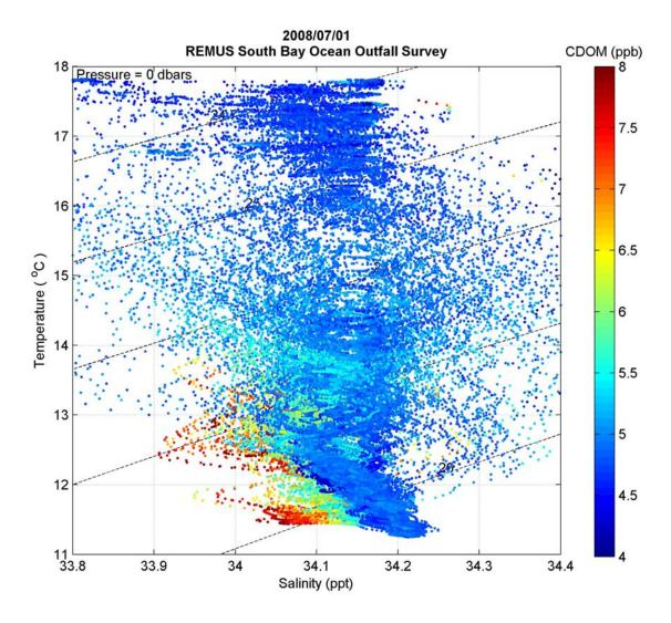
Temperature-Salinity (TS) diagram showing the distribution of watermasses by density (diagonal grid, units of  $kg/m^3 - 1000$ ) and CDOM concentration. The outfall plume is distinguished as a fresher (lower salinity) watermass with high CDOM concentrations (> 5.5 ppb).
