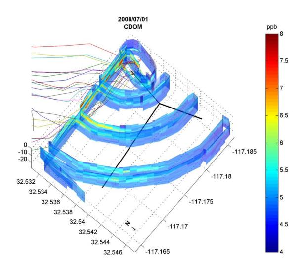
Elevated CDOM measurements (> 5.5 ppb) show good correspondence with the estimated SBOO plume trajectory (colored lines) based on near-realtime velocity profiles measured by the SBOO buoy.
