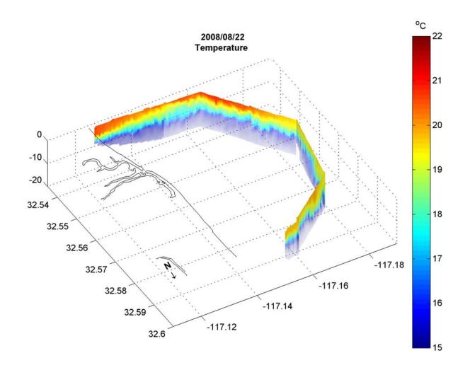
Temperature measurements show the water column is well stratified with surface values above 19 °C and deep water values of 15 °C.
