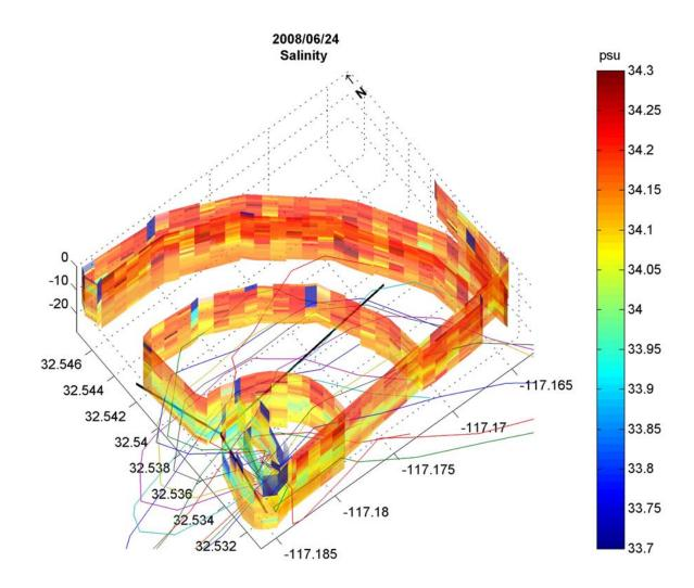
Salinity measurements shown with estimated SBOO plume trajectory (colored lines) based on near-realtime velocity profiles measured by the SBOO buoy. Low salinity near the outfall and eastward shows good agreement with the estimated trajectory.
