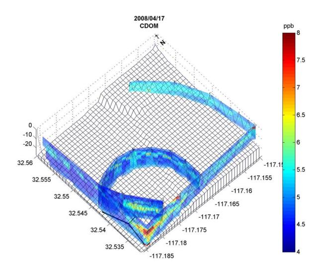
Elevated CDOM values (> 5 ppb) near the outfall toward the south indicate detection of the outfall plume. CDOM values of approximately 5.5 ppb in the northeast are within the kelp forest and are presumably due to elevated biological activity.
