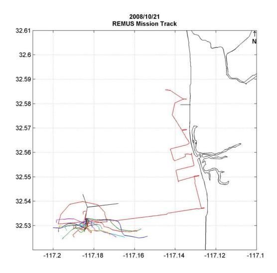
REMUS track (red) and estimated SBOO plume trajectory (colored lines) based on near-realtime velocity profiles measured by the SBOO buoy for a hybrid SBOO-Tijuana River mission.
