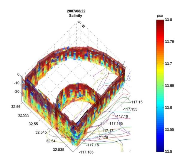
Salinity measurements shown with estimated SBOO plume trajectory (colored lines) based on near-realtime velocity profiles measured by the SBOO buoy. Noise at approximately 10m is due to transit across the thermocline. Low salinity near the outfall shows the SBOO plume rose quickly and may have surfaced.
