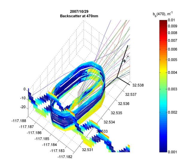
Near-field backscatter measurements at 470nm show good correspondence between elevated values (>0.003 m<sup>-1</sup>) and the estimated plume trajectory indicating elevated turbidity associated with the effluent.
