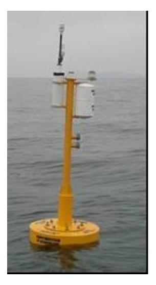
Figure D.2 Ocean Deployed Buoy Photograph of the deployed ocean buoy at the SBOO. The white cylinder on the right is a radar reflector and the cylinder on the left is a GPS tracking device.
