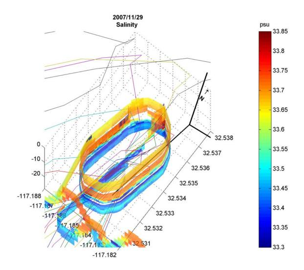
Salinity measurements shown with estimated SBOO plume trajectory (colored lines) based on near-realtime velocity profiles measured by the SBOO buoy. Low salinity at depth indicates the distribution of the SBOO plume.
