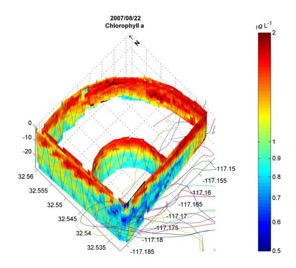
Chlorophyll a measurements shown with estimated SBOO plume trajectory (colored lines) based on near-realtime velocity profiles measured by the SBOO buoy. Correspondence between salinity and the estimated plume trajectory suggests that the SBOO plume is low in chlorophyll a ( $<0.7~\mu g L^{-1}$ ).
