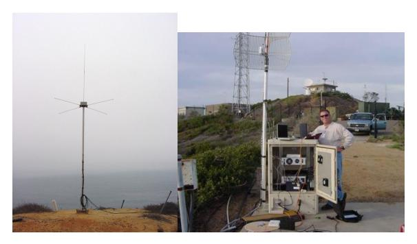
**Figure 14.** A surface current mapping HF radar antenna (left) and the electronics enclosure which houses the equipment. The photographs are from the tip of Point Loma.
