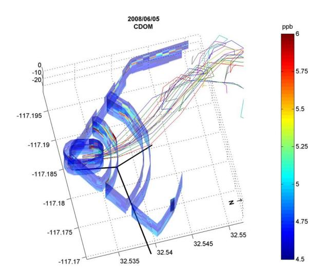
Elevated CDOM measurements (> 5 ppb) show good correspondence with estimated SBOO plume trajectory (colored lines) based on near-realtime velocity profiles measured by the SBOO buoy.
