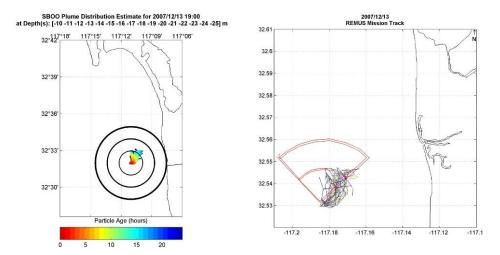
Figure A.2 SBOO Plume Trajectory (left) Near real-time SBOO plume trajectory estimate overall depths from the SBOO mooring indicating northerly flow. (right) SBOO REMUS mission programmed to capture plume signature.
