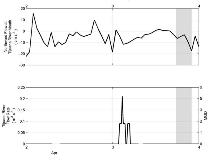
Alongshore surface current velocity measured by HF-Radar at the Tijuana River mouth (top) and flow rate from the Tijuana River as measured by the IBWC gauge (bottom). The grey panel indicates the sampling period.
