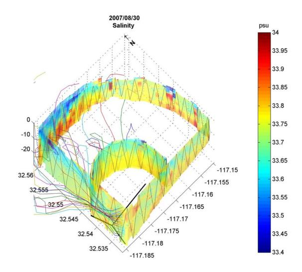
Salinity measurements shown with estimated SBOO plume trajectory (colored lines) based on near-realtime velocity profiles measured by the SBOO buoy. Low salinity near the outfall and northward shows the SBOO plume rising and surfacing.
