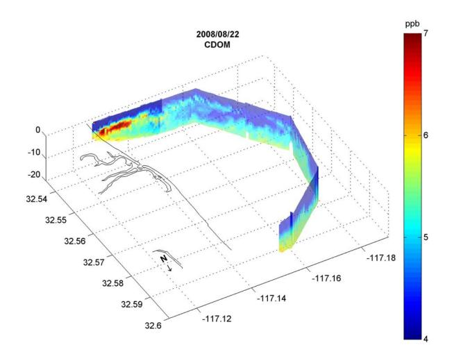
CDOM shows elevated values (> 5 ppb) near the seafloor and just below the thermocline. Possible sources of elevated CDOM include sediment resuspension and biological activity.
