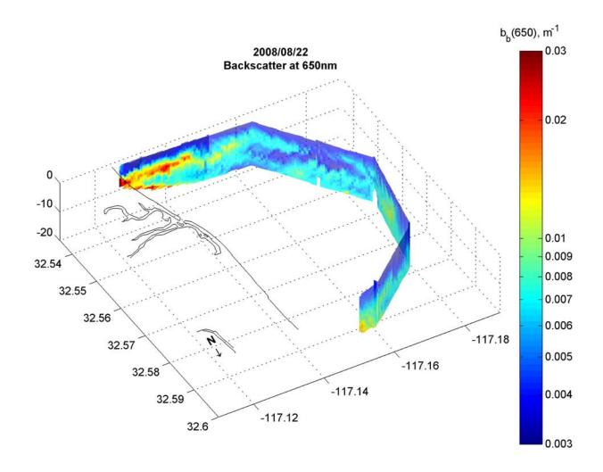
Backscatter measurements at 650 nm shows elevated values (>0.006 m<sup>-1</sup>) near the seafloor and just below the thermocline. Possible sources of elevated backscatter include sediment resuspension and phytoplankton.
