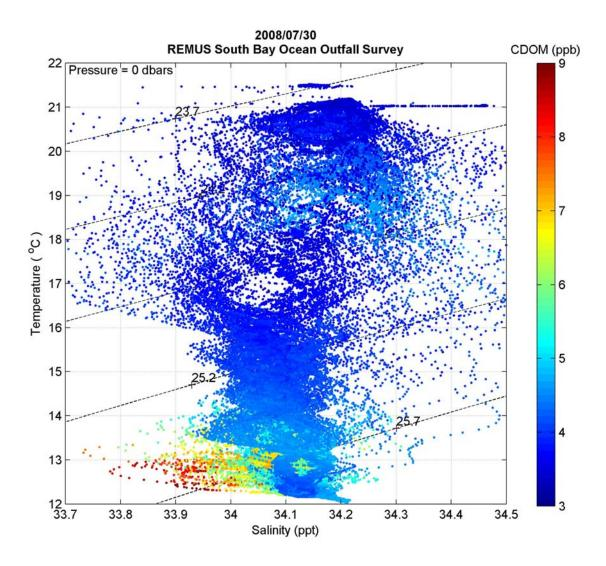
Temperature-Salinity (TS) diagram showing the distribution of watermasses by density (diagonal grid, units of kg/m<sup>3</sup> – 1000) and CDOM concentration. The outfall plume is distinguished as a fresher (lower salinity) watermass with high CDOM concentrations (> 5.5 ppb).
