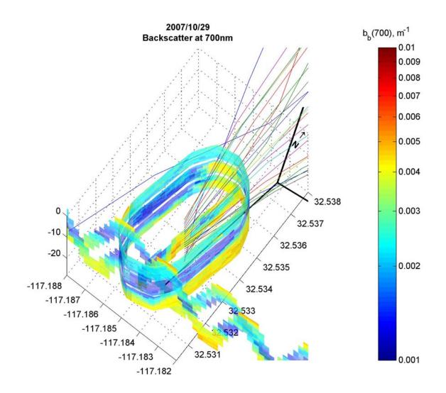
Near-field backscatter measurements at 700nm show good correspondence between elevated values (>0.004 m<sup>-1</sup>) and the estimated plume trajectory indicating elevated turbidity associated with the effluent.
