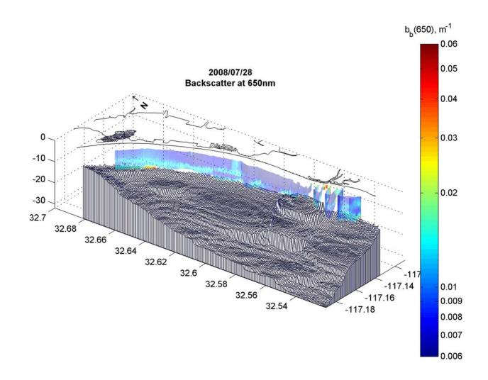
Backscatter measurements at 650 nm shows elevated values (>0.02 m<sup>-1</sup>) near the surface at the Tijuana River mouth indicating exchange with the estuary during periods of no flow. Elevated values (>0.01 m<sup>-1</sup>) near the seafloor may be due to sediment resuspension by currents scouring bottom sediment.
