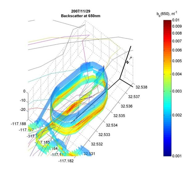
Near-field backscatter measurements at 650nm show good correspondence between elevated values (>0.004 m<sup>-1</sup>) and the estimated plume trajectory indicating elevated turbidity associated with the effluent.
