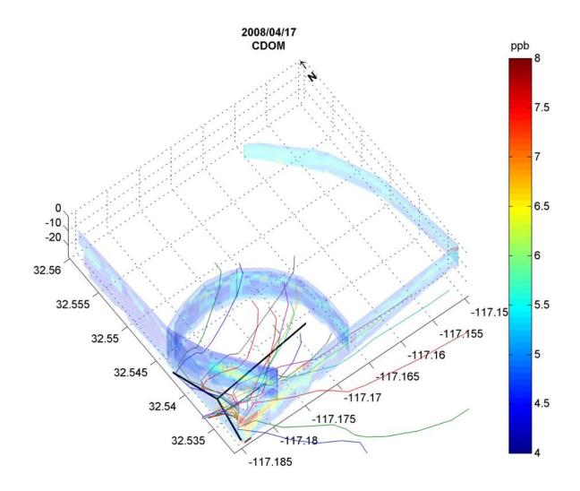
Correspondence between elevated CDOM measurements in the southwest over the outfall and estimated SBOO plume trajectory (colored lines) based on near-realtime velocity profiles measured by the SBOO buoy.
