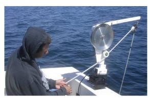
Figure B.2 Deploying Profiler (left) SIO staff deploying profiler during REMUS mission. (right) Profiler is lowered with controlled winch to improve data quality.
