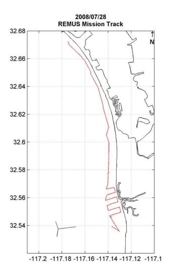
REMUS track (red) for a nearshore 'baseline' mission aimed at revealing background values for physical and optical parameters during dry weather and southward alongshore flow.
