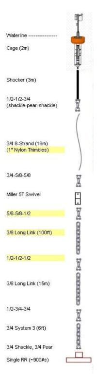
Figure D.3 SBOO Buoy Mooring Diagram
