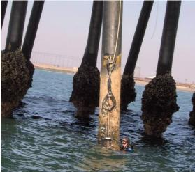
Figure D.4 Acoustic Wave and Current Profiler (left) Acoustic Wave and Current (AWAC) profiler installed offshore of the Imperial Beach Pier. (right) temperature chain deployed on a pier piling for ocean stratification measurements
