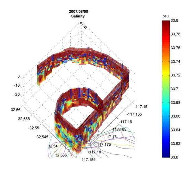
Salinity measurements shown with estimated SBOO plume trajectory (colored lines) based on near-realtime velocity profiles measured by the SBOO buoy. Noise at approximately 10m is due to transit across the thermocline. Low salinity (< 33.72 psu) near the outfall and around estimated trajectories indicate detection of the SBOO plume.
