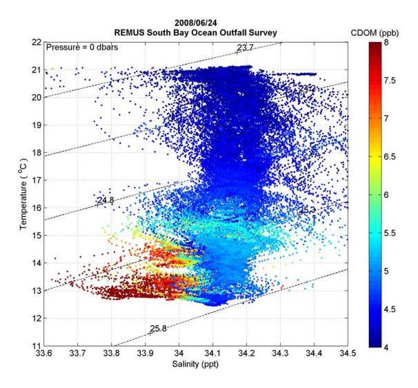
Temperature-Salinity (TS) diagram showing the distribution of watermasses by density (diagonal grid, units of kg/m³ – 1000) and CDOM concentration. The outfall plume is distinguished as a fresher (lower salinity) watermass with high CDOM concentrations (> 7 ppb).
