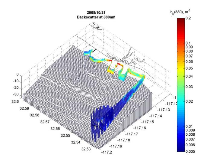
Backscatter measurements at 880 nm shows elevated values (>0.05 m<sup>-1</sup>) near the Tijuana River mouth indicating exchange with the estuary during periods of no flow.
