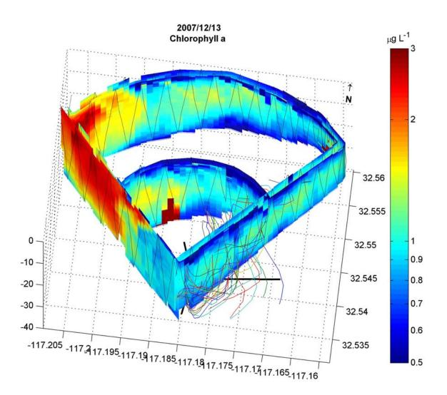
Chlorophyll a measurements shown with estimated SBOO plume trajectory (colored lines) based on near-realtime velocity profiles measured by the SBOO buoy. Correspondence between salinity and the estimated plume trajectory suggests that the SBOO plume is low in chlorophyll a (<0.7  $\mu$ g L<sup>-1</sup>).
