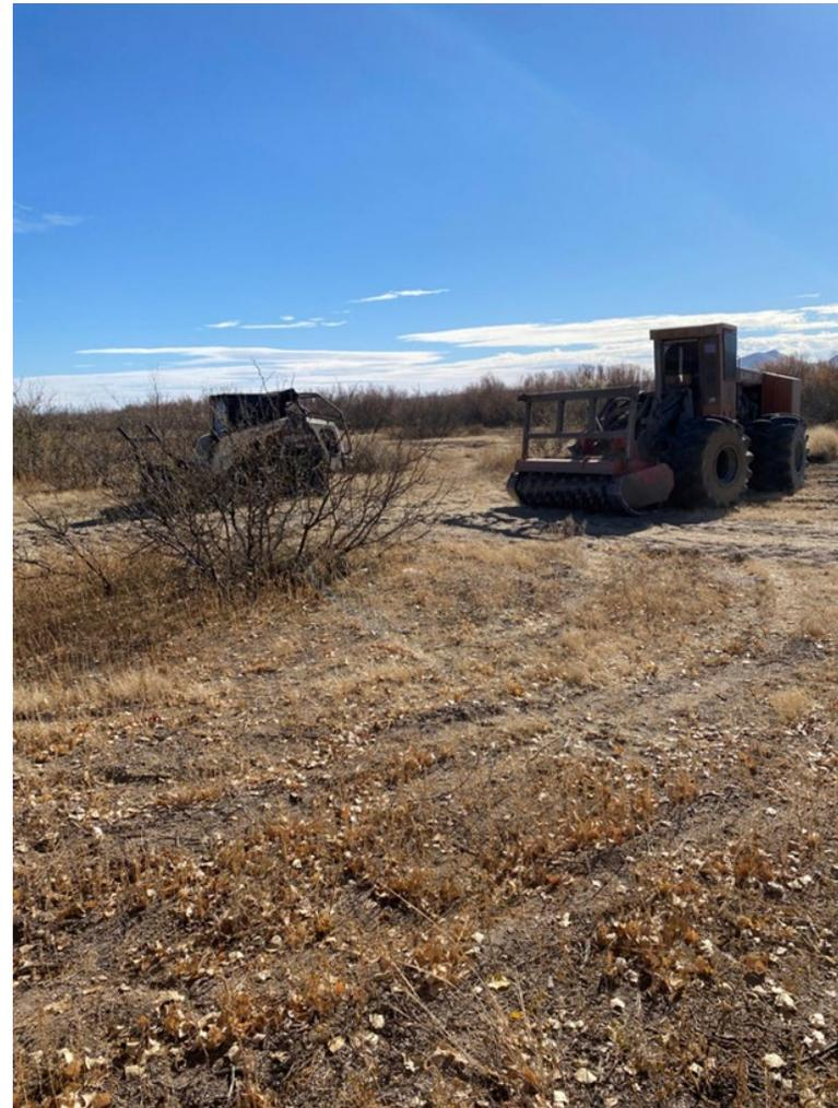
**Figure B-26. Barko 937 Mulcher and Terex R350T Skid Steer with Toshihog Mulching Head (Photo #164)**
