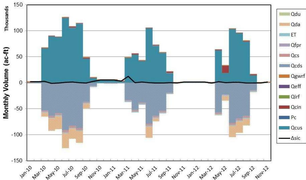
**Figure 14.** Stacked bar chart showing monthly volumes of the RGCP-scale channel water budget analysis and the resulting monthly change in-channel storage in Segment 1
