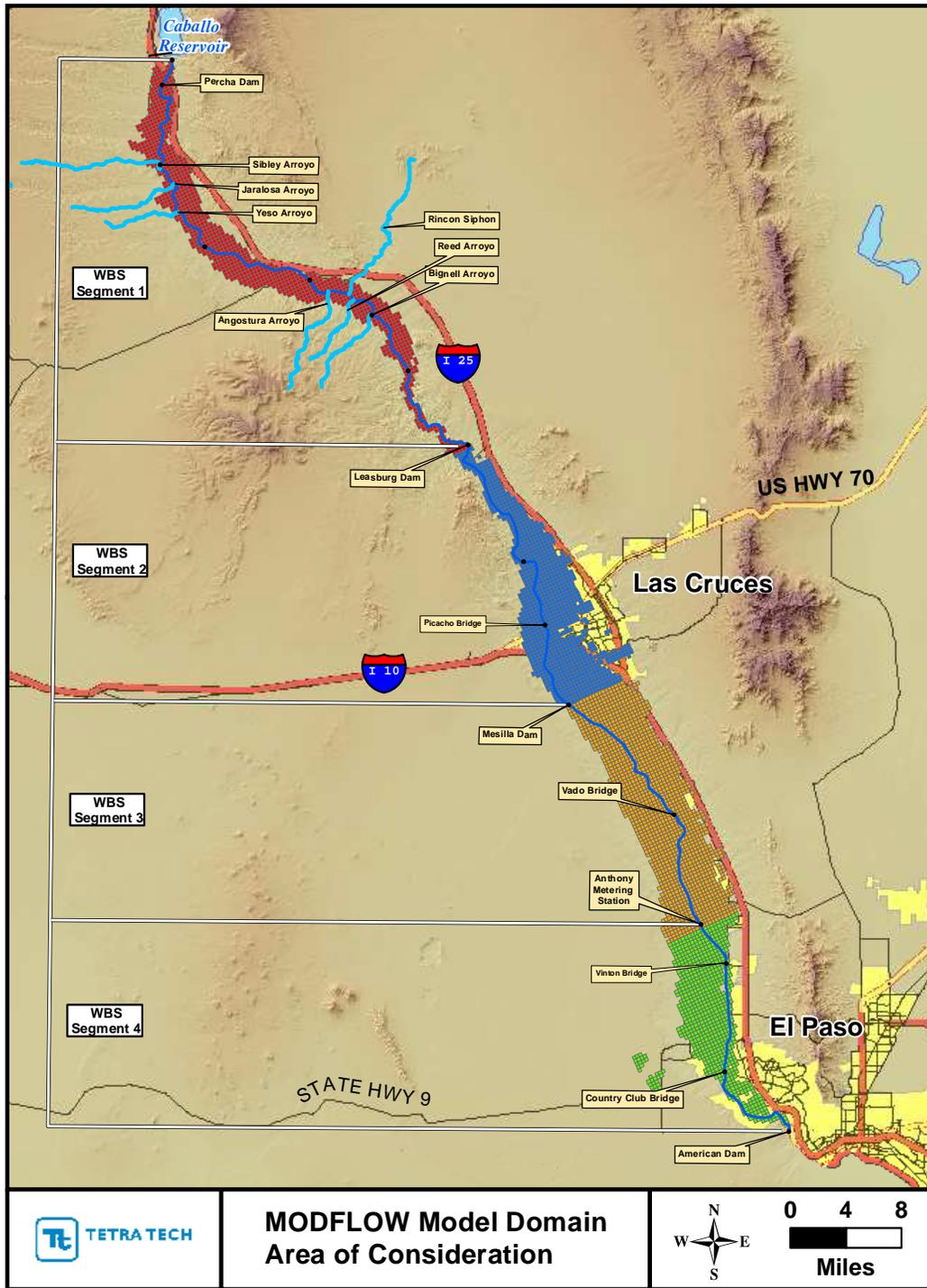
**Figure 12. Geographic zones representing the portion of the MODFLOW model domain that were used to extract groundwater fluxes from the model**
