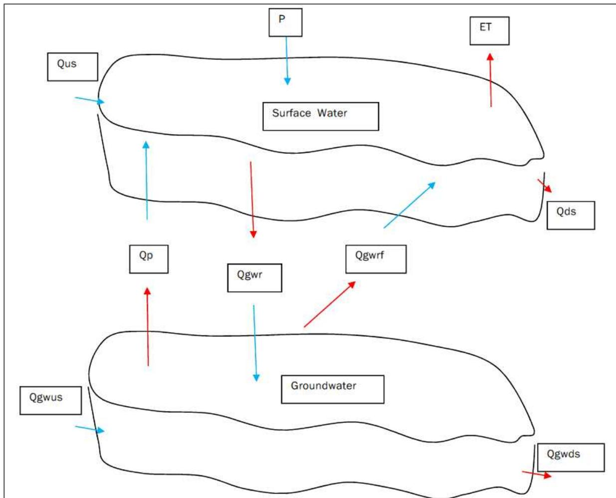
For a given time  $\Delta t$ , the equation for the surface water budget is:
