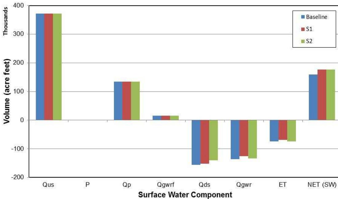
**Figure 31. Comparison of the local-basin-scale surface-water components under baseline (actual) conditions and under Scenarios S1 and S2**
