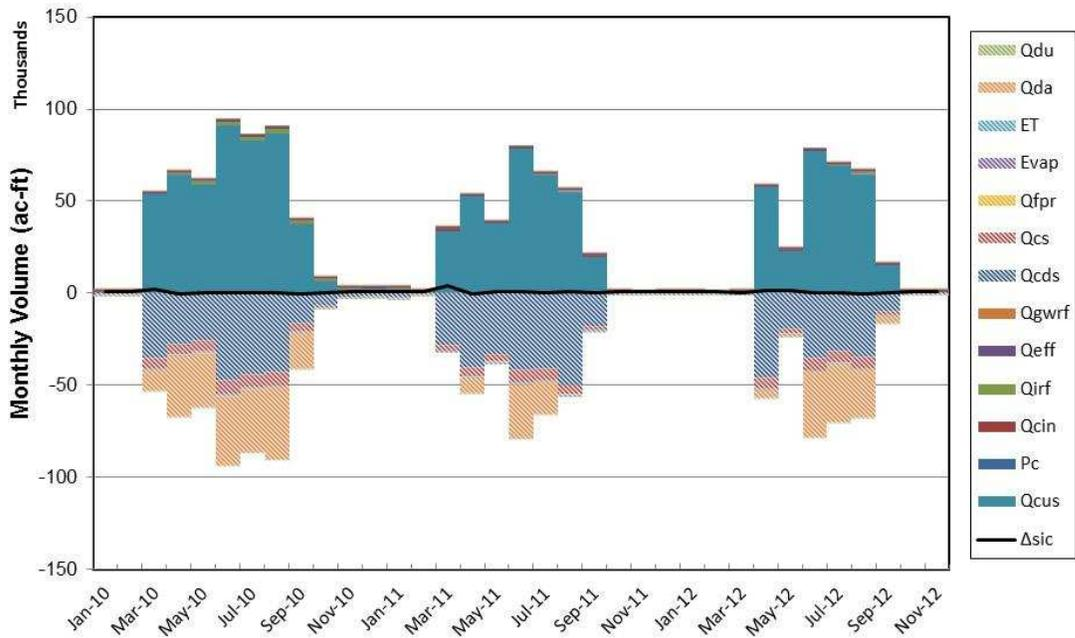
Figure 16. Stacked bar chart showing monthly volumes of the RGCP-scale channel water budget analysis and the resulting monthly change in-channel storage in Segment 2
