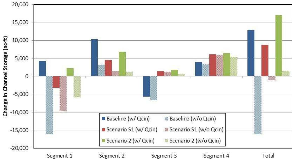
**Figure 28.** Total change in-channel storage with and without the  $Q_{cin}$  component at the end of the 2012 release under baseline (actual) conditions and under the hypothetical release scenarios (Scenarios S1 and S2)
